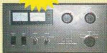
The TL-922A is an HF Linear amplifier designed to provide maximum legal power. By utilizing two 3-500Z high performance transmitting tubes, you'll have plenty of reserve power for those DX and contest contacts. Features include 2kw PEP output, 2 meters, variable ALC, delay cooling, class AB<sub>2</sub> bias and a look to match those Kenwood products.
