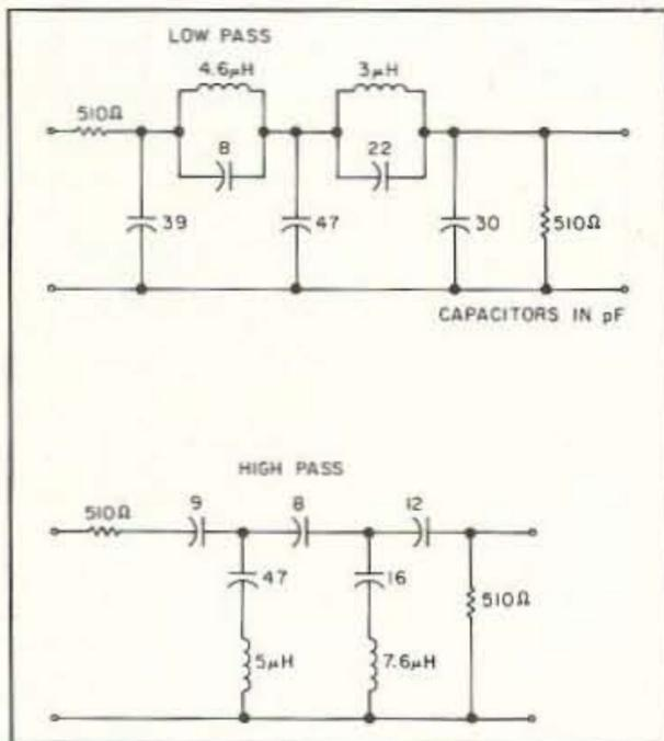
Figure 6. Filter schematics.
