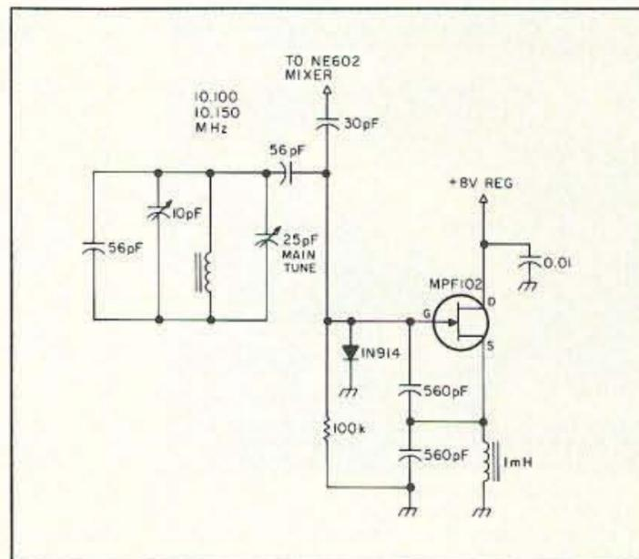
Figure. The oscillator from hell.
