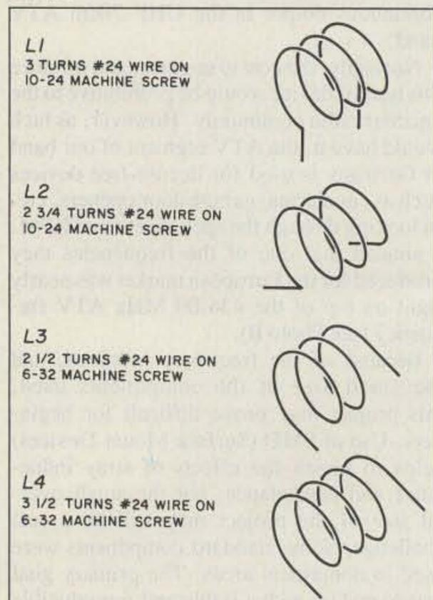
Figure 4. Coil winding details.
