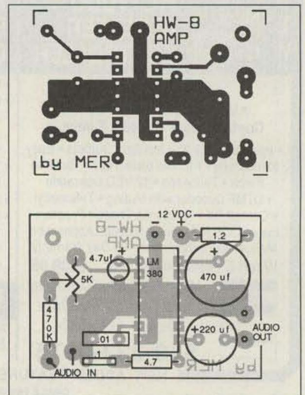
Figure 3. (a) PC board foil pattern for the audio amplifier. (b) Parts placement.
