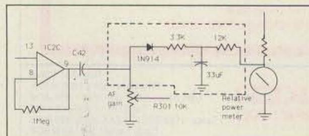
Figure 1. An S-meter for the HW-8.
