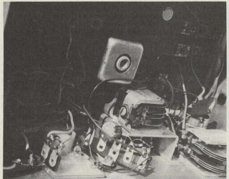
Photo C. Terminal strip holding the S-meter parts. The grain-of-wheat bulb is barely noticeable behind the meter's face.
