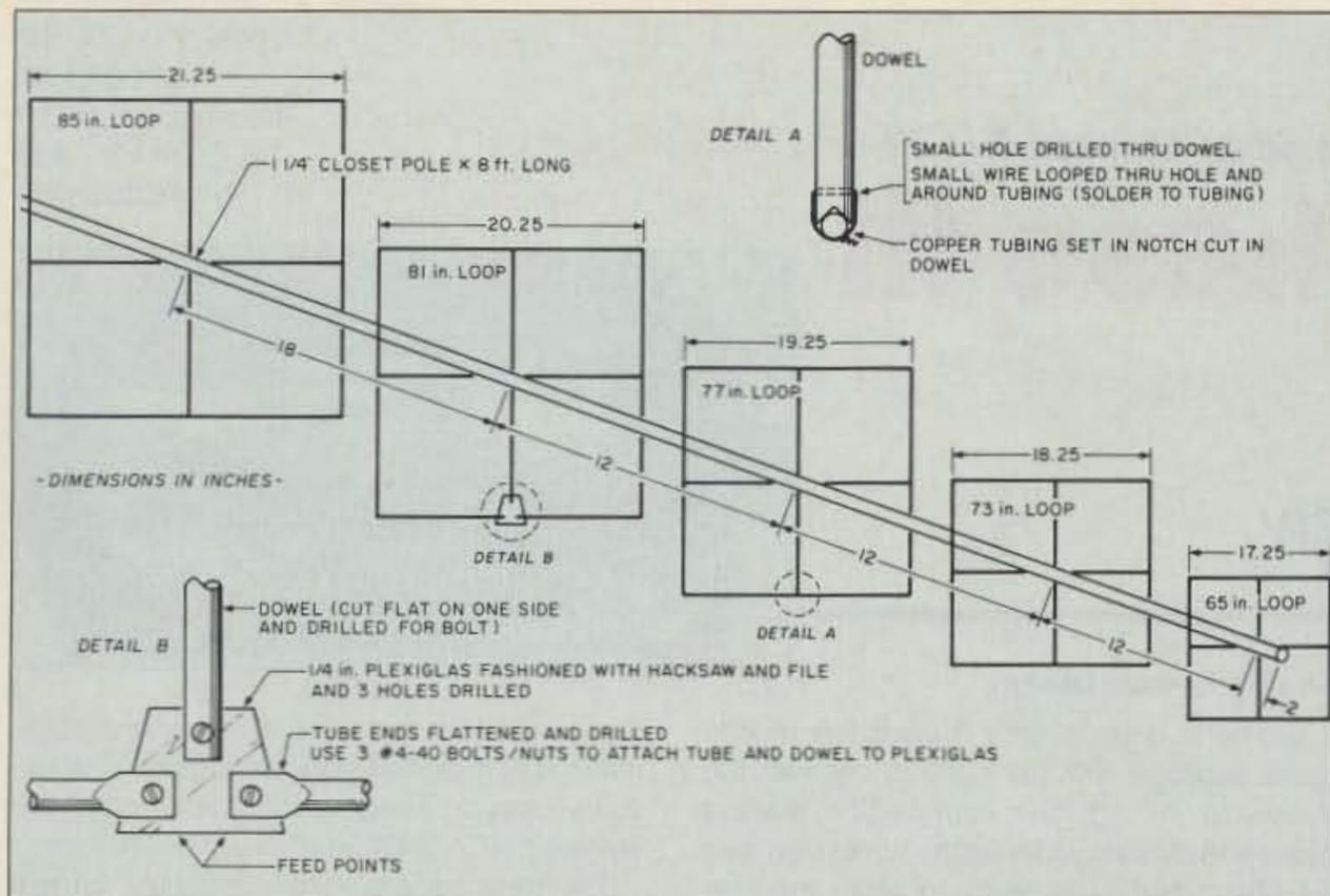
Figure 1. Constructing the 2 meter beam.
