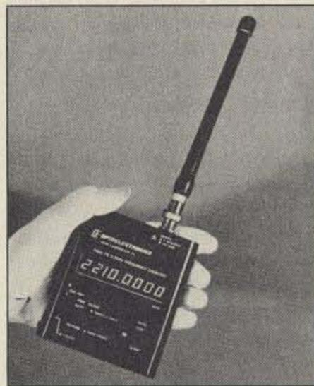
test instrument that will fit in a toolbox or in the palm of your hand. It measures 4" x 3.5" x 1" (14 cubic inches) and weighs only 9 ounces. Despite its small size, the Model 2210-A specifies an operating range from 10 Hz to 2.4 GHz and is useful to 2.8 GHz. It detects and displays two overlapping frequency ranges: 10 Hz-12 MHz and 10 MHz-2.4 GHz, with resolution of 1 Hz and 100 Hz respectively. The accuracy is  $\pm 1$  PPM.
