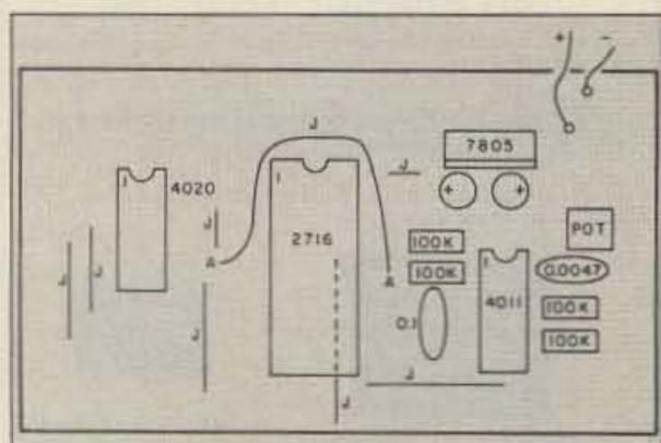
Figure 2. Parts placement, component side.
