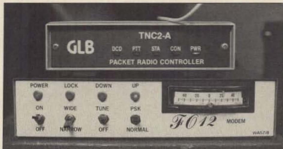
Photo A. A G3RUH 1200 baud PSK modem hooked up to a packet TNC for Microsat or Fuji digital communications.
