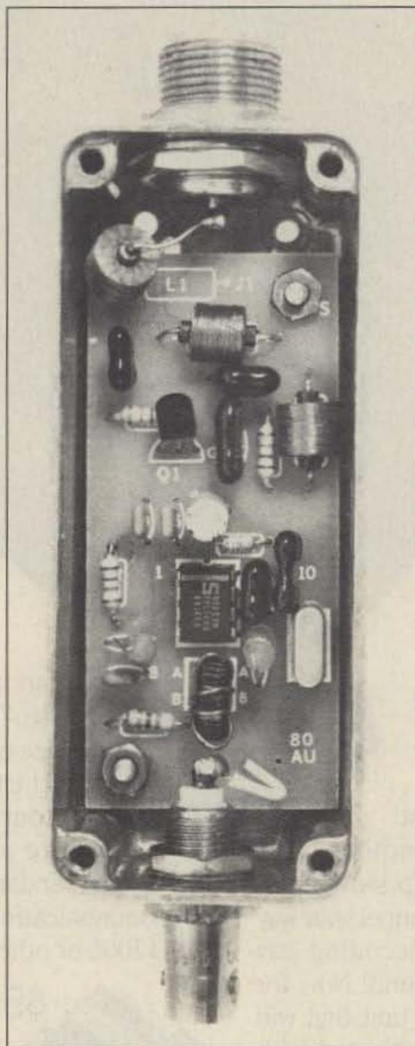
Photo A. Inside the 80AU converter.
