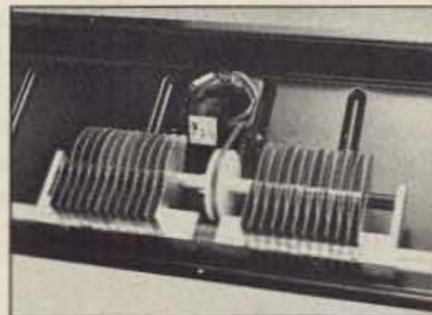
IsoLoop precision stepper motor provides accurate tuning.
