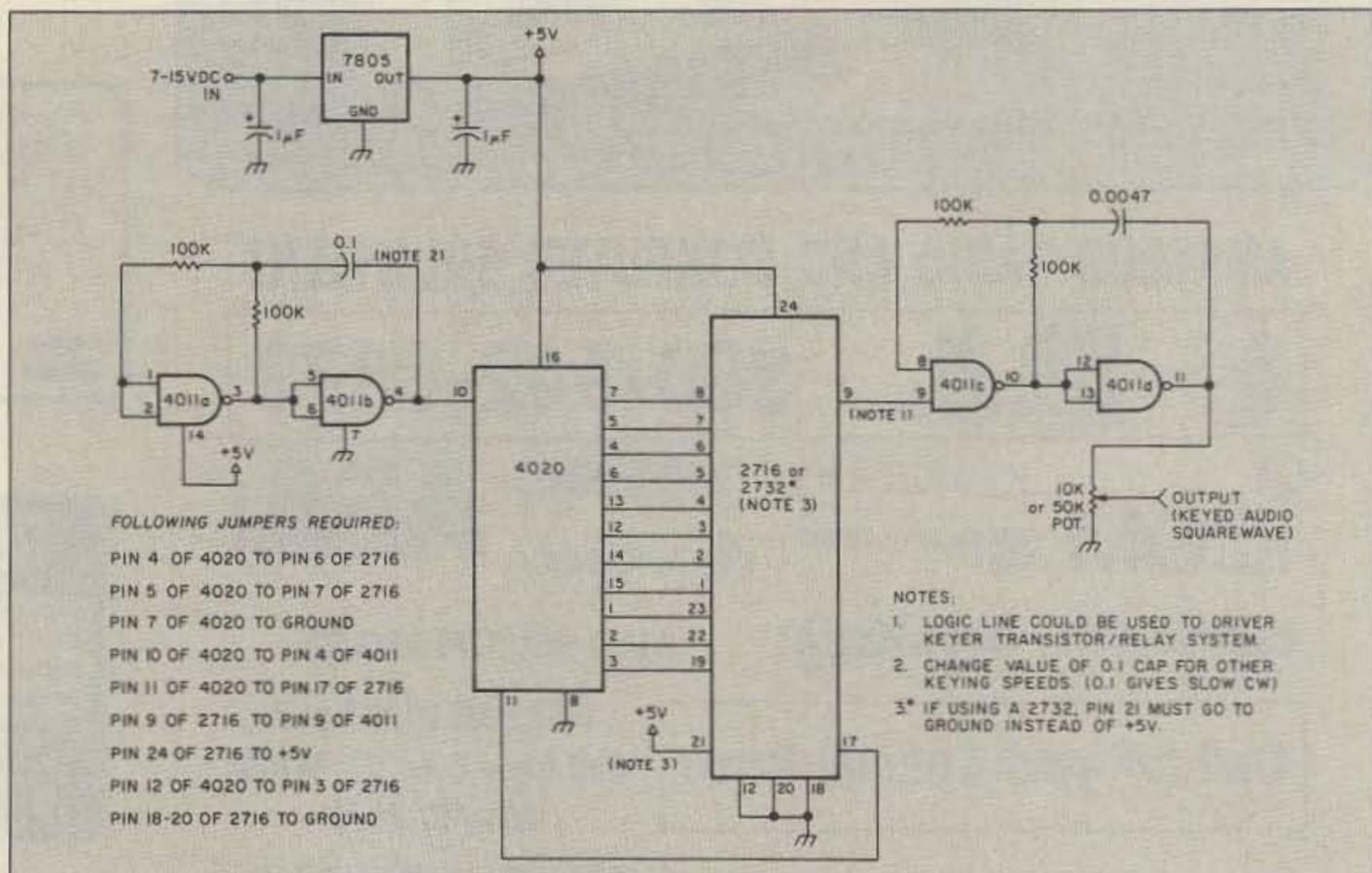
Figure 1. Circuit for the CW IDer.
