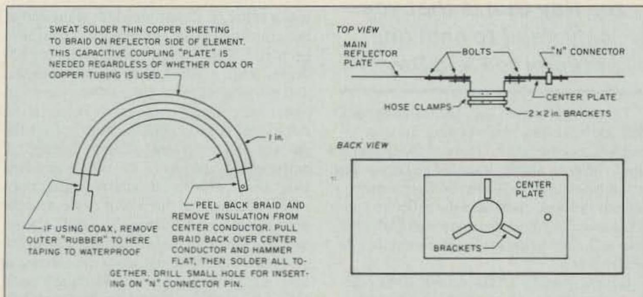
Figure 3. Final construction details.
