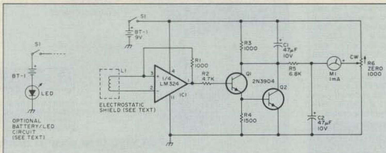
Figure 1. Schematic of the experimental gaussmeter.
