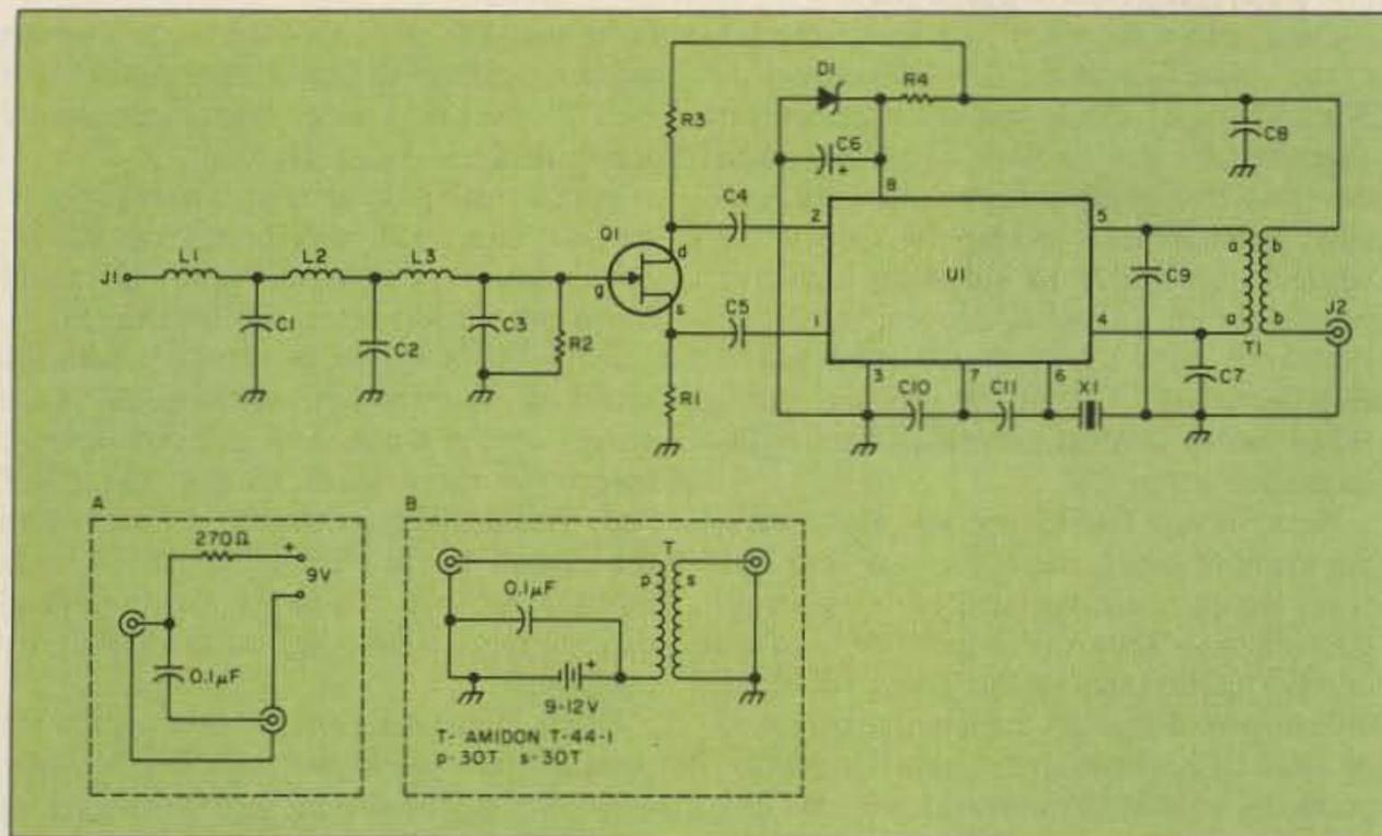
Figure 1. Schematic for the 80AU converter.
