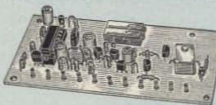
**MO-202 FSK DATA MODULATOR kit.** Run up to 1200 baud digital signals through any fm transmitter with full handshakes. Radio link computers, telemetry gear, etc. .... \$39
