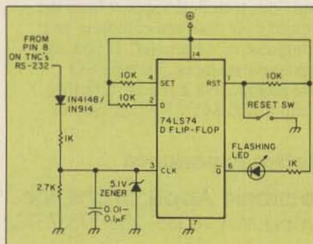
Schematic of the TNC connect alarm.
