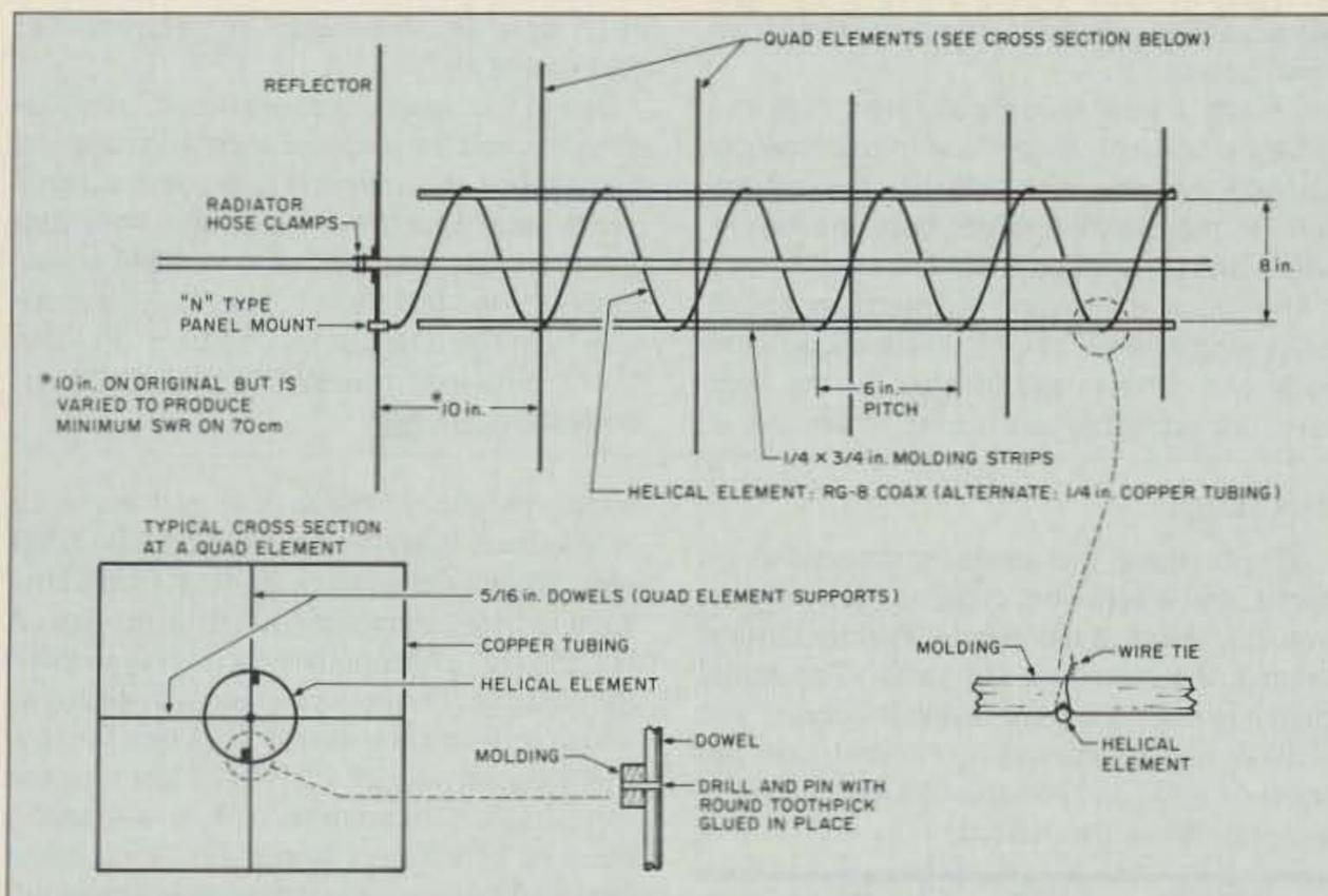
Figure 2. Constructing the helix.
