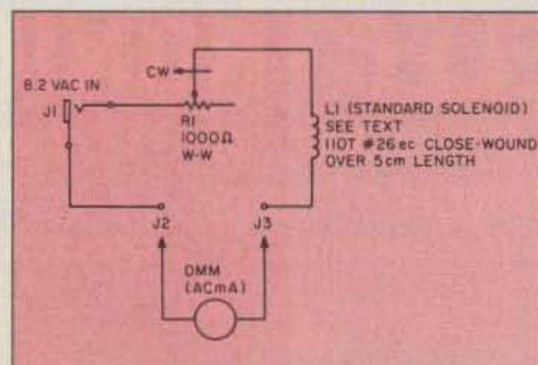
Figure 1. Standard magnetic field generator.
