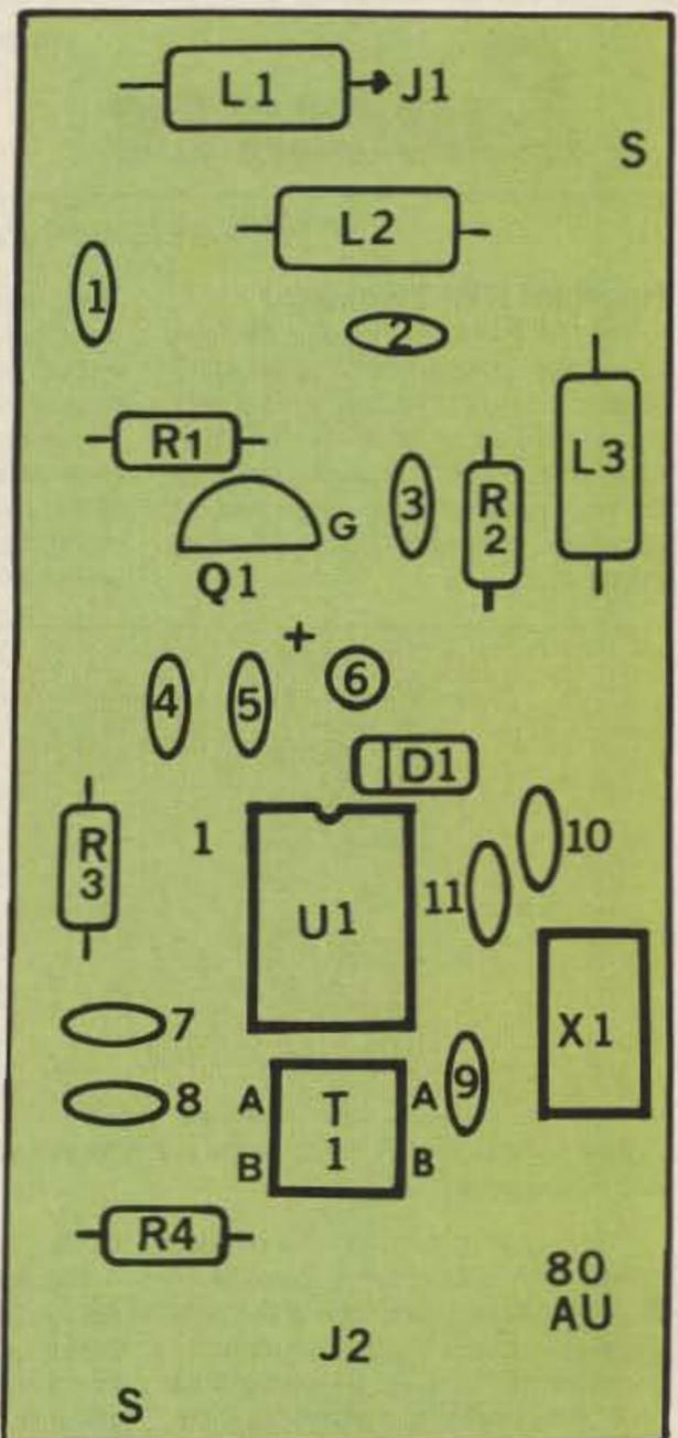
Figure 2. Components layout diagram.
