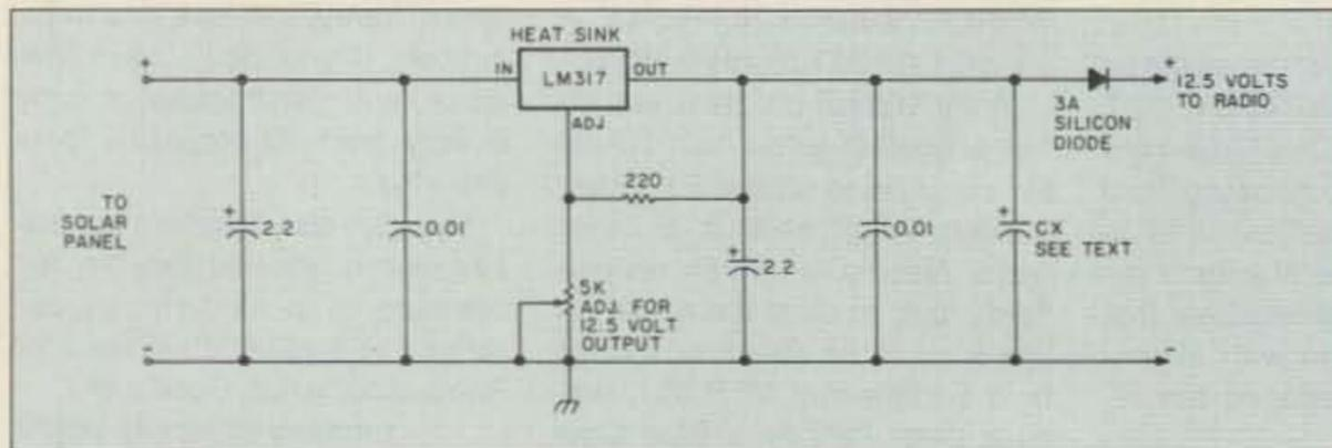
A simple circuit for a small voltage regulator.
