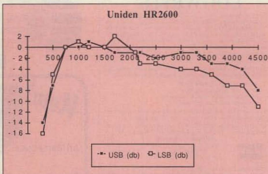
Figure. HR-2600 frequency response curve.
