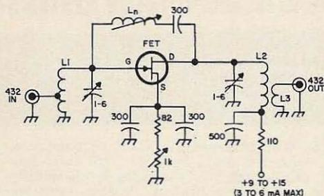
Fig. 1. Grounded source circuit for FET's.
