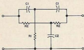
Fig. 1. The Parallel-T Network.
