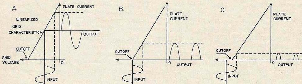
*Class A—Output is replica of input current flows throughout cycle*
