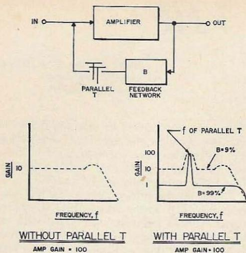
Fig. 2. A parallel-T in series with the feedback network of a degenerative amplifier.
