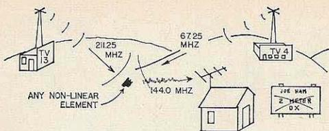
Fig. 9—It's not just the TV audience who get hurt by the problem of cross-modulation. Any two signals can do it, and one of the prime examples is that occurring when TV channels 4 and 13 operate in the same locality. 2-meter DX around 144.0 MHz is completely wiped out by the interference which results. Since any type of non-linear element can cause the mixing action, it's not normally practical to eliminate this problem; most of us just learn to live with it.
