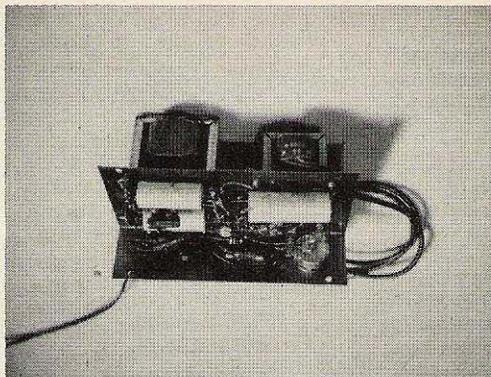
220 volts) plus the drop through the 4.7 k 2 W resistor. Second, the operating point is established for the screen by having a voltage limit of only one neon drop at the lower end of the 20 k pot: this gives rather precise control of the modulated AM output in AB<sub>2</sub>. Without the neon's, cathode bombardment may result from the excessively high plate and screen voltages when *not* transmitting or driving with some rf signal, but leaving the mode switch on DSB.
