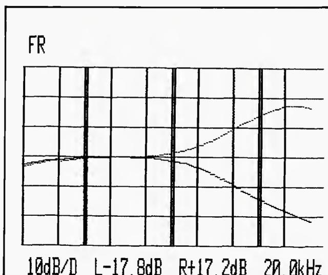
Figure 3.(A) Boost and cut range of high frequency control for the equalizer section of the input modules.
