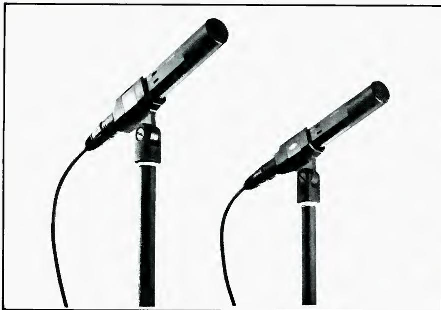
Sennheiser's transformerless MKH 20 P48 omni-directional studio condenser microphone utilizes the same symmetrical capsule as its cardioid sister, the MKH 40. Optimal resistive loading of the microphone diaphragm results in a highly linear frequency response and an inherent noise level that is virtually imperceptible by modern digital recording equipment. The MKH 20 responds to both high and low sound pressure levels
