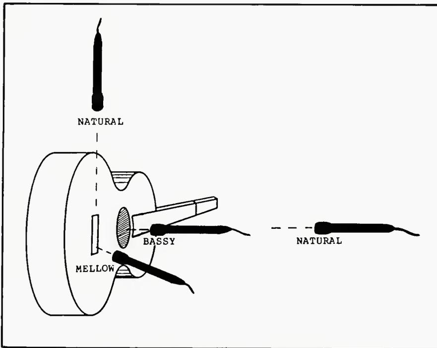
Figure 7. Microphone placement affects the recorded tonal balance.
