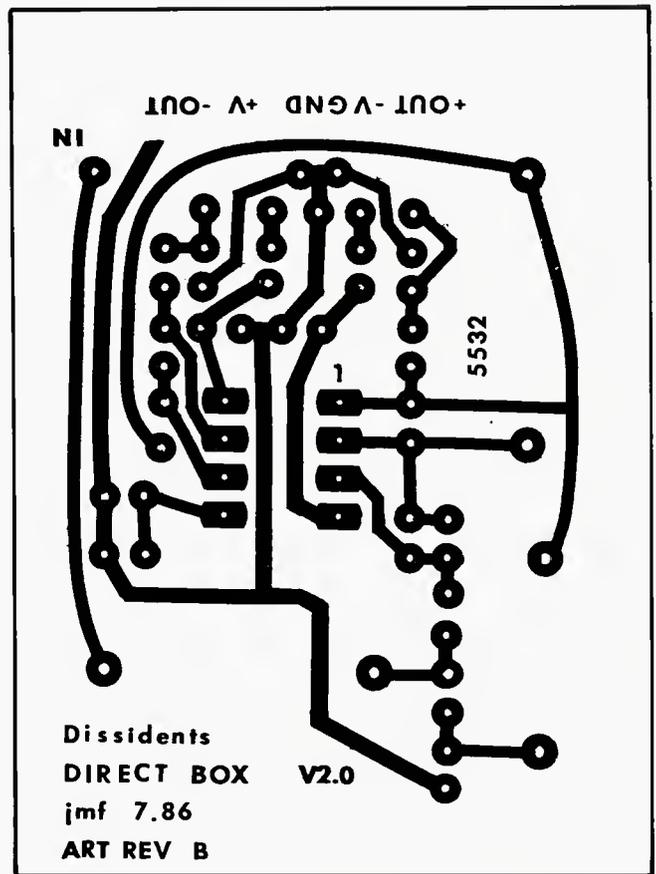
Figure 2. Foil side of the printed-circuit board.
