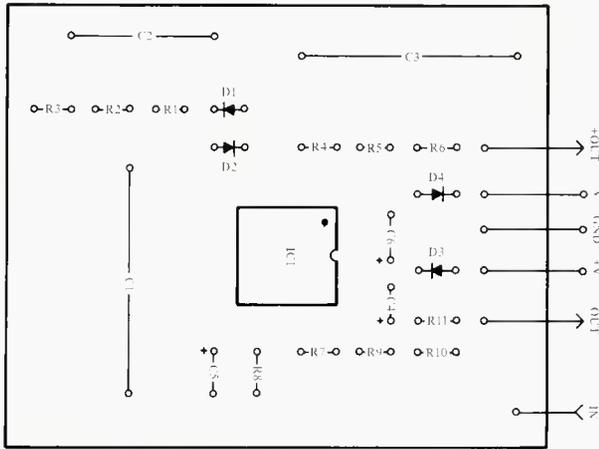
Figure 3. Stuffing guide for the circuit board.
