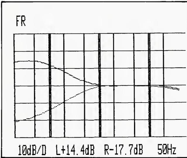
Figure 3.(D) Boost and cut range of the low frequency control for the equalizer section of the input modules.
