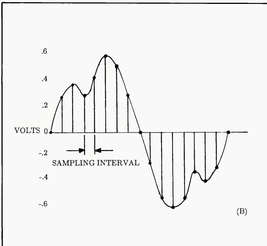
(B)The voltage is measured or sampled at regular intervals.
