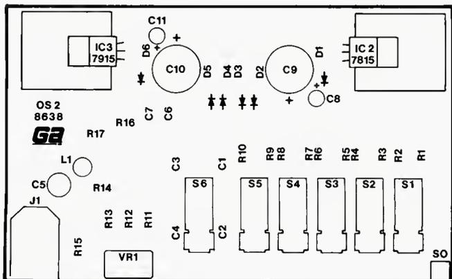
Figure 3. A component assembly guide showing component placement on the PC board.
