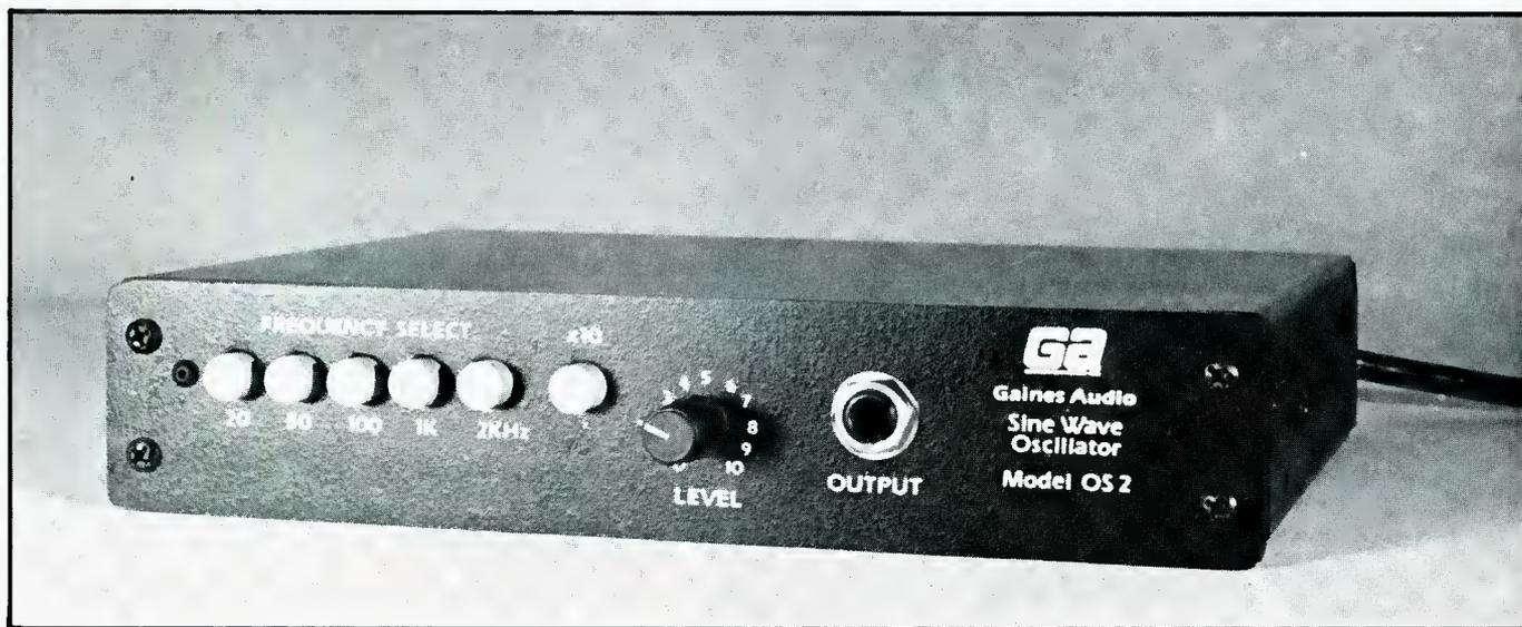
*Completed sine wave oscillator.*
