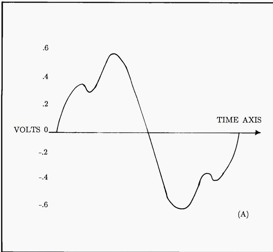
Figure 2.(A)The audio waveform enters the A/D converter.
