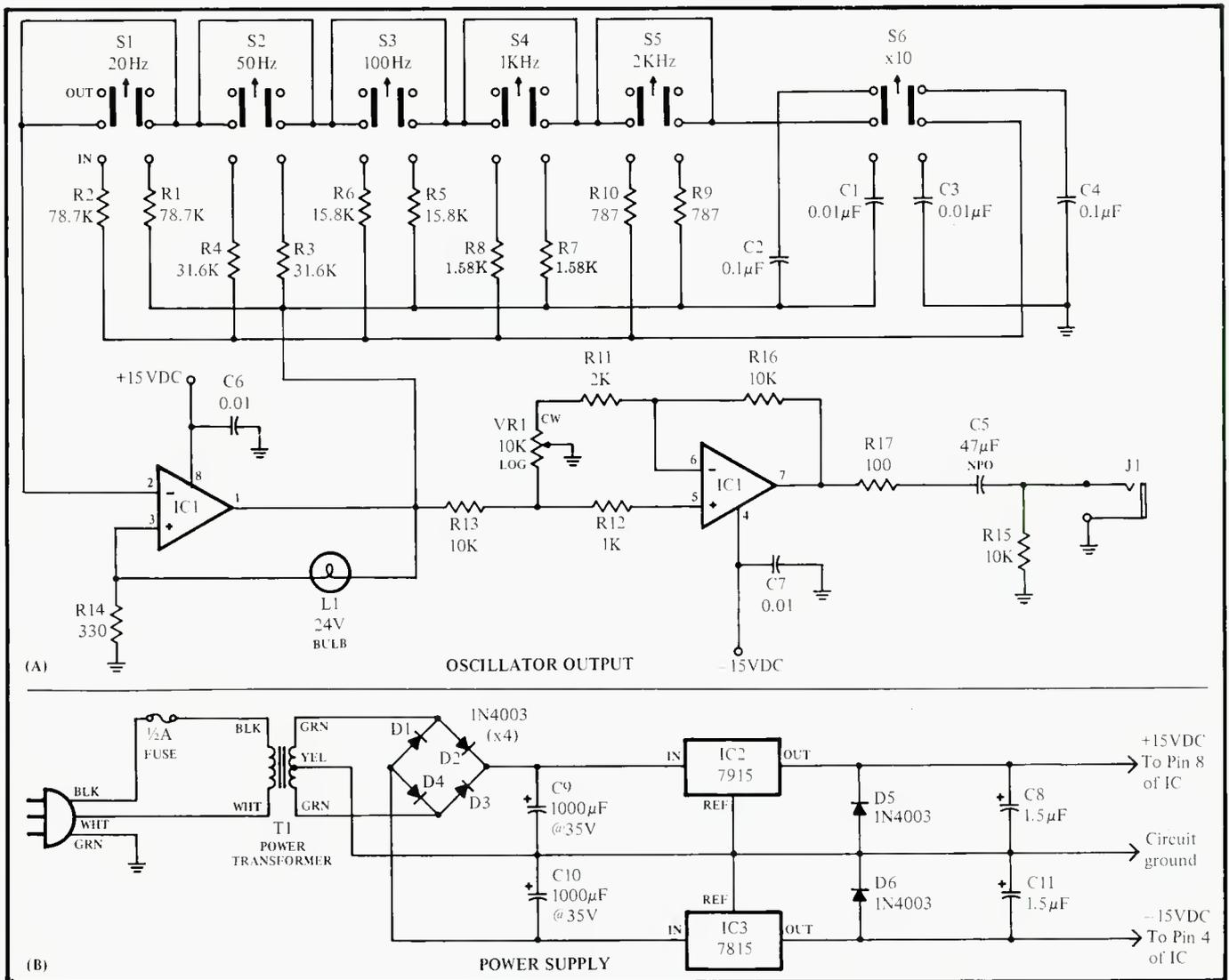
Figure 1. The schematic diagram for the oscillator circuit (A), and power supply circuit (B).
