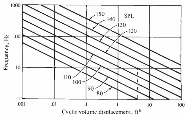
Figure 6. The cyclic volume displacement required for a baffled piston to generate the indicated sound pressure levels at a distance of 10 feet. For example, for a 10 Hz signal, a cyclic volume displacement of 4 ft<sup>3</sup> is required to produce a *SPL* of 120 dB at a distance of 10 feet from the speaker.
