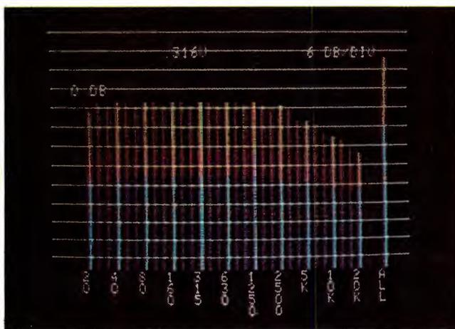
changing the measured value. In Badap 1, the peak value is a word in memory, and it will remain there, unchanged, until the memory is erased or the machine unplugged.
