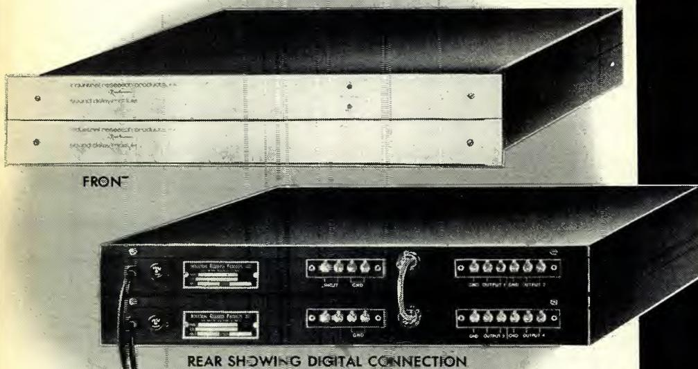
Where more than two outputs and 96 milliseconds of time are required we have added a digital connector that can link two of our DD-4012's with no signal degradation. This linkage gives the same high quality signal with 160 ms and four independent outputs.
