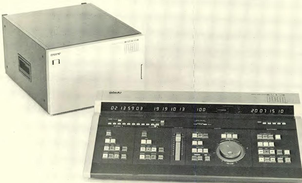
The DAE-1100 Digital Editor. Note the large edit-search dial on the front panel. The system memory stores six seconds of program material, which may then be "rocked"
