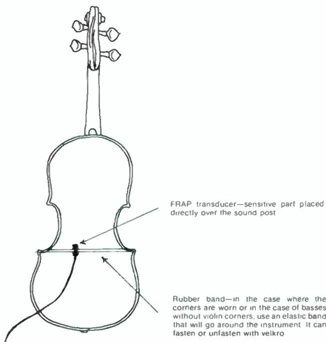
Figure 4. The transducer is placed directly over the sound post.
