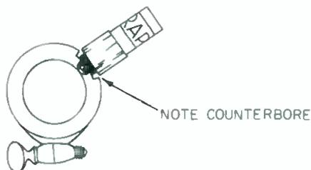
Figure 9. Installation of a screw-mount transducer.
