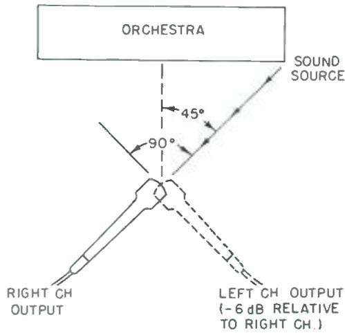
Figure 1. Coincident-pair technique. Cardioid microphones crossed at 90 degrees.
