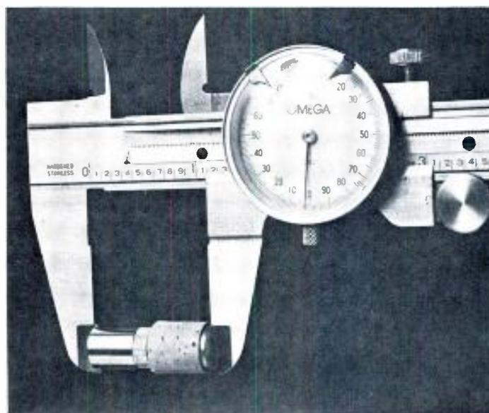
Figure 8. The Type W piccolo transducer.
