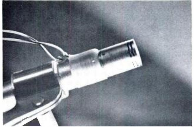
Figure 2. A condenser microphone outfitted with heater.
