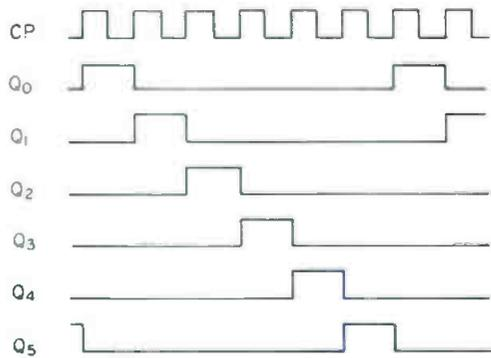
Figure 2. IC5 waveforms.
