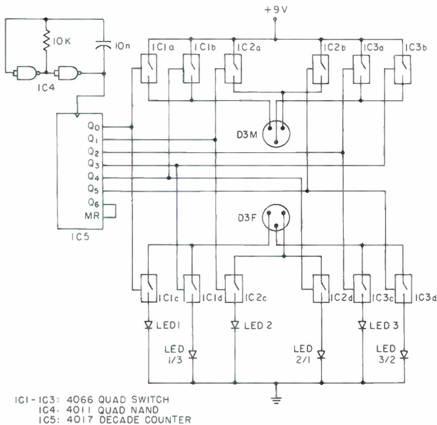
Figure 1. Schematic diagram for the microphone cable tester.
