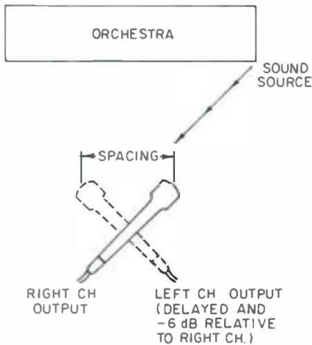
Figure 2. Near-coincident technique. Cardioid microphones crossed and spaced.
