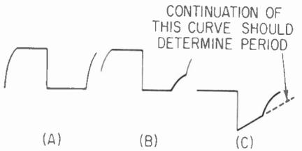
Figure 5. While the frequency went down with reduced base-supply voltage, the collector waveform looked like (A). When the frequency started going up again, it looked like (B). Voltage starts to rise before the end of the conducting half period. (C) This couples through the capacitor, making the other side reach zero (and conduction) sooner than it should.
