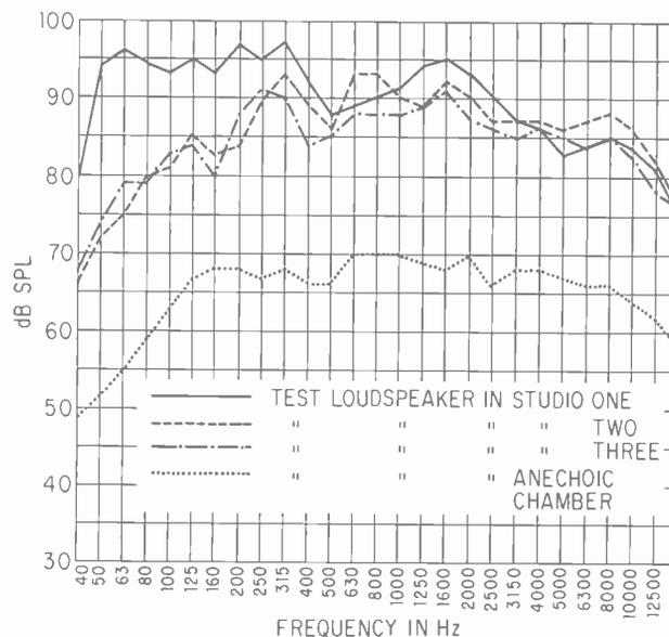
Figure 1. Each of these response curves was taken with the same test loudspeaker, but measured in different rooms. The anechoic chamber measurement was made in the large chamber in the Altec Lansing engineering laboratory.
