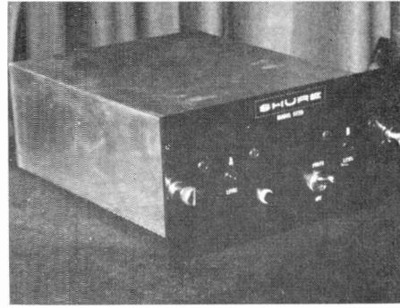
**Shure Brothers, Inc.** Model SE20 is a solid-state stereo transcription preamp. Precise RIAA/NAB equalization is included, noise and r.f. susceptibility are extremely low, full line capability is to +20 dBm. Distortion is under 0.5 per cent at +20 dBm 20-20,000 Hz. Input is 47,000 ohms; output is for 600- or 150-ohm balanced line. Price: \$336. Circle 68 on Reader Service Card.
