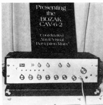
**R.T. Bozak Mfg. Co.** Model CAV-6-2 permits the user to adjust the balance between its two mono outputs so that the apparent location of sound sources correspond to the physical locations of microphones. There are six inputs, each divided to drive both left and right speakers. Power output is +18 dBm or 6 volts into 600 ohms. Price: \$399.00. Circle 58 on Reader Service Card.
