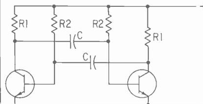
Figure 1. If you want to change the frequency of a multivibrator you can change either the capacitors  $C$ , or the base-feed resistors  $R_2$ . But neither of these are readily made electronically variable.
