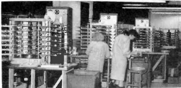
Figure 2. Part of the chain of common-capstan duplicators. The racks contain the master tape which may be in conventional reel-to-reel form, or an endless-loop storage bin toward the bottom of the rack.
