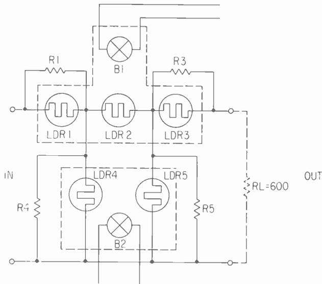
Figure 1. A constant-impedance attenuator.  $R_1$  and  $R_3$  . . .  $560\Omega$ ;  $R_4$  and  $R_5$  . . .  $4700\Omega$ .
