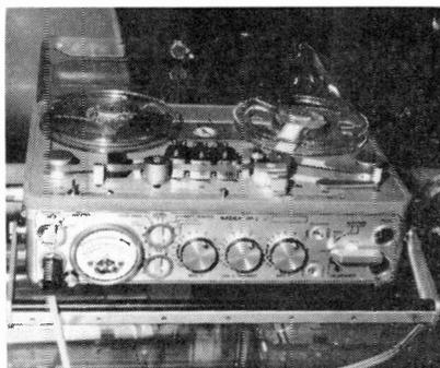
**Nagra Magnetic Recorders, Inc.** The IV-L model has two mic and one line input, mixing facility, manual or automatic level control, low-frequency rolloff, and unbalanced line output. This model also adds three speeds (15,  $7\frac{1}{2}$ , and  $3\frac{3}{4}$  in./sec.) and limiting and fading features. Camera-sync. facility can be added to any unit at additional cost. Price: \$1,660.00. Circle 59 on Reader Service Card.
