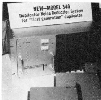
**Dolby Laboratories, Inc.** Model 340. Has been designed to process noise-reduction recordings at the high speeds used in commercially-recorded dubbing operations. Frequency response extends to 640 kHz, providing full 20 kHz bandwidth at up to 32-times normal speed. The end result will be an NAB recording with substantially the same noise level as if it had been made at the original recording session. Price: \$1,950.00. Circle 57 on Reader Service Card.
