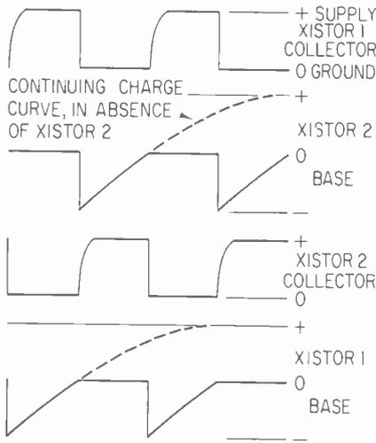
Figure 3. The triggering action in the multi-vibrator circuit shown in Figure 2.
