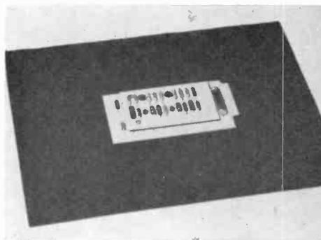
**Spectra-Sonics.** Model 601 is a compressor/limiter on a plug-in card. Field-effect transistors are used to provide independent compressor and limiter action up to 30 dB at under 0.05 per cent t.h.d. (1 kHz). Attack and release times are automatically variable. Price: \$111.60. Circle 60 on Reader Service Card.
