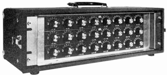
Figure 8. The Altec Lansing model 9014A narrowband equalizer in its portable carrying case.
