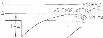
Figure 4. The voltage across the base resistor at the beginning of a half period is  $(1 + a)$ . At the end of the half period it is  $a$ .
