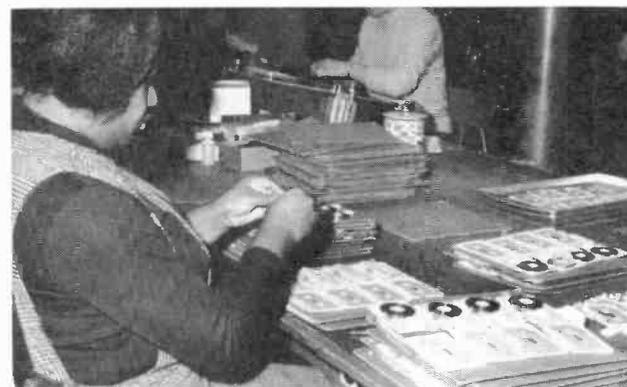
Figure 8. An operator places the recorded hub into the body of the cassette and threads the looped leader onto the other hub.
