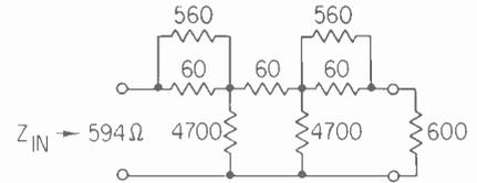
Figure 2. The equivalent circuit of an attenuator without added attenuation. Insertion loss is 3 dB.
