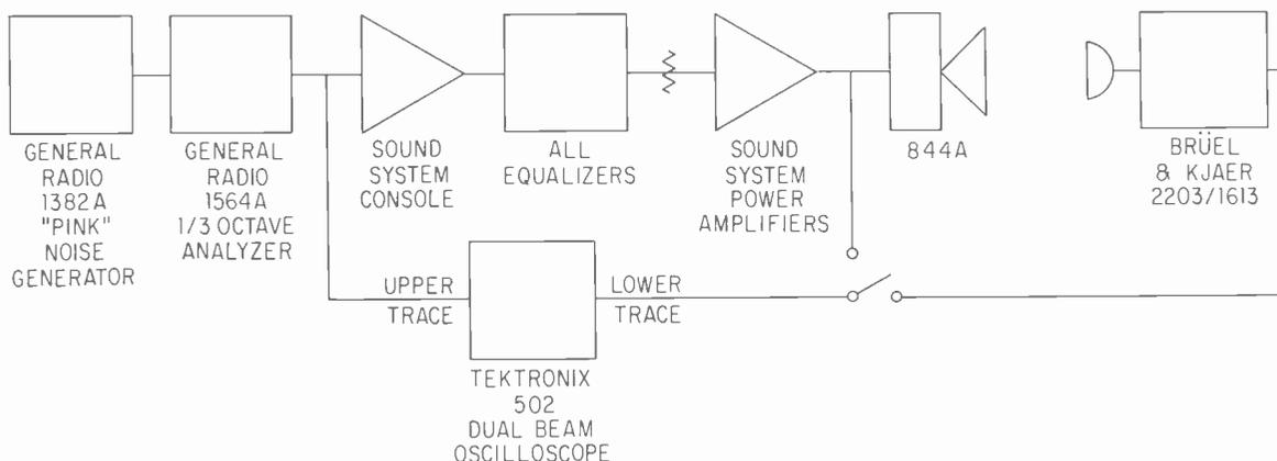
Figure 2. The type and interconnection of test equipment such as was used in Figure 1. Standing-wave effects have been averaged at low frequencies. Repeatability of these measurements is high—variations of curves made by several engineers was  $\pm 1$  dB in any of the spaces measured.
