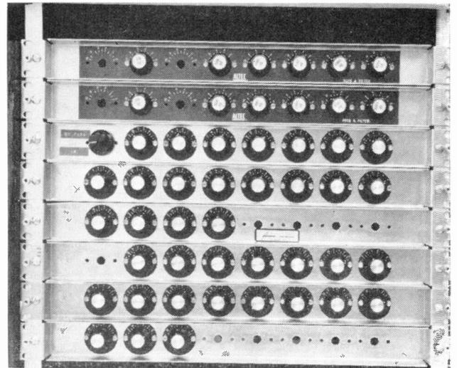
Figure 9. The actual filter sections used at one of Century's rooms. The top two chassis have the needed filters from a 9018A equalizer. The bottom six contain the necessary filters from a pair of 9014A equalizers. The filtering system is tuned for a two-channel audio system. Note the A-B comparator switch to allow comparisons with or without equalization.
