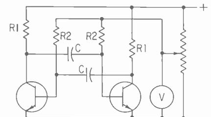
Figure 2. A potentiometer can be used to electronically vary the top-end supply voltage for purposes of exploration.
