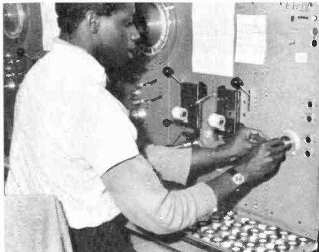
Figure 6. This close-up of the loading machines seen in Figure 5 shows the operator controlling the winding of a cassette hub. The two white rolls on the machine (to the left of the operator's hands) contain the leader material.
