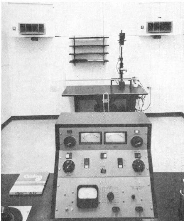
Figure 4. The view from the operator's seat at the console in Century's quality-control room. The two speakers (Altec 844A) are aimed at the operator's head. The sound-level meter was placed at the camera position for equalization measurements.
