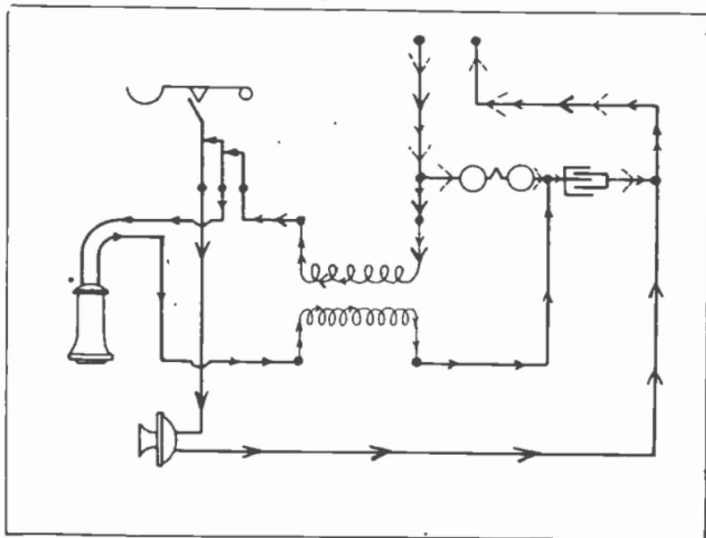
Fig. 4. Wiring diagram for a simple telephone to be used on a central energy system. This telephone gets all the energy from the line and central supply.
