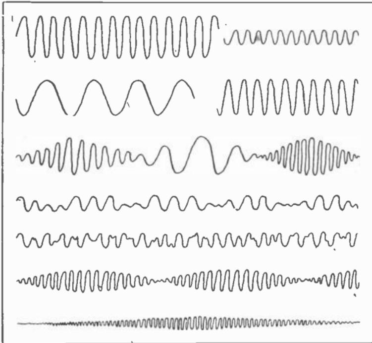
Fig. 1. This sketch shows a number of different forms of sound waves represented by curves. The upper line shows two groups of waves, both of about the same frequency, but the first group of considerably greater volume than the second. The second line shows two groups of about the same volume, but the first is of much lower frequency than the second. The third line shows waves of varying volume and varying frequency.
