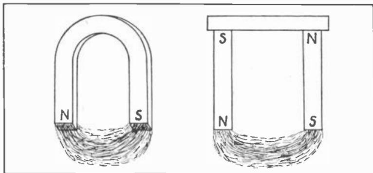
Fig. 79A. Horseshoe magnets have a much shorter flux path through air from pole to pole.
