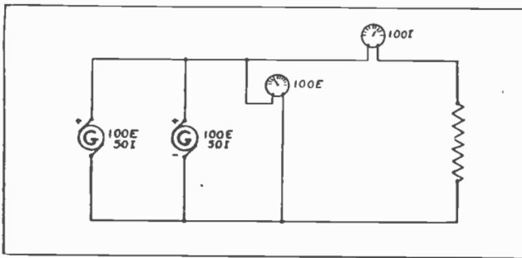
Fig. 45. Electric Circuit With Two Generators In Parallel.
