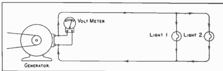
Fig. 36. Electric Circuit With Two Lamps In Parallel.
