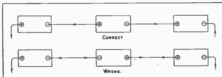
Fig. 47. Polarities of Sources Connected In Series.
