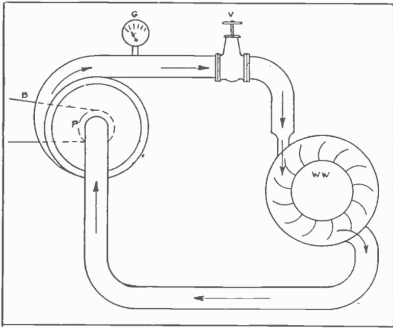
Fig. 33. Water Circuit With Its Parts In Series.
