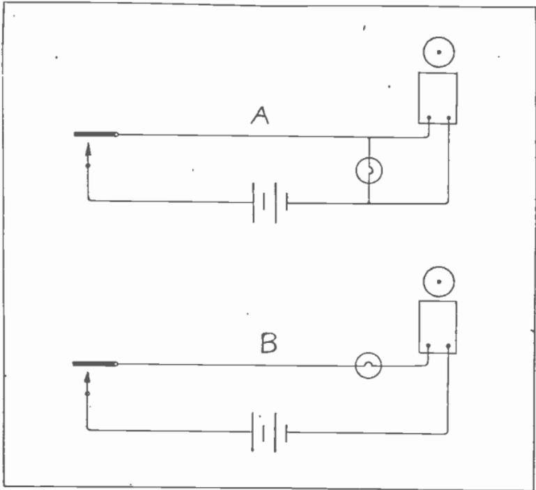
Fig. 13A. Signal lamp connected in parallel with a bell so they both operate at once.
