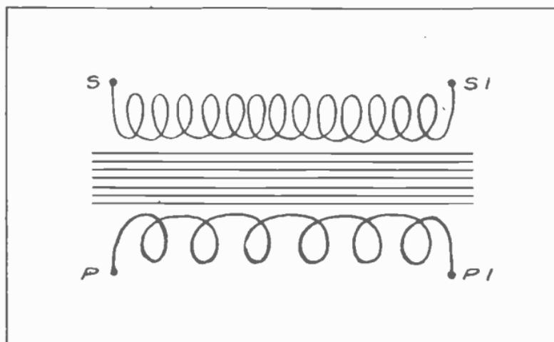
Fig. 15. The primary and secondary windings and core of an induction coil are often shown in the above manner in electrical diagrams.
