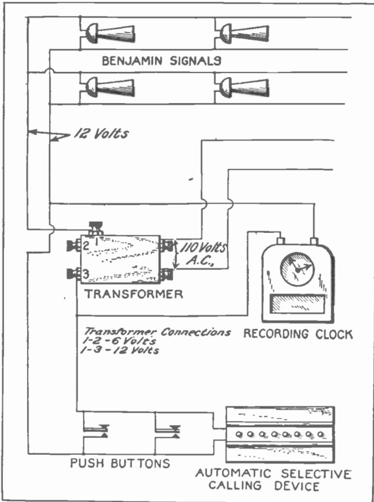
Fig. 24. This diagram shows the connections for signal horns operated from a transformer, and controlled either by a time clock or automatic signal device.
