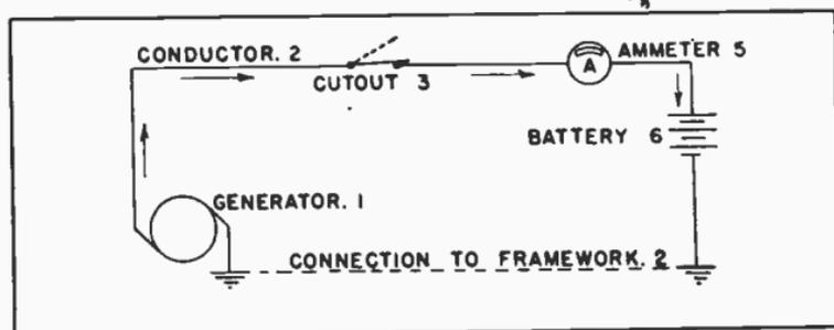
Fig. 10. Simplified Diagram of the Auto-electric System.
