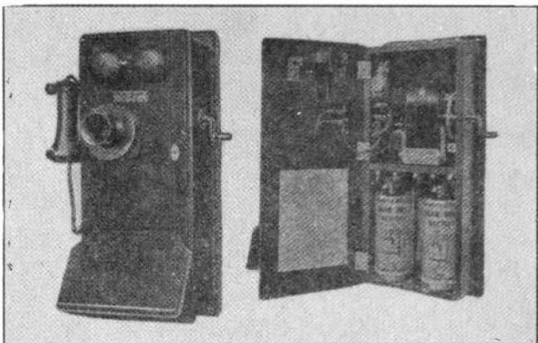
Fig. 1. Common type of party line telephone used on rural lines. This telephone is complete with its own batteries and magneto.
