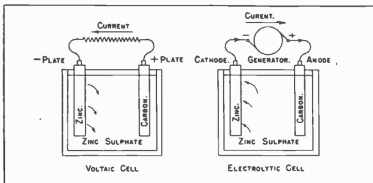
Fig. 61. Current Flow In Voltaic and Electrolytic Cells.
