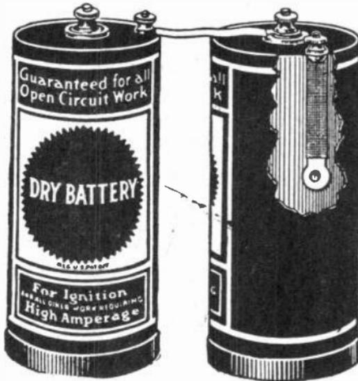
Fig. 3. Two common dry cells such as used extensively in signal systems. One is cut away to show terminal strip attached to the zinc.
