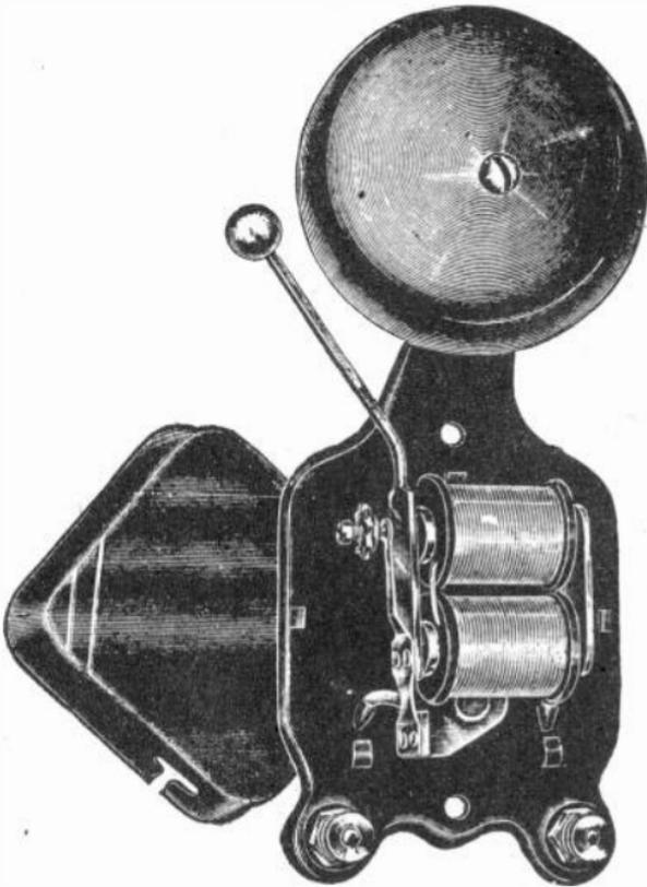
Fig. 1. View showing common vibrating bell with cover removed. Note carefully the construction and arrangement of coils, armature, and contacts.
