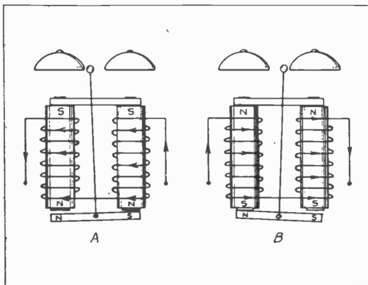
Fig. 20. This sketch shows the construction and windings of another type of polarized bell, which uses a permanent magnet for its armature. Note the polarity and position of armature at "A," and again at "B," after the current has been reversed.
