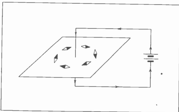
Fig. 88. Small compass needles showing shape and direction of lines around a conductor.
