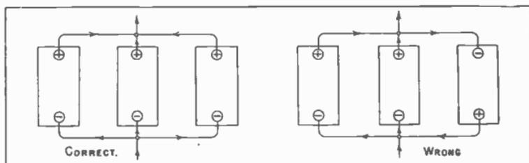
Fig. 48. Polarities of Sources Connected In Parallel.
