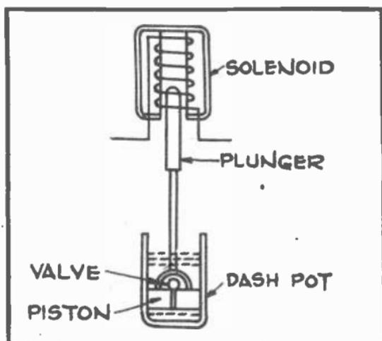
Fig. 11. This sketch shows the use of a dash-pot to slow the action of solenoids and electro-magnets.
