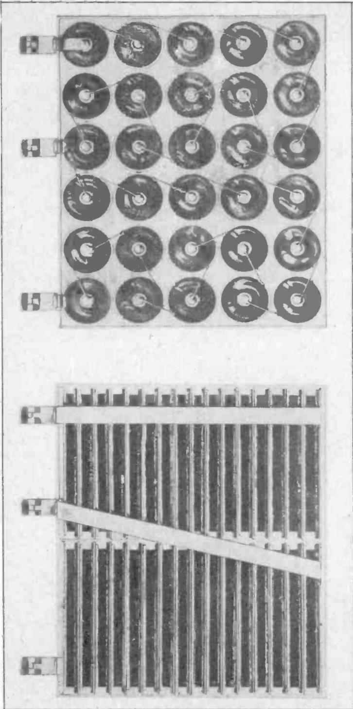
Fig. 60. Internal Construction of Two Types of Radio "B" Batteries.
