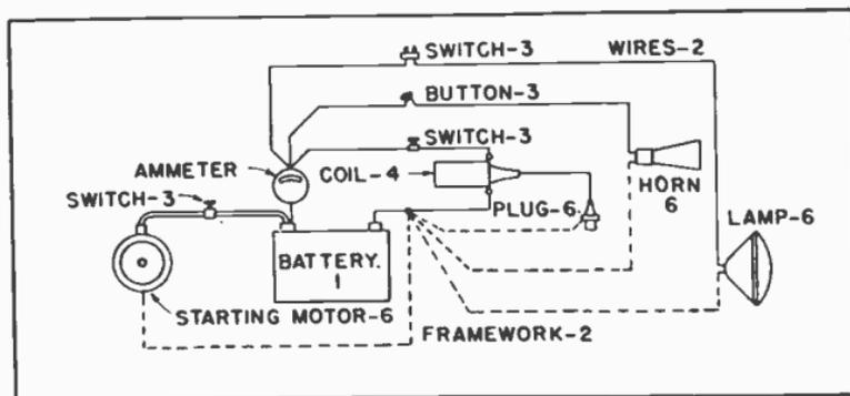
Fig. 12. More Parts of the Auto-electric System.
