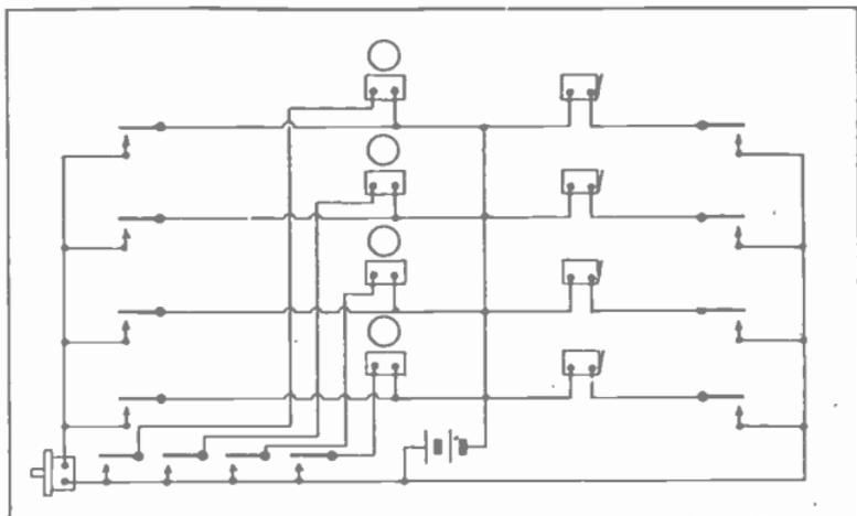
Fig. 23. Doorbell and door-opener system, including separate local buzzer circuits.
