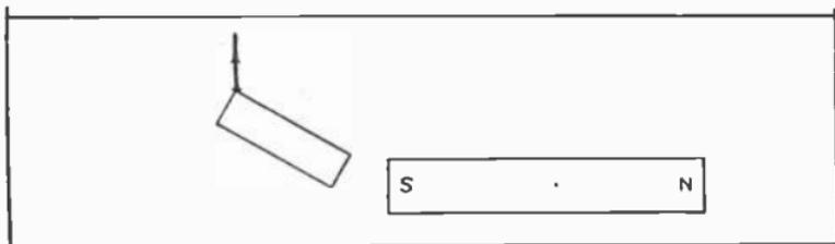
Fig. 68. The small bar or iron attracting the nails, obtains its magnetism by induction from being near the large magnet.
