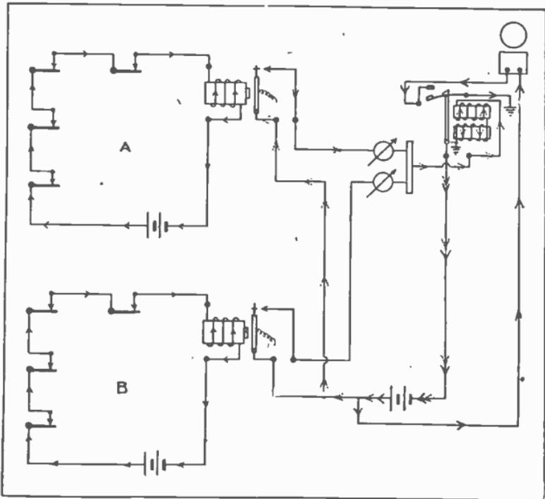
Fig. 26. Two section alarm system using a drop relay for constant ringing, also an annunciator to show which section of the building the alarm was disturbed in
