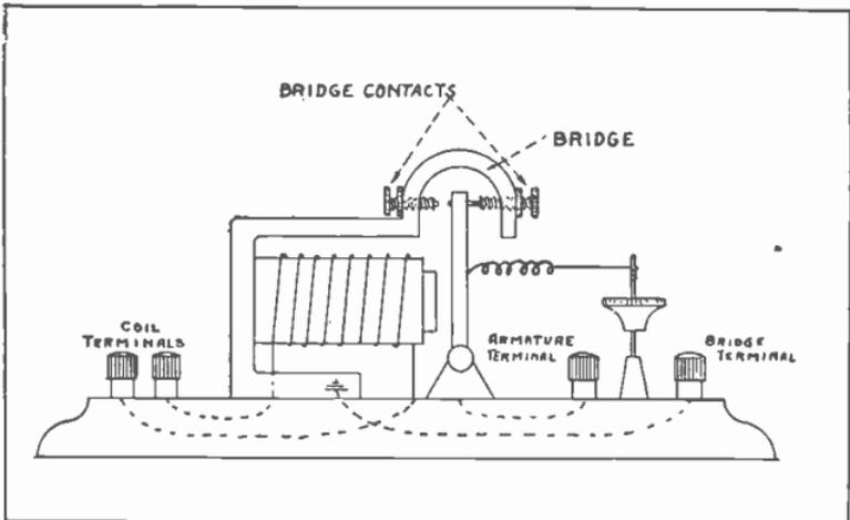
Fig. 22. Diagram showing the arrangement of the electrical circuits and terminals of a Pony Relay.
