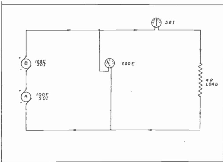
Fig. 42. Electric Circuit With Two Generators Connected In Series.
