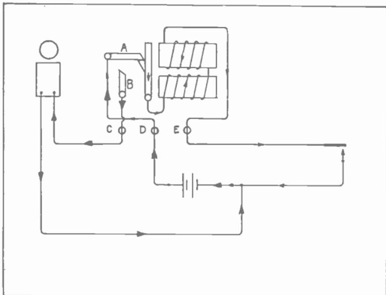
Fig. 20. This sketch shows the method of connecting a drop-relay such as shown in Fig. 19 to a bell battery and push button for constant ringing signals.
