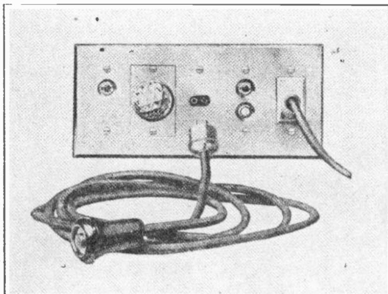
Fig. 12. Panel and cord for silent hospital signal. The lamp is located behind the glass "bulls-eye" at the left.
