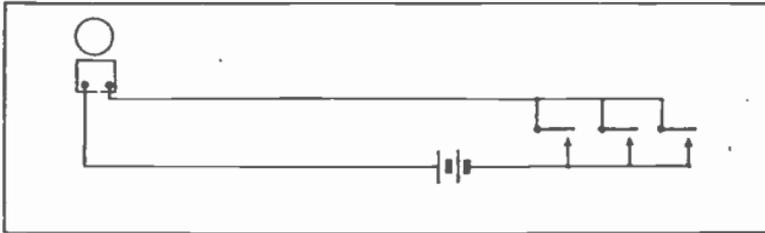
Fig. 10. Simple signal system using three buttons in parallel, any one of which will ring the bell.
