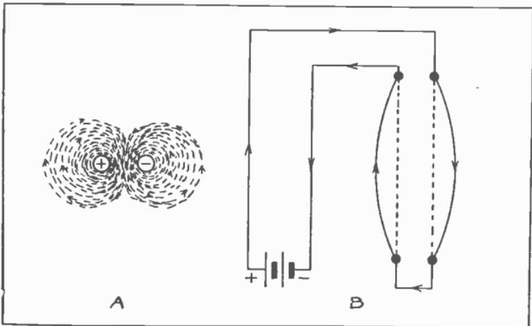
Fig. 91. This sketch shows the repulsion of parallel wires, carrying current in opposite directions.
