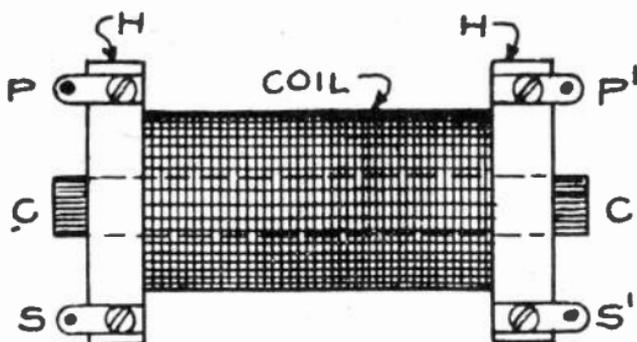
Fig. 13. This sketch shows the construction of the windings and core of a telephone induction coil.
