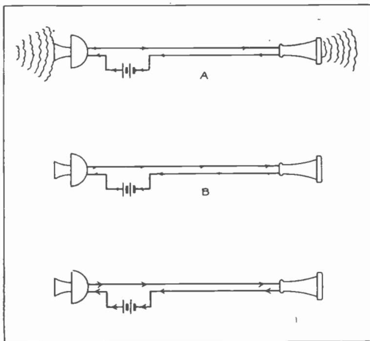
Fig. 3.—A. Sound waves striking the transmitter are reproduced electrically by the magnets in the receiver.
