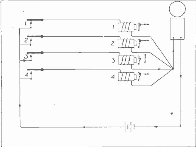
Fig. 2. Circuit diagram of the connections for a four-drop annunciator. Note that the drop number 3 has been operated.
