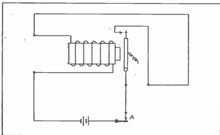
Fig. 1. Diagram illustrating the principle of a closed circuit holding relay.
