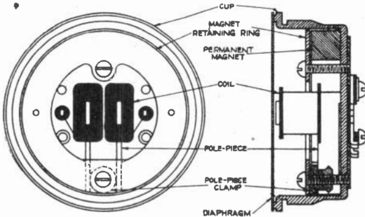
Fig. 11. Sectional view and front view of watch case receiver, such as used on telephone operators' head sets.
