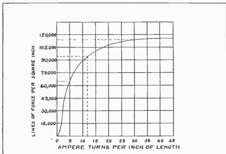
Fig. 100. Curve showing number of lines of force that can be set up in soft sheet iron, with various numbers of ampere turns.
