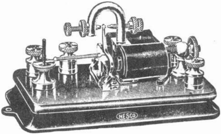
Fig. 23. Another type of Pony Relay similar to the one in Fig. 21, but of slightly different mechanical construction.
