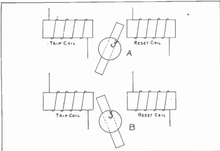
Fig. 7. Sketch illustrating arrangement of coils and number disks on an "electrical reset" annunciator.
