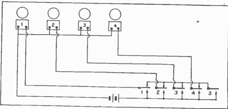
Fig. 18. Selective call system with Master Switch. This is a type of system very often used in executives' offices.
