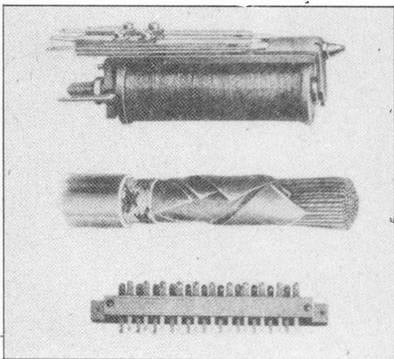
Fig. 20. The upper view shows a telephone relay. In the center is shown a section of telephone cable. Below is a group of terminal springs in a terminal block.
