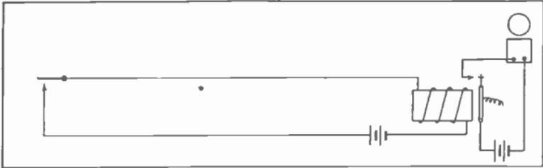
Fig. 26. Connection diagram for an open circuit relay used to operate a bell at a considerable distance from the push button.
