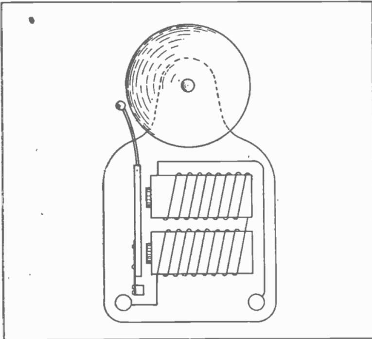
Fig. 5. Circuit diagram of a single stroke bell. Note that it does not have "make and break" contacts.
