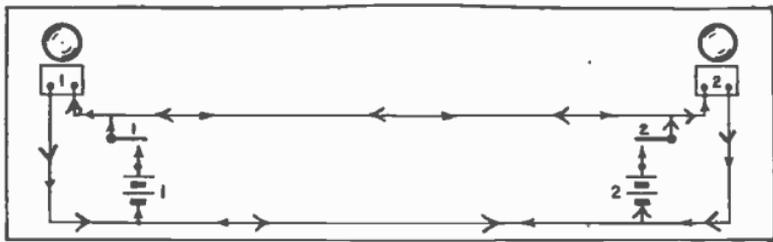
Fig. 13. Return call system using two batteries, thereby saving one wire.
