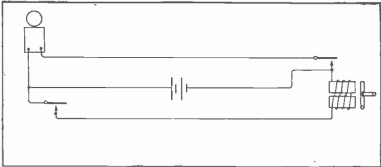
Fig. 16. Sketch showing connections for a door bell and magnetic door opener.
