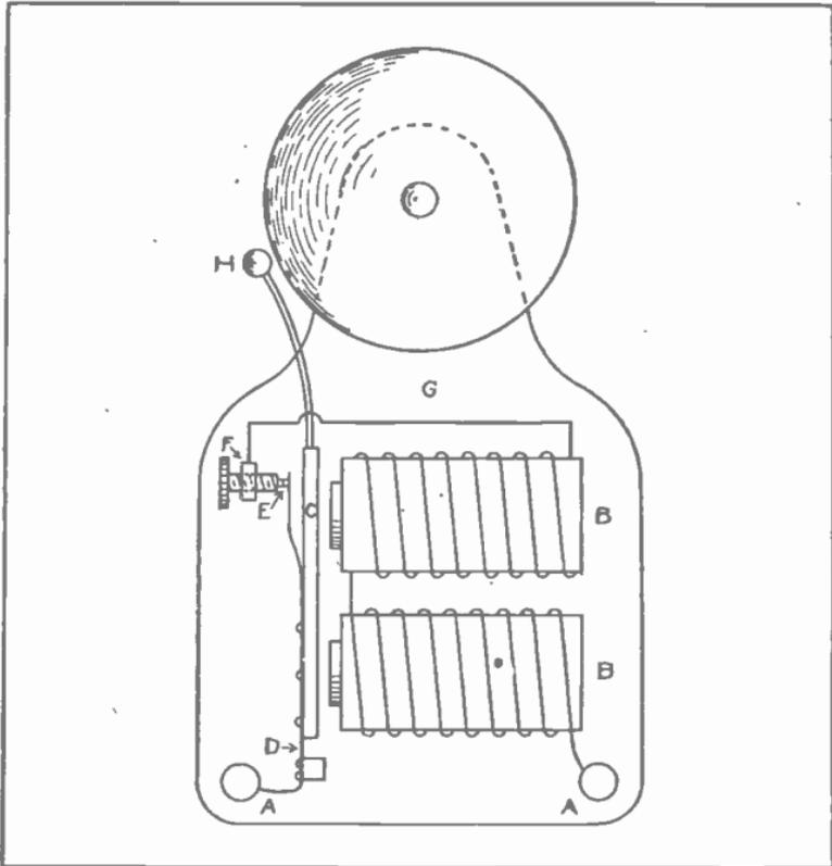
Fig. 2. Sketch showing electrical circuit and connections of common vibrating bell. Observe very carefully the parts of this diagram, and the explanation given.
