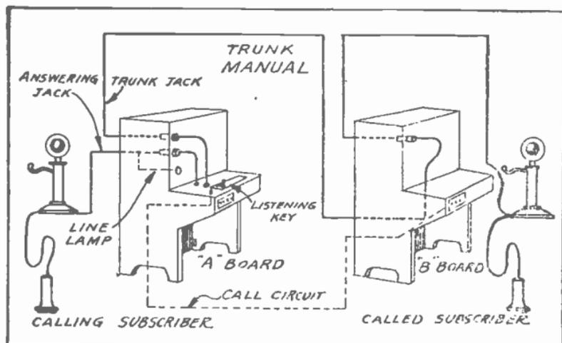
Fig. 21. Simple "one-line" diagram showing a telephone circuit through two exchanges and a trunk line.
