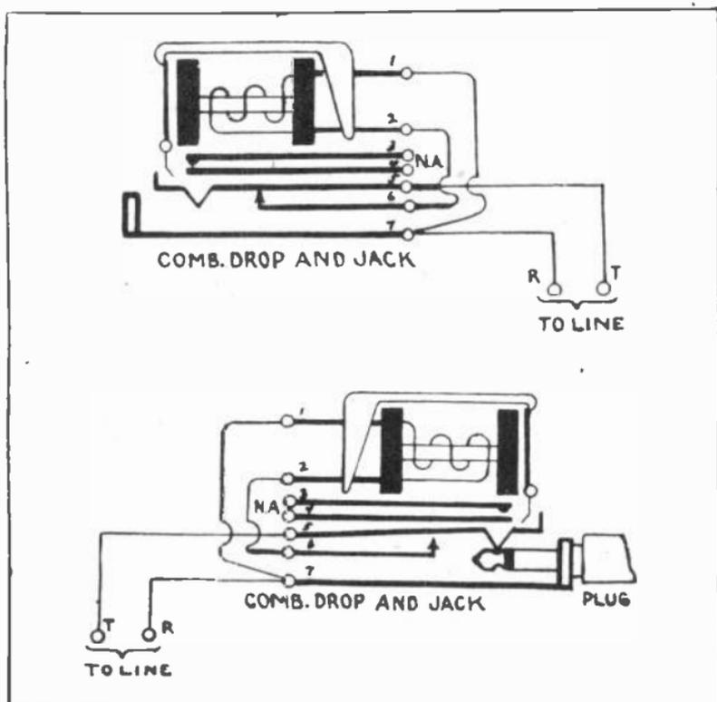
Fig. 15. The upper sketch shows the electrical connections and position of contact springs without the plug inserted. Below are shown the electrical circuit and position of springs with the plug in the jack.
