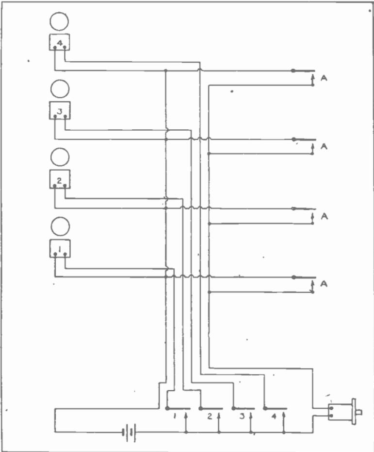
Fig. 22. Combination doorbell and magnetic door-opener system. Note the use of certain wires as common "Feeder" and "Return" wires.
