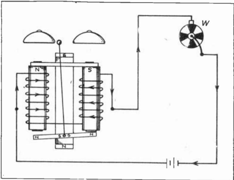
Fig. 18. This sketch shows how a "pulsator" or interruptor can be used to supply pulsating current from a battery and for the operation of telephone bells.
