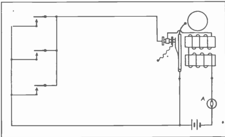
Fig. 27. Simple method of arranging an ordinary vibrating bell to secure constant ringing feature.
