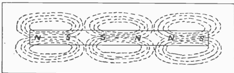
Fig. 84. Consequent poles in a bar magnet.
