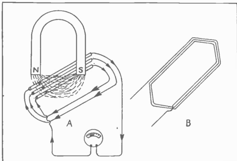
Fig. 110-A. Using several wires connected in series to obtain higher induced voltage.
