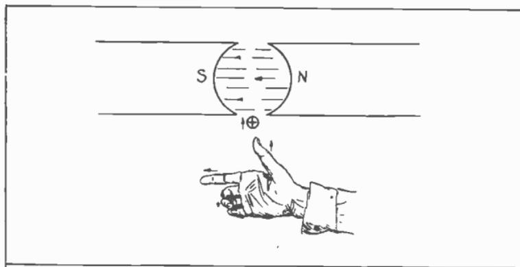
Fig. 109. Right hand rule for direction of induced voltage. Compare position of fingers with direction of flux and wire movement.
