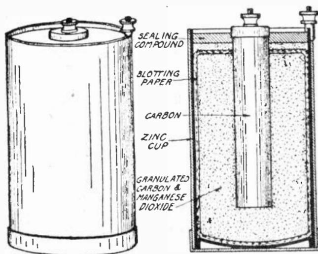
Fig. 59. The Outside and the Internal Construction of a Dry Cell.
