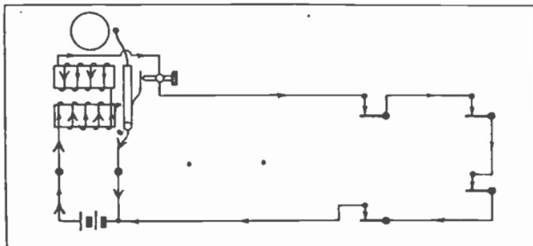
Fig. 20. Simple and economical barn or garage alarm of closed circuit type.
