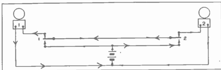
Fig. 14. Return call system using double circuit switches. Trace this circuit carefully.
