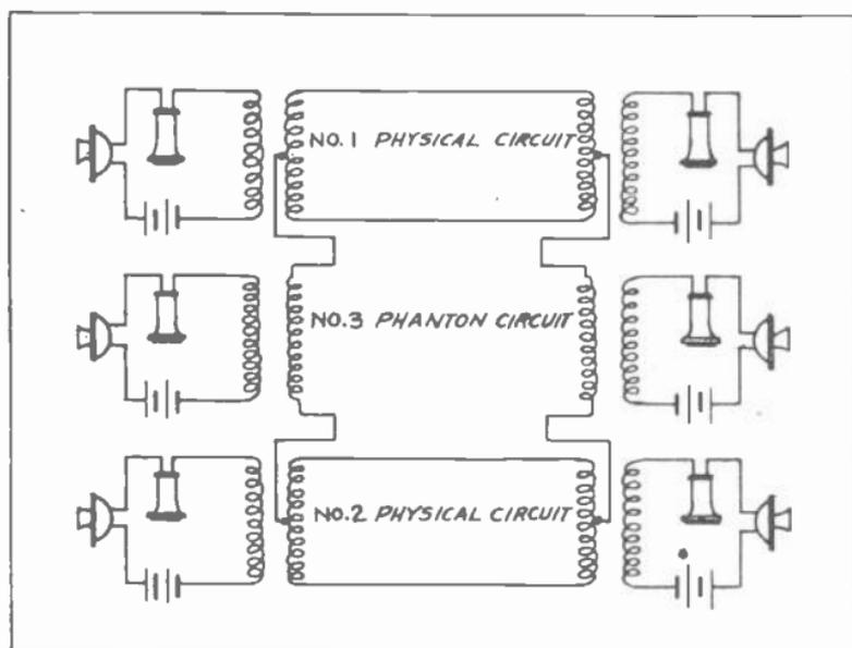
Fig. 15. Elementary sketch showing how a phantom circuit is obtained from two metallic or physical circuits.
