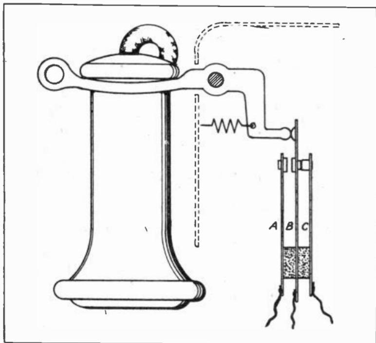
Fig. 12. Sketch showing the principle of a simple "receiver hook switch." Note what the operation of the spring contacts would be if the receiver was raised and lowered.
