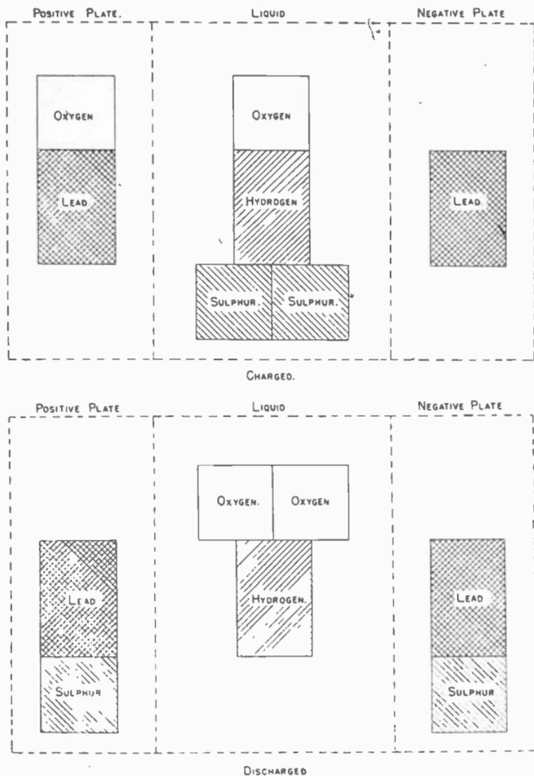
**Fig. 16. Chemical Changes in a Lead-acid Storage Battery Cell.**
