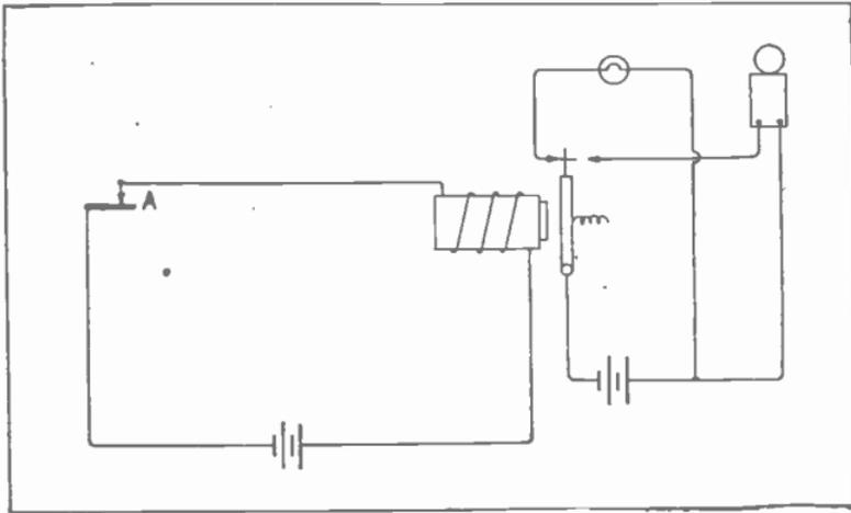
Fig. 28. Diagram and connections for a double circuit relay to operate a lamp when the system is undisturbed, and to ring a bell when the closed circuit is molested in any way.
