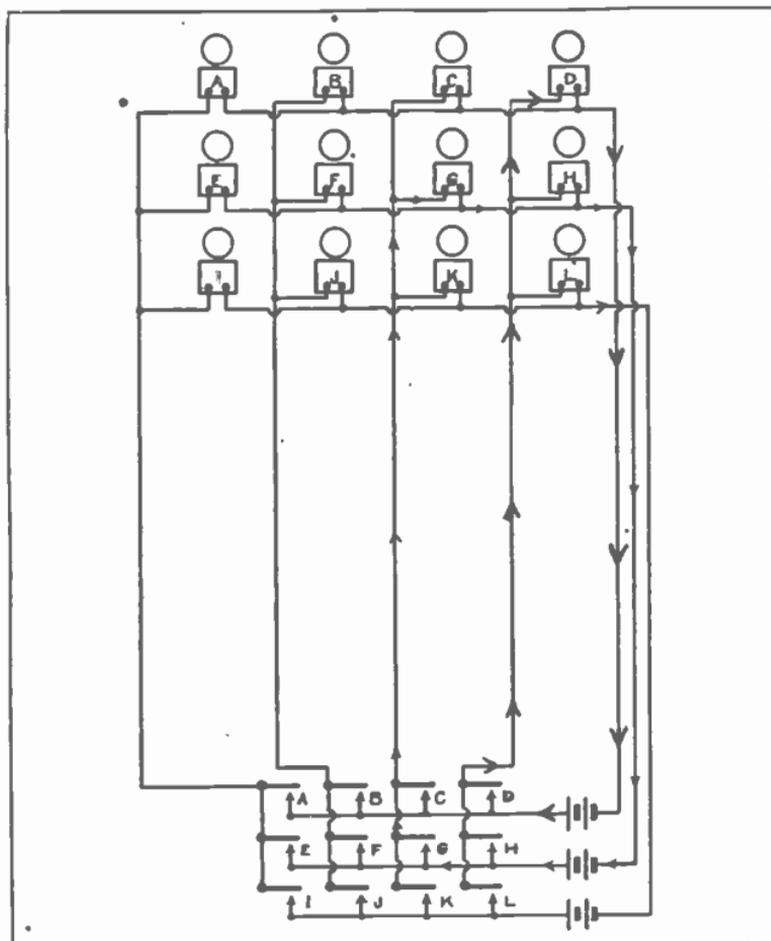
Fig. 25. "Group" method of connecting a large number of bells and switches to secure independent operation of each, with the least number of wires.
