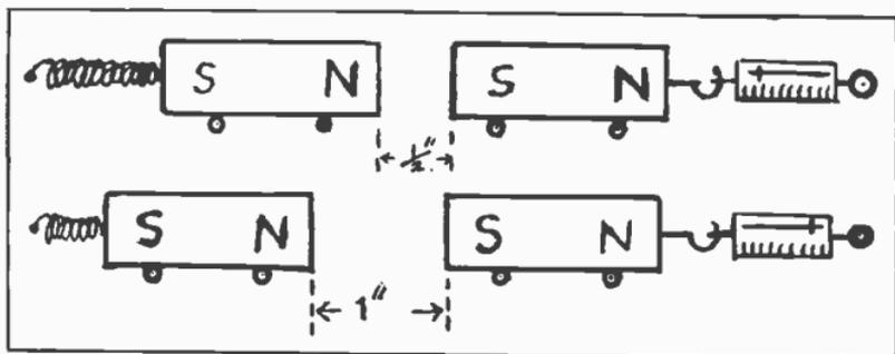
Fig. 82.-A. & B. Doubling the distance between two magnets, decreases their pull to  $\frac{1}{4}$  of what it was.
