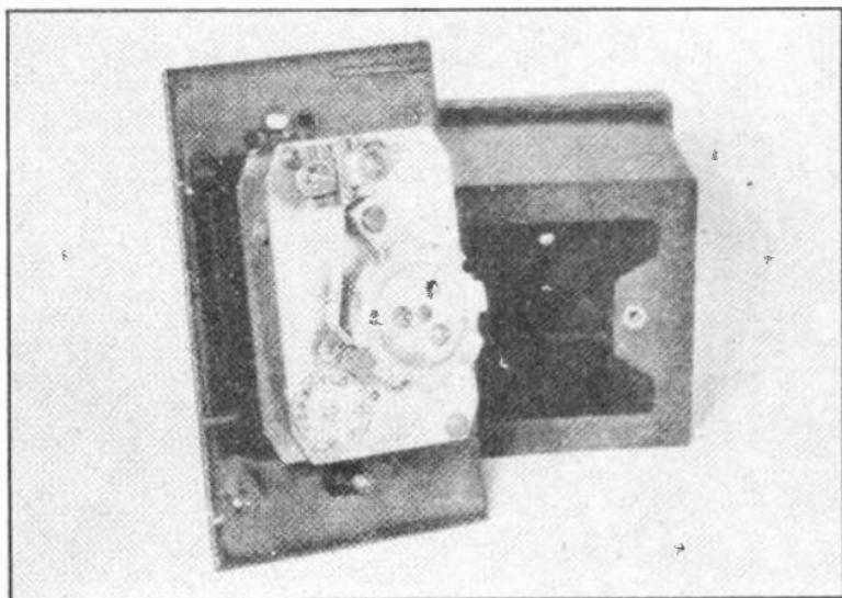
Fig. 13. Signal or alarm box of the code calling type, showing code wheel and contact springs.
