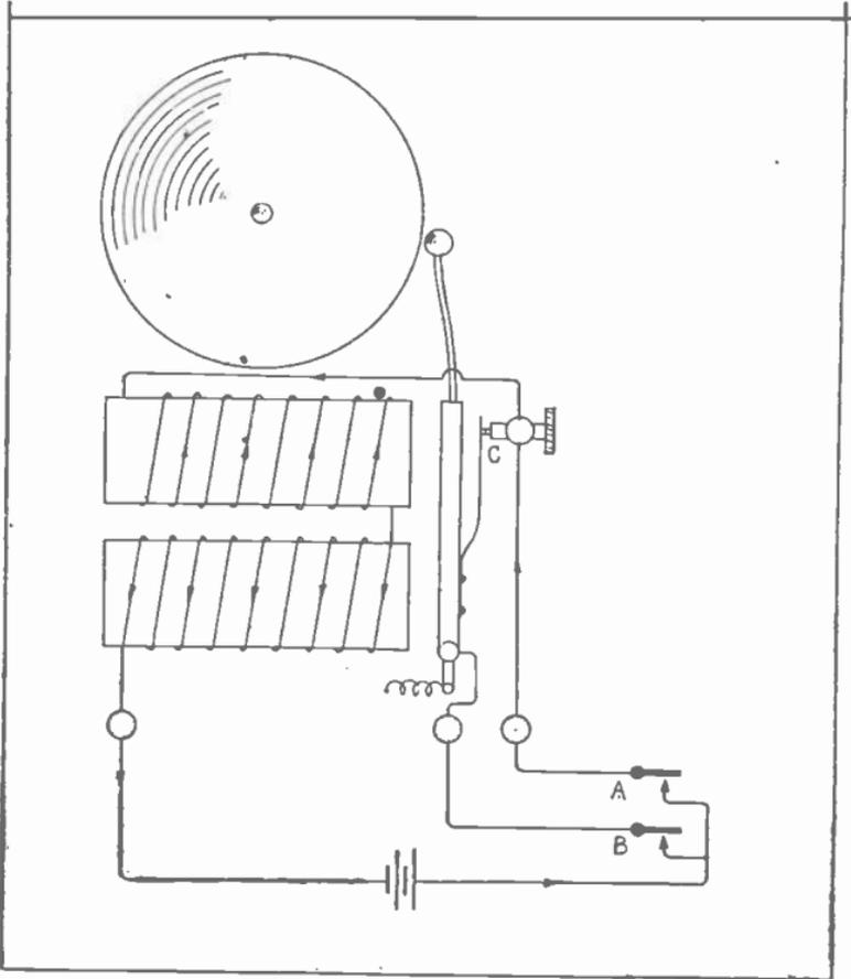
Fig. 6. Connections for a combination bell to be used either single stroke or vibrating. Trace this circuit carefully.
