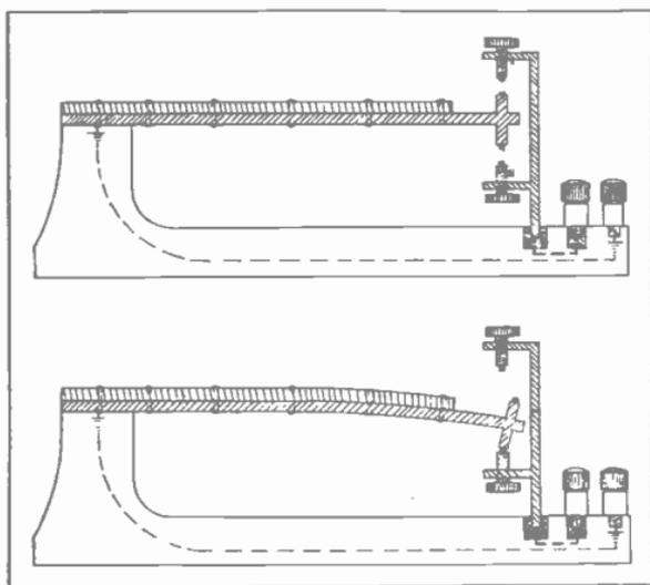
Fig. 28. Two sketches of thermostatic switch, showing the strip in normal position in the upper view, and warped to close the contacts in the lower view. Note how the circuit is completed through the metal frame of this device.
