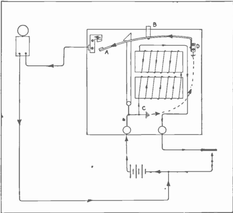
Fig. 18. Sketch showing complete circuit and connection of drop-relay of the type shown in Fig. 17. Examine this sketch and trace the circuit very carefully.
