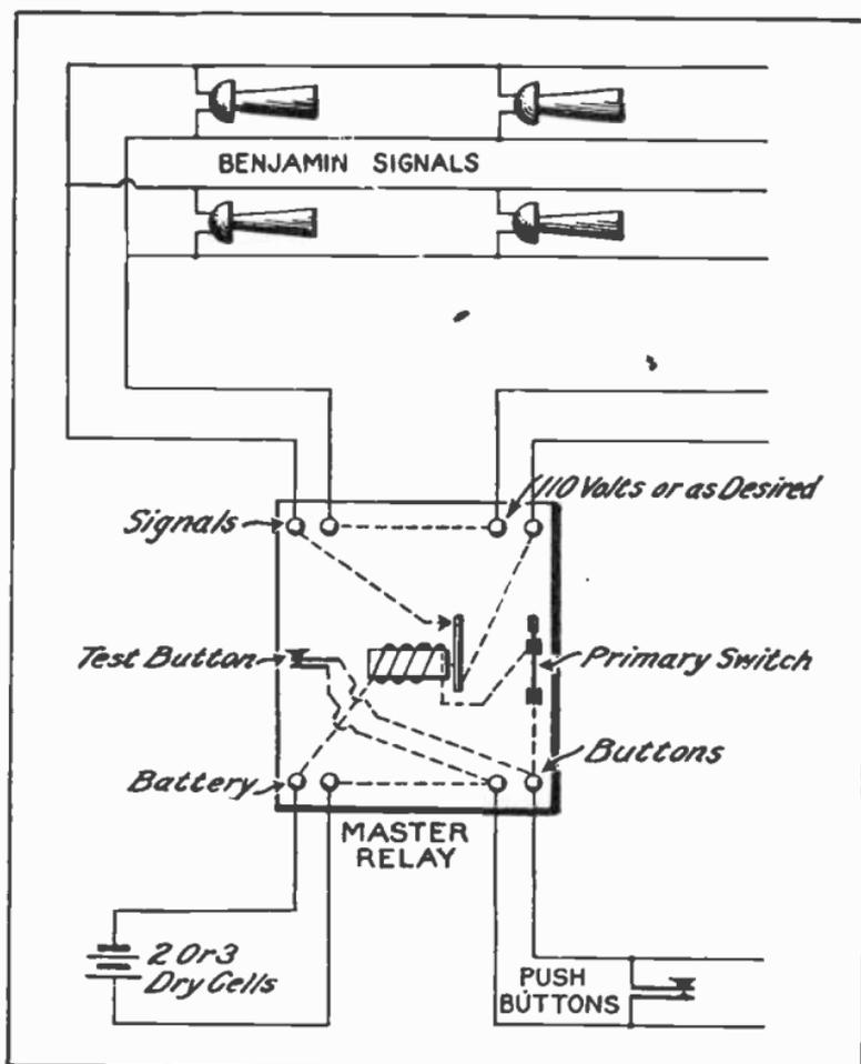
Fig. 23. Connection diagram for signal horns and Master relay. This relay operates on low voltage and very small current, and closes a high voltage, heavy current, circuit to the horns. (Courtesy Benjamin Electric Company.)
