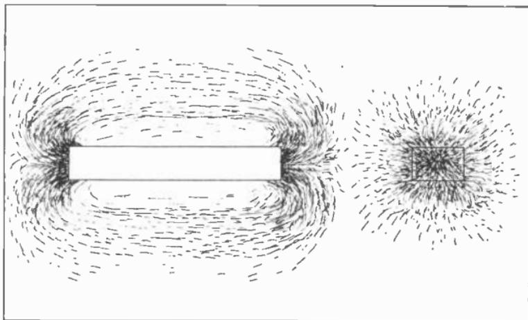
Fig. 71-A. Iron filings on a paper over a bar magnet, show shape of lines of force around the magnet. (Left).
