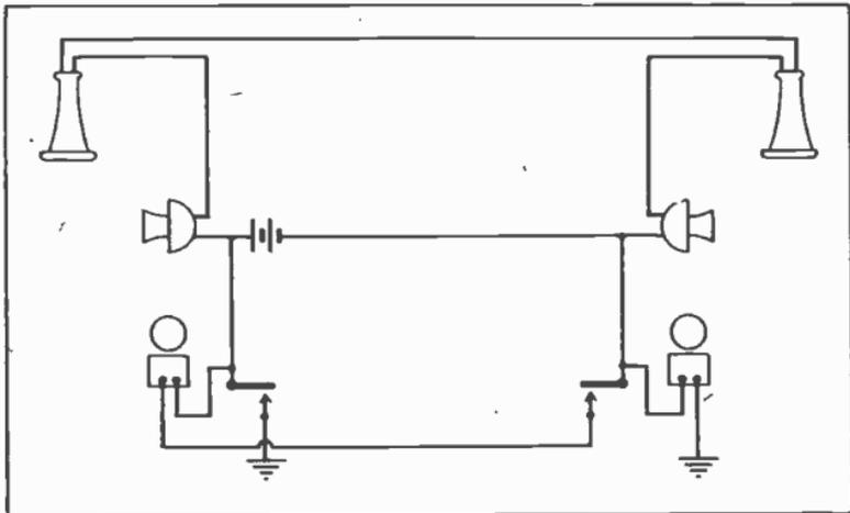
Fig. 5. Simple telephone system for two-way conversations, and including bells and buttons for calling the parties to the telephone.
