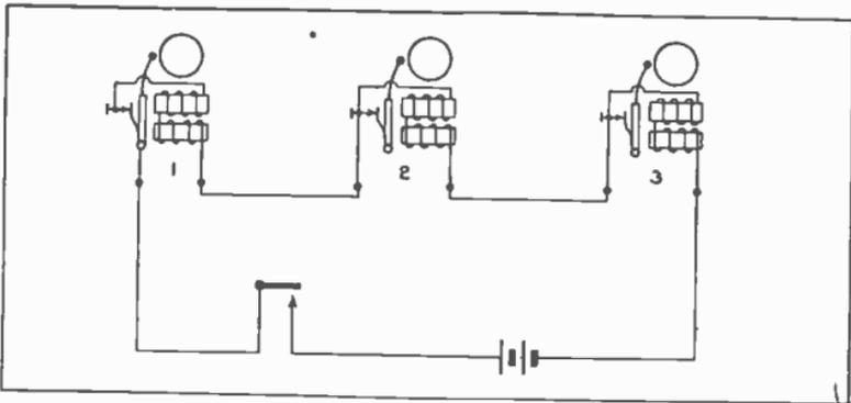
Fig. 19. This sketch shows the proper method of connecting vibrating bells in series, to secure best results.
