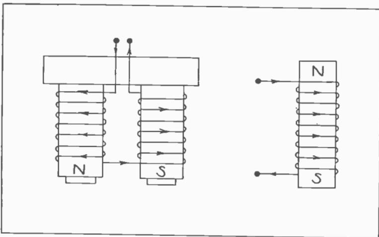
Fig. 104. Double and single electro-magnets.
