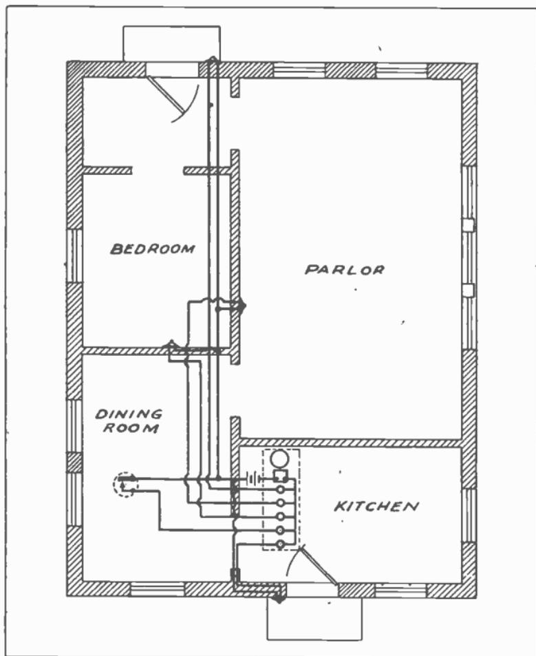
Fig. 6. Diagram showing layout of wiring for doorbell and convenience call system with annunciator. Such systems are commonly used in modern homes and are very well worth their cost of installation.
