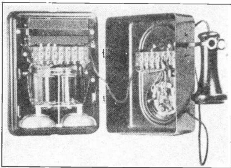
Fig. 5. Photograph of wall type telephone for central energy systems.
