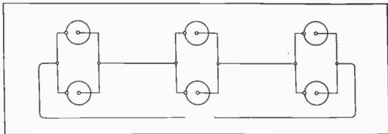
Fig. 50. Six Dry Cells Connected In Parallel-series.
