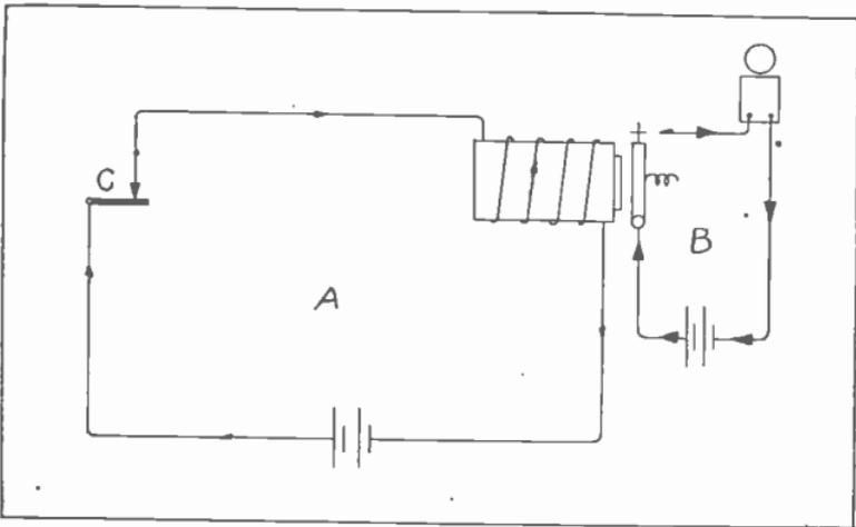
Fig. 25. Connections for a closed circuit relay used to operate a bell in a simple burglar alarm system.
