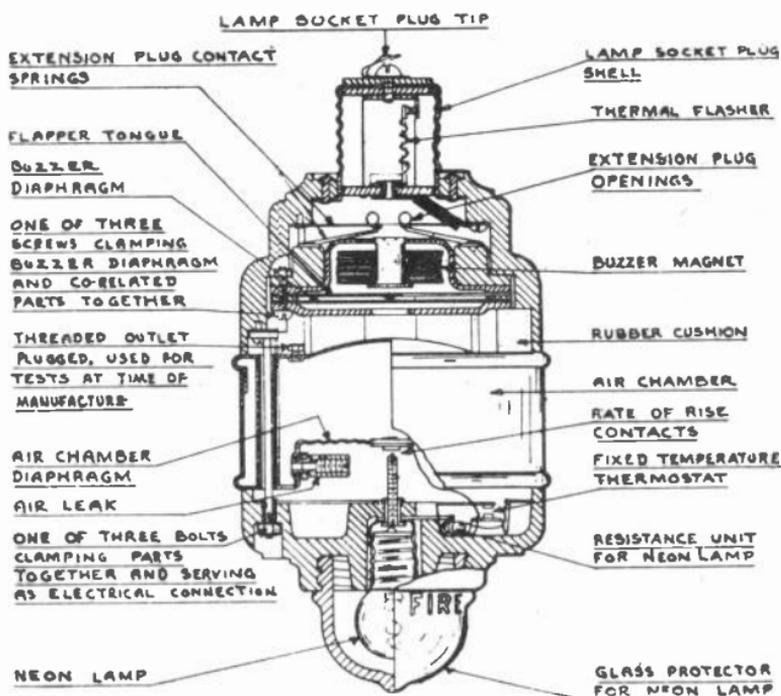
Fig. 26. A complete sectional drawing showing all of the parts used in the alarm unit shown in Fig. 25.
