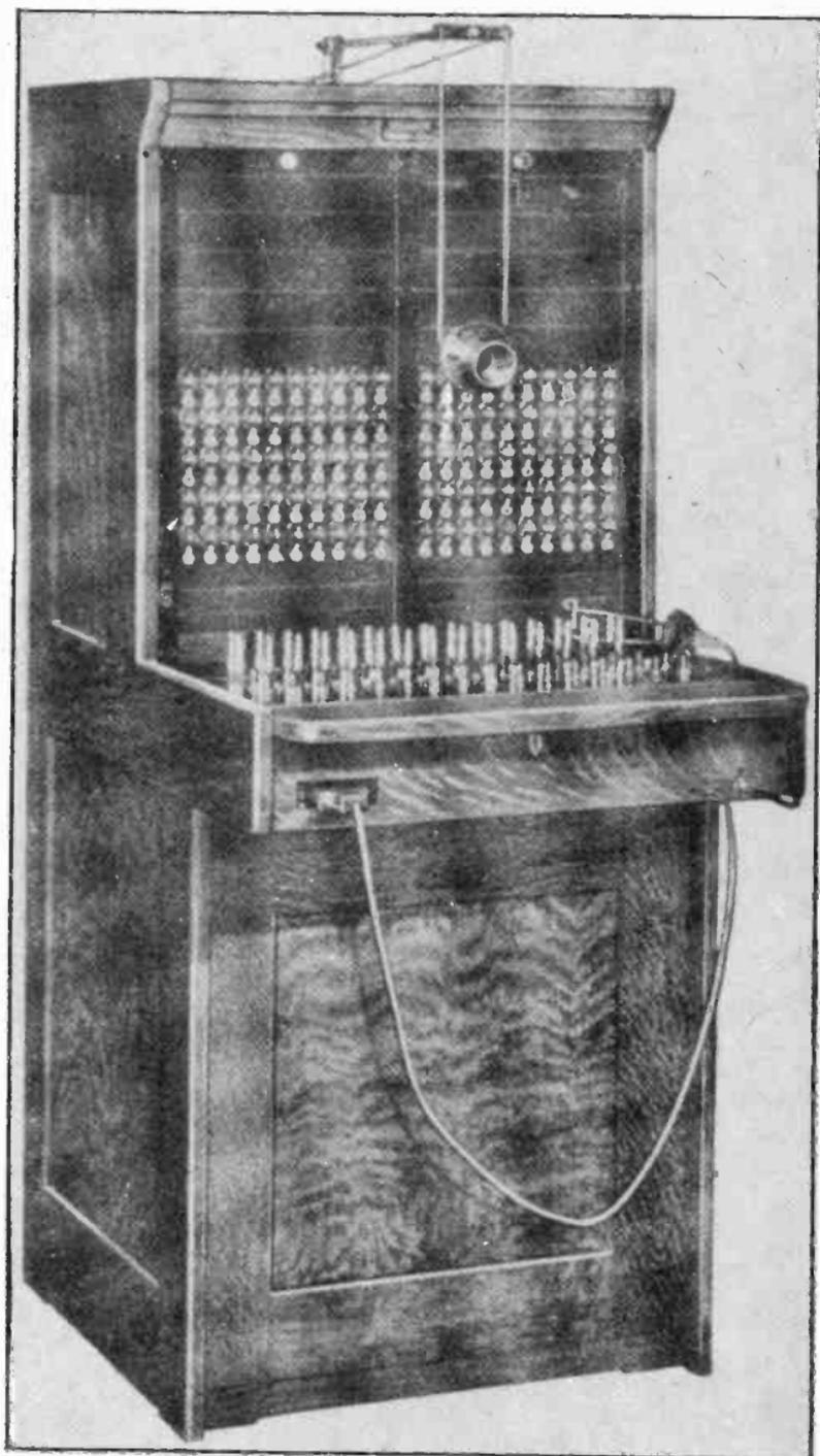
Fig. 7. A small exchange switchboard of the magneto type, showing plugs, jacks, and the operator's transmitter and receiver.
