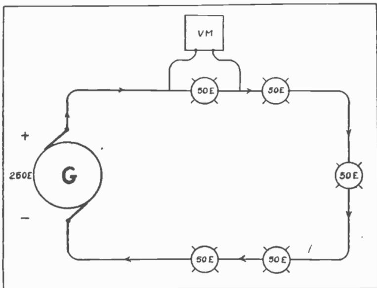
Fig. 26. Five 50-volt Lamps Connected In Series.
