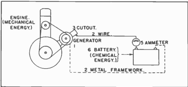
Fig. 9 A Portion of the Auto-electric System.
