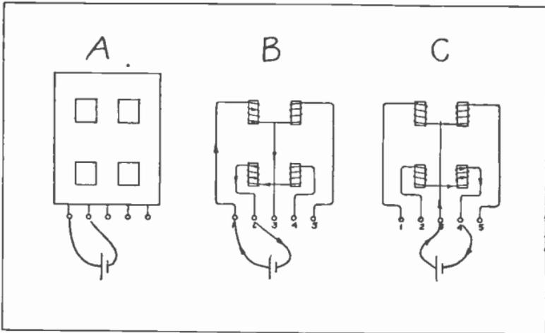
Fig. 5. Observe these test diagrams very carefully with the instructions given for locating annunciator terminals.
