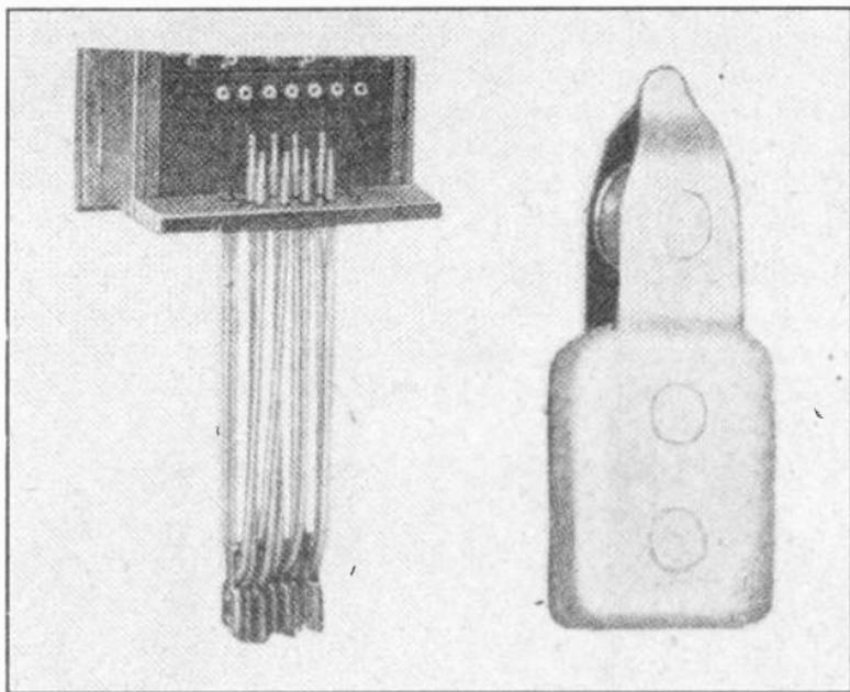
Fig. 8. The view on the left shows the manner in which the plug cords are held straight by the weighted pulleys. A larger view of one of these pulleys is shown on the right.
