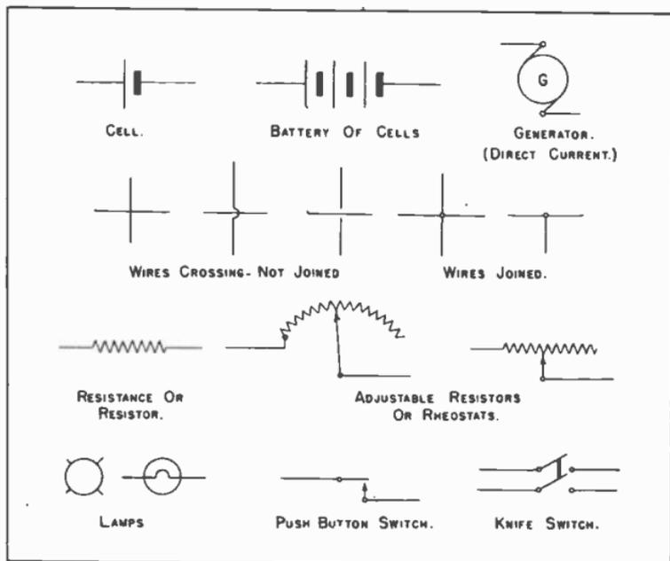
Fig 22 Symbols Used In Electrical Wiring Diagrams.
