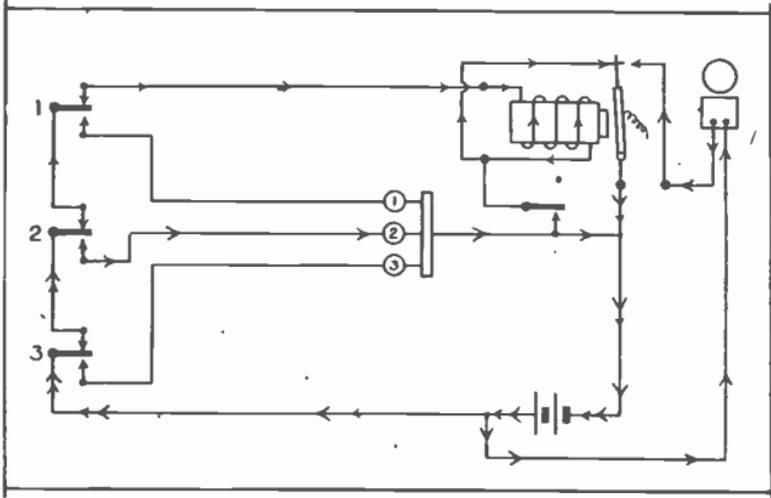
Fig. 5. Combination alarm system using double circuit switches to operate both the holding relay and the annunciator.
