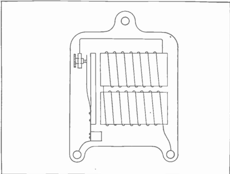
Fig. 9. Sketch showing coils and circuit of a buzzer of the type shown in Fig. 8.
