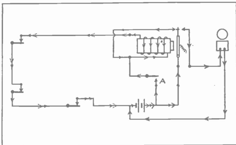
Fig. 3. Double circuit holding relay used in a closed circuit burglar alarm system. This is a very simple and efficient alarm circuit.
