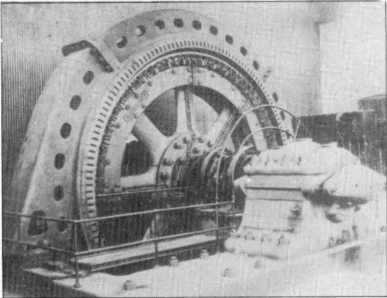
Fig. 8. Type 1-28/56-6500 HP 107/53-6600 Volt Form M Induction Motor with changing switch installed in the 60 in. Universal Plate Mills, Illinois Steel Company, Gary, Indiana.
