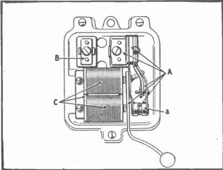
Fig. 3. Heavy duty bell frame and parts. Note the extra heavy carbon contacts for making and breaking the circuit at "a."
