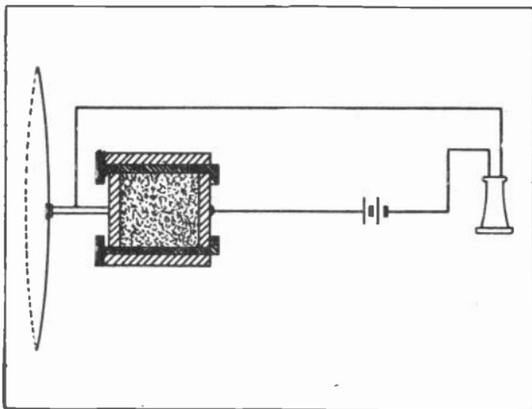
Fig. 7. Simple sketch showing principle of telephone transmitter button, and how the varying pressure on the carbon granules varies the resistance and current flow in the circuit.
