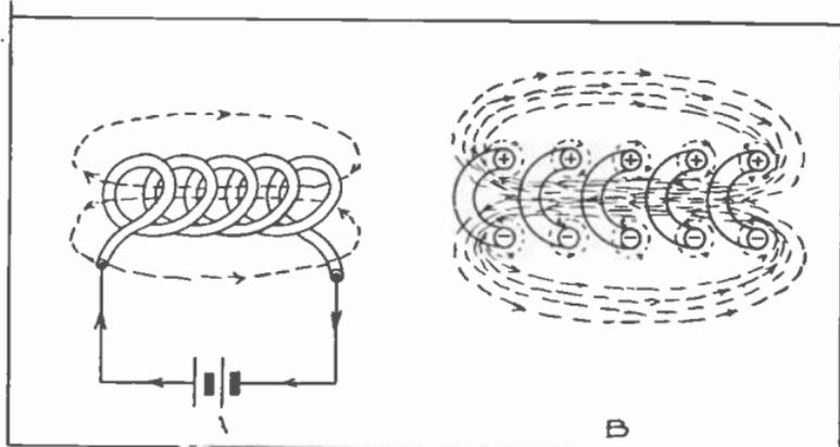
Fig. 93-A. The lines of force around the turns of a coil join together, in one very strong field.
