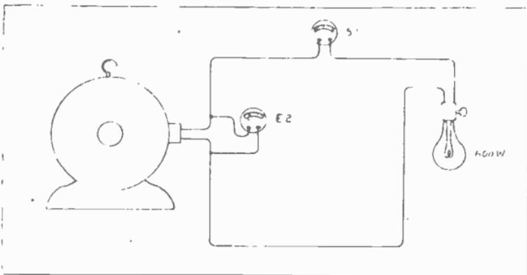
Fig. 9. Generator supplying 5 amps to a 600 watt lamp. What is the generator voltage?
