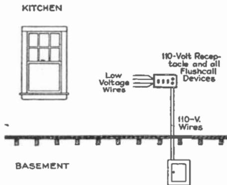
Fig. 9. An installation where the flush type equipment is used requires less wire as shown by the above figure. Compare this diagram with Fig. 8. (Courtesy Edwards & Co.)
