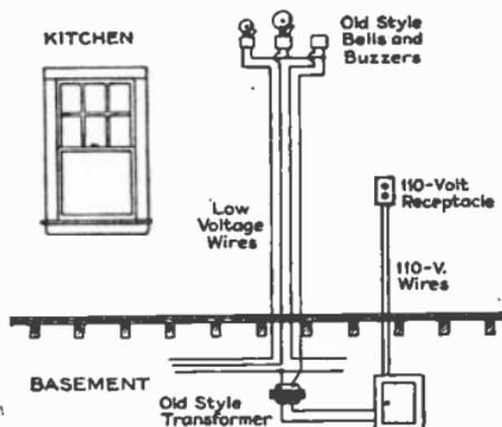
Fig. 8. A typical signal installation showing the wiring required when using regular bell and buzzer signals.
