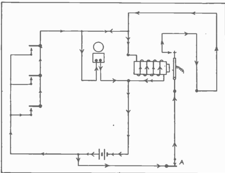
Fig. 2. Open circuit alarm system using a holding relay for constant ringing when alarm is tripped.
