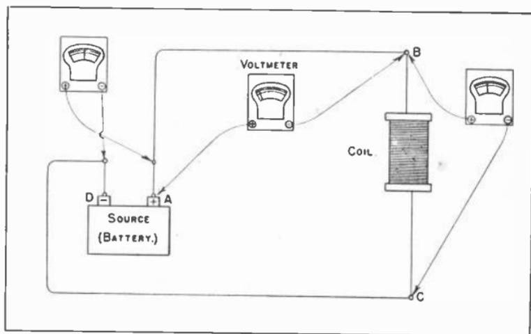
Fig. 20. Using a Voltmeter To Measure Potential Differences.
