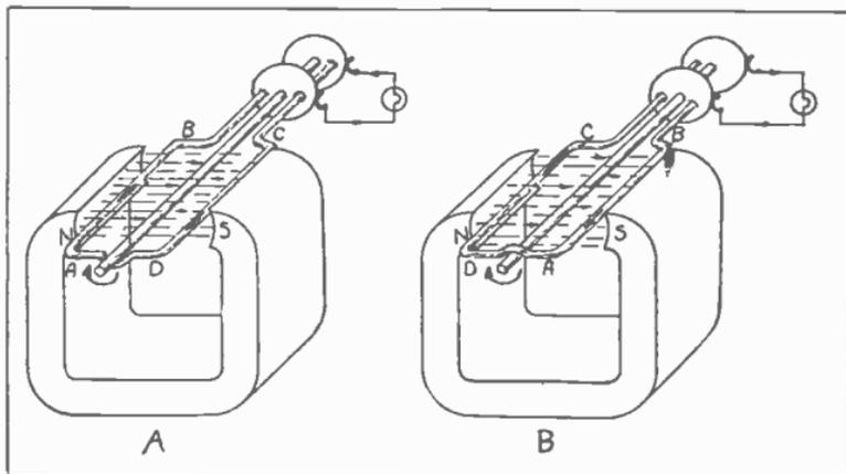
Fig. 111-A. Simple electric generator of one single wire loop, in the flux of a strong permanent magnet.
