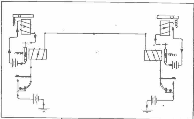
Fig. 27. Sketch of simple telegraph system showing line and ground circuit for the relays and keys, and local battery circuits for the sounders.
