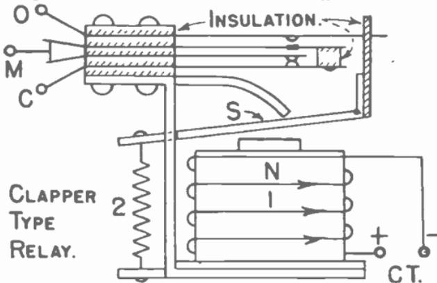
it out as soon as the coil is deenergized. The moving section should not touch the core, and the tension on the spring should not be too low or too high. The relay switch contacts must be clean.
