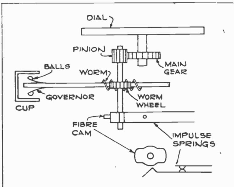
Fig. 2. This sketch shows the mechanism and operating principles of the dial and impulse springs.
