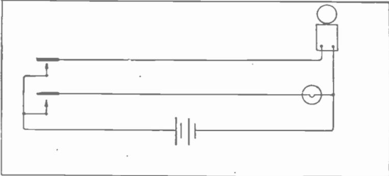
Fig. 14. Connections for operating either a bell call or silent lamp signal, as desired.
