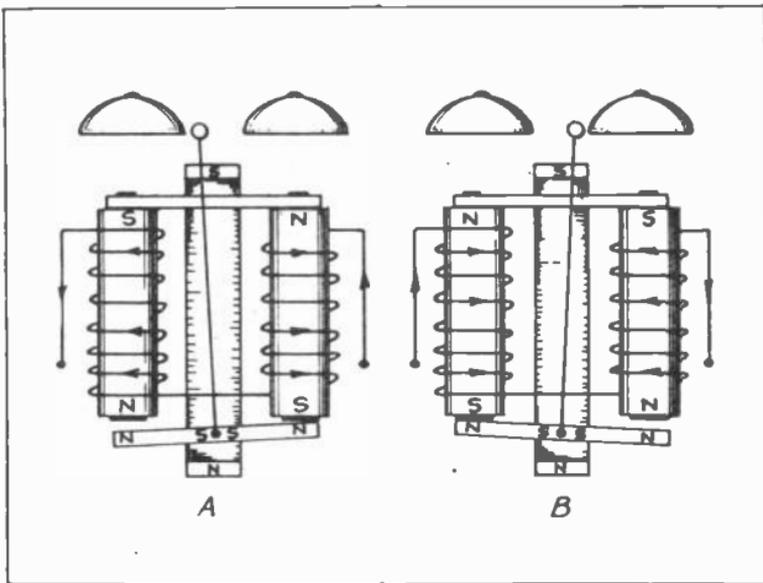
Fig. 17. These sketches show the electrical circuit of a polarized telephone bell. Note the polarity and position of the armature in "A," and again in "B," after the current has been reversed.
