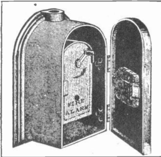
Fig. 10. This is a fire alarm "pull box" which sends in numerical or code signals to indicate its location.
