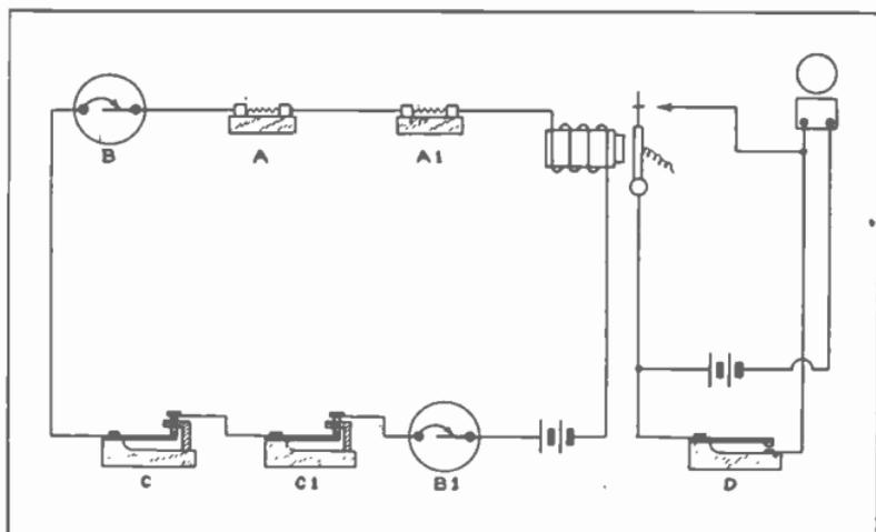
Fig. 17. This sketch shows the connection of several different types of fire alarm switches in one system.
