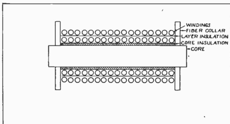
Fig. 101. Sectional view of electro-magnet, showing core, insulation and winding.
