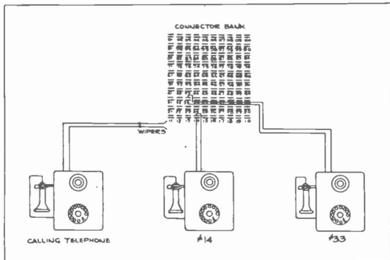
Fig. 6. Simple sketch showing the arrangement and principle of the connector bank of an automatic exchange.
