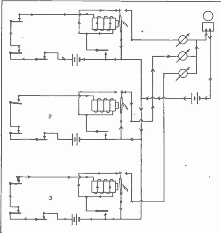
Fig. 4. Closed circuit burglar alarm system of three sections, each using holding relays for constant ringing; and an annunciator to indicate point of disturbance.
