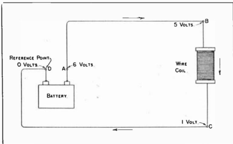
Fig. 18. Electric Circuit In Which There Are Drops of Potential and Differences of Potential.
