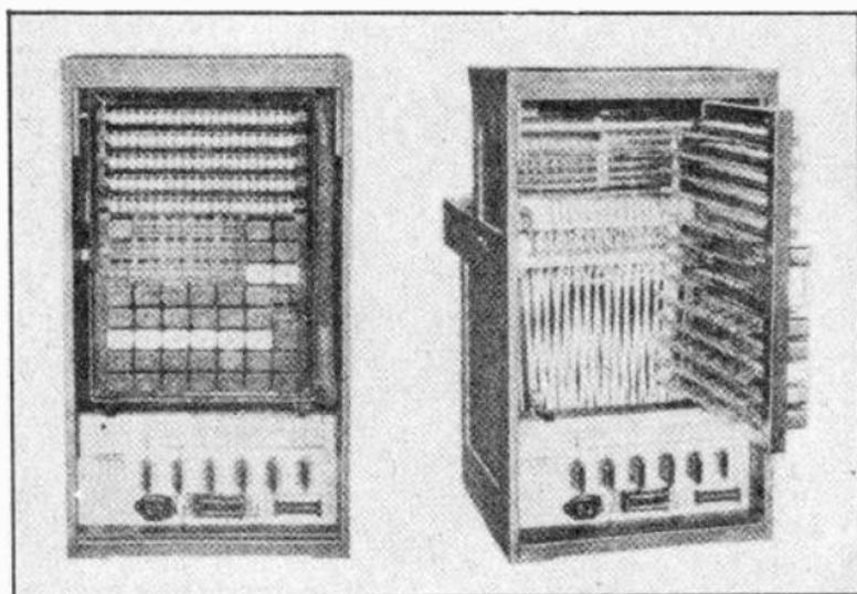
Fig. 18. These two views of the rear of a switchboard show the relays, drops, and cords very clearly. Note the neat and compact arrangement of all parts and wires.
