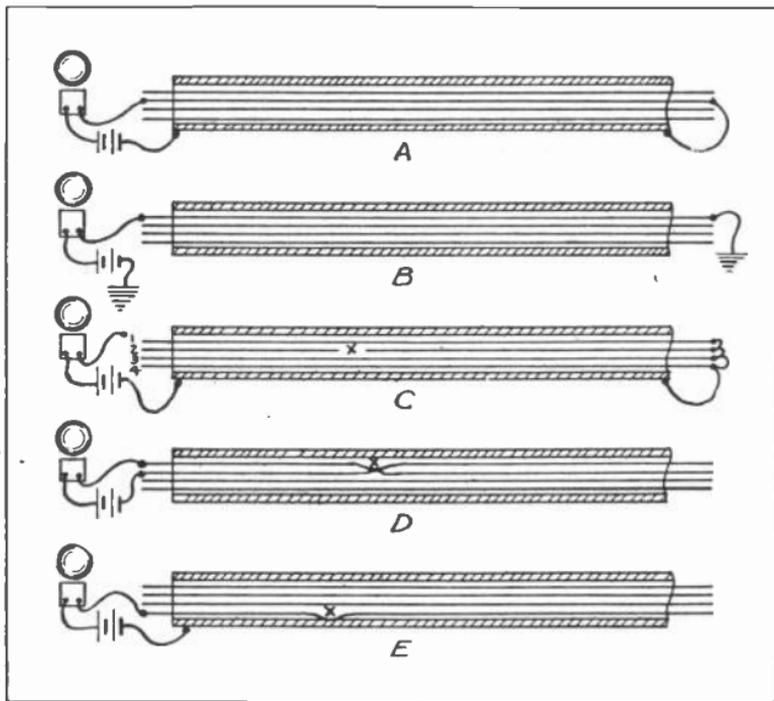
Fig. 2. Sketches showing methods of testing for various faults in wires run in conduit. Compare carefully with test instructions given.
