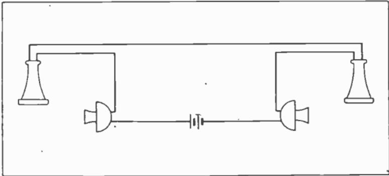
Fig. 4. Two transmitters and two receivers connected in series to form a simple two-way telephone circuit.
