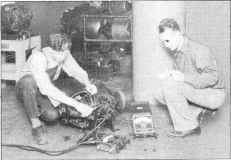
Fig. 15. Using Meters To Test the Operation of an Electric Motor.
