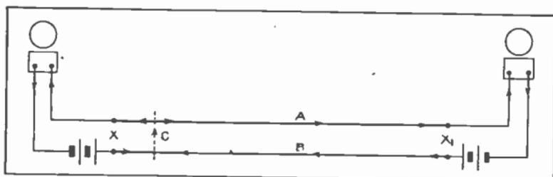
Fig. 16. Mine signal or alarm circuit which uses no switches. The bells are caused to ring by short circuiting wires "A" and "B".
