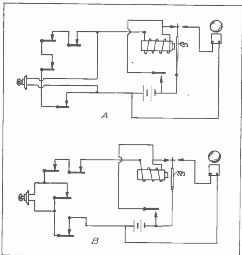
Fig. 8. These circuits "A" and "B" show two different methods of connecting a lock switch to a burglar alarm circuit.
