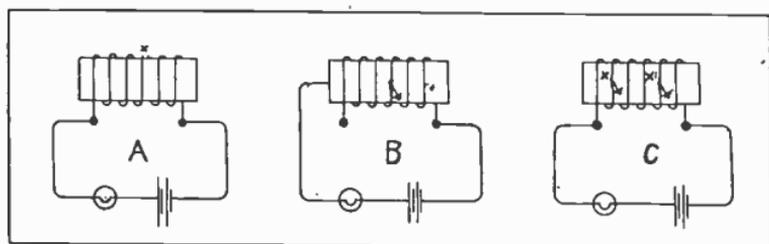
Fig. 102. Methods of testing coils for faults.
