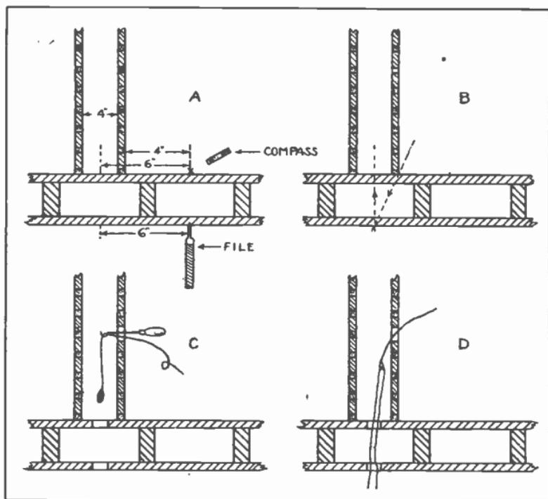
Fig. 1-A. Sketch showing uses of magnetized file and compass to locate spot to drill for wires. "B," dotted lines show how the "feeler drill" can be used. "C," dropping a "mouse" on a string, through holes in wall and floor. "D," pulling the wires in with the cord which was attached to the "mouse."
