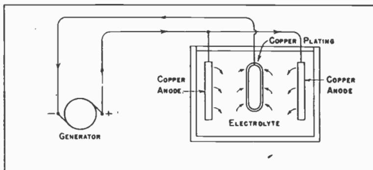
Fig. 63. Plating With Anodes of the Metal Being Plated.
