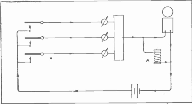
Fig. 6. Diagram showing connections of a three-drop annunciator in an open circuit signal system. This annunciator uses a ballast coil shown at "A," and connected in parallel with the bell to allow the proper amount of current to flow to operate the drops.
