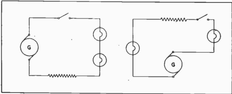
Fig. 24. Series Circuits.
