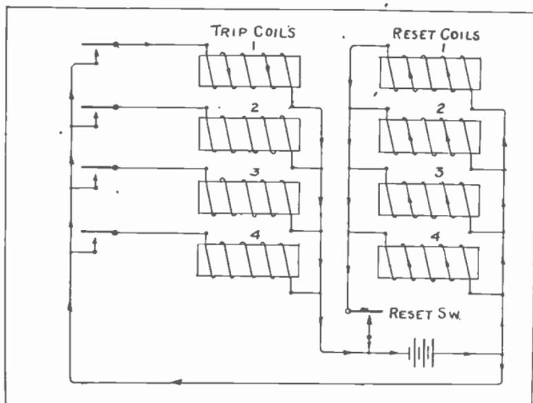
Fig. 8. Complete diagram of a four-drop annunciator using "electrical reset" magnets.
