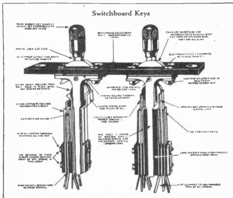
Fig. 10. Here we have an excellent view of two key switches, showing how the key levers and rollers operate the spring contacts, and open and close various circuits.
