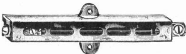
Fig. 16. One type of thermostatic fire alarm switch, that can be adjusted to open or close an alarm circuit by expansion at temperatures above normal.
