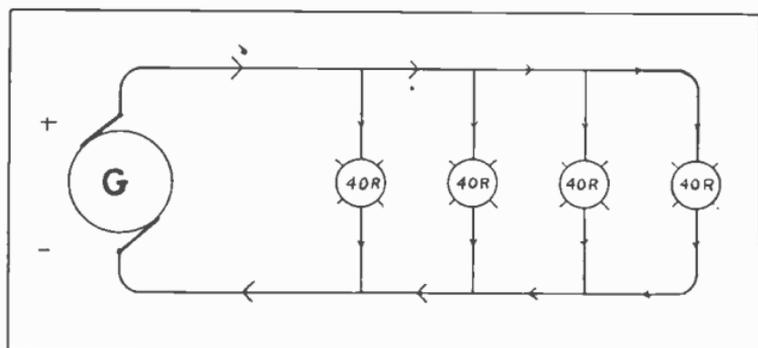
Fig. 39. Equal Resistances In Parallel.
