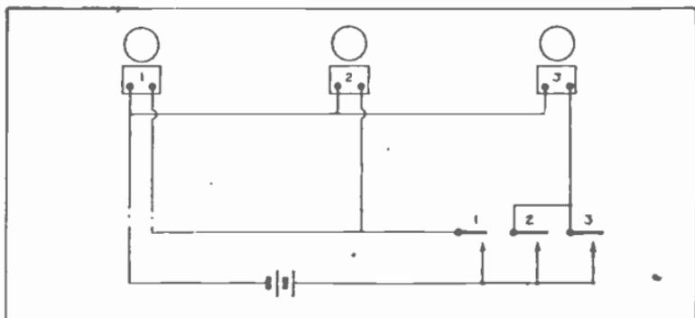
Fig. 11. Selective call system. Button No. 1 will ring bells 1 and 2; buttons Nos. 2 and 3 will ring bell No. 3.
