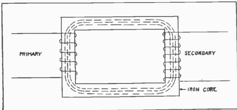
Fig. 116. Core and windings of a simple transformer.
