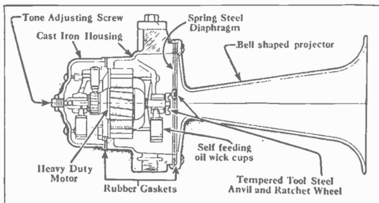
Fig. 22. Sectional view showing parts and construction of motor operated horn. (Sketch courtesy of Benjamin Electric Company.)
