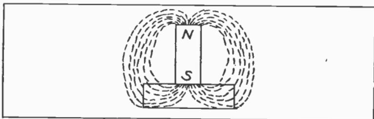
Fig. 81. Bar magnet attracting a piece of iron. Note the long path through air, which the lines of force must take.
