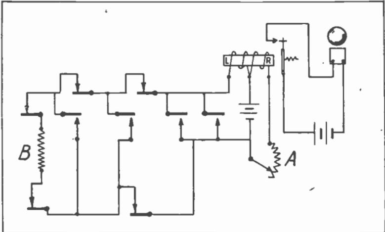
Fig. 7. Balanced resistance alarm circuit. This is a very dependable alarm system, as it is almost impossible to tamper with it without causing the alarm to sound.
