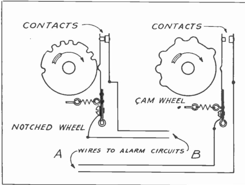
Fig. 12. This sketch shows the arrangement of the code wheel and contacts of closed and open circuit code call systems.
