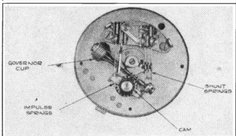
Fig. 4. This photograph shows an excellent view of the impulse springs and cam, shunt springs, and governor of a dial.
