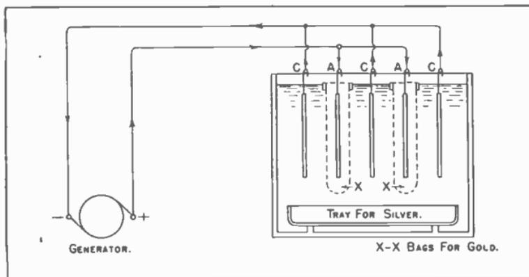
Fig. 65. Cell for Electrolytic Refining of Silver.
