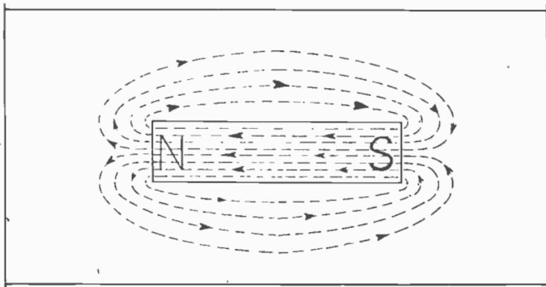
Fig. 72. Sketch of magnetic field, showing direction of lines, inside and outside the magnet.
