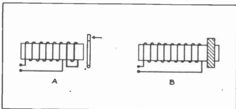
Fig. 10. Two types of slow acting relays. The one on the left has a short-circuited coil of a few turns, and the one on the right has a larger copper ring around the end of the core.
