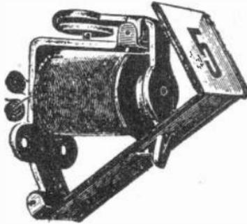
Fig. 3. This view shows the mechanical construction of one type of annunciator drop. Note how the drop is held up by a small hook on the end of the armature.
