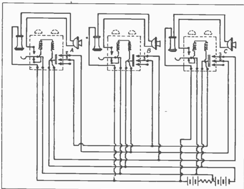
Fig. 25. Wiring diagram of three telephones on an inter-communicating system.
