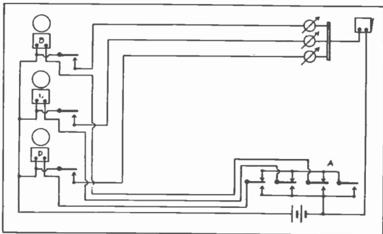
Fig. 24. Selective signal circuit with Master Control, return call and annunciator features. This is a very popular form of signal system.
