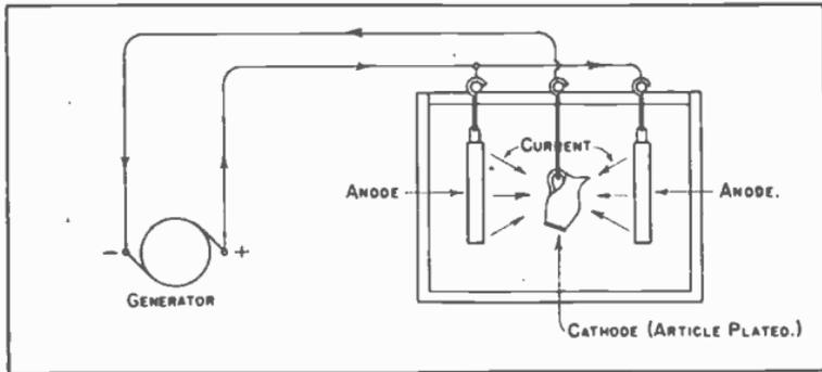
Fig. 62. Principle of Electroplating.
