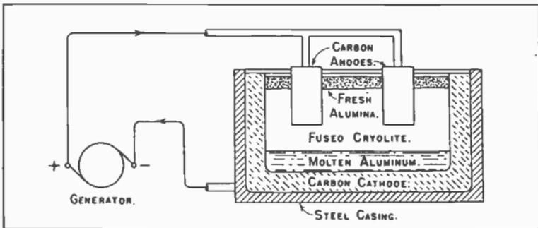
Fig. 66. Electrolytic Furnace for Producing Metallic Aluminum.
