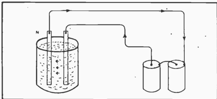
Fig 13. A "Voltammeter" Which Measures Quantities of Electricity.
