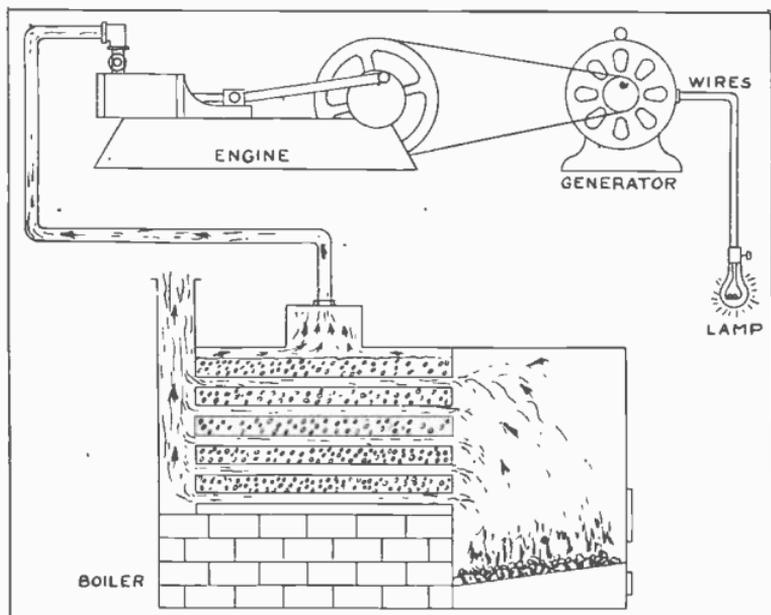
Fig. 6. Sketch showing how heat energy of coal is changed into mechanical energy by the engine, then to electrical energy by the generator, and into heat and light again by the lamp.
