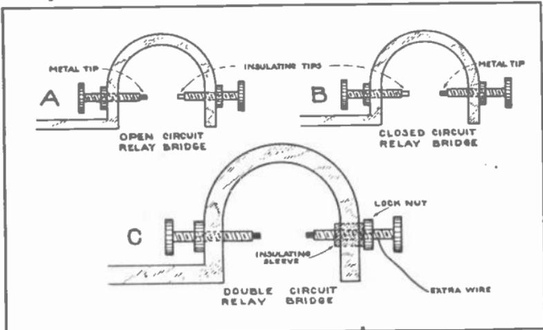
Fig. 24. This sketch shows in detail the manner of arranging and insulating relay bridges for open circuit, closed circuit, and double circuit operation.
