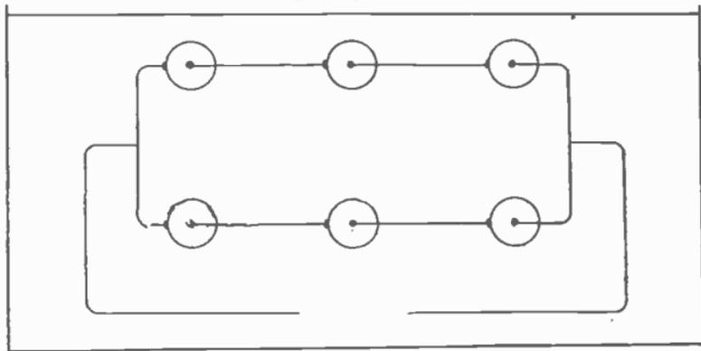
Fig. 49. Six Dry Cells Connected In Series-parallel.
