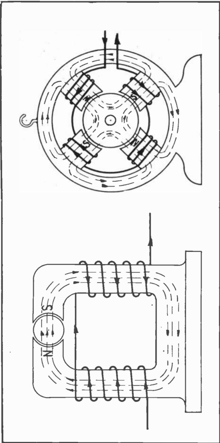
Fig. 106-A. Flux path in a simple early type of motor.
