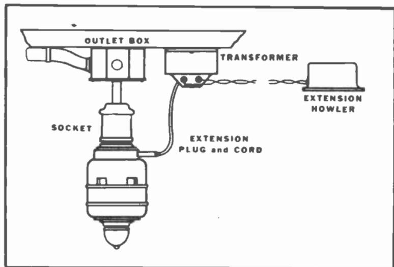
Fig. 28. A vitalarm fire detector installation showing an extension howler connected through a transformer.
