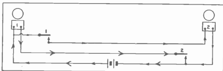
Fig. 12. Return call system. Button No. 1 will ring bell No. 2; button No. 2 rings bell No. 1.
