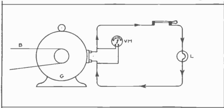
Fig. 34. Electric Circuit With Its Parts In Series.
