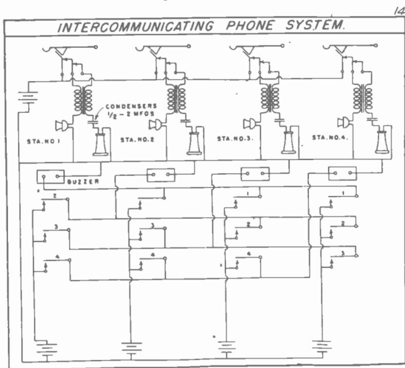
With the arrangement shown, the person at any station may call any other station by merely pressing the appropriate switch; this action operates the buzzer at the called station. When the receivers are lifted, the phones are connected as shown in the diagram, for the hook switches open all transmitting and receiving circuits when they are down. Examination of the sketch shows that a person at any station can call and talk to any or all other stations.
