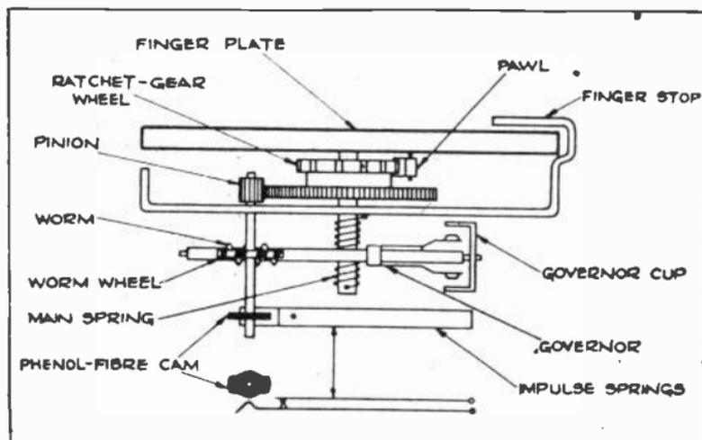
Fig. 3. Another view showing some parts of the dial mechanism more clearly.
