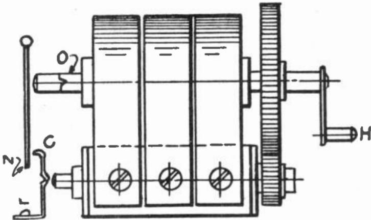
Fig. 21. Diagram of telephone magneto showing shaft extension which operates contact springs.
