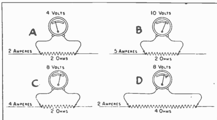
Fig 27 Relations Between Amperes, Volts and Ohms.
