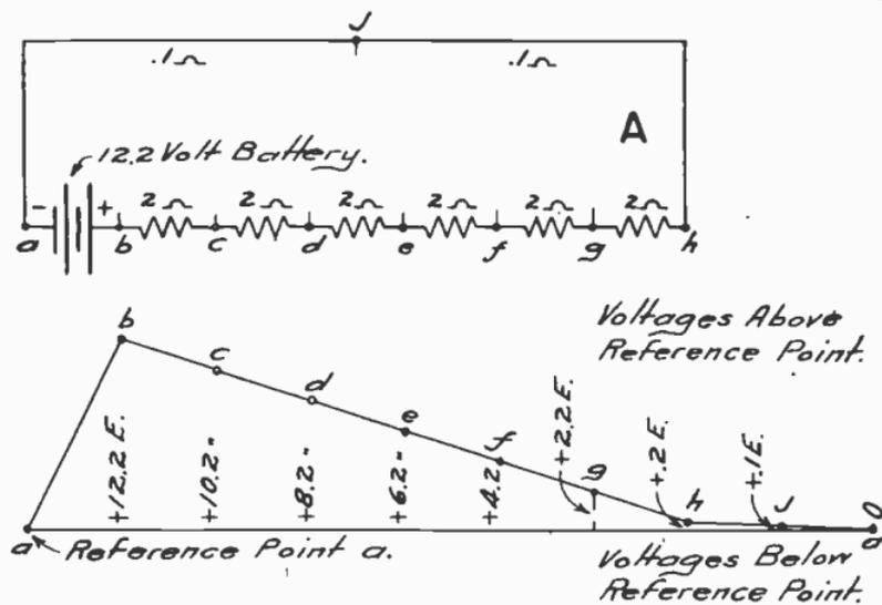
Thus point "d" in Fig. A is marked +8.2 in Fig. C, whereas point "h" is marked +2, for the last figure indicates that point "h" has a pressure that is 8.0 volts below point "d".
