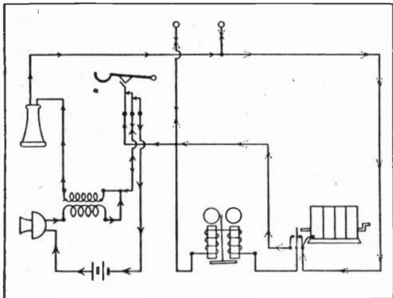
Fig. 3. Circuit diagram of another telephone using a different hook switch and set of magneto contacts. Trace the circuit carefully and observe its operation.
