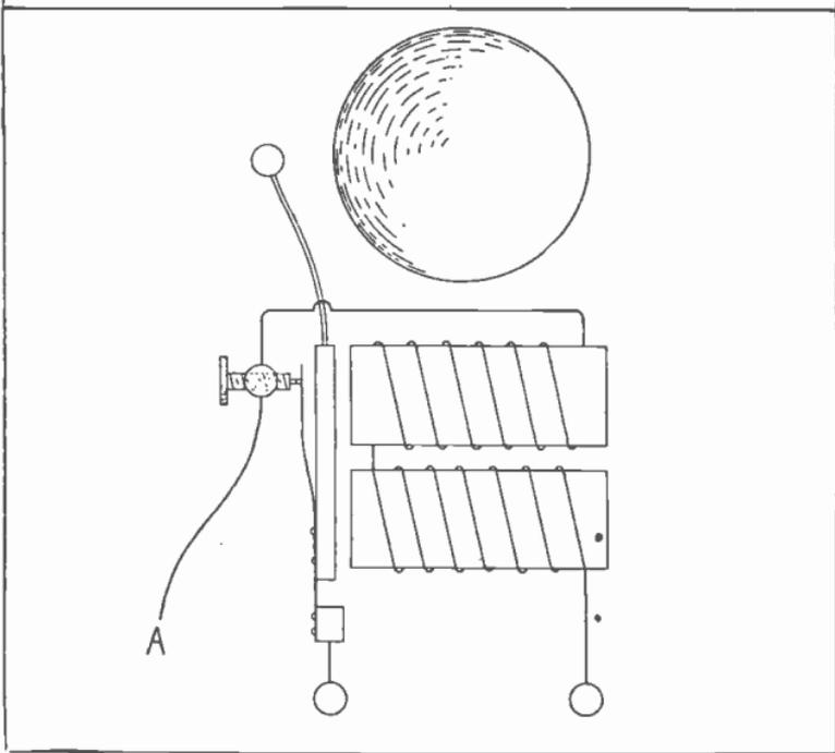
Fig. 7. Sketch showing method of attaching an extra wire to the stationary contact to convert an ordinary vibrating bell for single stroke or combination operation.
