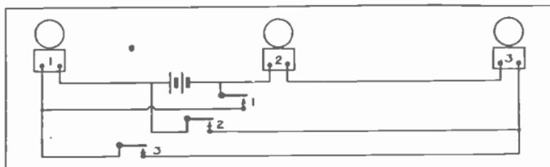
Fig. 17. Selective signal circuit. Check its operation carefully with the instructions.
