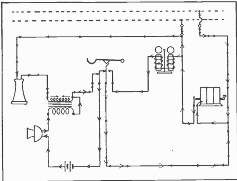
Fig. 2. Diagram showing connections and circuits of a telephone such as shown in Fig. 1.
