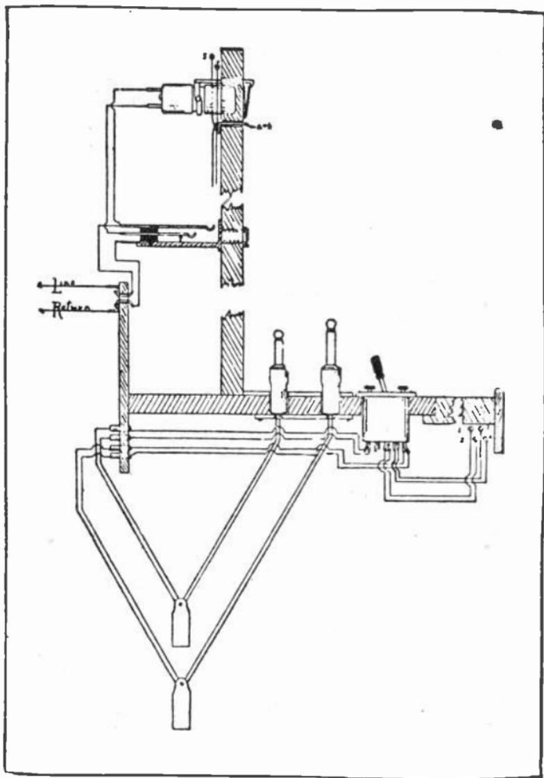
Fig. 16. This simple sketch shows the general operating principle of a manual switchboard.
