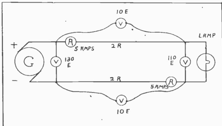
Fig. 12. Generator, lamp and meters connected for testing "voltage drop" and proving Ohms Law Formulas. This is typical of problems encountered by the head electrician in the field.
