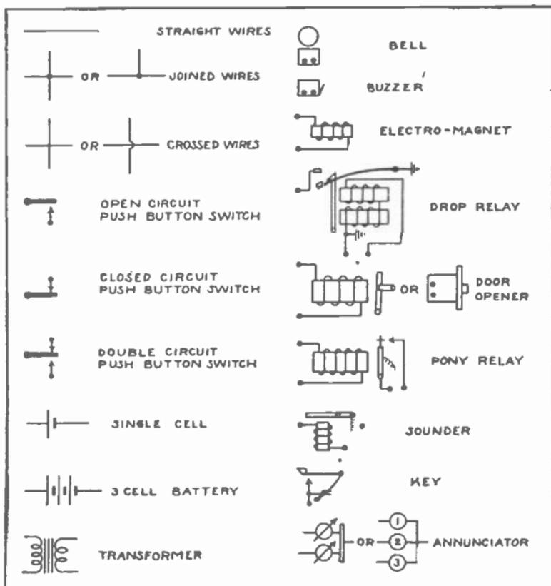
Fig. 9. These are some of the most important symbols used in signal diagrams and circuits. They should be memorized so you can easily recognize them when tracing any diagram in the future.
