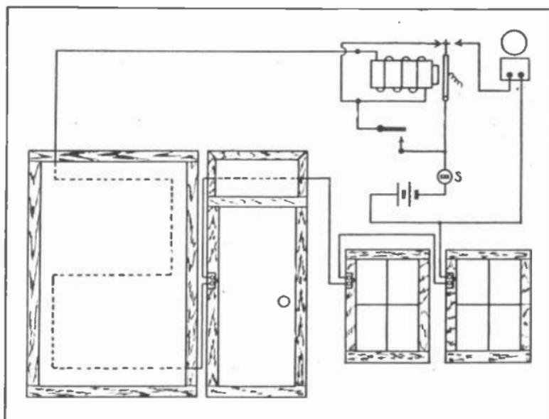
Fig. 6. This diagram shows the use and application of burglar alarm foil for the protection of glass windows and doors.
