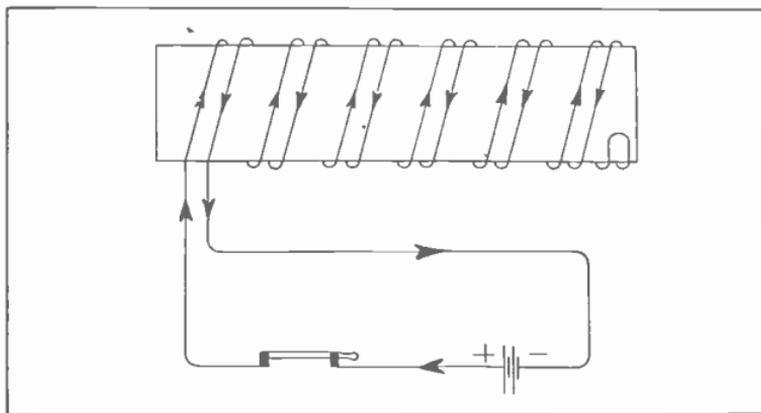
Fig. 99. Non-magnetic winding. One half of the turns oppose the other half, so the core does not become magnetized.
