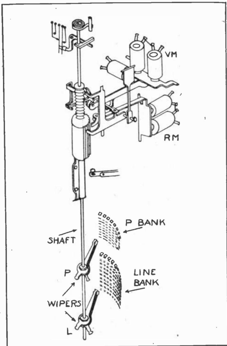
Fig. 7. This diagram shows the arrangement of the selector mechanism with its vertical magnets, rotary magnets, wipers, and wiper shaft.
