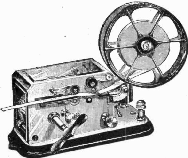
Fig. 15. Recording device for receiving code calls on paper tape. Fire and police departments use such recorders.
