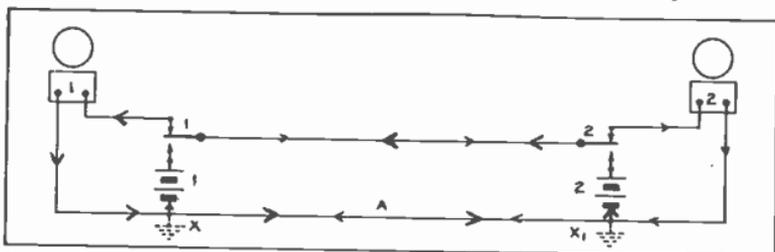
Fig. 15. Return call system showing how wires can be saved by the use of double circuit switches, two separate batteries, and a ground circuit.
