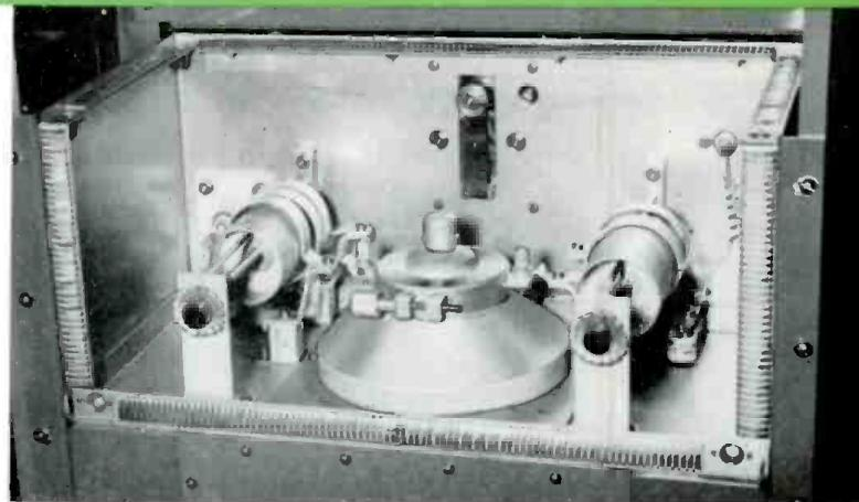
R-f cavity with shielded cover removed.
