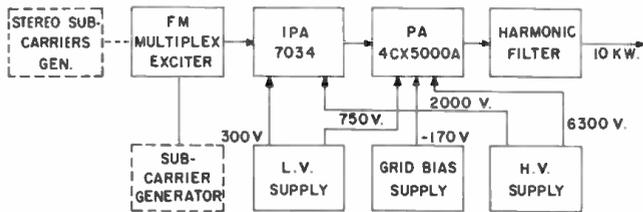
Block diagram of the BTF-10D 10 KW Transmitter.
