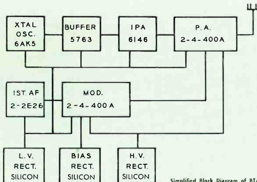
Simplified Block Diagram of BTA-1R1 AM Transmitter.
