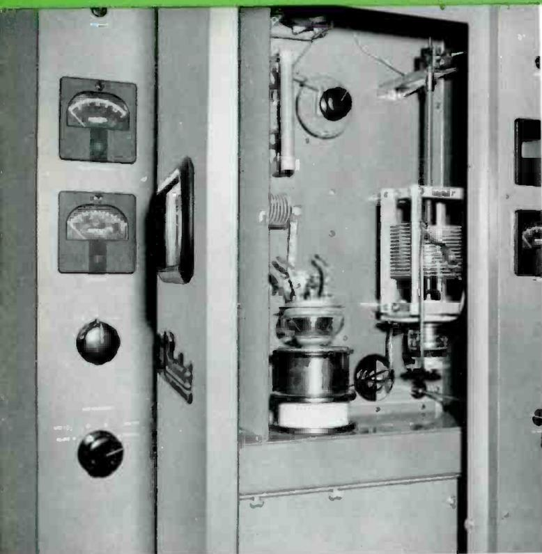
BTA-5T PA stage comprising one 5762 tube used for the high efficiency operation. The coil shown on the right, is the third harmonic coil used in the plate circuit of the PA to increase efficiency by shaping the plate waveform.
