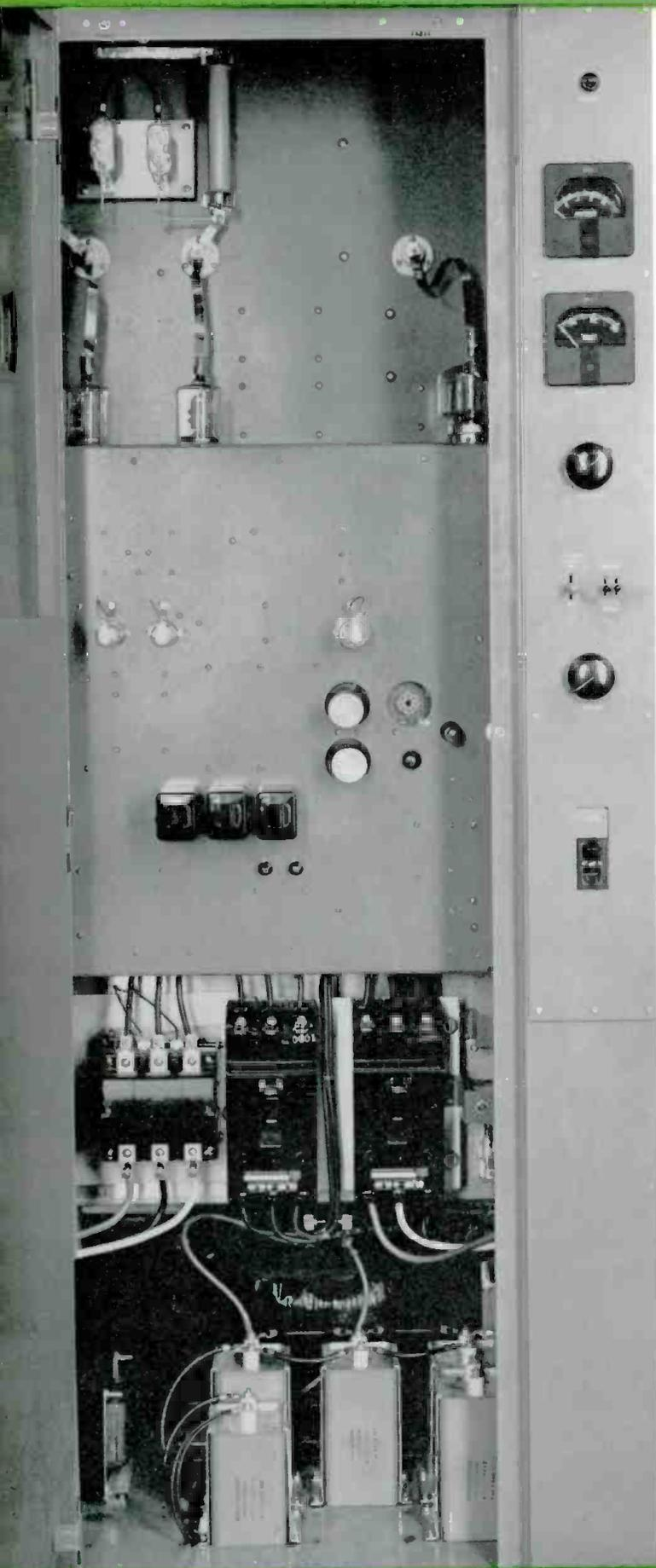
BT-10U driver including exciter and control panel. Provisions on central panel for third Crystal Oscillator for Conelrad operation is shown.
