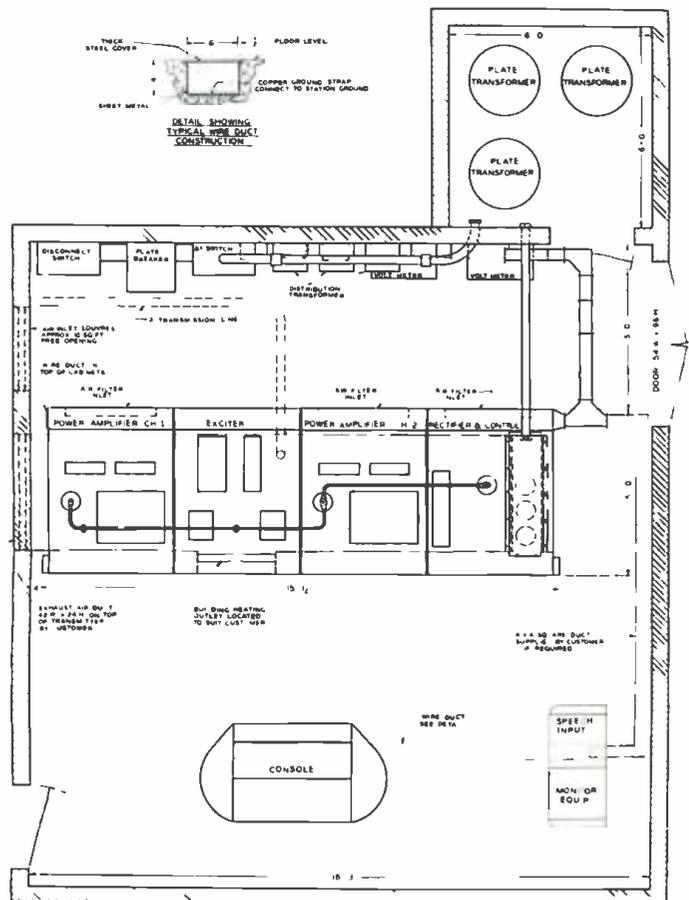
transmitter buildings. The mounting of these components, however, is not critical as to location. They can be mounted in existing power distribution areas if desired. These components include the main plate circuit breaker, a delta-wye switch, a distribution circuit breaker, a 460 to
