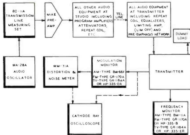
Test set-up for transmitter aural measurements.
