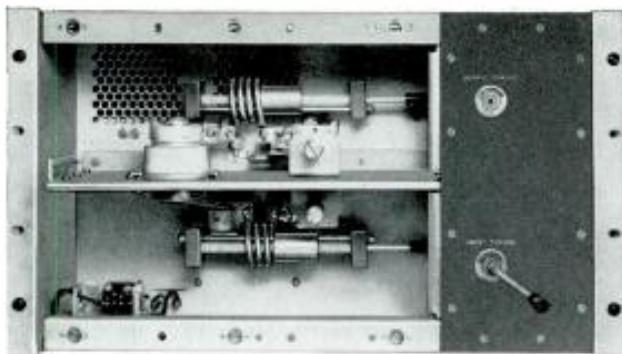
BTF-5D 250-Watt IPA with front panel removed.
