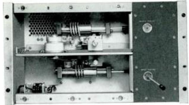
400-Watt IPA stage used to drive the dual 10-kw PA stages of the BTF-20D.
