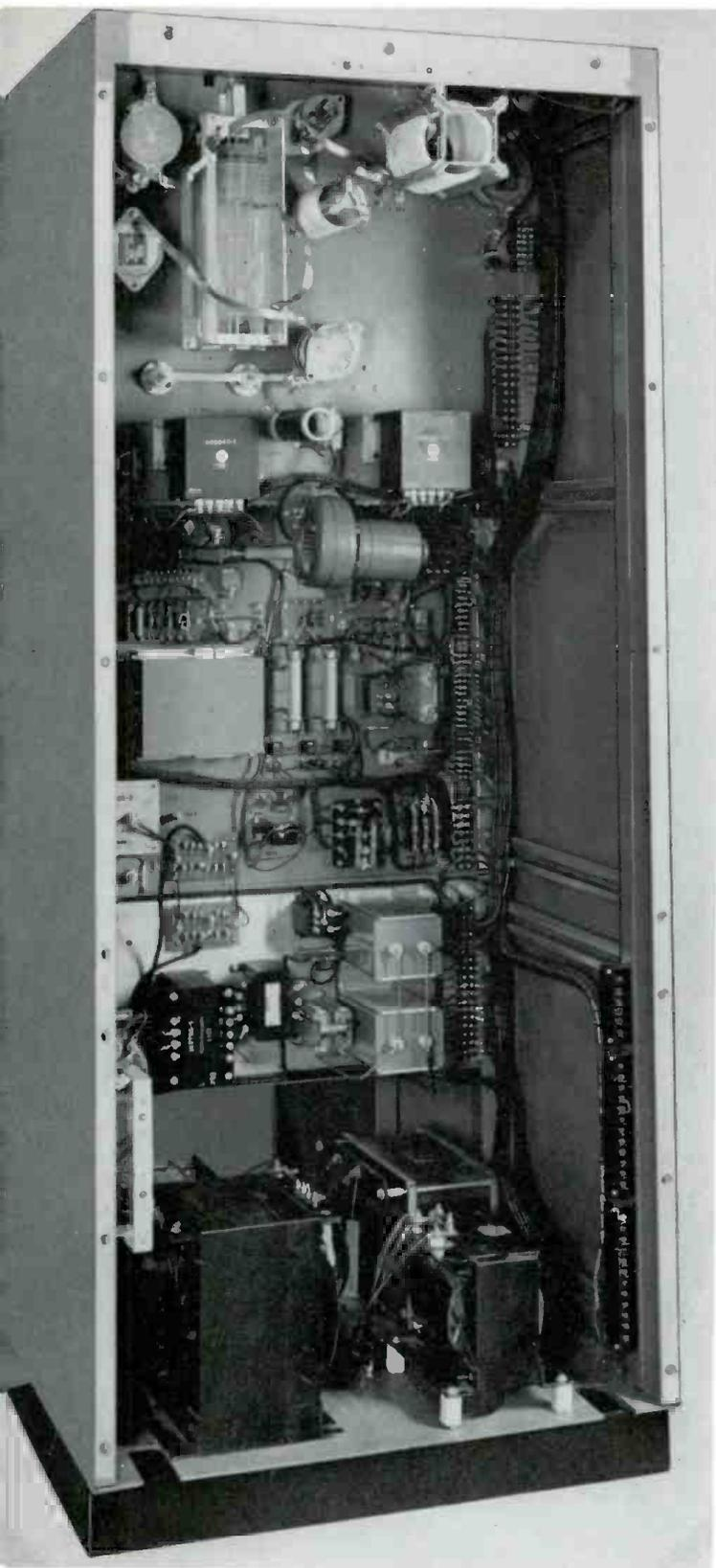
Rear view of BTA-1R, with rear panels removed, showing vertical construction and accessibility of component parts.
