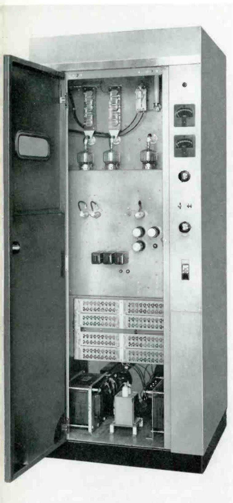
BTA-1R1 Transmitter with front door open showing accessibility of tubes and components. Power Amplifier and Modulator tubes are shown on top chassis; below is exciter chassis. All normal operating controls are shown on two side panels.
