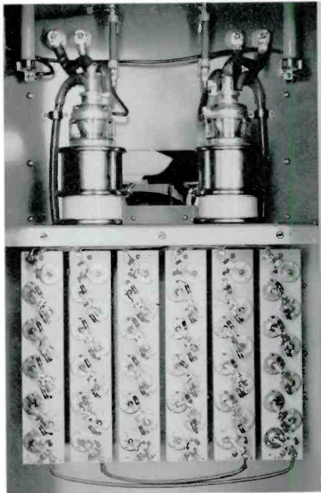
a step-start and damping circuit. This at one time was only available in the higher-power transmitters, but now longer life and added reliability are provided in the BTA-5U/10U with the incorporation of this circuit for the suppression of starting transients. The damping circuit and the primary line reactors afford continuous protection against possible operational transients.
