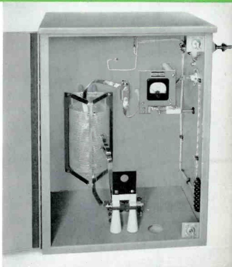
Basic 1 KW Antenna Tuning Unit, MI-27767-A.
