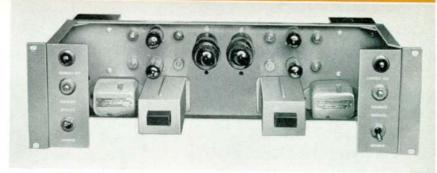
The remote power indicator also operates from the output reflectometer circuits. Two cathode follower circuits are used. One provides a voltage reference level, and the other provides a low voltage which varies with the input signal (reflectometer output). The voltage appearing at the output terminals is therefore proportional to the reflectometer voltage and has good linearity due to the cancellation of Edison effect in the tubes.
