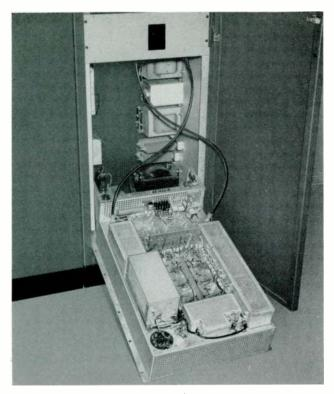
Aural and visual exciter circuits of the TTL-100AL/AH are mounted on a single hinged chassis allowing access to transformers, filters and other components housed in bottom of transmitter cabinet.
