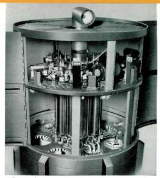
Close up showing the cluster of seven air-cooled 5762 triodes used in the 25 kw amplifier section.
