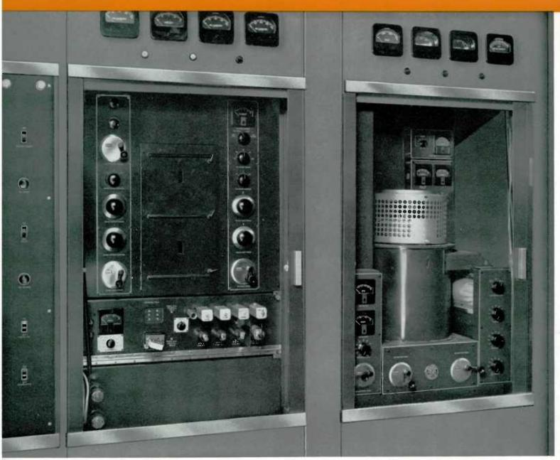
Visual transmitter section of the 10 kw driver used for the low power section of the TT-50AH transmitter. Photo shows visual driver chain and r-f amplifier cabinets.
