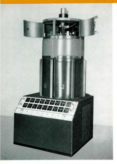
External view of the high band amplifier for channels 7 to 13.
