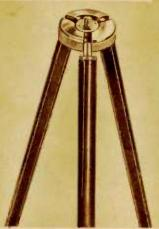
Designed especially for portable use, these all-metal tripods are extremely compact and very use, these all-metal tripods are extremely compact and very sturdy. Head is constructed to precision standards and finished in bright chrome, Upper leg sections are black enameled, lower sections polished brass. Each section is fitted with retractable pins to lock sections. Tripod
