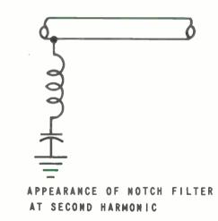
AT FREQUENCIES BELOW RESONANCE THE "STUB" APPEARS AS AN INDUCTANCE.
