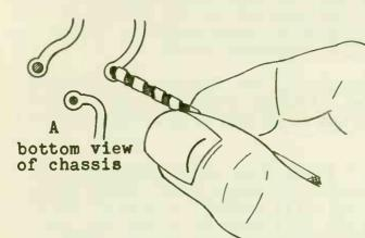
Use a small metal twist drill (1/8" dia. or less) to clear the <u>hole only</u> in the fillet of solder. Twirl the drill by hand. Do not attempt to remove all of the solder in one turn, do it slowly and carefully.
