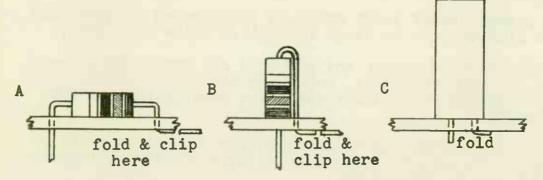
(A) & (B) Fold the leads on the new part to the same spacing as the mounting holes. Insert the part and fold the leads under the chassis to hold the part tightly against the top of the chassis. Clip off the excess wire.
