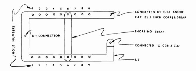
FIG 7-16 CHART-COARSE TUNING FMIG/H M 6483
