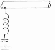
At frequencies below resonance the "Stub" appears as an inductance.
