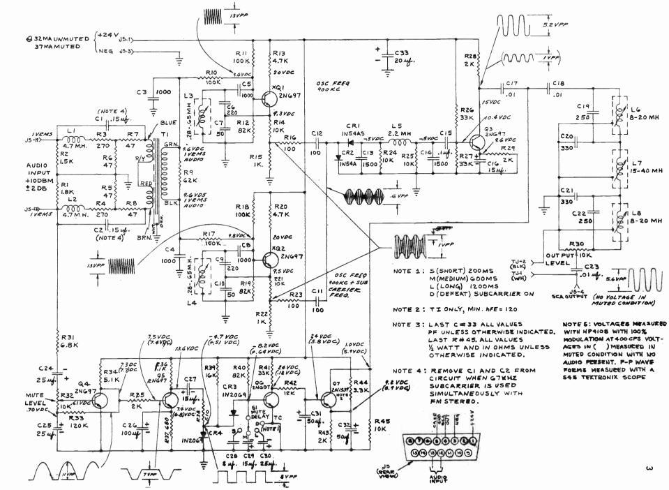
SCHEMATIC SCA GENERATOR M6507 FOR M6424 SOLID STATESMAN FM EXCITER
