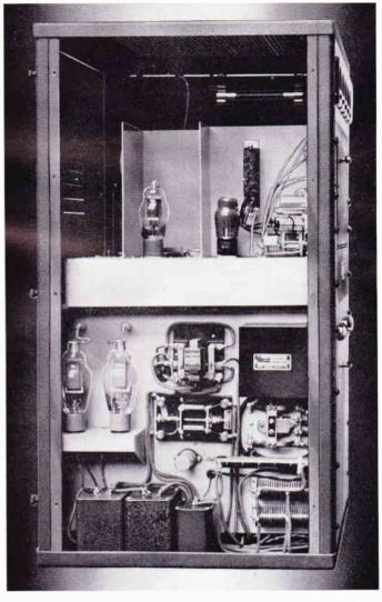
VIEW OF MO-2535 TRANSMITTER SHOWING RELAY PANEL. MODULATOR TUBES, AND OSCILLATOR DOUBLER SECTION
