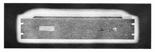
Smaller supplies are often times desirable for rack or open bench operation. This compact unit on a  $3\frac{1}{2}$ " by 19" panel provides 6.3 volts at 3 amperes and 250 to 300 volts at 50 Ma. D. C. is pure and may be used for all applications that would be required of batteries. Banks of these may be installed on racks to operate large setups of multiple units.
