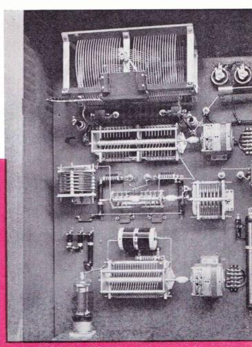
The RF circuit is shown in this illustration. It's easy to see that any component can be examined or removed without disturbing any other one.
