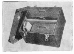
Remote Compact and Power Supply in carrying case. Note additional room available for microphone.
