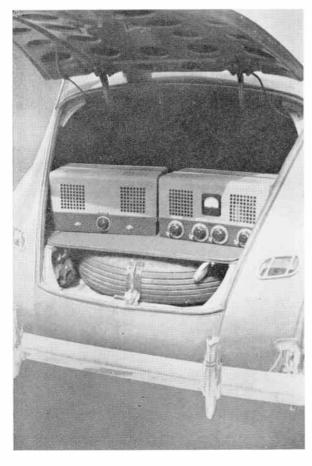
In the rear of a Standard Sedan Automobile the Gates Porto-Transmitter fits perfectly, requiring only battery and antenna connections to complete the set up.
