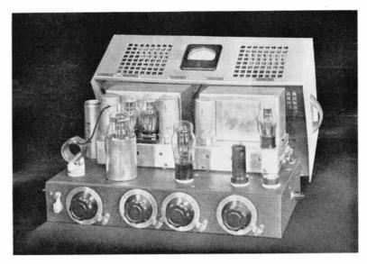
Above, Inside view of R. F. and Power Section of Gates Porto-Transmitter. Note Dual Power Pack for 6 or 110 Volt Operation.
