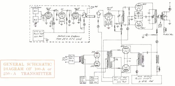
Tuning in the antenna circuit for exact power output is derived through a tuning link or variable link between the tank coil and antenna coil. This method assures the best possible transfer of radio frequency energy without affecting the tuning in any other part of the circuit, harmonic content or balance in the push pull stage.
