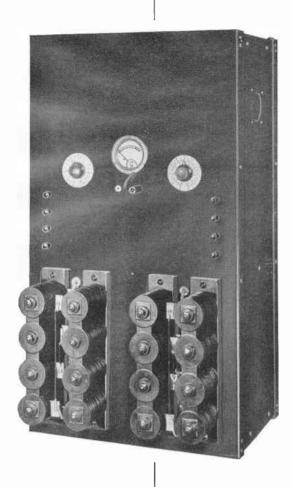
Above is shown a typical selenium type DC rectifier. The unit illustrated is two complete 15 volt 10 ampere rectifiers with complete filter for lower than .25% ripple content. These may be parralled to obtain 20 amperes or series to obtain 30 volts. Voltage may be lowered to as low as 8 volts by means of rheostats provided. Other voltages and amperages available in this unit.
