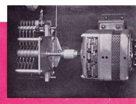
This is a close-up of the motor used to tune the final grid circuit. Considerably more power is available than is necessary to assure smooth operation at all times.
