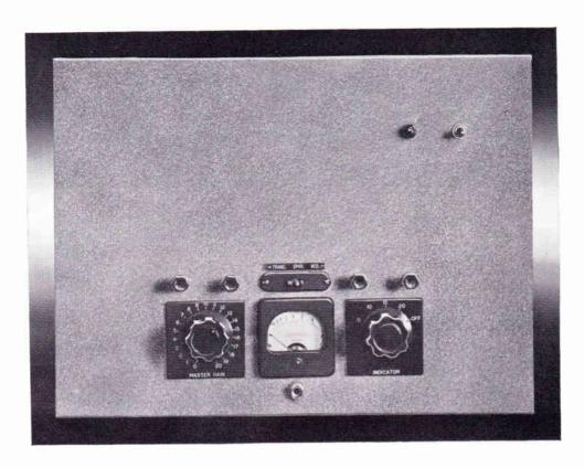
In the new and improved model 106-C amplifier will be found many features reflecting the modern and up-to-date broadcasting instrument requirements. It is complete and self contained, has no separate power supply, yet the noise level is guaranteed to be as low or lower than any similar equipment on the market today. Likewise it uses no voltage doubler type power supply but a full design full wave transformer type equipment not requiring isolation transformer or extreme care in grounding.
