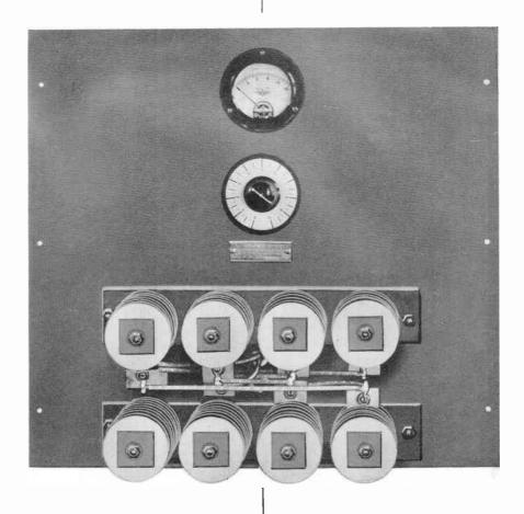
The rectifier shown above is another typical selenium type rectifier for all purposes. The unit shown provides 12 to 15 volts at 10 amperes. Is completely filtered for equal to battery operation. Rheostat and meter provide means and indication for varied voltages. This unit may be had with less filter for applications requiring only a medium or rough grade of direct current.
