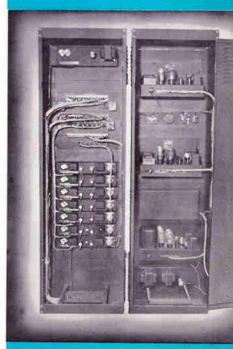
Each unit in the 5C is individually tested and then installed in the cabinet and then the whole assembly is tested for overall performance. All you have to do is connect the AC and the console.
