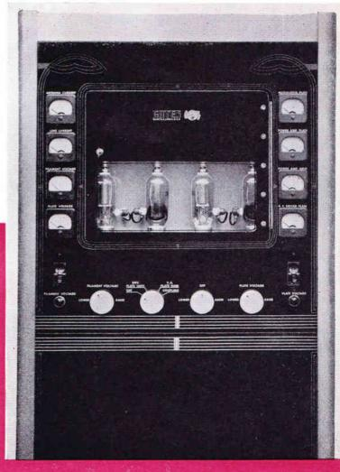
Meter arrangement for the 250-C is symmetrical and makes it easy to take the necessary readings. The plate glass door in the panel opens to allow access to the modulator and final RF amplifier tubes.
