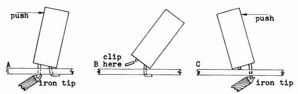
(A) hold iron tip on one of the folded leads, as soon as the solder melts - push gently but firmly on the side that will lift this lead. The capacitor should be pushed over just far enough to clear the lead from the hole.
