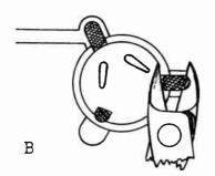
Using a pair of small sharp diagonal cutters, bend the mounting ears up and away from the copper conductor pads. DO NOT PRY THE MOUNTING EARS UP WITH A KNIFE OR SCREWDRIVER!
