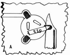
Place the iron tip on top of the folded over mounting ear. As the solder melts, slip a thin knife between the mounting ear and the copper conductor pad. DO NOT PRY THE TAB UP WITH THE KNIFE! See (4-B) for bending ears away from chassis. When the knife is completely under the ear, remove iron and let the solder cool.
