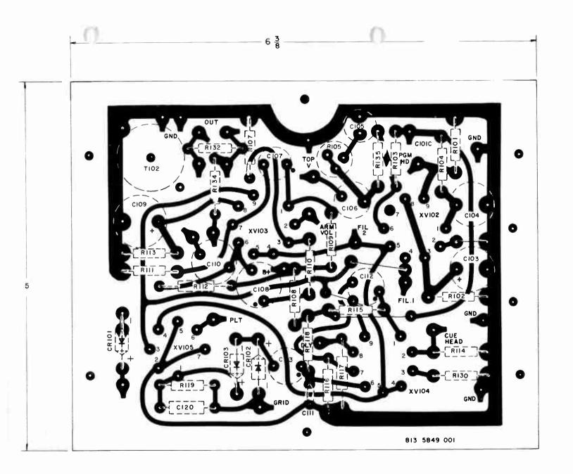
COMPONENT PLACEMENT Viewed from printed wiring side Ogram & cue Amplifier, Cartritape, M5944
