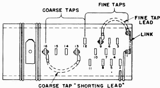
PLATE TANK INDUCTOR, 1L10 (REAR VIEW)
