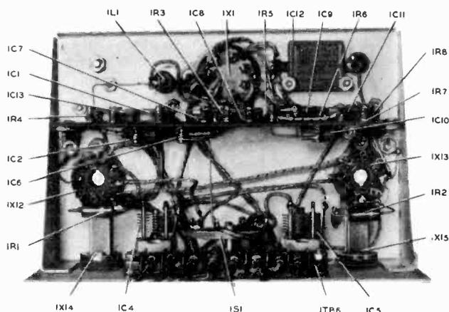
Fig. 10. Bottom View, Crystal Oscillator, Parts Identified (SY2070A)
