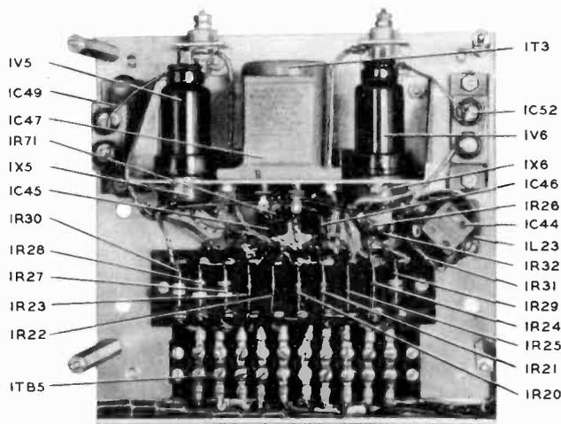
Fig. 11. Rear View, Audio Amplifier, Parts Identified (SY2381A)
