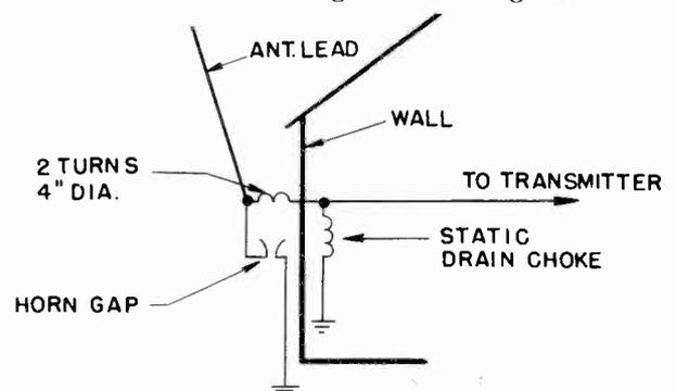
Fig. 3. Suggested Circuit for Lightning Protection
