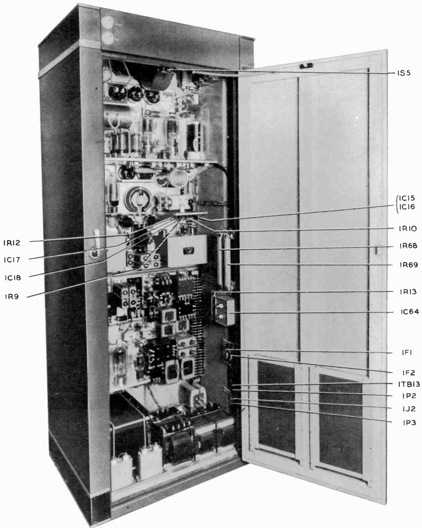
Fig. 8. Rear View, Parts on Left Side Identified (SY2382A)
