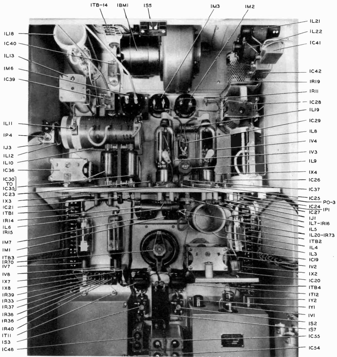
Fig. 12. Rear View, Upper Panel, Parts Identified (SY2380A)
