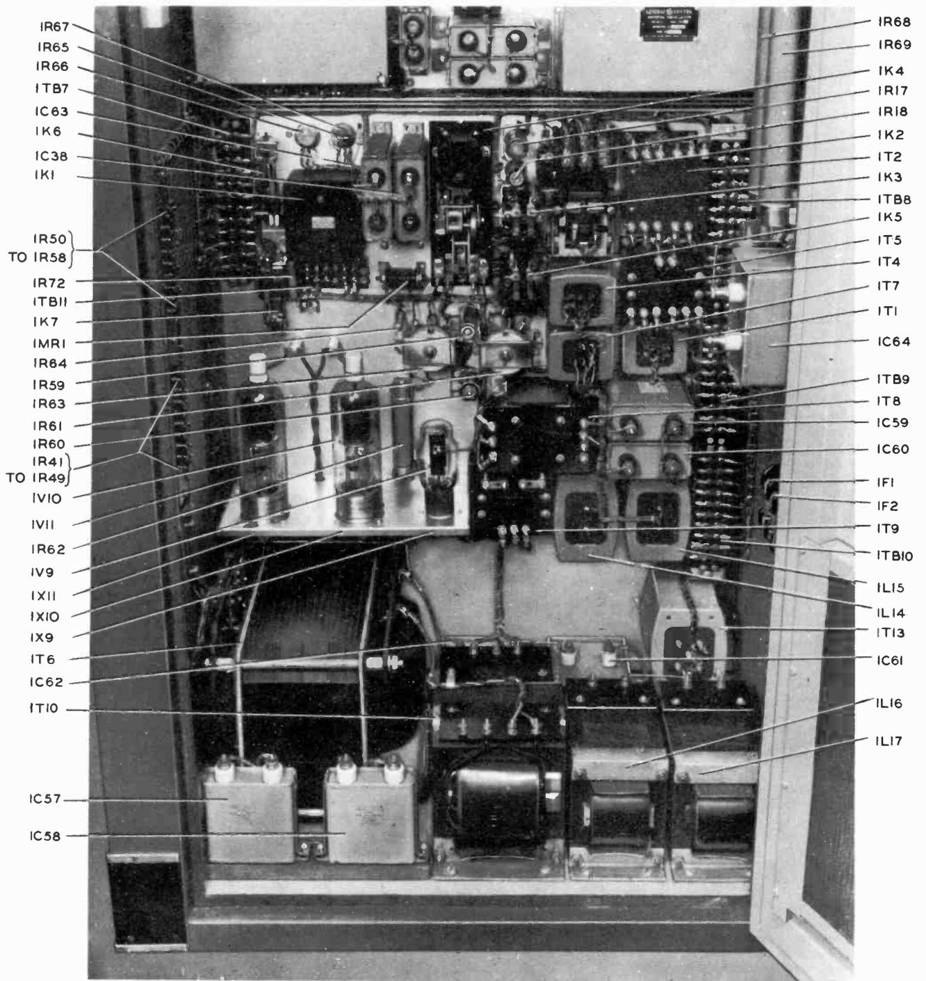
Fig. 13 Rear View, Lower Panel, Parts Identified (SY2377A)
