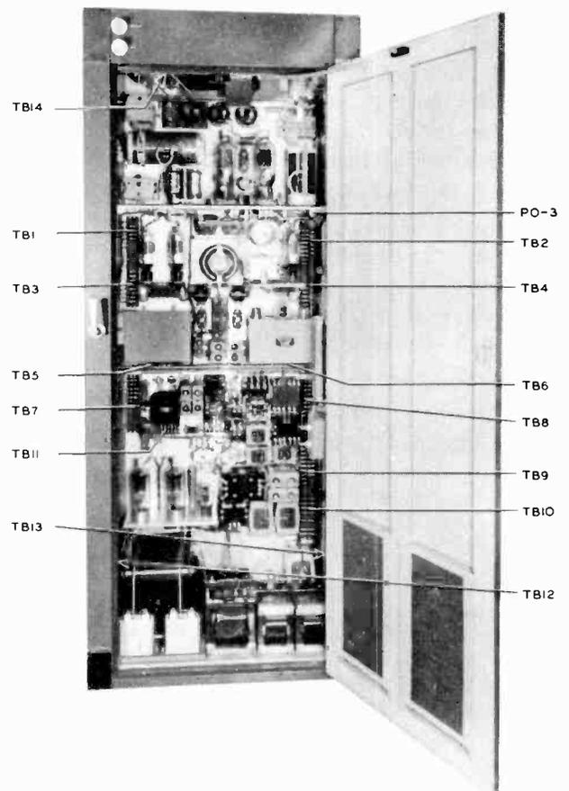
Fig. 6. Rear View, Parts Identified (SY2379B)
