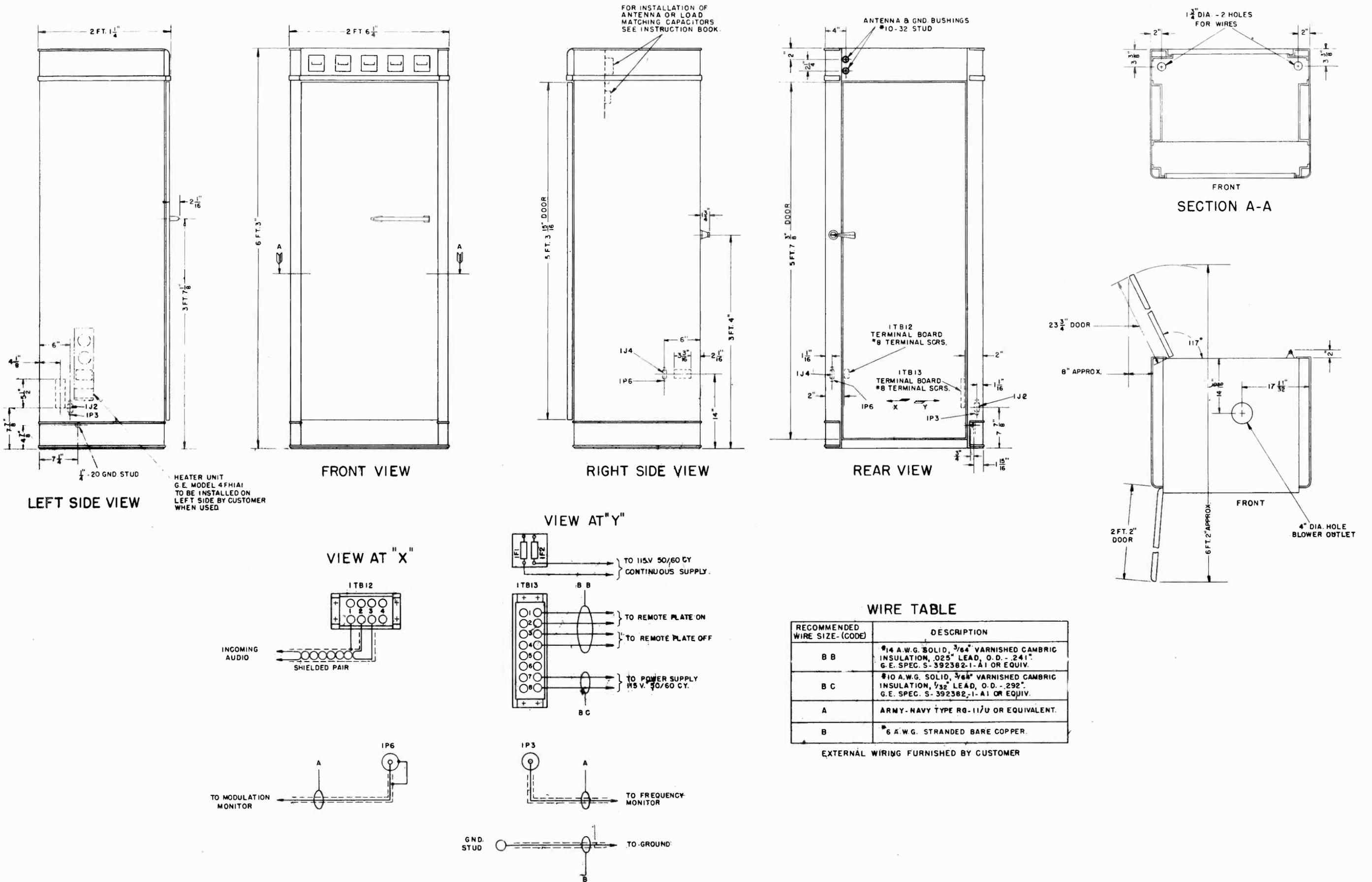
Fig. 14. Installation Requirements Drawing (T-7665065, Rev. 1)
