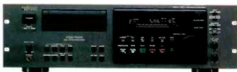
This machine is a full-function professional DAT machine. **Features:** high-reliability transport with 4 direct drive motors; jog/shuttle dial for easy operation; high S/N ratio with Super Bit Mapping recording function; 8-pin parallel remote control port; wireless remote control; independent L/R recording level controls; balanced XLR and unbalanced RCA analog I/O; AES/EBU and coaxial digital I/O.
