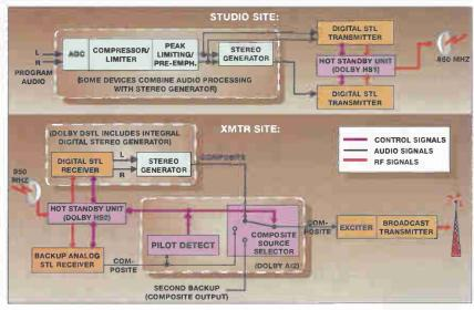
Figure 1. Hot-standby installations using digital STLs with analog backup must cope with discrete and composite audio signals. For fully automatic operation, the receiver must also sense whether the digital or analog system is using the STL channel. A pilot-detect circuit accomplishes the latter.
