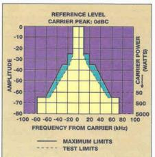
Figure 1. The NRSC-2 emission standard's RF mask. Note differences in last step for different stations' licensed power levels.
