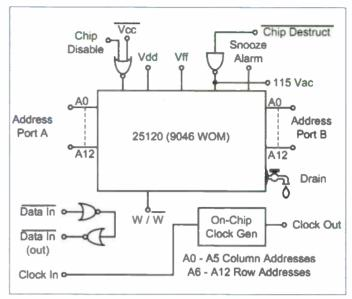
Pin out for the Signetics "Write Only Memory" released in 1972. While the 25120 is no longer available, the author can, upon request, supply a schematic using discrete components that duplicates the WOM function.
