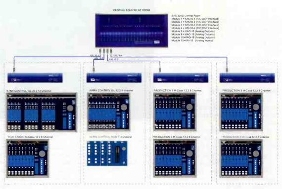
SAS system design for the KTNN facility, showing locations of i-SL, Rubi-T and M-Class control surfaces.
