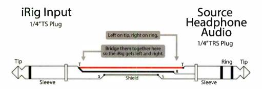
Simple wiring diagram for the iRig 2 specific cable. Left and Right are simply multed together on the Tip/sleeve connector.
