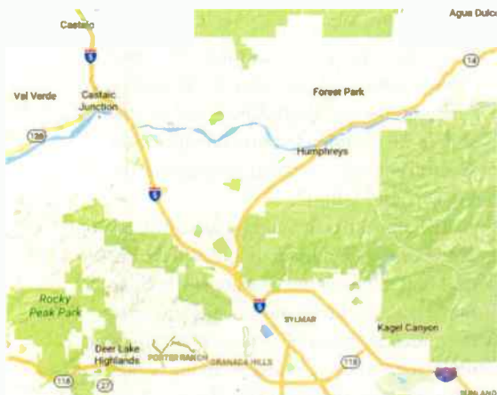
Fig. 4: Santa Clarita is located in the “V” formed by highways 5 and 14. Highway 5 between the 14 intersection, and that of highway 118, is a primary design consideration since any radio can hear both the booster and the main from Mt. Harvard. Interference was mitigated in this area.
