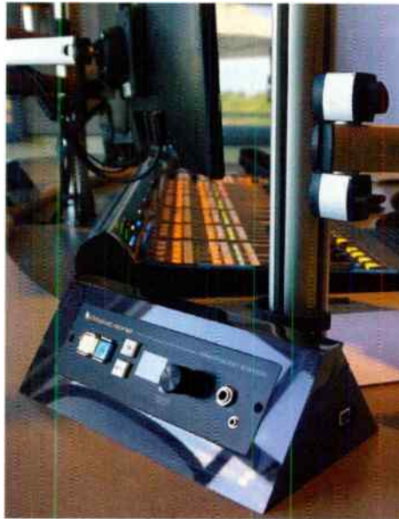
USB ports on studio talent stations wire directly back to Wheatstone M4-IP mic processors.
