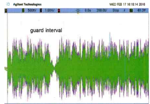
An example of guard interval, shown in time domain. (200 \mu s/div along X axis.)
