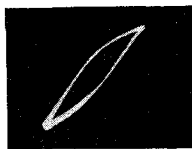
Fig. 146, left, Fig. 147, right. The amount of saturation in these two oscillograms is appreciably less than that shown in Figs. 142 to 145. The core loss due to hysteresis, indicated by the size of the area enclosed by the curve, is fairly large in Fig. 147.
