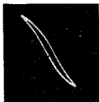
Fig. 146, left, Fig. 147, right. The amount of saturation in these two oscillograms is appreciably less than that shown in Figs. 142 to 145. The core loss due to hysteresis, indicated by the size of the area enclosed by the curve, is fairly large in Fig. 147.
