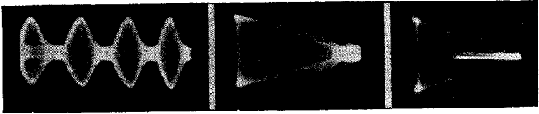
Fig. 413 (left) indicates the modulated wave during excessive regeneration and Fig. 414 (middle) shows the equivalent trapezoidal pattern. Fig. 414-A (right) is another trapezoidal pattern indicating improper neutralization adjustment.
