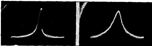
Fig. 302, left, 303, right. The lack of symmetry in the resonance curve in Fig. 302 is due to regeneration. See Fig. 303 for the corrected curve.
