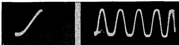
Figs. 183, left, 184, right. When the input voltage to the amplifier was increased, the input-output signal curve ends flattened a trifle, as shown in Fig. 183. Note the departure from a true sine wave in the output waveform in Fig. 184.
