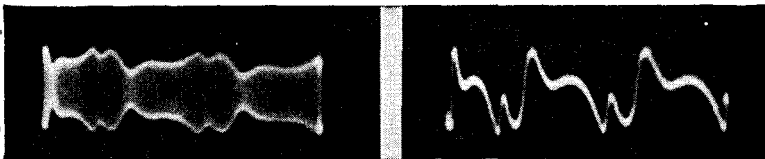
Fig. 236-A, left, Fig. 236-B, right. The same oscillator adjusted to 1000 kc. has a modulated waveform as shown in Fig. 236-A. The a-f. output resulting from the demodulation of A is shown in B.
