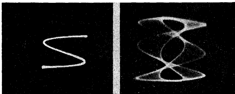
Fig. 97. G, left, H, right. The 3-1 pattern of G was made when the voltages had a phase difference of 180^\circ . In H one of the voltages was modulated.
