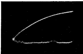
Fig. 257. An oscillogram of the sweep voltage employed in the Clough-Brengle frequency modulator. The horizontal line represents that period of the cycle when the shorting contact is closed and the rising portion of the curve is the time when the condenser is charging.
