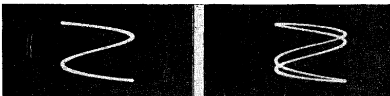
Fig. 97. A, left, B, right. A 3-1 ratio pattern is shown in both illustrations. The pattern in A was taken when the phase difference between the two voltages was 0^\circ .
