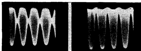
Figs. 387, left, 388, right. When the sweep voltage is incorrectly adjusted a pattern like that of Fig. 387 results. A correctly adjusted sweep voltage yielded the oscillogram of Fig. 388.
