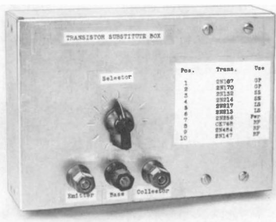
Fig. 332. The switch selects one of ten different transistors.
