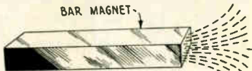
Fig. 1. Bar magnet, showing how the lines of force, or magnetic flux, create a magnetic field as indicated by dotted lines.
