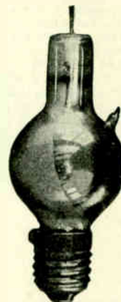
A typical rectifier tube of the Tungar type. The screw-base allows it to be inserted in a standard lamp socket from which current is obtained for the filament. Connection is made to the graphite disc by means of a Fahnestock connector which clips on to the wire post projecting from the other end of the tube.
