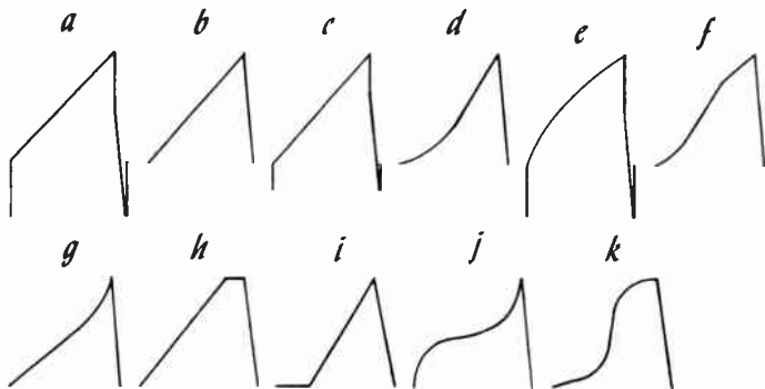
Fig. 824. Effects of poor linearity on the vertical sweep signal. Good waveforms, with and without the spike, are shown in (a) and (b).
