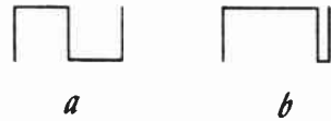
Fig. 817. Multivibrator square waves. The waveform in (b) is the output of an unsymmetrical circuit.
