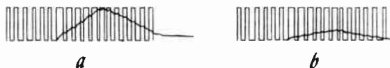
Fig. 809. Correct vertical integration (a). Poor vertical integration will produce a weak vertical sync pulse (b).
