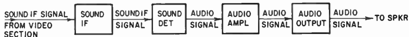
Fig 118. Block diagram of an audio section. In some sets, more than one sound if stage may be used.
