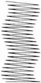
Fig. 915. Effects of hum in the horizontal oscillator and output stages. Both the raster and picture are affected.
