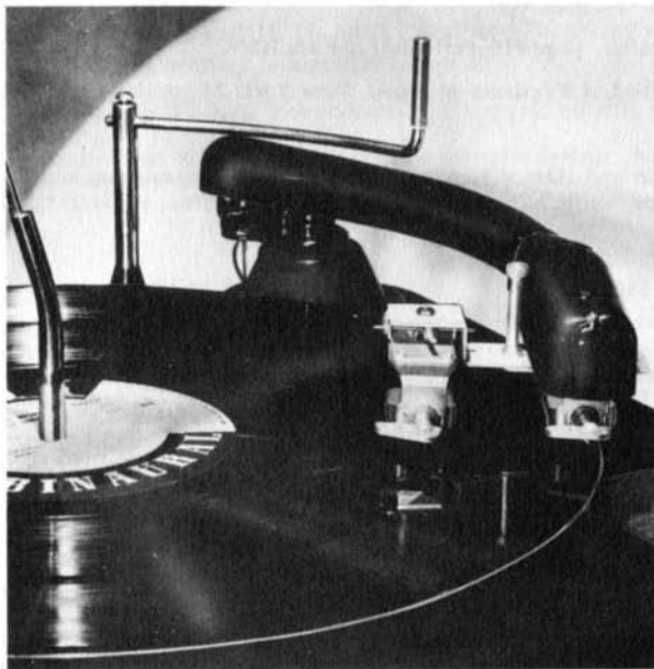
Fig. 215. Double tone arm system used a clip-on device for the second cartridge. (Cook Laboratories, Inc.)
