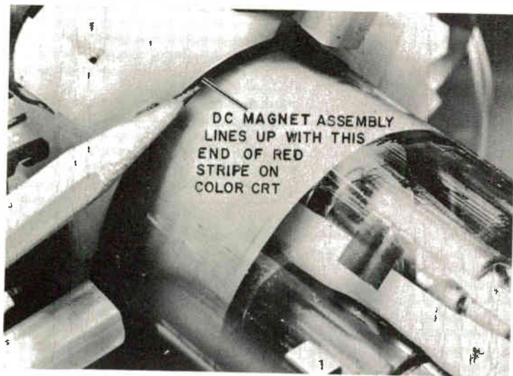
Fig. 412. Dc magnet assembly is lined up at this end of the red stripe on the color CRT.
