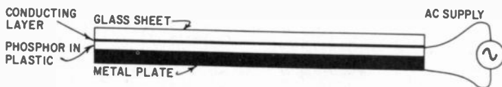
Fig. 907. Section of an electroluminescent panel, which glows under the stimulation of an alternating electric field.
