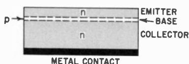
Fig. 714. The double-diffused technique enables transistors to be made with extremely thin bases.
