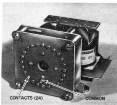
Fig. 1402. A 24-contact stepping relay is the heart of our expanded two-channel radio-control system.
