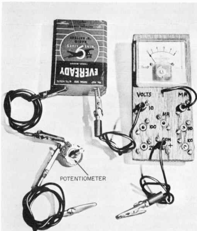
Fig. 207. The test meter can be used to measure resistance.
