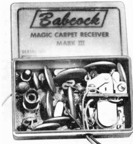
Fig. 614. The Babcock Mark III receiver.
