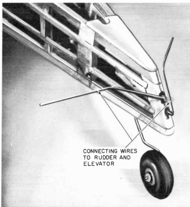
Fig. 1209. Wires connecting to rudder and elevator are brought out through the end of the fuselage.
