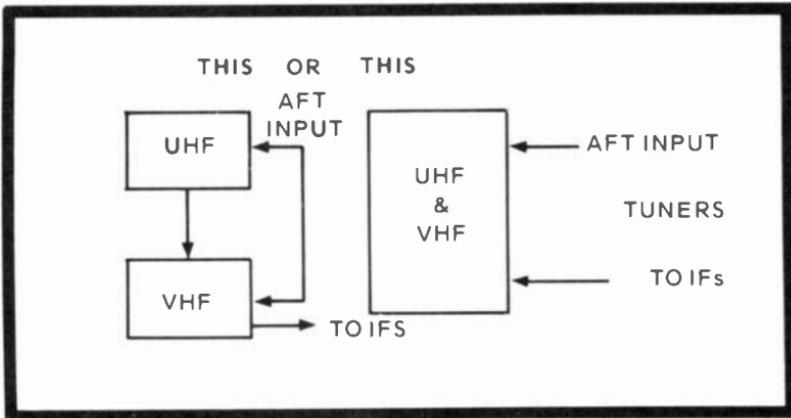
Fig. 1-13. Separate or combined UHF-VHF tuners are found in the newest television receivers. Most have AFT oscillator control from the third video IF.
