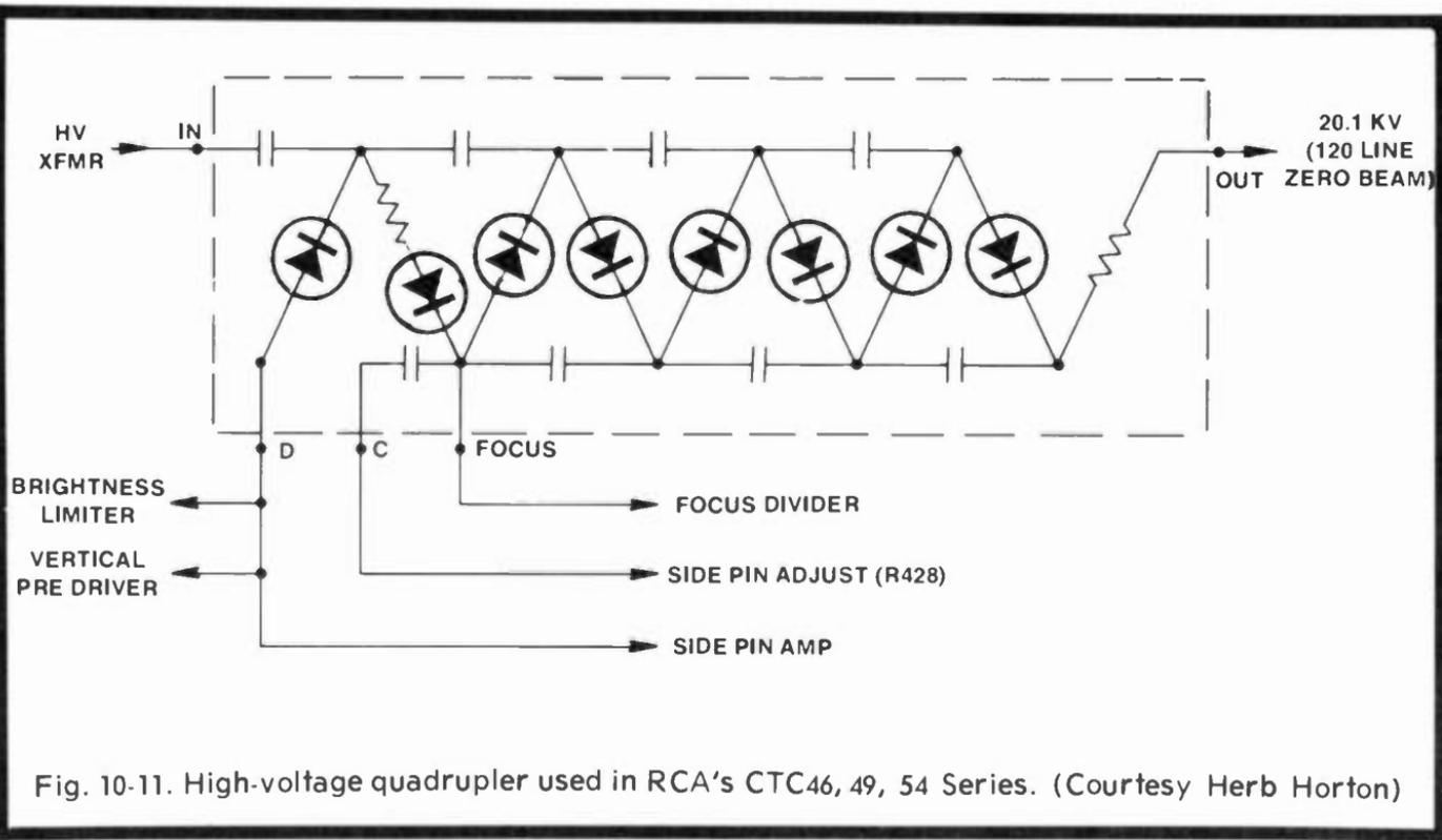
Fig. 10-11. High-voltage quadrupler used in RCA's CTC46, 49, 54 Series. (Courtesy Herb Horton)
