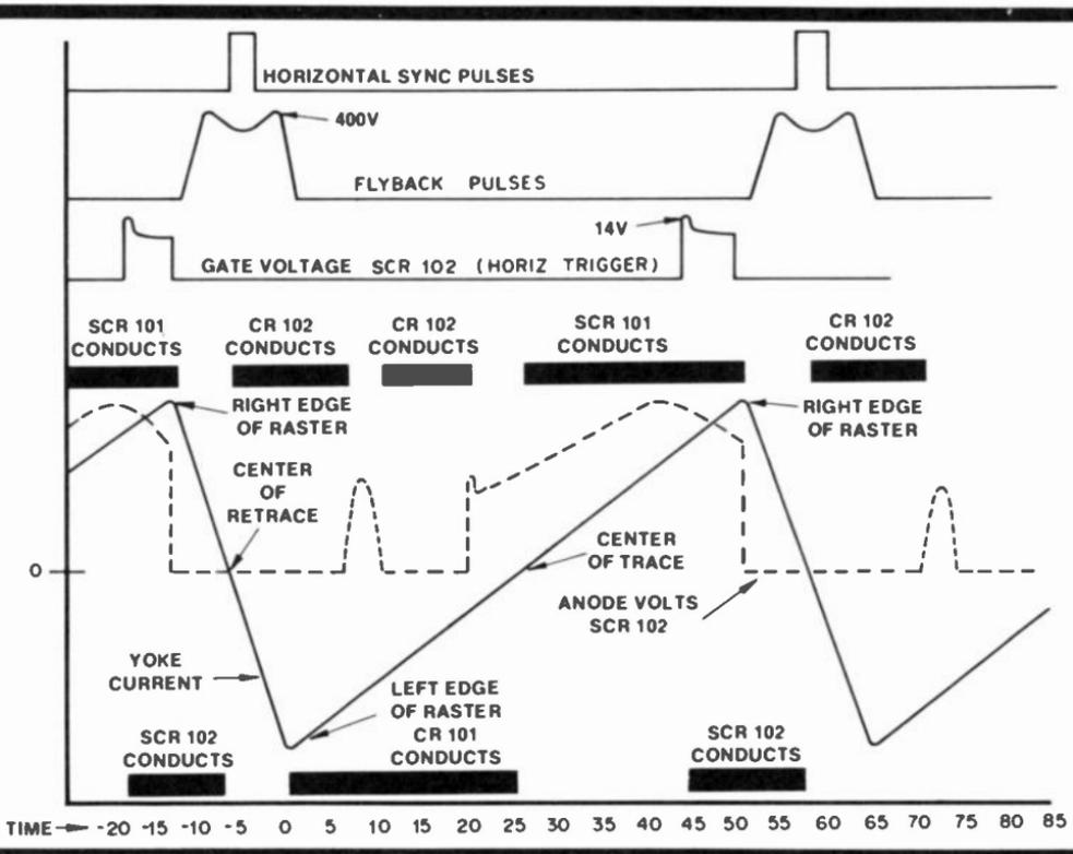
Fig. 9-10. Timing diagram of the RCA SCR horizontal deflection system.
