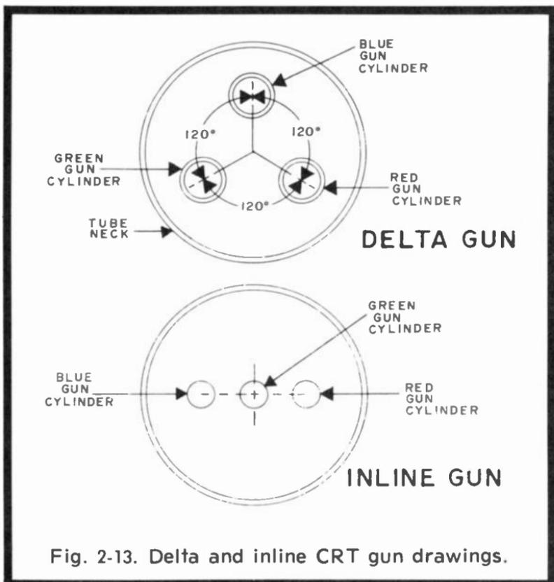
Fig. 2-13. Delta and inline CRT gun drawings.
