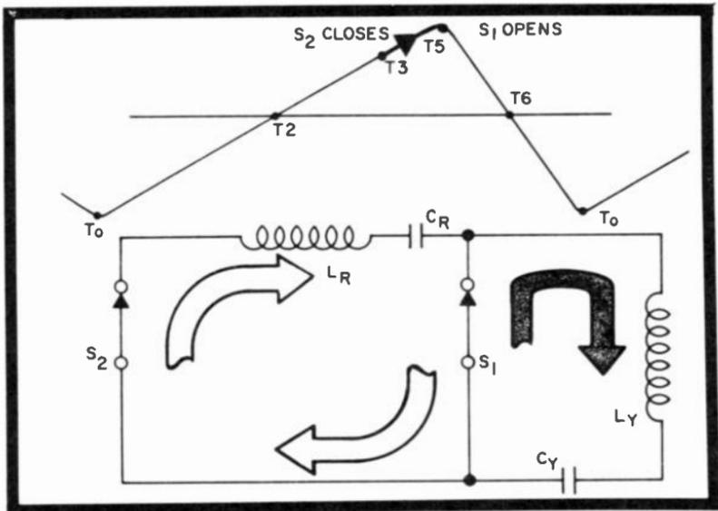
Fig. 9-18. Circuit current ( $T_2$  to  $T_5$ ) during retrace initiation.
