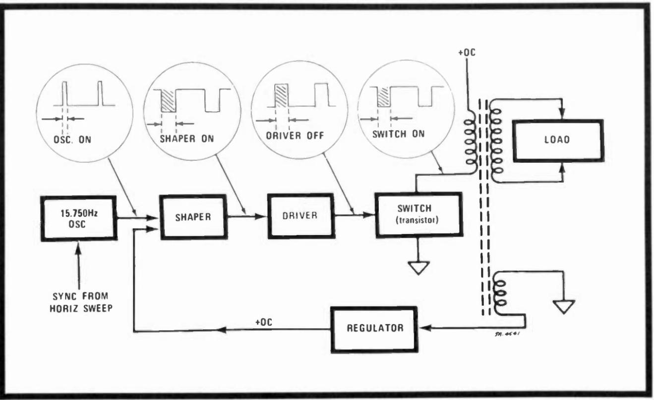
Fig. 11-9. Switched power supply operational diagram with rectangular waveforms. (Courtesy Stan King)
