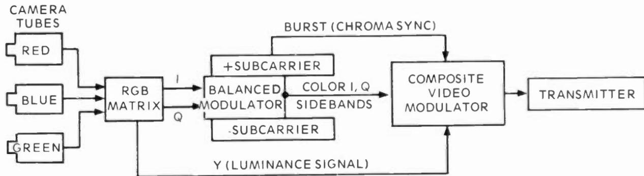
Fig. 1-10. Diagram illustrating how color signals are formed. I, Y and Q signals are combined with 90-degree out-of-phase subcarriers that are suppressed (cancelled) by balanced modulators. When there is no color, the two demodulators go to zero and only luminance is transmitted.
