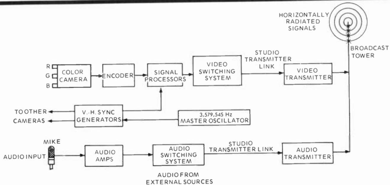
Fig. 1-11. Sync, blanking and audio are added to color (or monochrome) to complete the TV signal. Especially notice that the master oscillator for the entire system is the color subcarrier (Courtesy John Platt, NBC).
