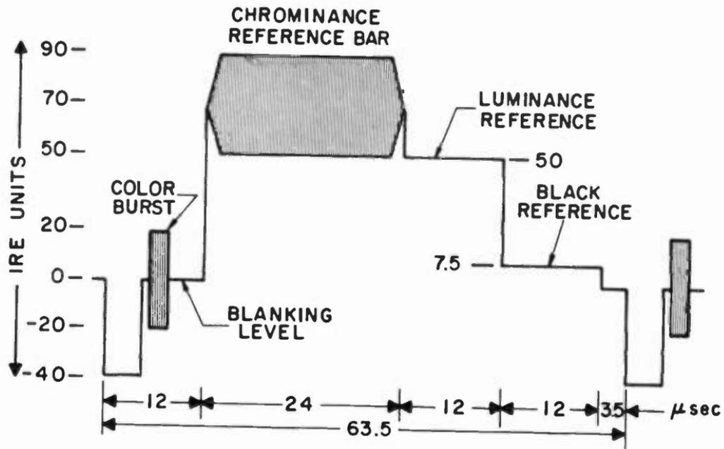
Fig. 3-12. The VIR signal scanning on line 20.
