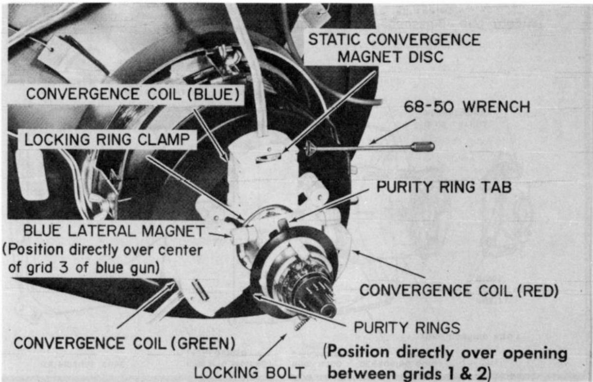
Fig. 4-2. Zenith's CRT gun and static-dynamic yoke assembly for both hybrid and solid-state receivers.
