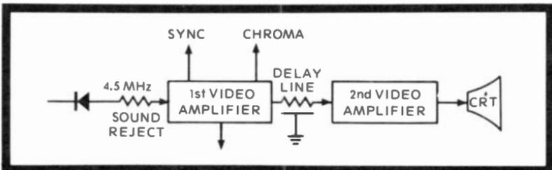
Fig. 6-1. Conventional video detector and video amplifier block diagram.
