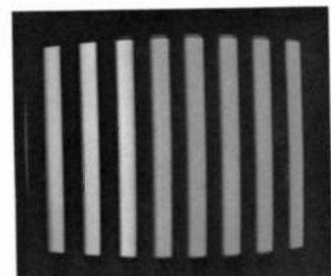
Fig. 14-62. Shorted green demodulator input.
