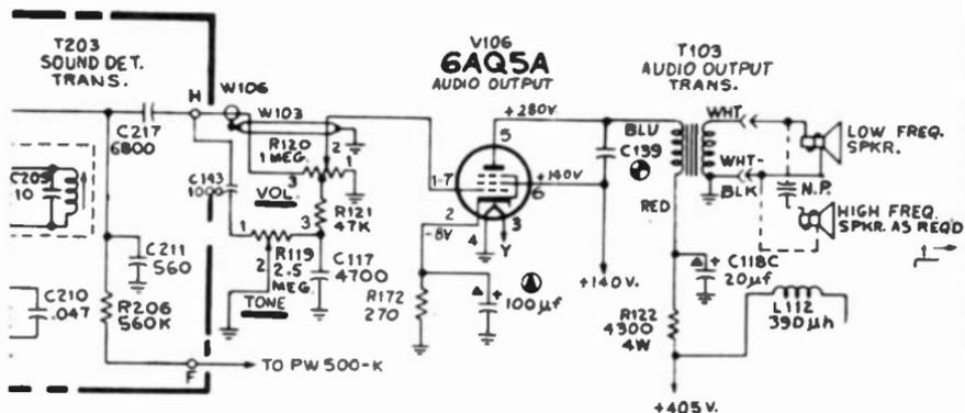
Fig. 6-16. RCA CTC25X vacuum tube sound subsystem circuits.
