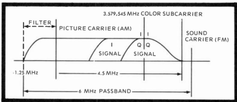
Fig. 1-3. The same monochrome characteristics in Fig. 1-2 are indicated here, but with color information now added. The drawing also shows the effect of a filter for negative vestigial sideband compression. Notice I and Q signals on either side of color subcarrier, plus the color sync subcarrier.
