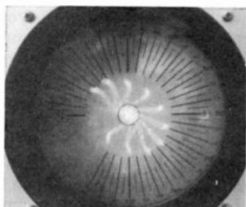
Fig. 14-50. Crosstalk can also cause bad crossovers, and this means washed-out colors.
