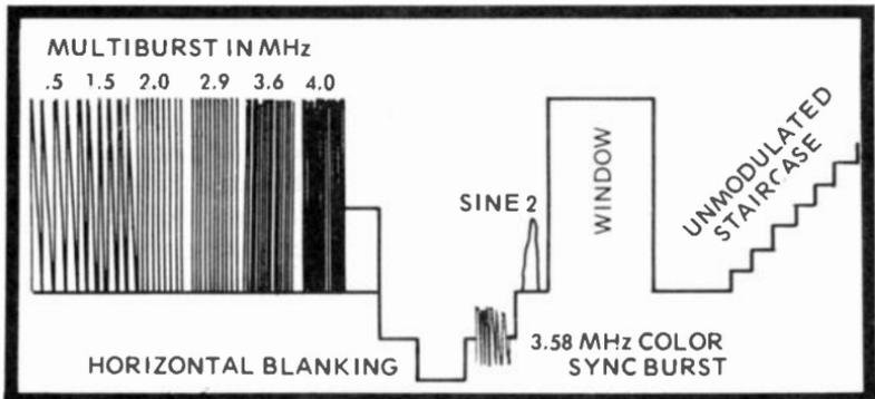
Fig. 3-8. Vertical interval test signal (VIT) transmitted between lines 17 and 20 of the vertical scan interval; another aid in checking receivers for proper operation, alignment, etc. Good resolution of this pattern takes a better than average scope—no AC recurrent sweep types. It must resolve horizontal lines cleanly at 10 microseconds per division.
