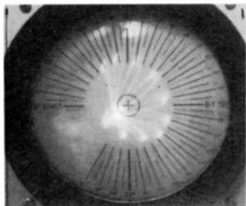
Fig. 14-30. A normal brightness setting on cathode-fed CRTs plays havoc with a vector display.
