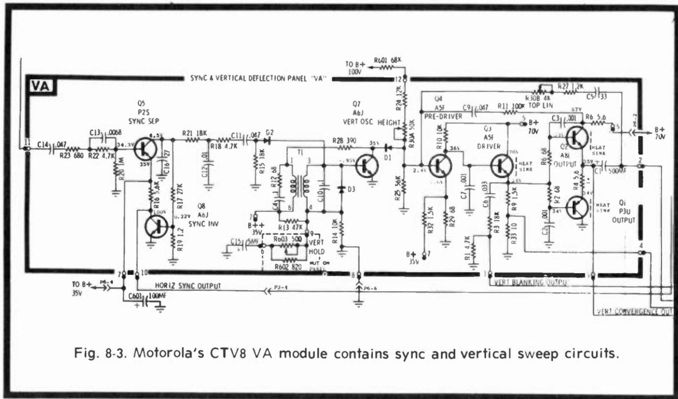
Fig. 8-3. Motorola's CTV8 VA module contains sync and vertical sweep circuits.
