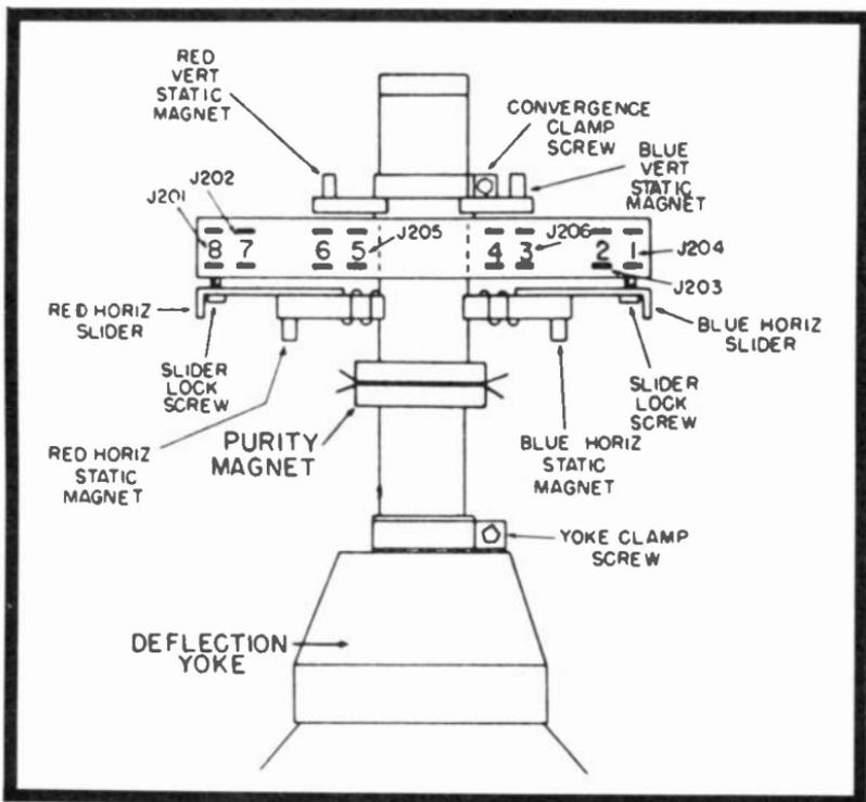
Fig. 2-14. Drawing showing the locations of the convergence magnets and slides for in-line gun tubes.
