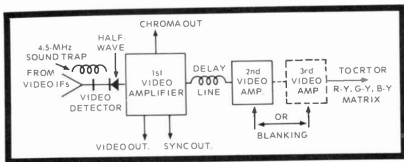
Fig. 1-15. Block diagram of a diode half-wave video detector followed by two or more video amplifiers with an 0.8-microsecond delay line in between.
