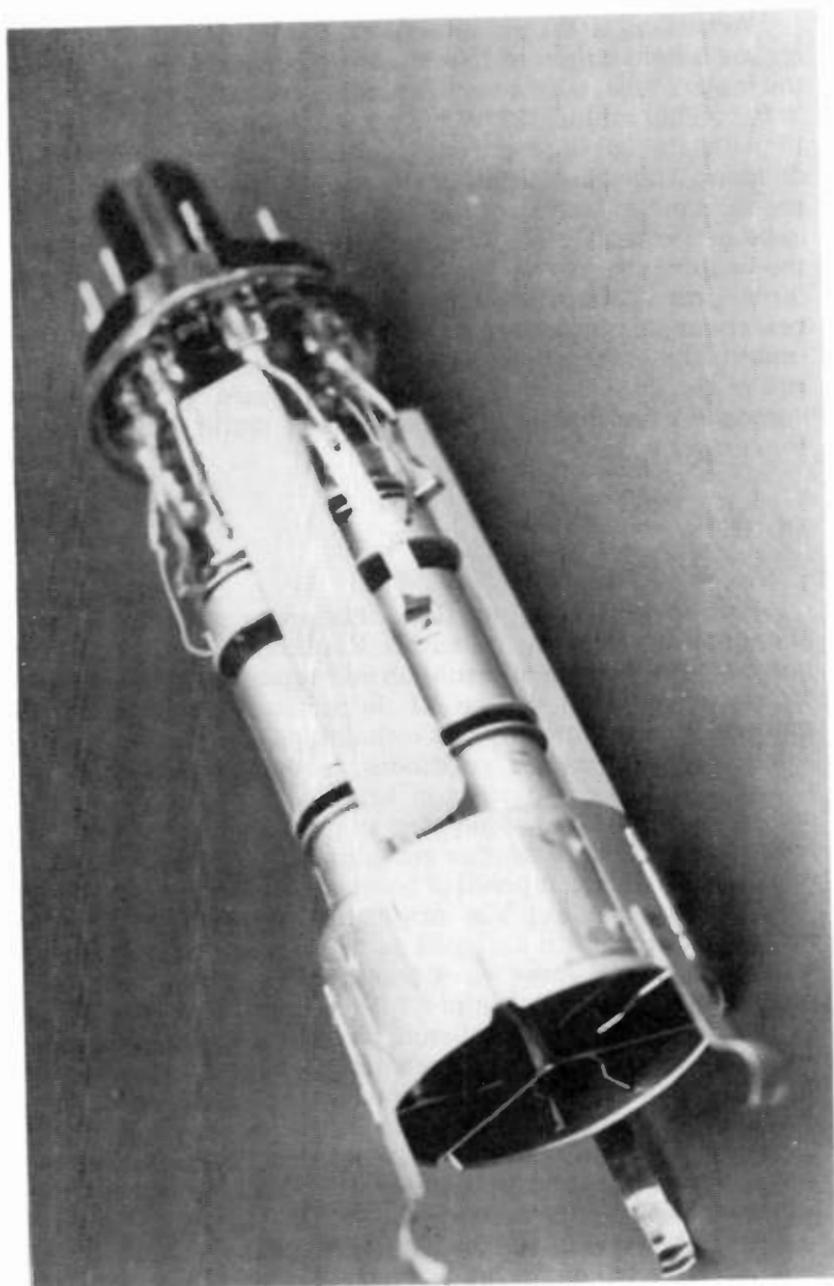
Fig. 2-15. Electron gun assembly for the Chromacolor tube showing the electrodes of the three guns.
