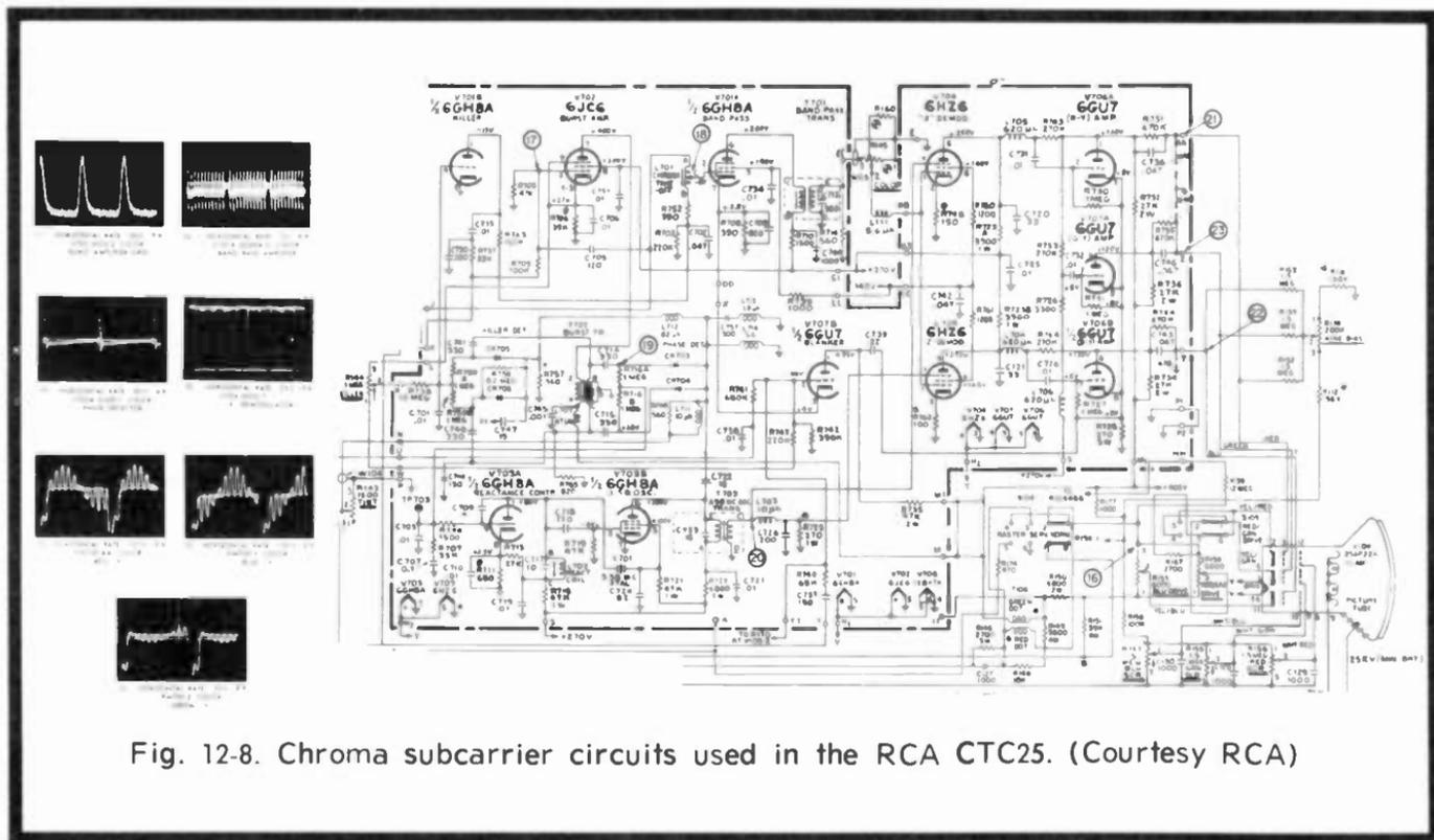
Fig. 12-8. Chroma subcarrier circuits used in the RCA CTC25. (Courtesy RCA)
