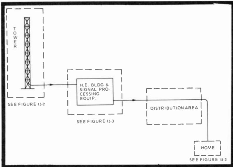
Fig. 15-1. "Standardized" type CATV system showing major blocks with details spelled out in Figs. 15-2, 15-3 and 15-4.
