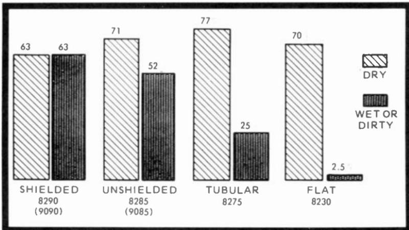
Fig. 13-1. Percentage of signal delivered to the set with clean, dry transmission line and wet, dirty cable.
