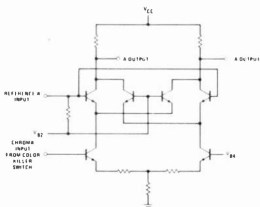
Fig. 12-29. One half of the chroma demodulator circuit.
