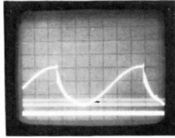
Fig. 14-11. These scope traces show the charge (faint trace) and discharge of C4008. The 1.5v trace is the residual waveform.
