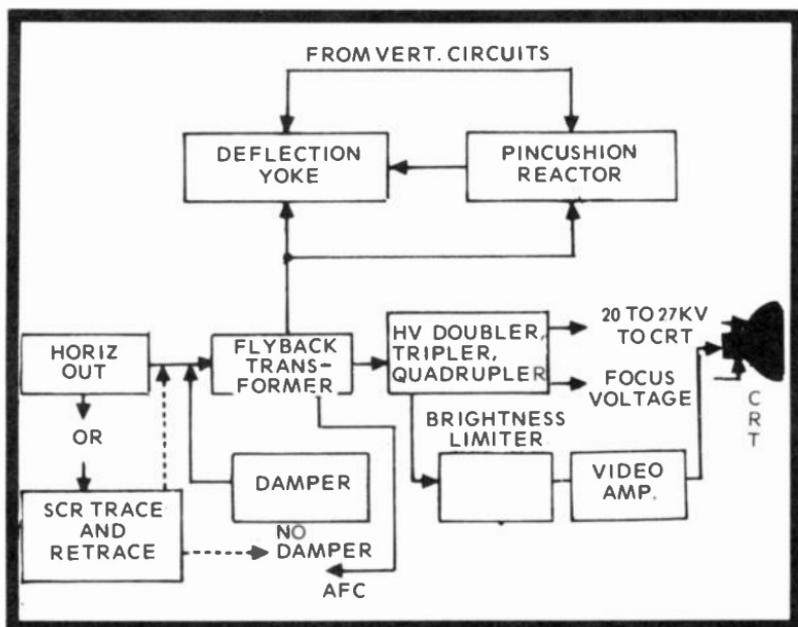
Fig. 10-9. Block diagram of a modern high-voltage sub-system.
