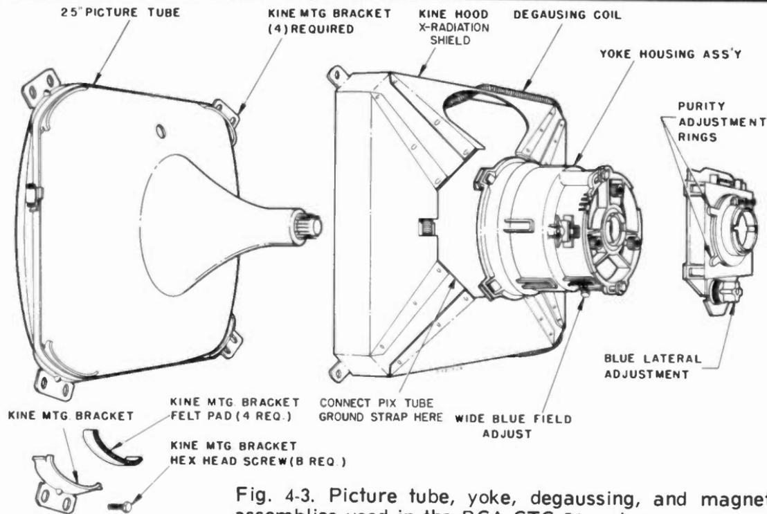
Fig. 4-3. Picture tube, yoke, degaussing, and magnet assemblies used in the RCA CTC 54 series.
