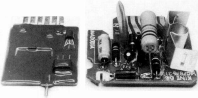
Fig. 12-21. Interior of MAD module from its beginning as a discrete, to thick film on ceramic substrate, then final encapsulation. (Courtesy RCA)
