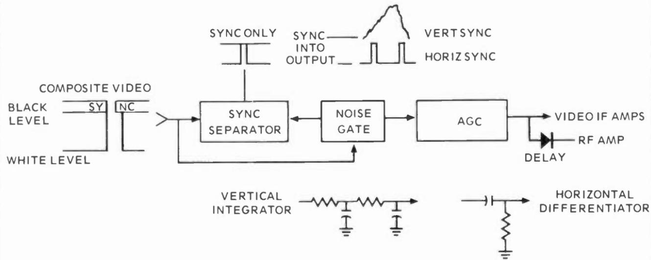
Fig. 7-1. Block diagram of a typical sync separator, noise gate and AGC system.
