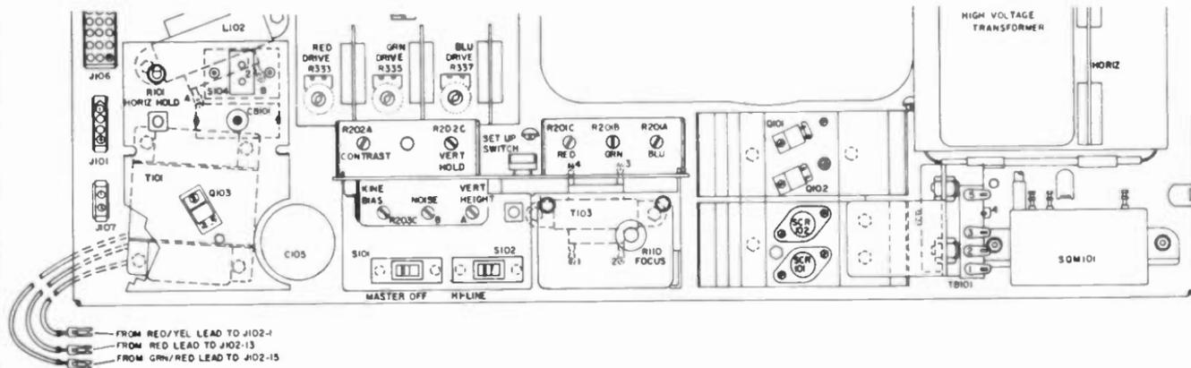
Fig. 4-7. RCA's CTC 49 rear panel setup adjustment locations.
