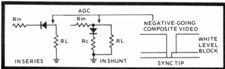
Fig. 6-2. Half-wave video detector diode in series and shunt, depending on bias, source and output impedances. Both pass only negative-going demodulated video as shown.
