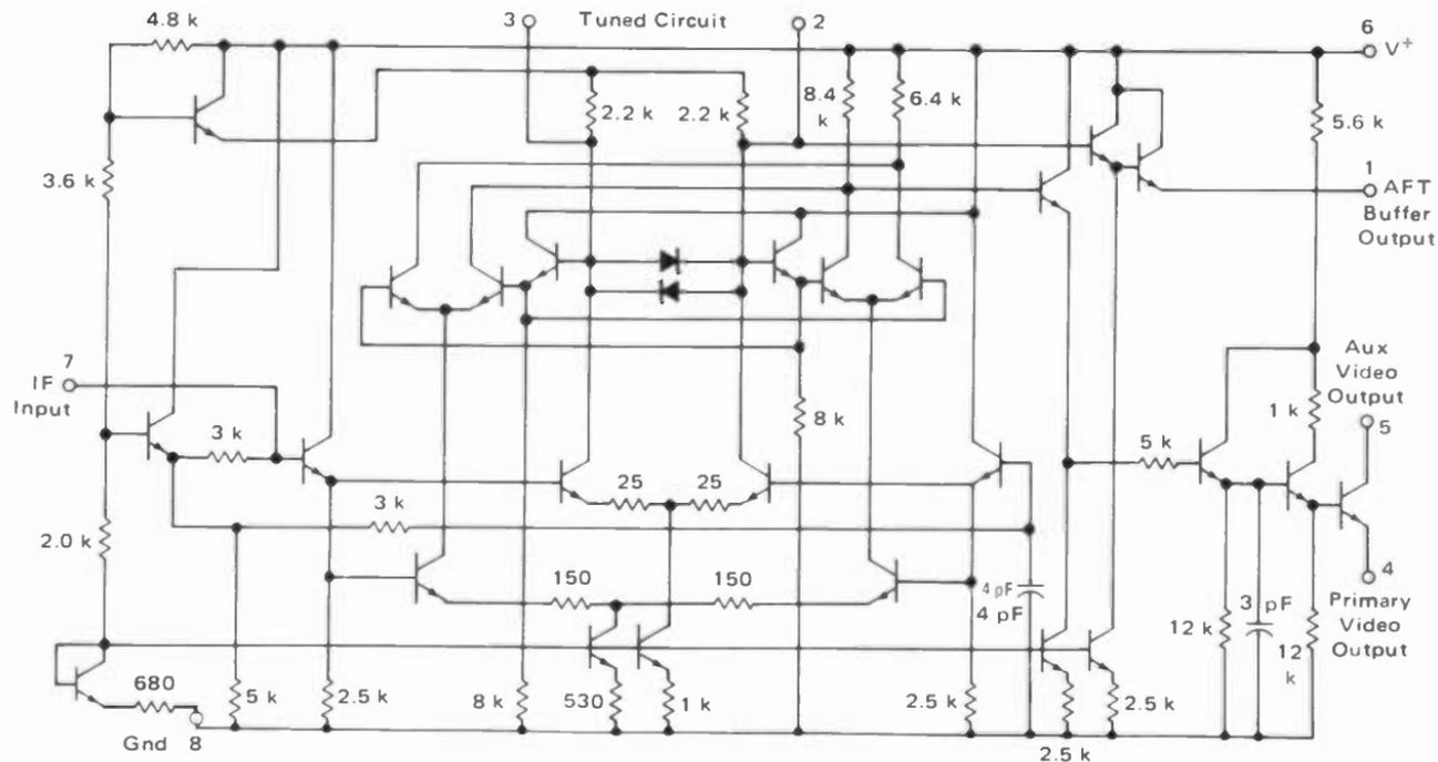
Fig. 6-9. Schematic of the MC1330P IC switching detector.
