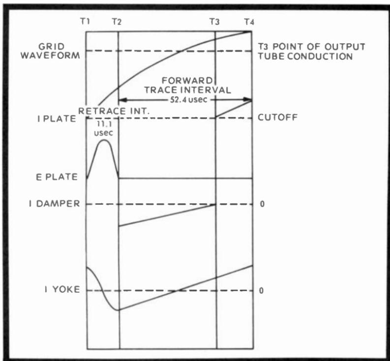
Fig. 10-3. These curves show one cycle of horizontal output beginning with retrace and ending with cutoff. (Courtesy Ray Guichard, Magnavox)
