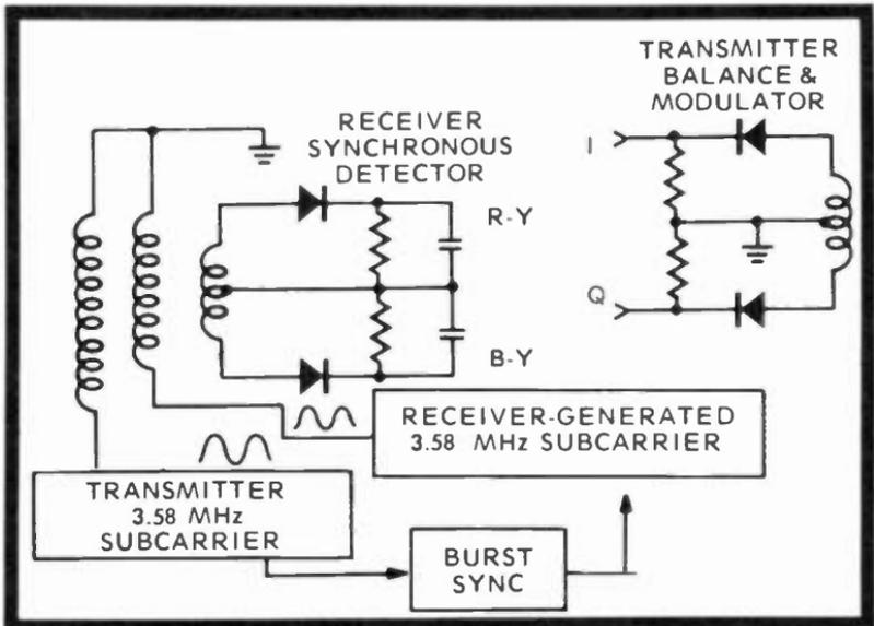
Fig. 12-7. Simplified modulation and demodulation diagram with subcarrier "sampling" diodes to produce colors at the conduction peaks. The transmitter 3.58-MHz oscillator syncs the receiver subcarrier oscillator by the sync burst.
