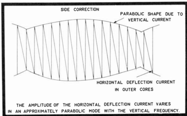
Fig. 10-8. Pincushion side correction currents used in the 4B25C19.
