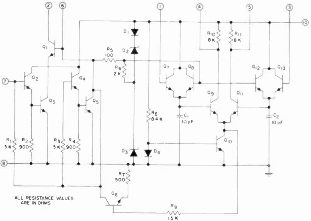
Fig. 5-21. Schematic of the CA3064 AFT IC.
