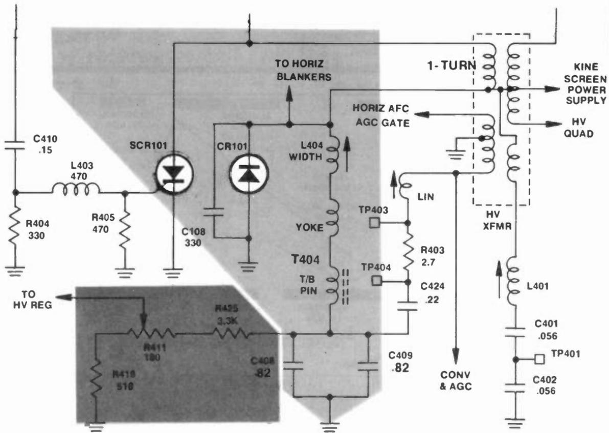
Fig. 9-9. Horizontal deflection and high-voltage regulation circuits.
