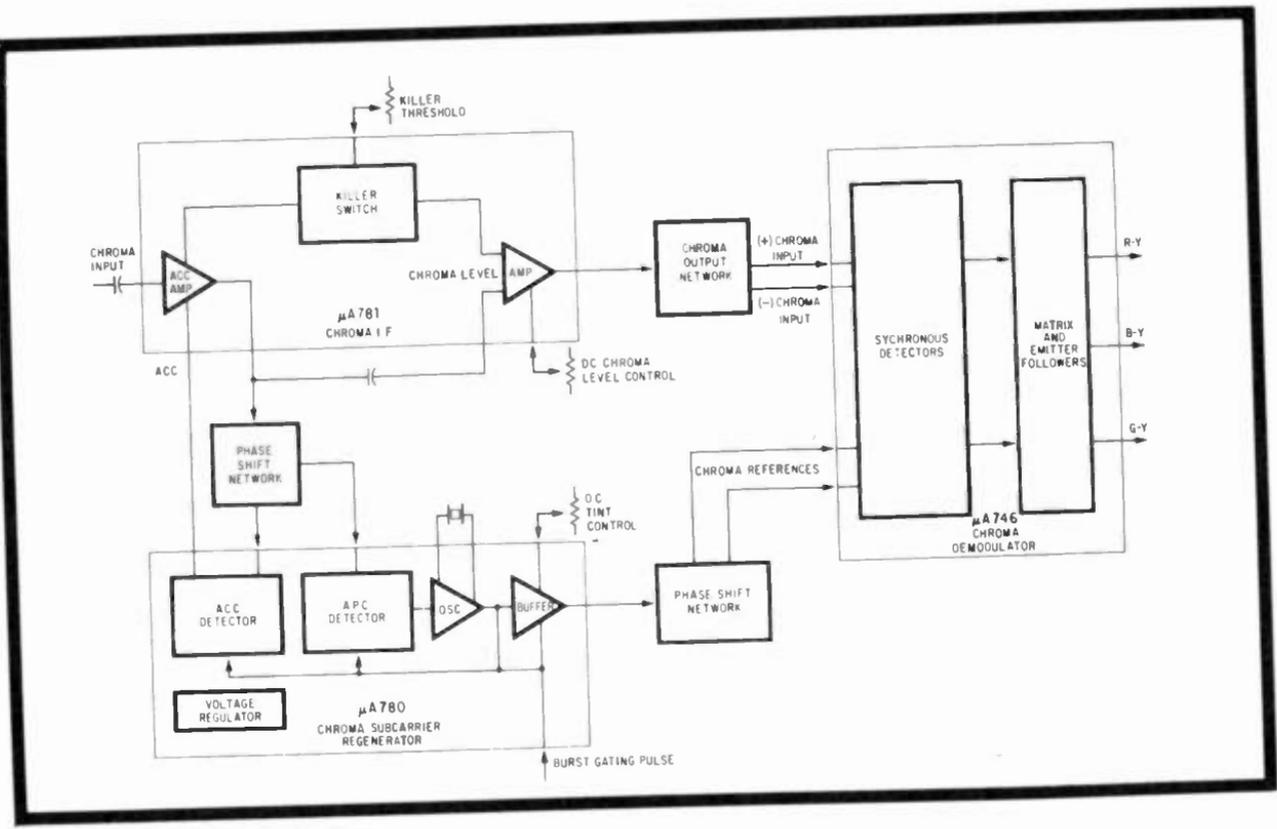
Fig. 12-15. IC manufacturer Fairchild's block diagram of the Zenith-developed three-chip processor. (Courtesy Don Smith)
