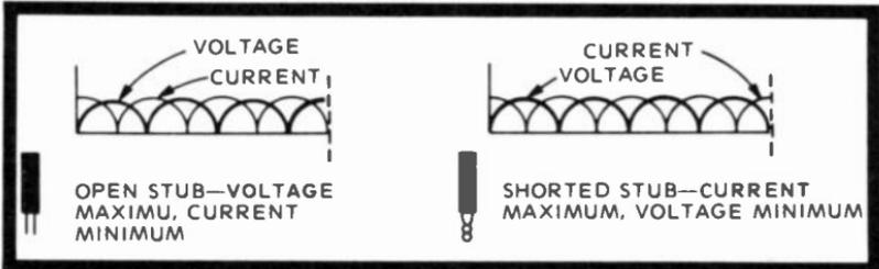
Fig. 13-3. Voltage and current on open and closed transmission lines.
