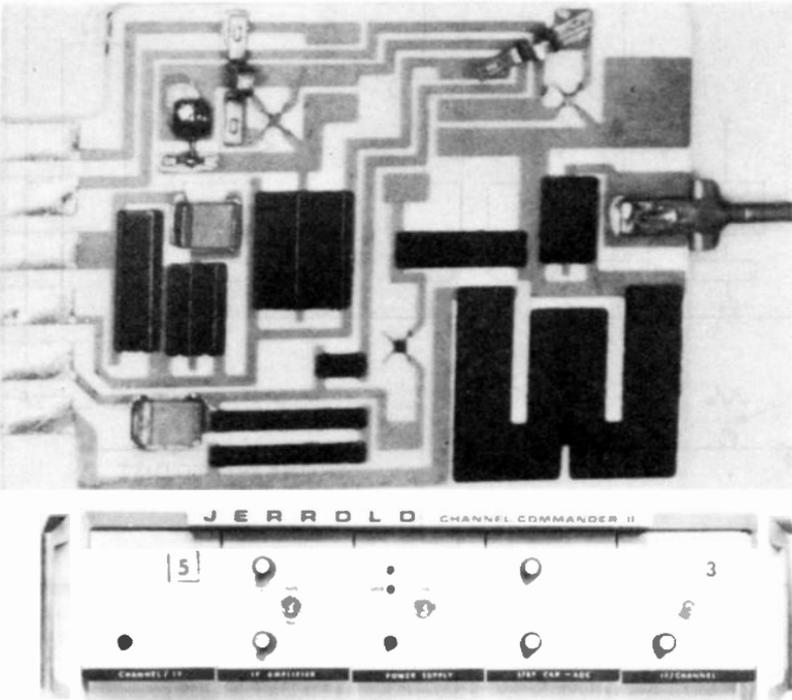
Fig. 15-5. Jerrold Channel Commander 11 signal processor. This one translates Channel 5 to Channel 3.
