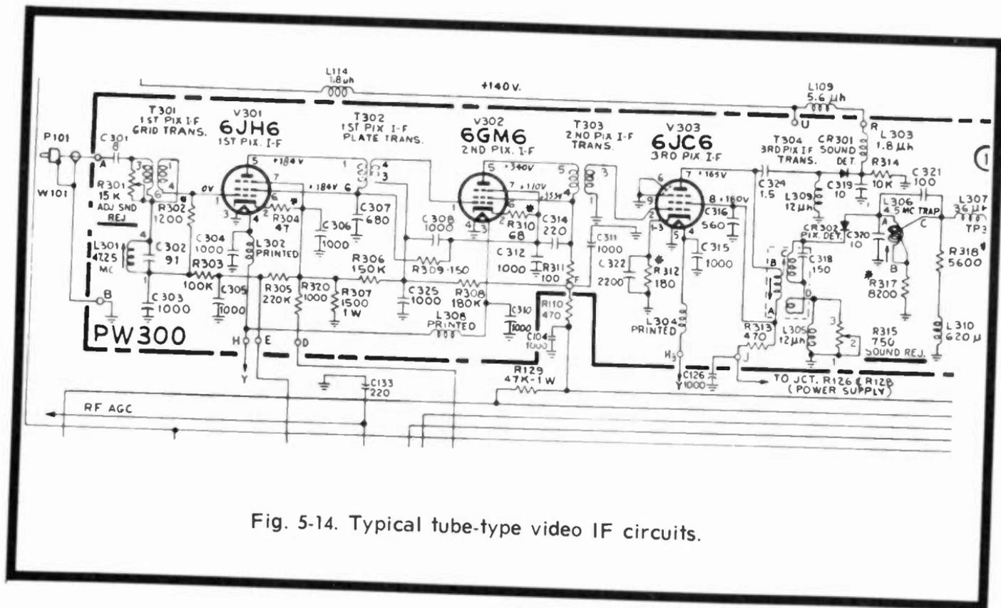
Fig. 5-14. Typical tube-type video IF circuits.
