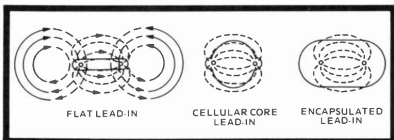
Fig. 13-4. Electromagnetic fields surrounding three types of lead-in cable. Observe that the encapsulated dielectric contains almost the complete field, substantially reducing skin losses.
