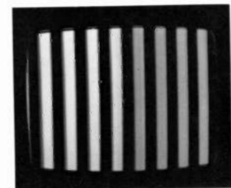
Fig. 14-63. Blue demodulator input failure.
