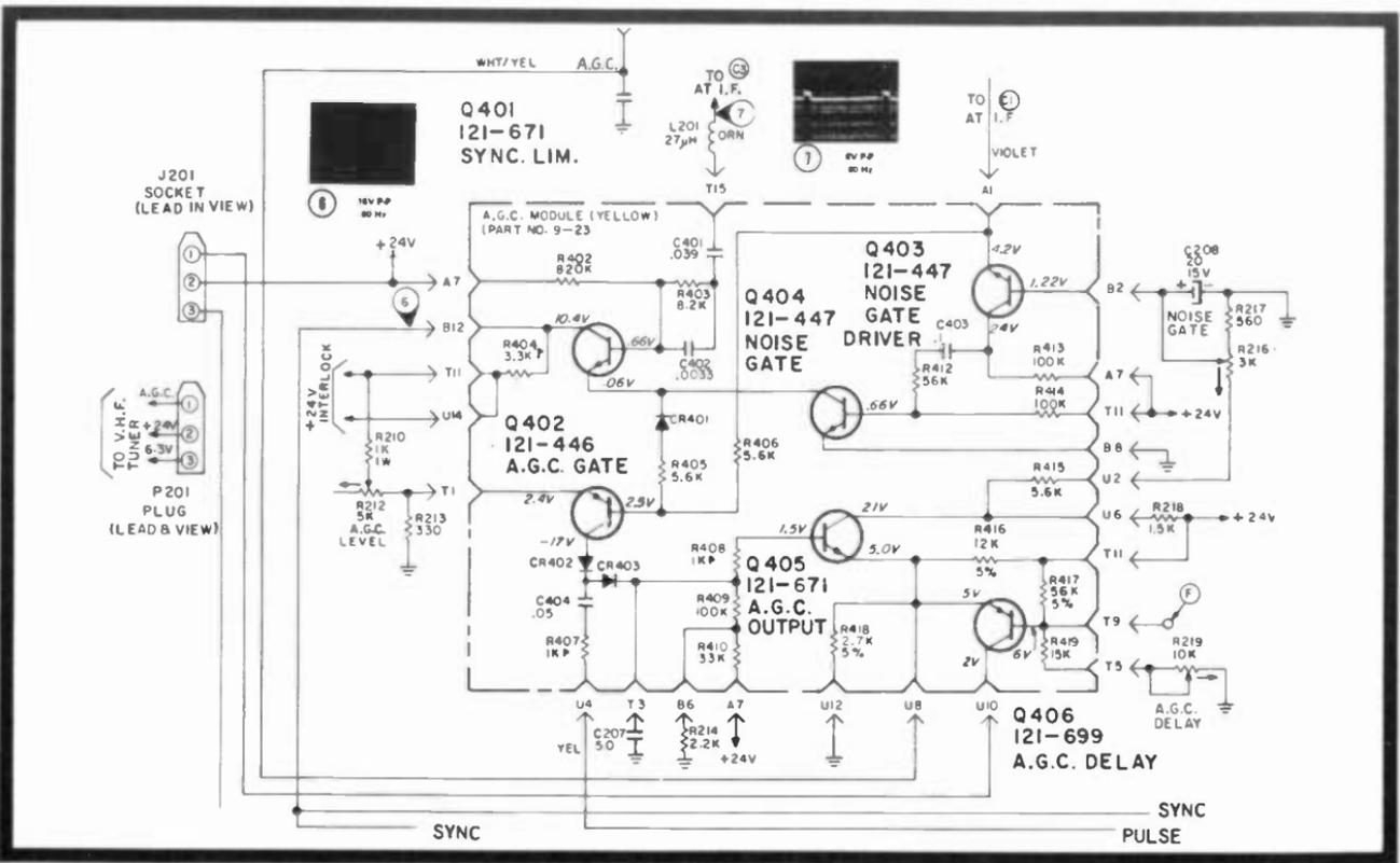
Fig. 7-3. Schematic of Zenith's 4B25C19 sync-AGC-noise module.
