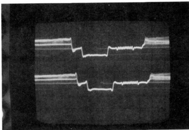
Fig. 6-5. If you want to check a delay line and see if it's actually working, here's how. The scope's time base is set at 2 microseconds per division. The delay is 0.8 microsecond; count it!
