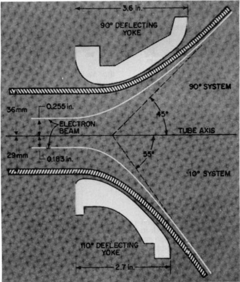
Fig. 2-11. Comparison of the 90- and 110-degree deflection yokes.
