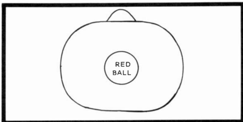
Fig. 4-5. A red ball appears as the tabs are adjusted for center purity, then the yoke is moved forward for a uniform red (or blue, green) field over the entire face of the CRT.
