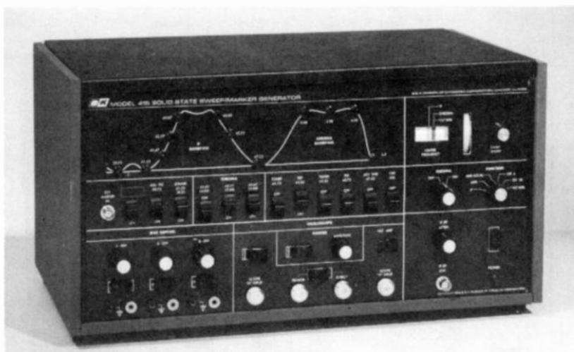
Fig. 14-20. B & K (Dynascan) Model 415 solid-state sweepmarker generator with RF on Channels 4 and 10 and lighted marker signals. Includes bias supplies, 400-Hz modulation, V and H markers and 14 crystals.
