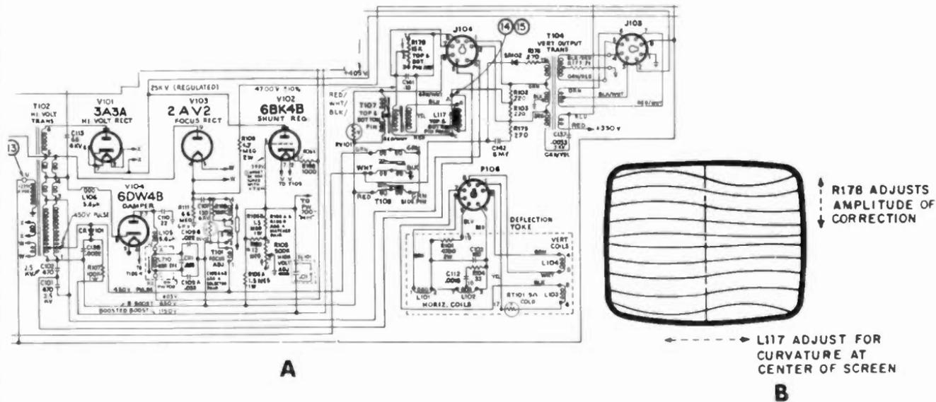
Fig. 10-2. A vacuum tube high-voltage subsystem with yoke and pincushion transformer circuits. The drawing illustrates the reason for center curvature and amplitude pincushion sweep corrections.
