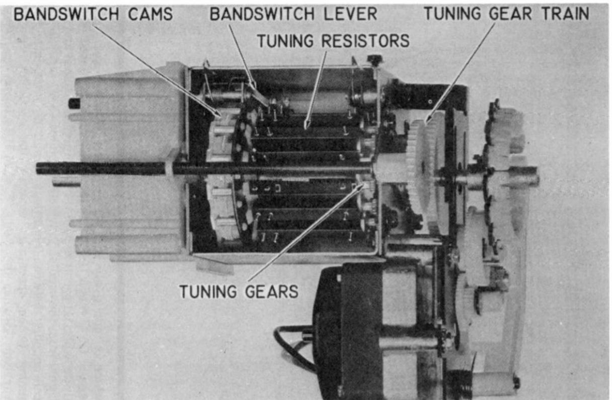
Fig. 5-9. UHF-VHF bandswitch, cams, and tuning resistors in Zenith's all-varactor tuner.
