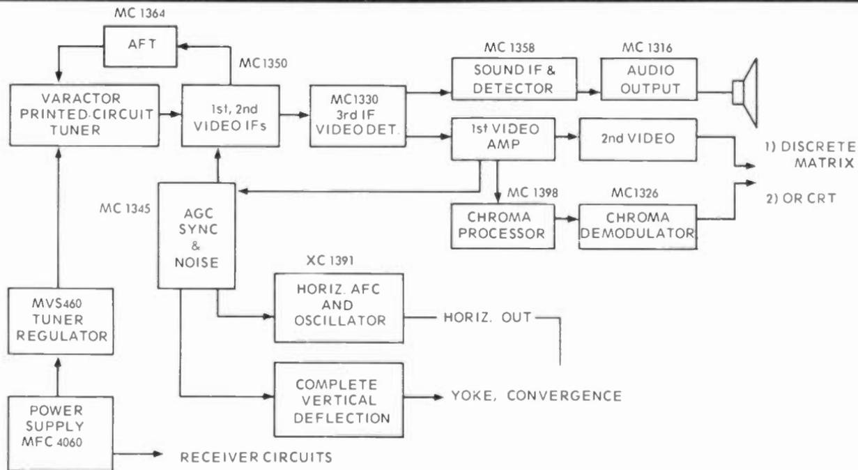
Fig. 1-21. A Motorola (Phoenix) version of a virtually all-integrated circuit receiver (Courtesy Ben Scott and Motorola, Phoenix, Ariz.)
