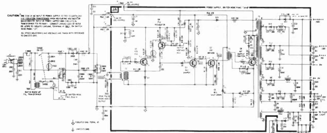
Fig. 11-7. Motorola's switch mode power supply schematic diagram. (Courtesy EI Mueller)
