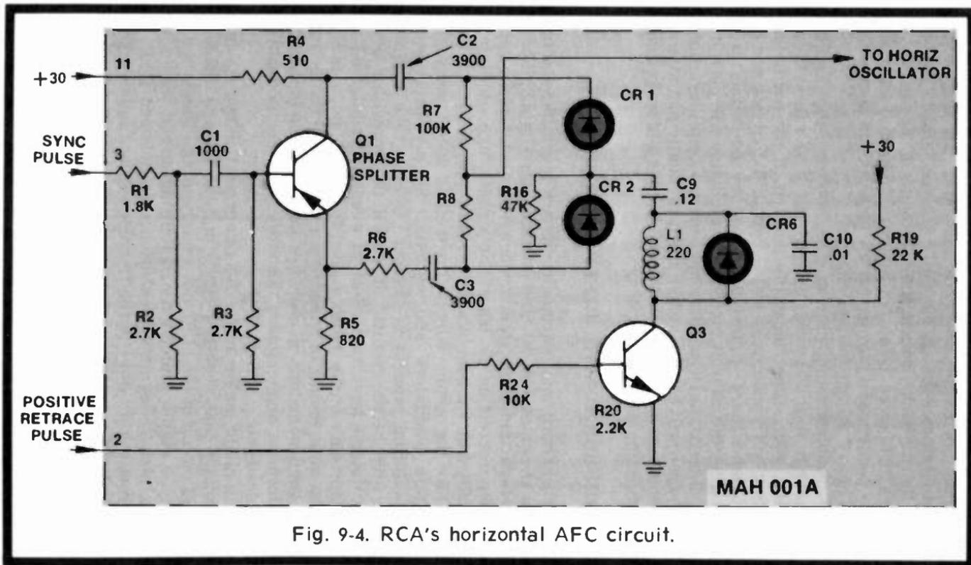
Fig. 9-4. RCA's horizontal AFC circuit.
