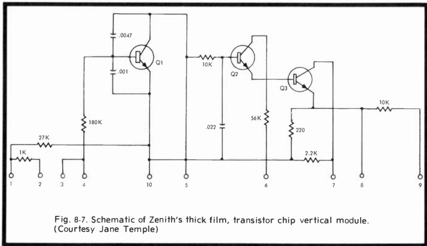
Fig. 8-7. Schematic of Zenith's thick film, transistor chip vertical module.
