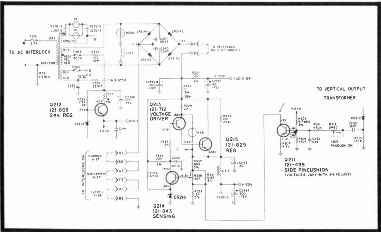
Fig. 11-4. The original low-voltage supply circuit for the 40BC50 Zenith and side pincushion correction circuit.
