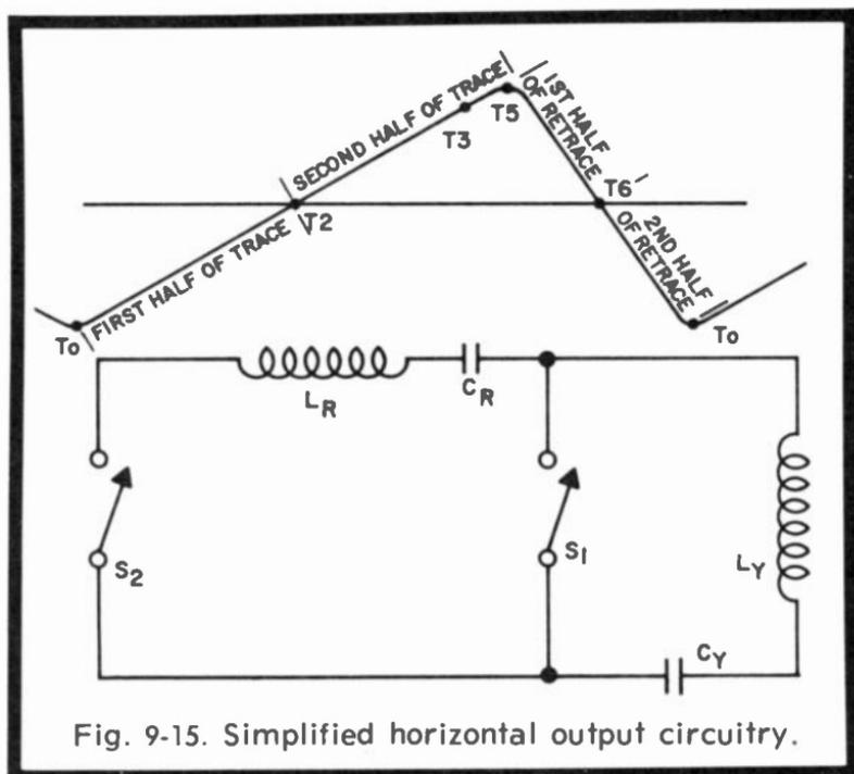
Fig. 9-15. Simplified horizontal output circuitry.
