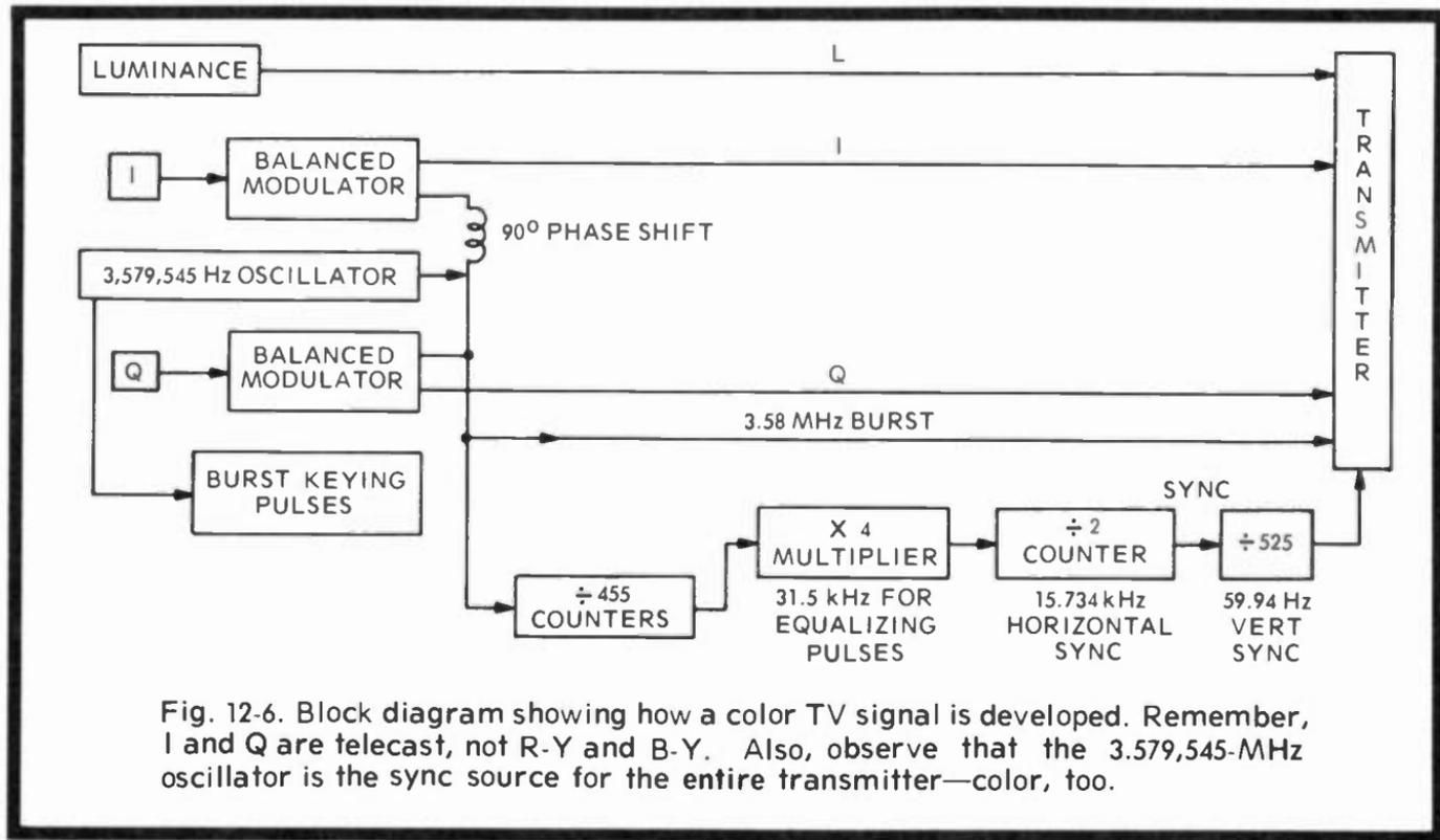
Fig. 12-6. Block diagram showing how a color TV signal is developed. Remember, I and Q are telecast, not R-Y and B-Y. Also, observe that the 3,579,545-MHz oscillator is the sync source for the entire transmitter—color, too.
