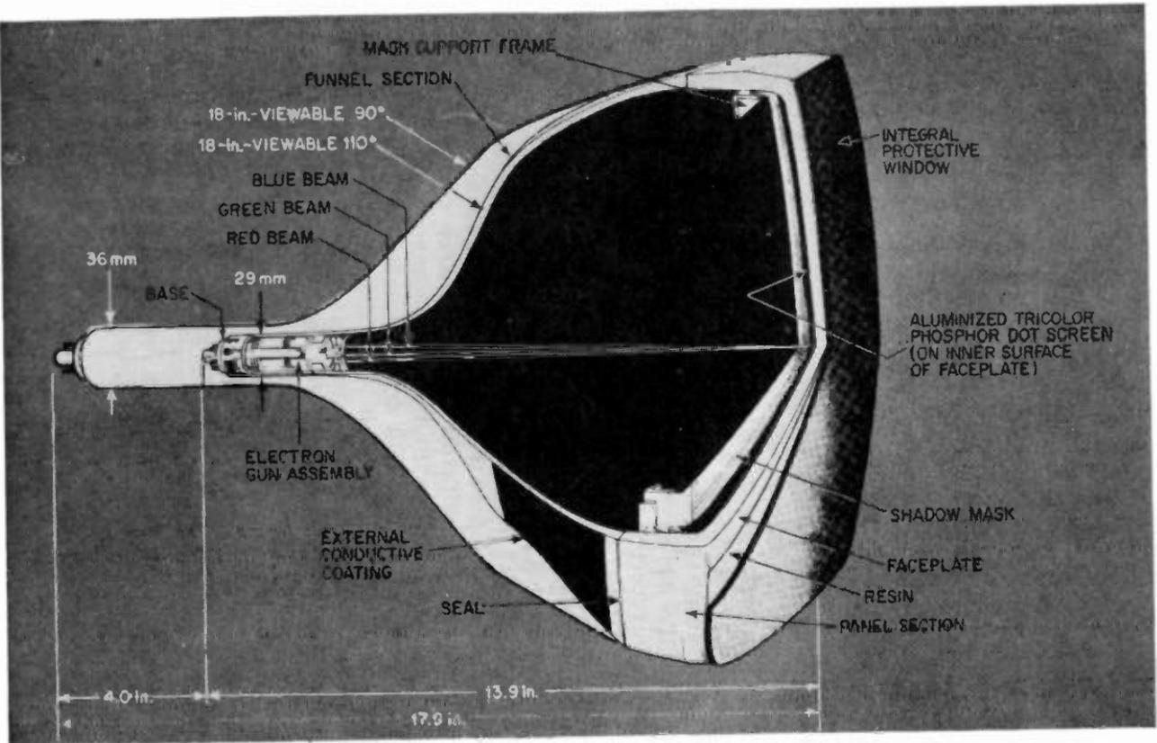
Fig. 2-10. Comparison of 90- and 110-degree cathode ray tubes exhibiting slim profile of the latter and the thinner, shorter tube neck. (Courtesy C.A. Meyer, RCA)
