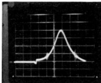
Fig. 14-41. Poor Channel 10 response, but markers are firmly in position, so try another more favorable channel.
