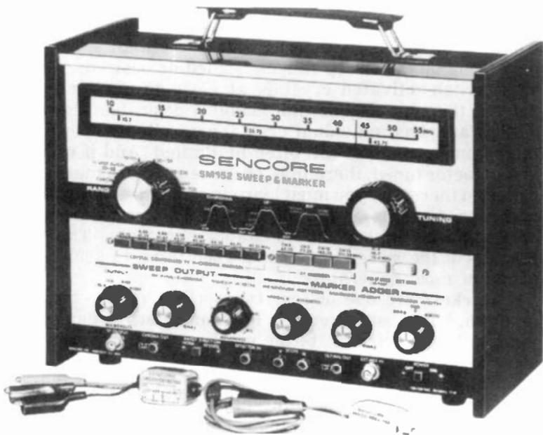
Fig. 14-18. Varactor-tuner SM152 Sencore sweep, crystal-controlled marker generator with ranges for 10 MHz to 900 MHz. It contains 13 close frequency crystal markers with both vertical and horizontal markers, virtually flat output.
