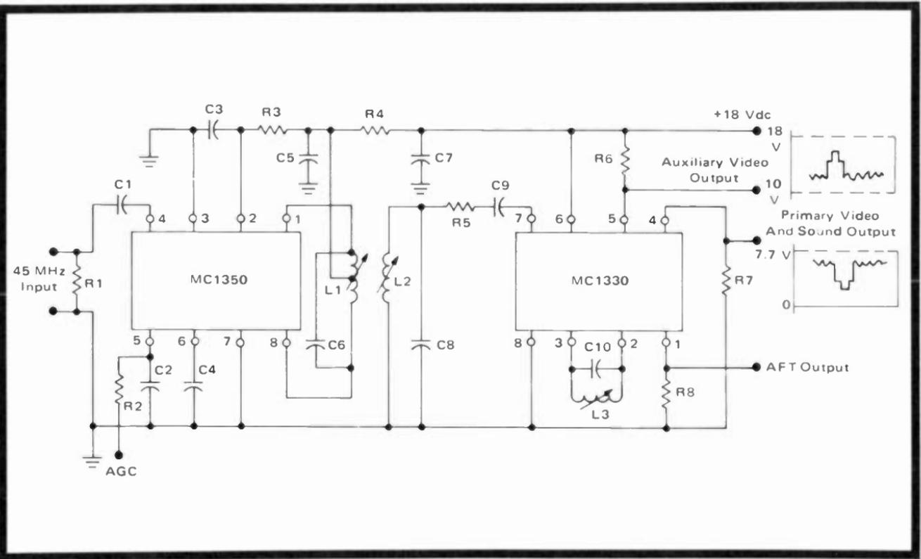
Fig. 6-12. IF system using an MC1350 (two IF amplifiers) and an MC1330 (final IF and synchronous detector).
