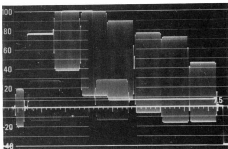
Fig. 3-6. Line rate display of EIA color bars. Notice the levels of the blanking and color burst. Both should always be seen in this display. (Courtesy Tektronix.)
