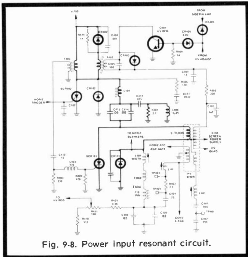
Fig. 9-8. Power input resonant circuit.
