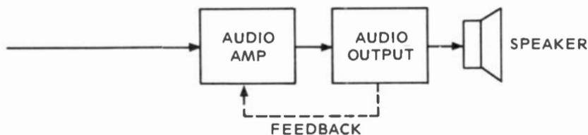
stages of audio amplification. The speaker in more recent receivers may be capacitor or transformer coupled.
