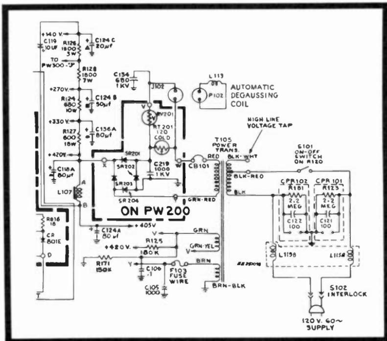
Fig. 11-2. Standard unregulated bridge-type supply circuit for vacuum tube receivers.
