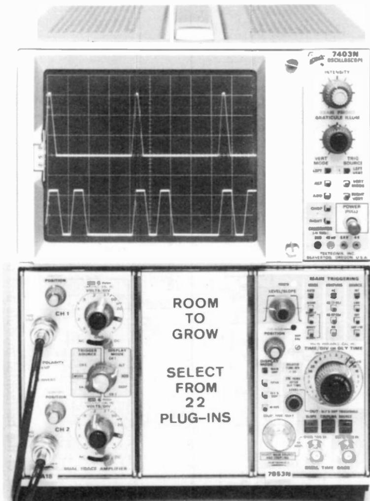
fig. 14-2. Tektronix 50-MHz oscilloscope with three plug-in units. It is accurate to 2 percent, with 1.22 cm per division. The unit features an 8 x 10 graticule, 5 mv per division vertical sensitivity, two time bases, and room to grow.
