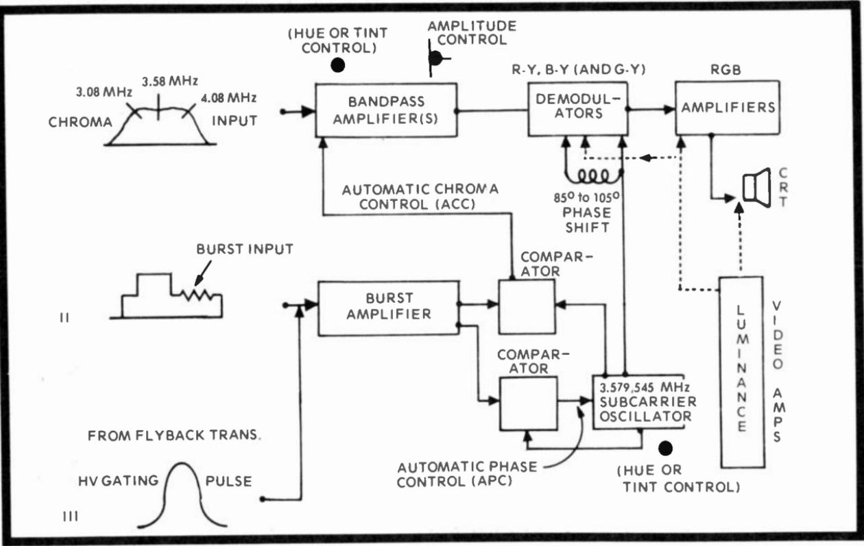
Fig. 12-1. Block diagram of the chroma subsystem found in any U.S. made color receiver. The arrows point in the direction of signal flow.
