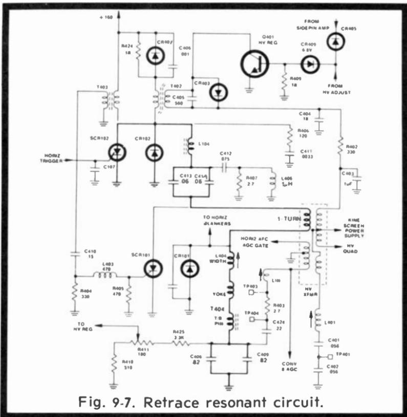
Fig. 9-7. Retrace resonant circuit.
