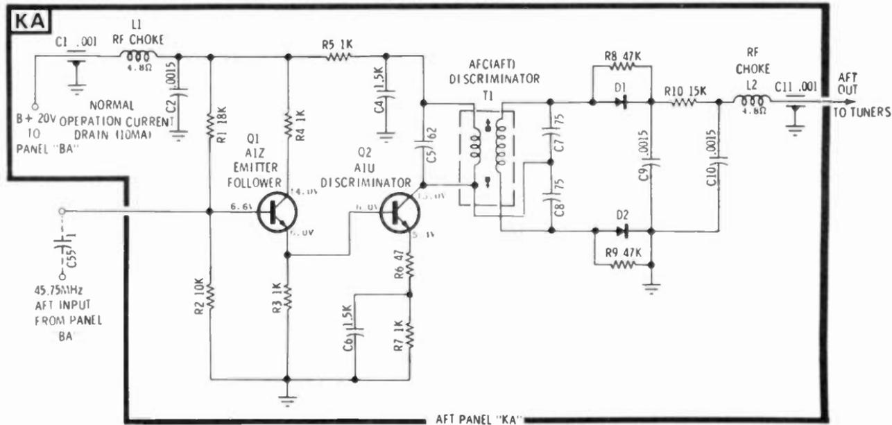
Fig. 5-19. Motorola's two-transistor AFT circuit built on a plug-in panel.
