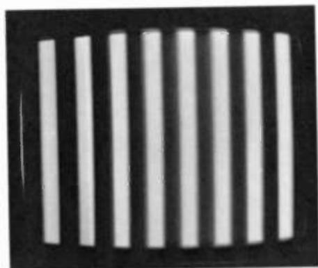
Fig. 14-61. Open input to the red demodulator.
