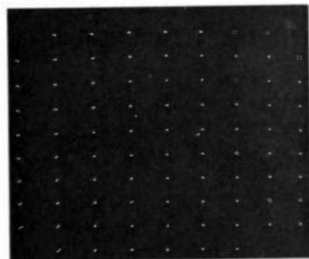
Fig. 14-77. Tiny, symmetrical dots readily show blue and red misconvergence at either edge.
