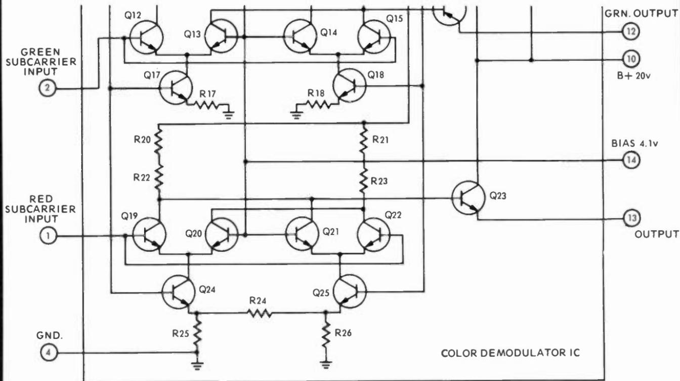
Fig. 12-12. Schematic of Motorola's tri-phase demodulator IC. The chip provides brightness, blanking, and voltage regulation functions. (Courtesy Bob Hansen)
