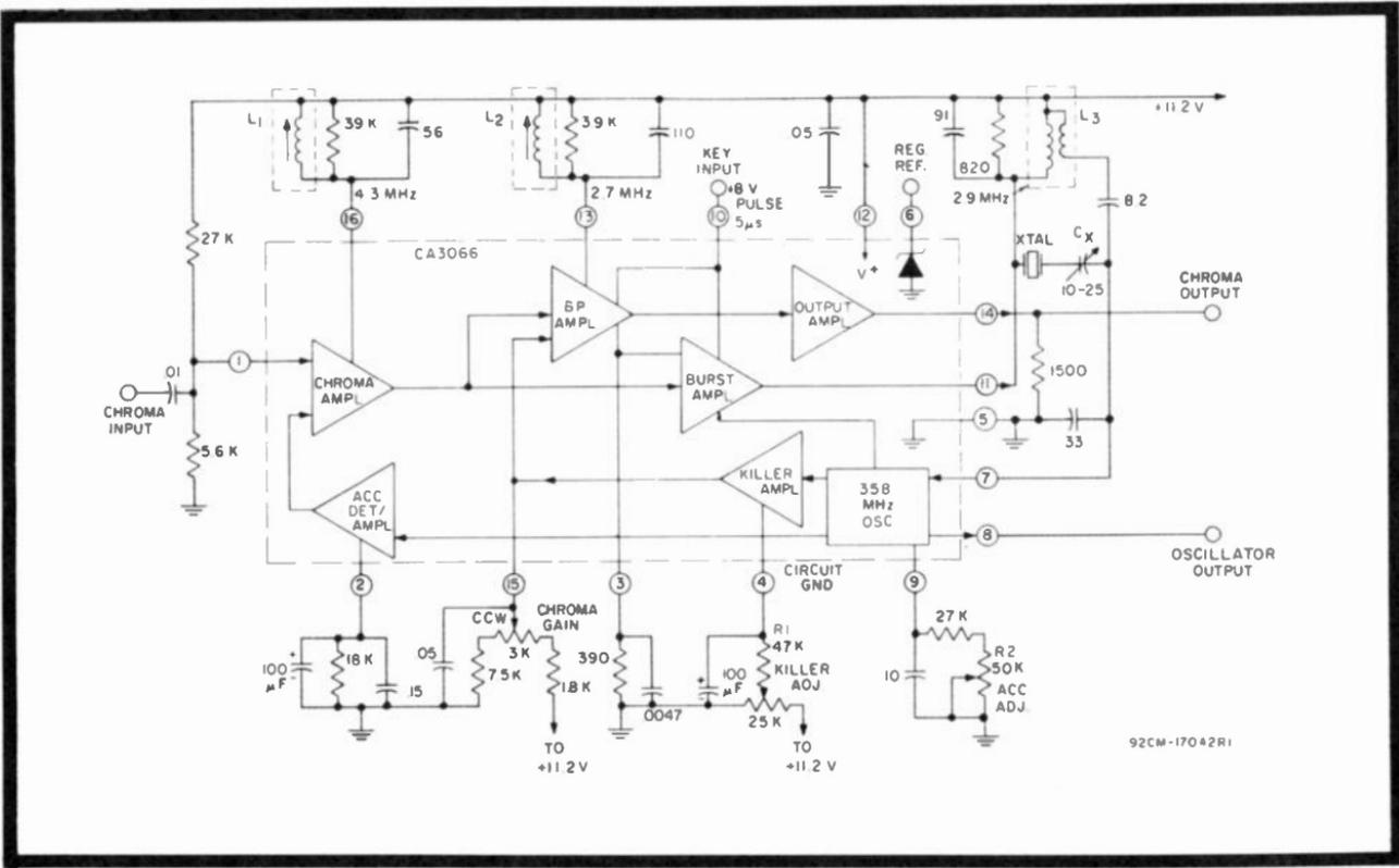
Fig. 12-22. Block diagram of the CA3066 chroma signal processor. (Courtesy RCA)
