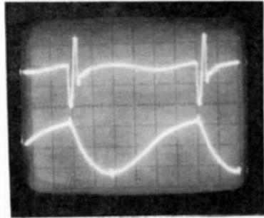
Fig. 14-13. Peaks are even in the oscillator output (top), and the lower drive pulses are clean. But this isn't the solution, believe it or not.
