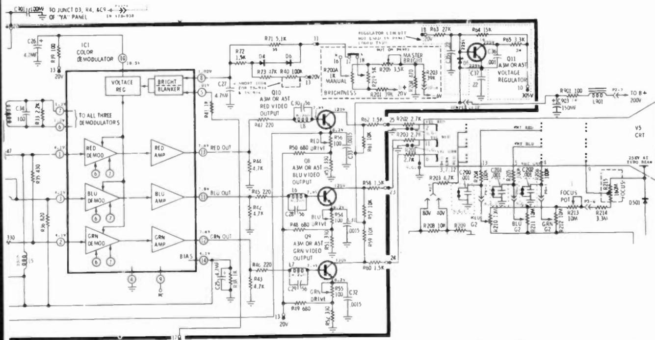
Fig. 12-10. Schematic of Motorola's color subsystem with two ICs and the discrete Instamatic circuits in between. Notice that luminance is added at the secondary centertap of T1 going into the demodulators. Other systems insert luminance after the demodulators.
