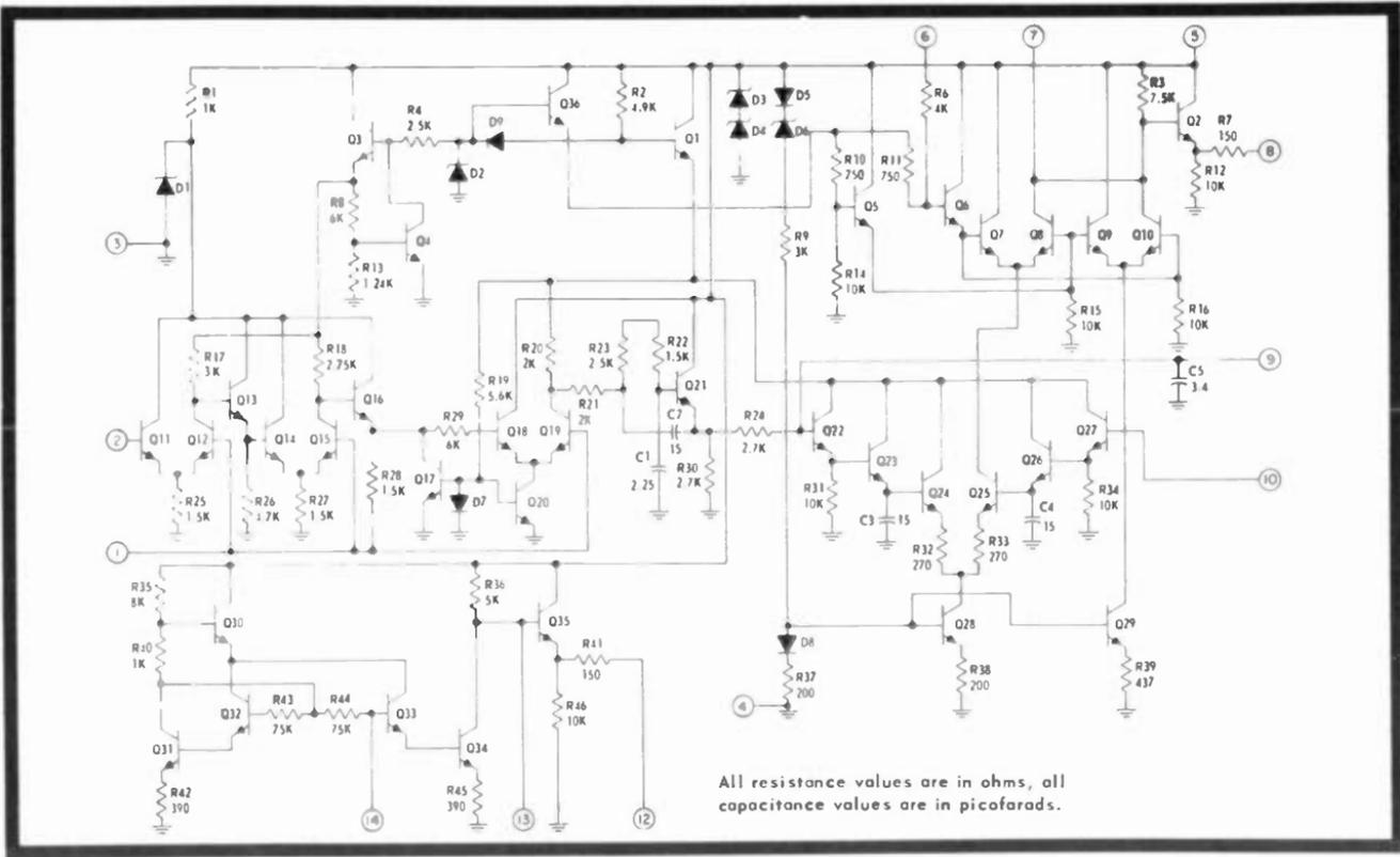
Fig. 6-21. Schematic diagram of the CA3065 IC sound detector.
