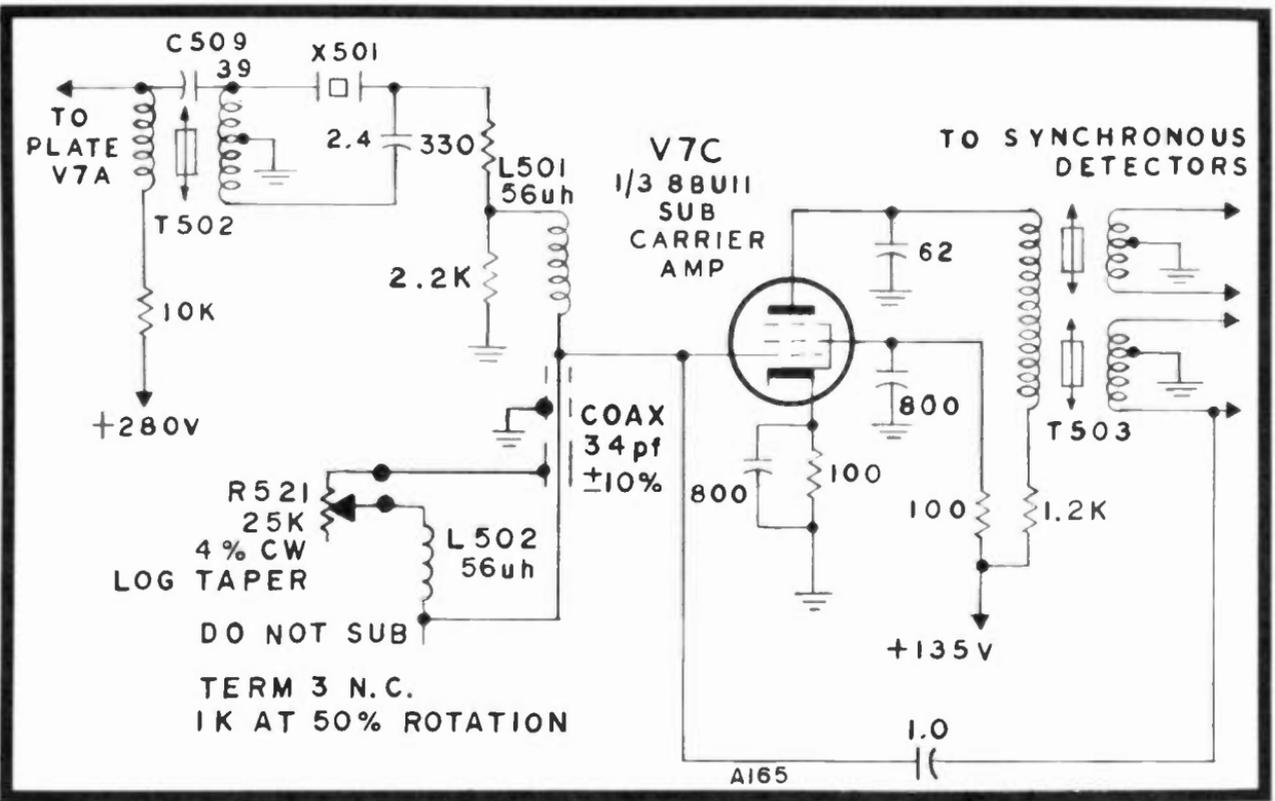
Fig. 12-9. General Electric's 3.58-MHz crystal ringing circuit. (Courtesy Bob Hannum)
