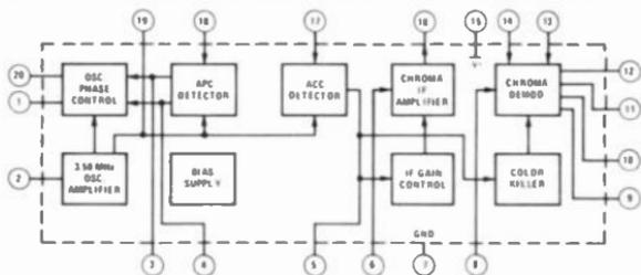
Fig. 12-26. uA782 block diagram.
