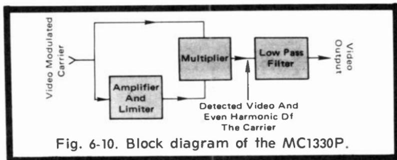
Fig. 6-10. Block diagram of the MC1330P.
