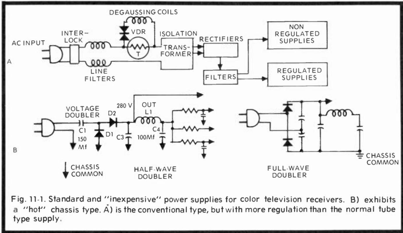
Fig. 11-1. Standard and "inexpensive" power supplies for color television receivers. B) exhibits a "hot" chassis type. A) is the conventional type, but with more regulation than the normal tube type supply.
