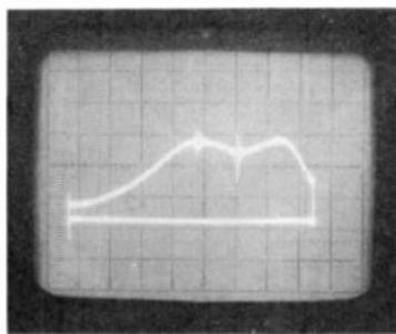
Fig. 14-35. Small markers help make precise adjustments in close chroma alignment.
