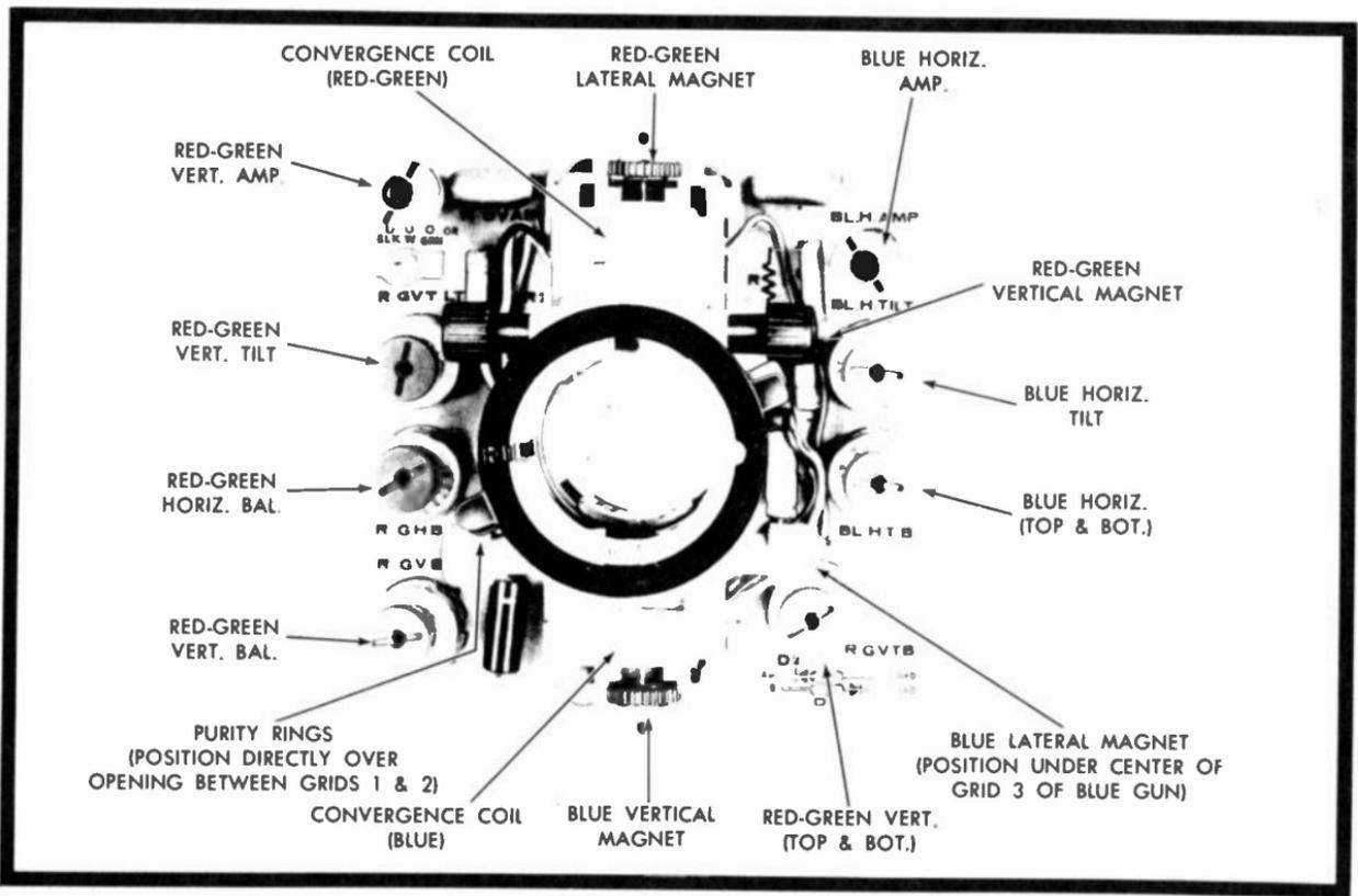
Fig. 4-17. View of the two-pole static and dynamic convergence components on the CRT neck in Zenith's 14CC14 through '16 chassis. Notice the red-green lateral magnet and different control terminology.
