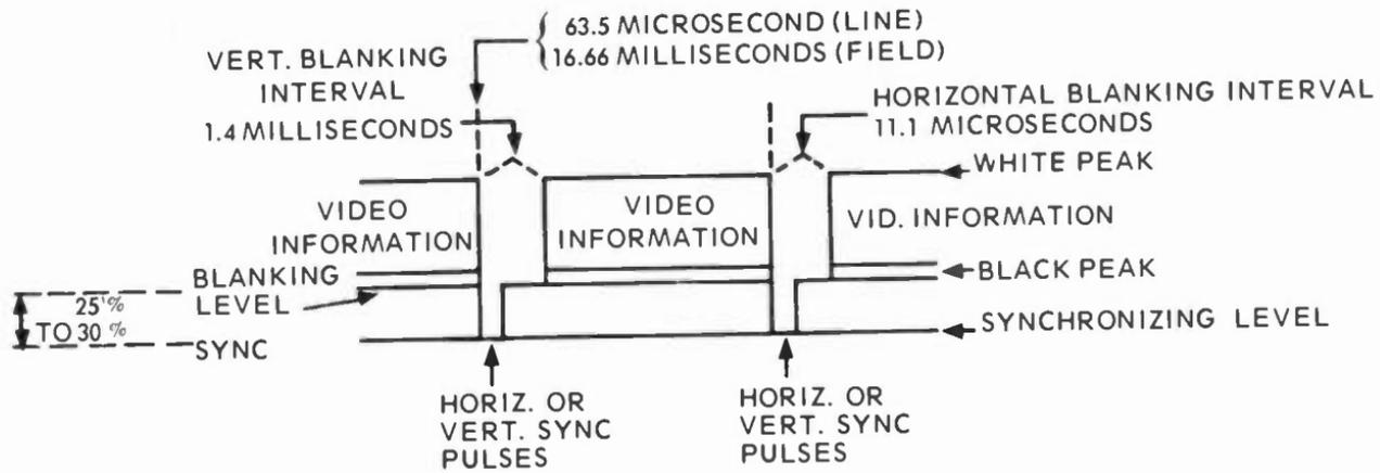
Fig. 1-8. A standard video waveform is very similar in appearance at both line (horizontal) and field (vertical) scope sweep frequencies. The difference is that at the line rate you're only viewing one or perhaps two lines of information, while at the field rate you see the entire raster scanned once for a field and twice (two complete cycles) for a frame (complete picture).
