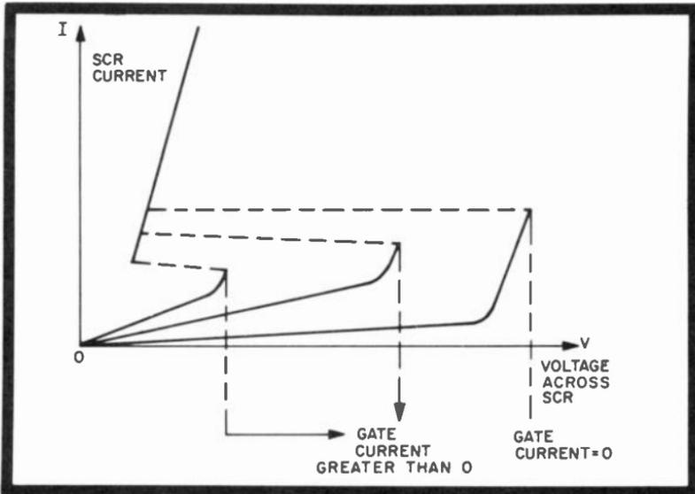
Fig. 9-12. SCR conduction and gate current relationship.
