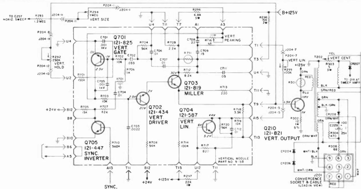
Fig. 8-6. Zenith's 40BC50 Duramodule vertical deflection subsystem circuits.
