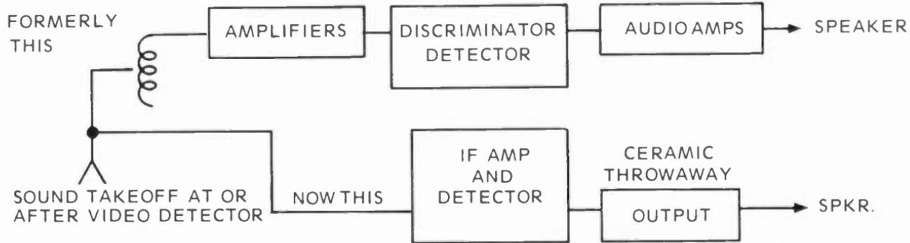
Fig. 1-20. The sound subsystem uses either tubes, discrete semiconductors, or all integrated circuits.
