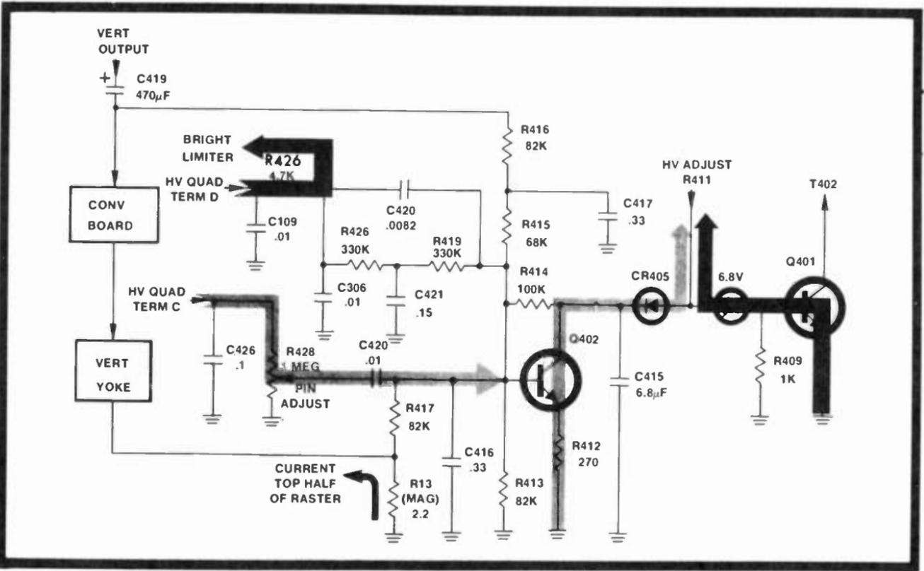
Fig. 10-10. RCA solid-state side pincushion amplifier. (Courtesy Carl Moeller)
