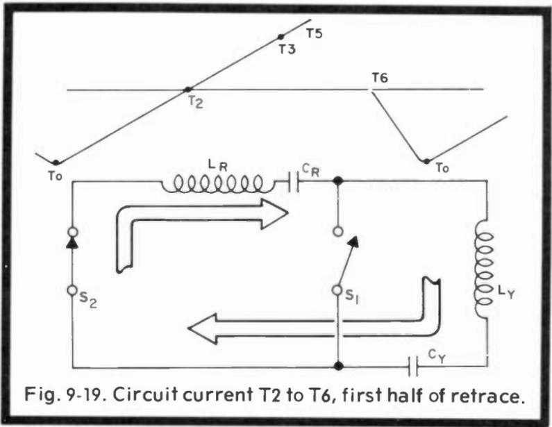
Fig. 9-19. Circuit current T2 to T6, first half of retrace.
