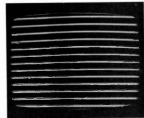
Fig. 14-75. These horizontal bars are almost useless because of line width variation.
