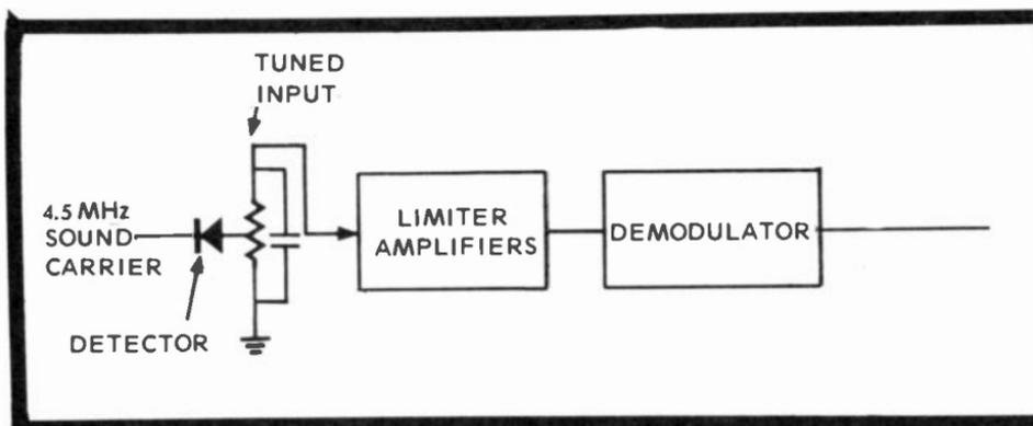
Fig. 6-13. Block diagram of a typical audio system showing detector diode, amplifiers, demodulator, and two
