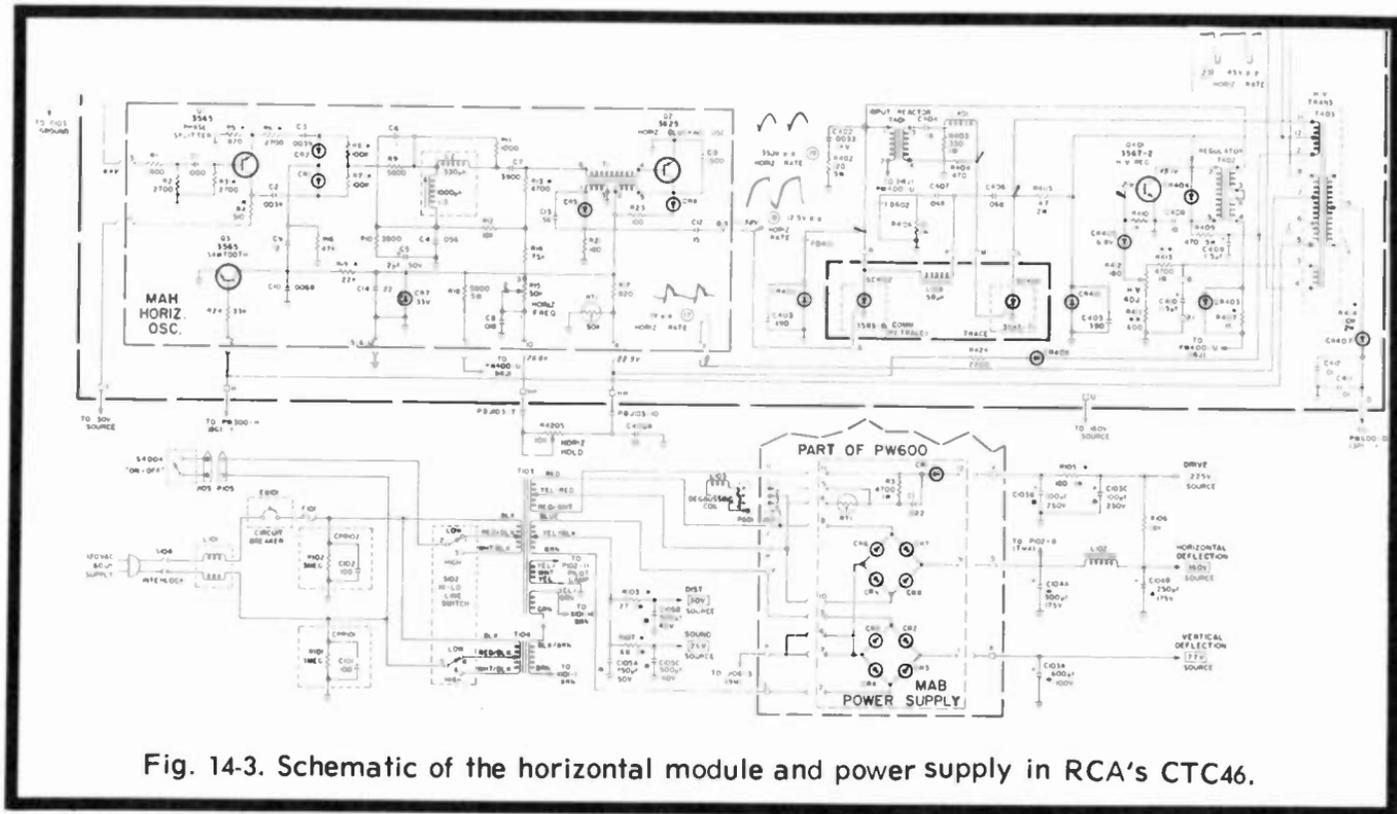
Fig. 14-3. Schematic of the horizontal module and power supply in RCA's CTC46.
