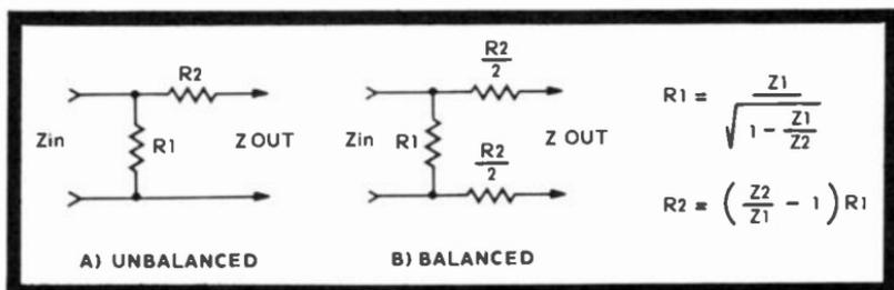
Fig. 13-8. Useful L pads in both balanced and unbalanced versions for matching different impedances with lowest loss.
