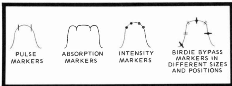
Fig. 14-17. Various types of markers are used. Markers must be added to the response curve only after the sweep has passed through all tuned circuits to prevent distortion.
