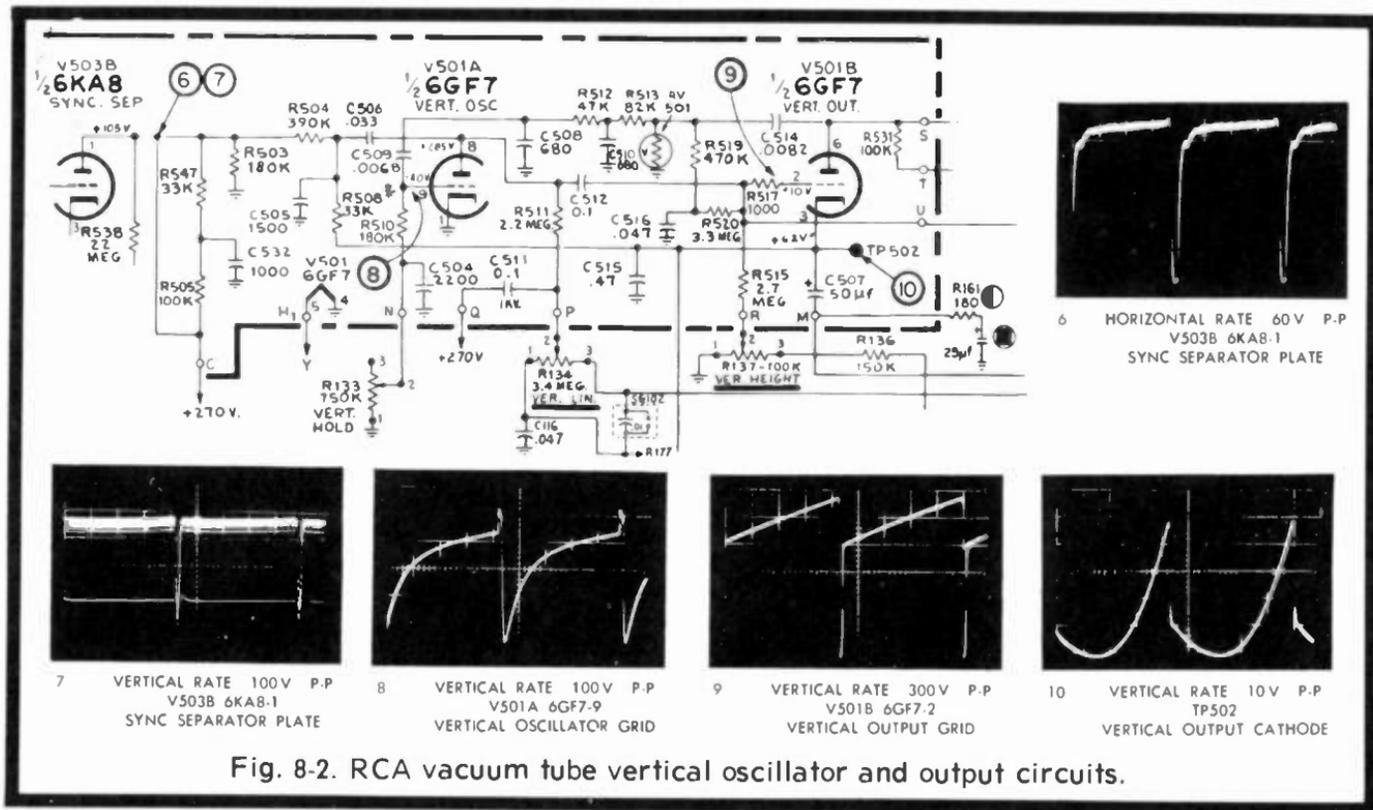
Fig. 8-2. RCA vacuum tube vertical oscillator and output circuits.
