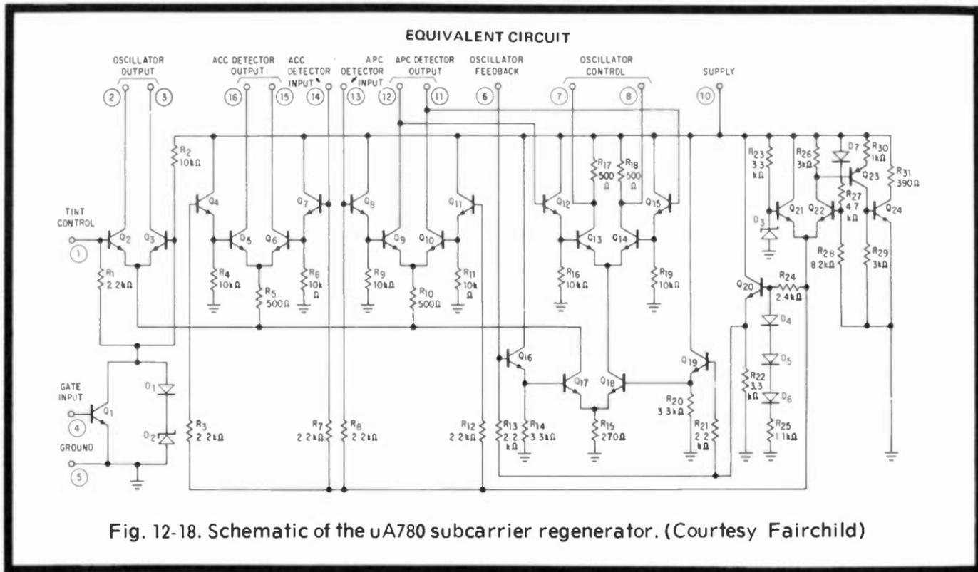
Fig. 12-18. Schematic of the uA780 subcarrier regenerator. (Courtesy Fairchild)
