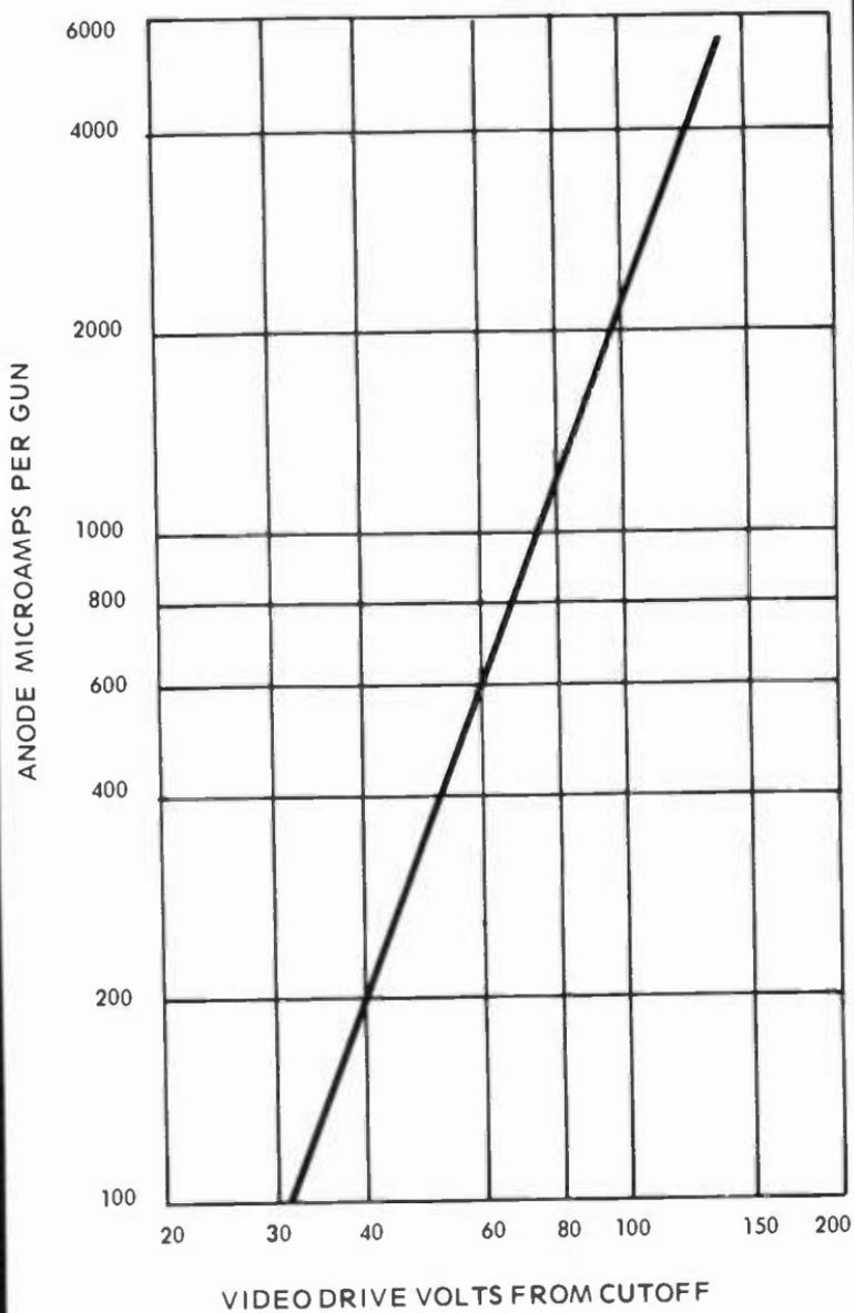
Fig. 2-17. Cathode drive-anode current relationship.
