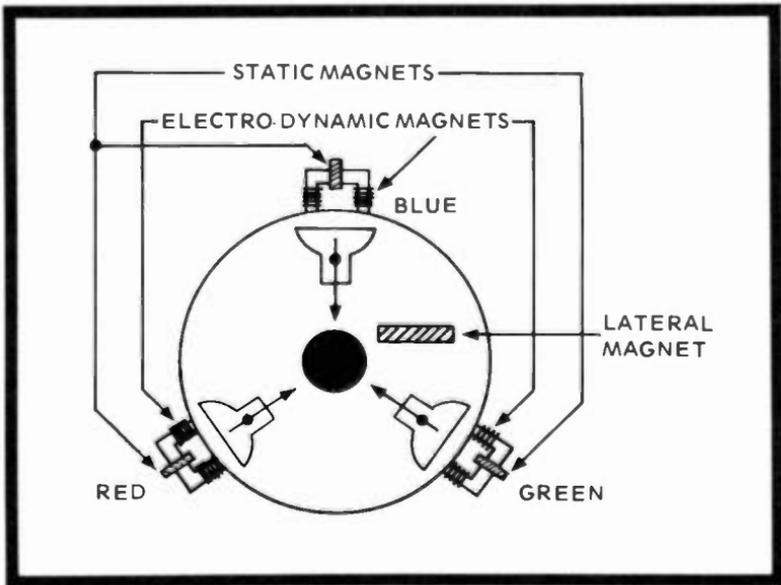
Fig. 4-8. Drawing of the convergence assembly placed over the three pole pieces inside the CRT gun. The arrow shows the direction of beam movement.
