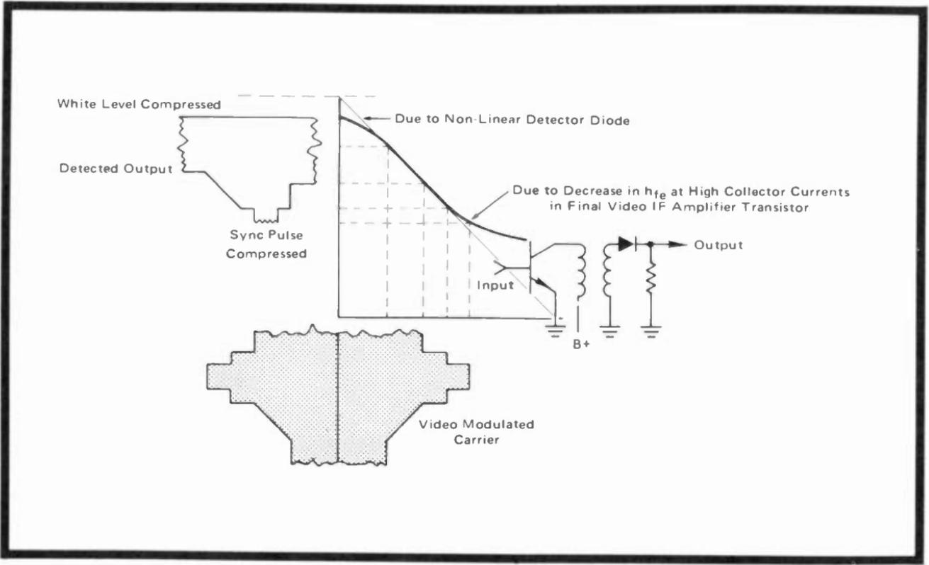
Fig. 6-7. Last video IF and diode detector transfer characteristics, showing the usual nonlinearities.
