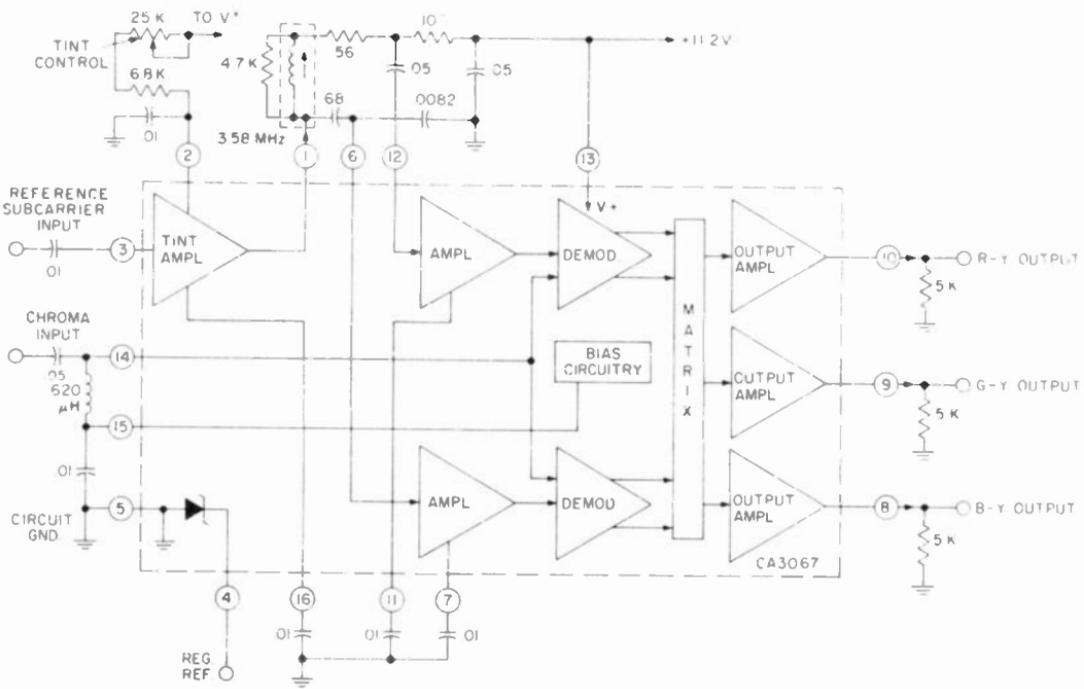
Fig. 12-24. RCA's CTC46, 54 Series CA3067 chroma demodulator functional drawing.
