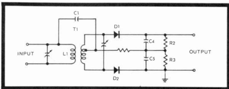
Fig. 6-14. Durable Foster-Seely discriminator circuit.
