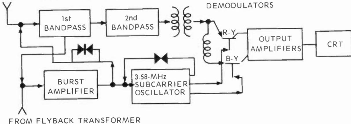
Fig. 1-19. Chroma amplifiers, bandpass amplifier, demodulators, output amplifiers, and the cathode ray tube comprise the chroma circuits. G-Y, as such, is not transmitted.
