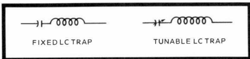
Fig. 13-13. Fixed and tunable LC traps can be used to shunt aside an unwanted frequency. A 20- to 100-pf capacitor is usually used for C.
