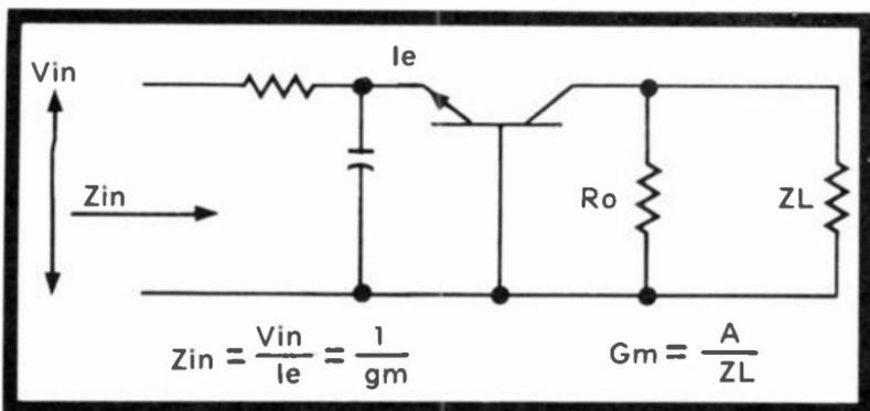
Fig. 7-7. Very simplified drawing of a common-base transistor IF stage. Gain is controlled by changing the input impedance.
