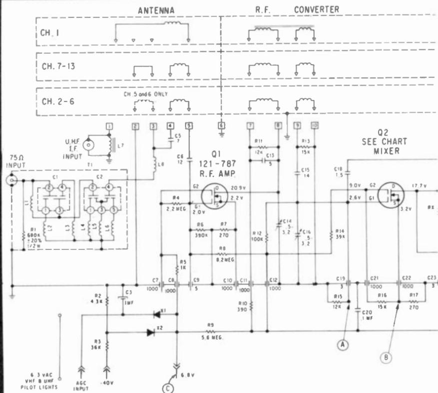
Fig. 5-8. Zenith's 175-1800 solid-state Gold Video Guard VHF turret tuner with two MOSFETs and a bipolar oscillator.
