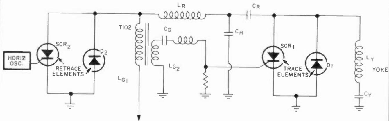
Fig. 9-14. Simplified horizontal output circuit schematic.
