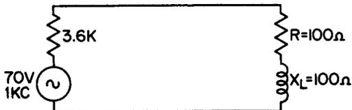
**Fig. 22.** Simple circuit for inserting impedance-matching transformers.
