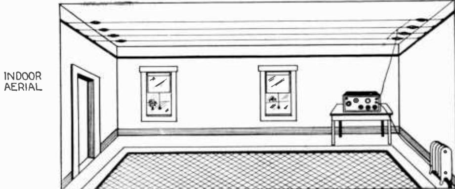
Fig. 3. Showing one method of installing an indoor aerial. While this illustrates a multi-wire type, a single wire run around the moulding of the room may give excellent results
