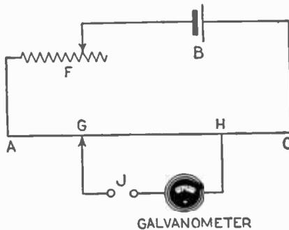
Fig. 2. A simple form of potentiometer used for electrical measurements.
