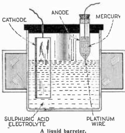
**LIQUID BARRETER**—An electrolytic detector which utilizes a very fine platinum wire dipped to a small depth in nitric or sulphuric acid. These detectors were formerly used to some extent in receiving wireless code messages. The electrolytic detector of the *barreter* type was invented and named by *Fessenden* (q.v.). The illustration shows a liquid barreter. In the glass jar is a platinum glass-anode, lead cathode and sulphuric acid electrolyte.
