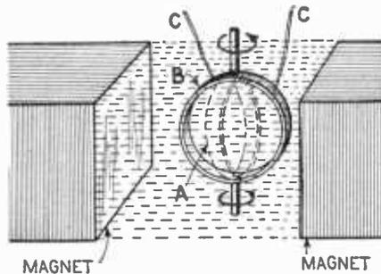
Fig. 2. Same coil, showing cutting of field due to the rotation of the coil.
