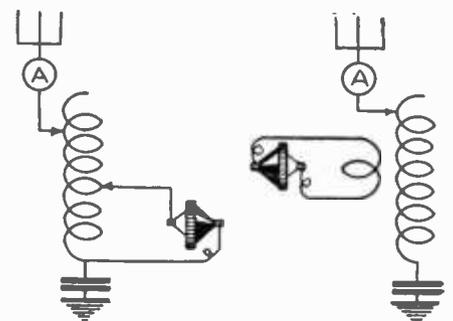
Fig. 19. Method of modulating output current.
