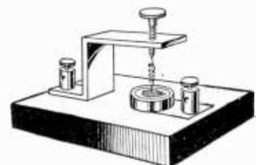
Fig. 1. Crystal detector using contact wire, or "cat-whisker."
