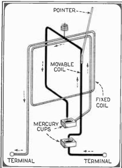
Electro-dynamometer with the current or moving coil shown by heavy lines and the stationary or voltage coil by light lines.
