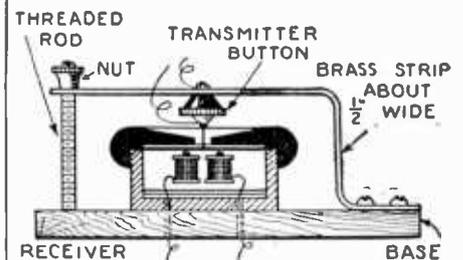
Fig. 7. Method of fastening a button to ear phone.
