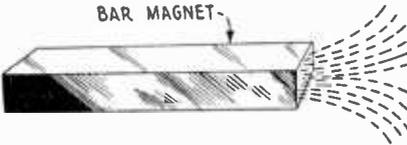
Fig. 1. Bar magnet, showing how the lines of force, or magnetic flux, create a magnetic field as indicated by dotted lines.
