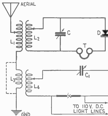
Fig. 1.—The original form of heterodyne receiver.
