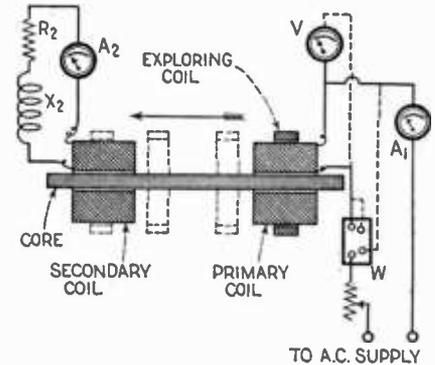
Diagram illustrating mutual induction. The reactance of the coil *A*<sub>1</sub> is reduced by the proximity of coil *A*<sub>2</sub>, since the circuit of *A*<sub>2</sub> contains no source of electromotive force. The effect of the secondary coil depends not only upon its distance from the primary coil but also upon *R*<sub>2</sub> and *X*<sub>2</sub>. The presence of the iron core greatly increases the action.
