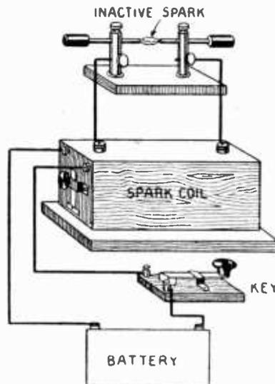
Fig. 1. Showing how an inactive spark is produced
