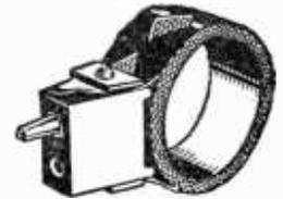
Honeycomb coil used in radio reception.
