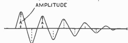
Fig. 2. Train of damped waves.
