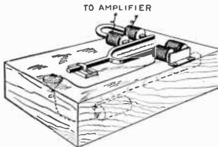
Fig. 14. A tuning fork oscillator.
