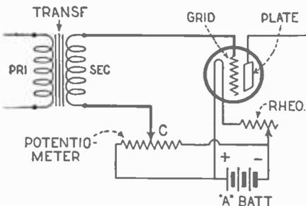
Fig. 2.—Method of connecting potentiometer in grid circuit.
