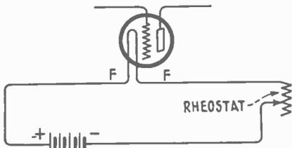
Method of connecting "A" battery in series with rheostat to regulate filament of vacuum tube.
