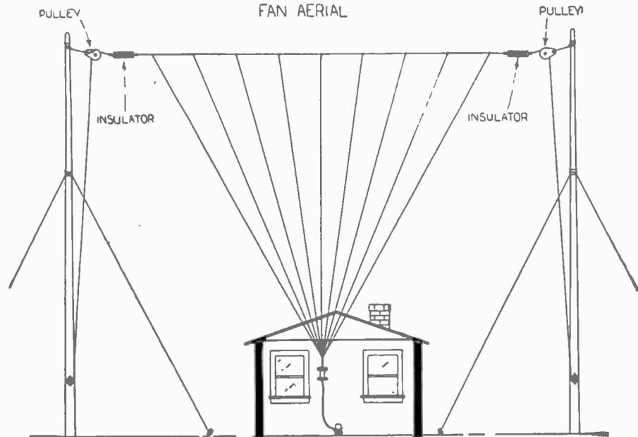
Fig. 5. The fan aerial has its wires spread apart at the farthest point, forming a fan
