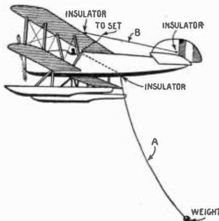
*terpoise* (q.v.) in this case may be another wire suspended on and insulated from the fuselage as indicated at B. When the plane is in flight, the hanging wire trails up and backward, depending on the speed of the plane and the size of the weight used. This type of antenna will be slightly *directional* (q.v.) in the direction the plane is traveling. If it is impractical to
