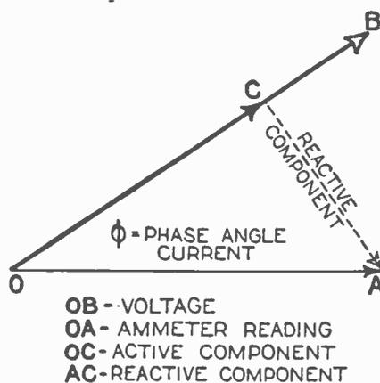
The current represented by vector OA may be considered as divided into two components. OC in phase with the voltage, and CA the reactive component.
