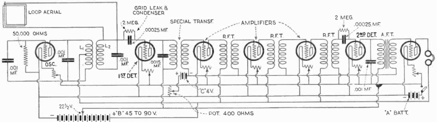
Fig. 2.—Wiring diagram of a standard 7-tube super-heterodyne.
