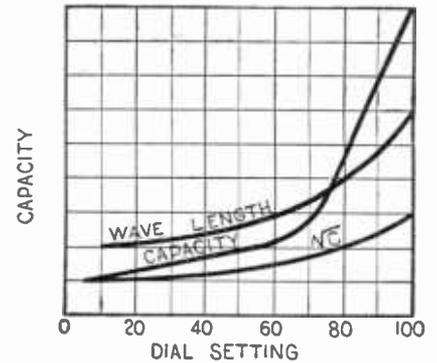
Fig. 1A. Curve for compression type condenser.
