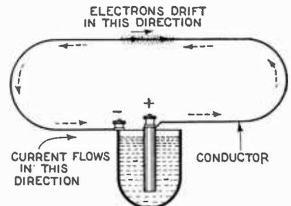
Fig. 2. Showing reverse action of current and electrons.
