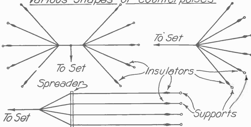
Fig. 11. Different methods of arranging counterpoises for either transmission or reception
