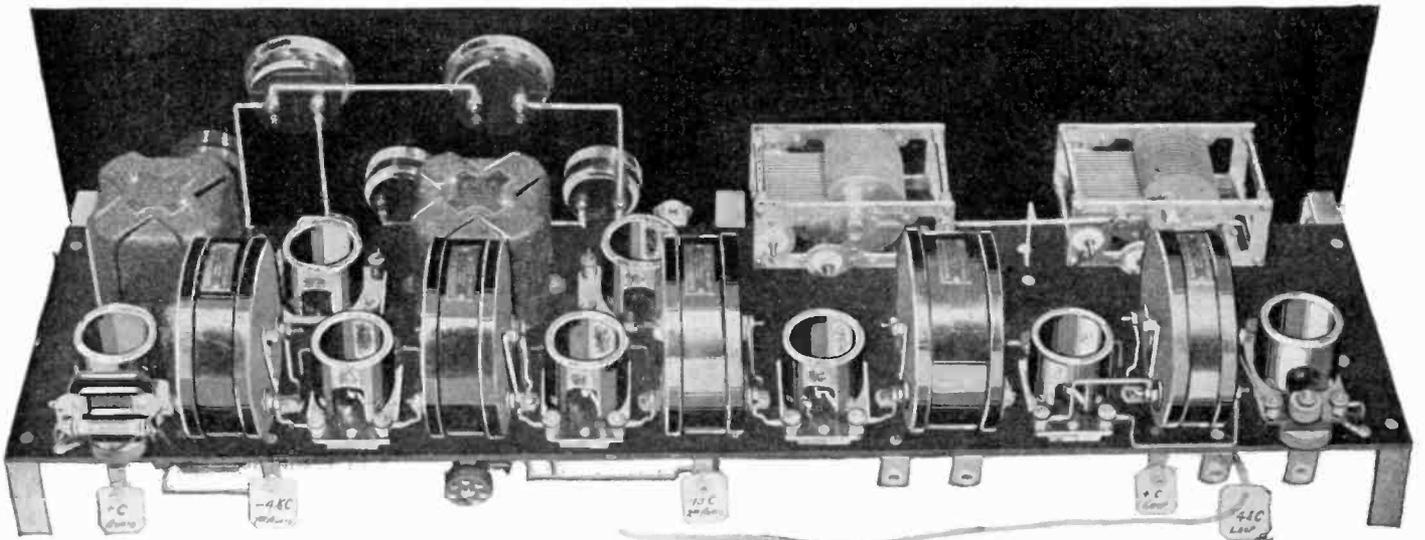
The photograph above shows an eight-tube super-heterodyne set of extra fine quality. Each of the heterofomers are shielded in nickel-plated metal shields. The two variable condensers for tuning the aerial and oscillator circuits should be of the straight line frequency type. The two audio frequency transformers are extra large concert type, the first stage of audio being all that is necessary for average reception on a loud speaker.
