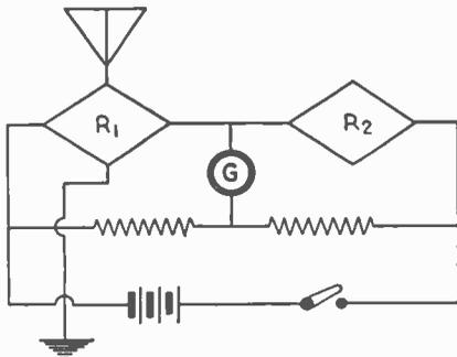
A thermal detector. By means of the change of resistance of a conductor, due to heating, electro-magnetic waves are detected. R<sub>1</sub> and R<sub>2</sub> are two rectangles of very fine iron wire.
