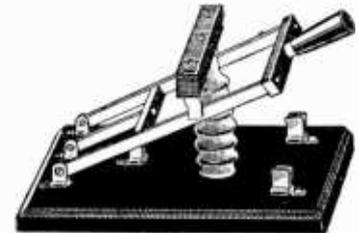
Fig. 4. An Aerial Switch with an extra blade
