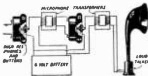
Fig. 11. An effective radio amplifier.
