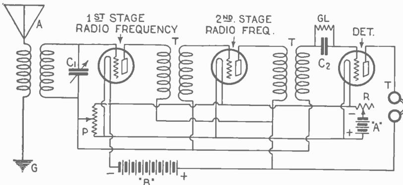
Fig. 1.—Circuit diagram showing two stages of cascade radio frequency amplification and detector.
