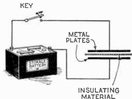
Fig. 1. A simple circuit for illustrating electrostatic induction.
