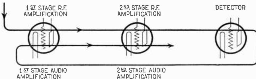
Diagram showing the current path and reflexing in an ordinary reflex circuit.
