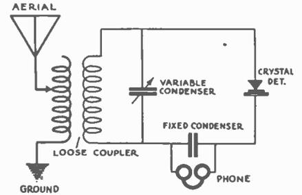
Fig. 3. Selective crystal receiver with loose coupler for tuning.
