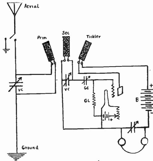
Fig. 72-D.—DeForest honeycomb coil type of receiver.
