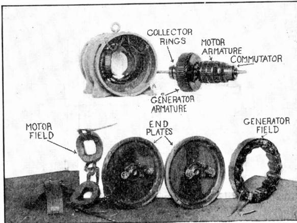
Fig. 15.—Exploded and Assembled Views of a Two-Kilowatt, Five Hundred Cycle Motor Generator Having Revolving Armature. (Courtesy of Crocker-Wheeler Company, Am-
