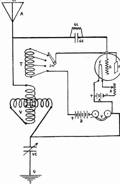
Fig. 72-C.—Diagram of single circuit Re-generative Audion Receiver
