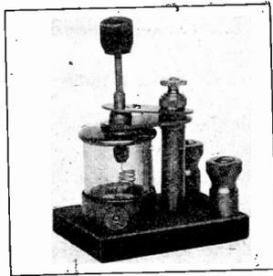
Fig. 62.—An Inclosed Type of Crystal Detector.
