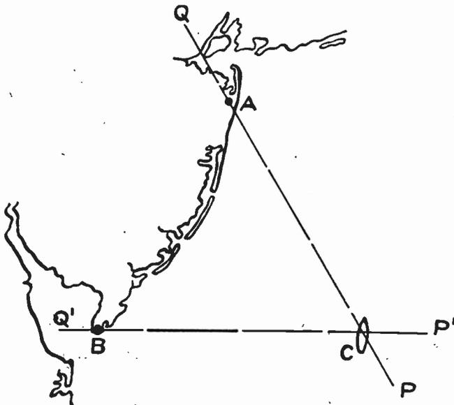
Fig. 75.—Method of Determining Absolute Direction and Location of Transmitting Station. (Courtesy of Robinson's Manual of Radio Telegraphy.)
