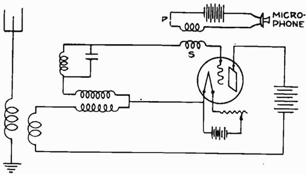
Fig. 55-B.—Diagram of simple microphone transmitter.
