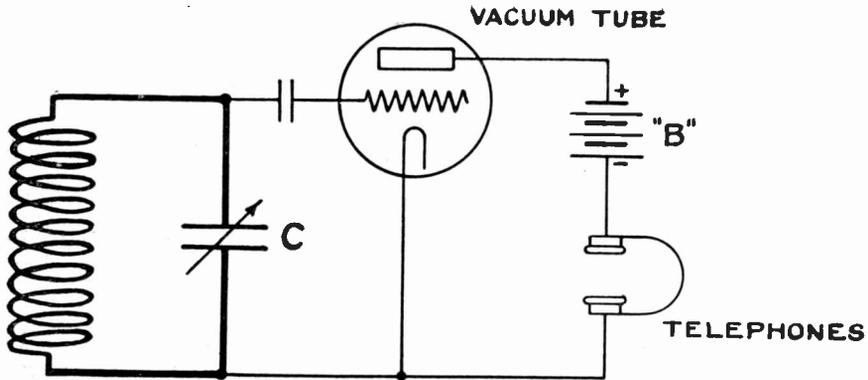
Fig. 74.—Arrangement of Tuning Coil and Detector. (The A or Filament Battery is Omitted Here. See Figure 66 for These Connections.) (Courtesy of Robinson's Manual of Radio Telegraphy.)
