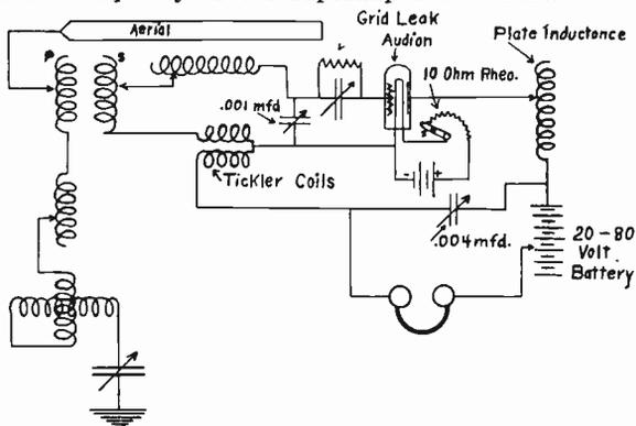
Fig. 72.—Wiring Diagram for a Regenerative Audion Hook-up.
