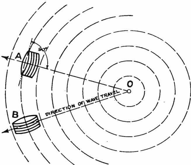
Fig. 73.—Showing Coil in Two Positions Relative to Field of Transmitting Antenna. (Courtesy of Robinson's Manual of Radio Telegraphy.)
