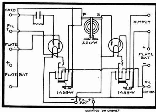
Fig. 72-B.—Diagram of connections of Audion and one step of Amplification
