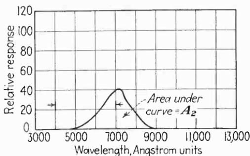
FIG. 40.—Response of the photoelectric surface to the spectral distribution of Fig. 39, determined by multiplying the curves in Figs. 35 and 39. The area under this curve,  $A_2$ , is compared with the area  $A_1$  under the curve in Fig. 36 to obtain the value of luminous sensitivity to the nonstandard light source.
