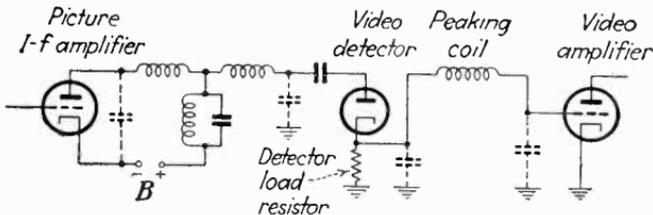
FIG. 189.—Typical video detector circuit.
