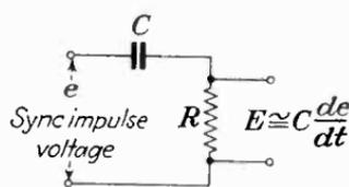
FIG. 221.—RC differentiating circuit.
