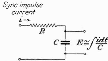
FIG. 222.— $RC$  integrating circuit.
