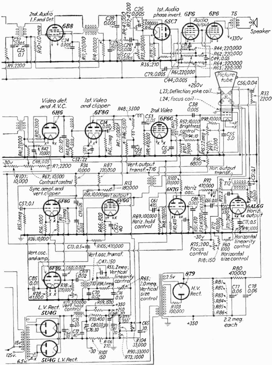
picture-tube receiver shown in Fig. 283.
