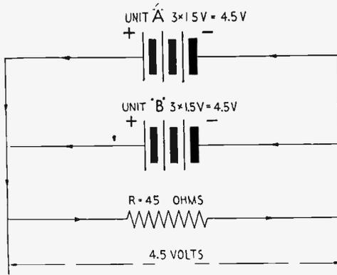
Fig. 8—Cells Grouped in Series Parallel.
