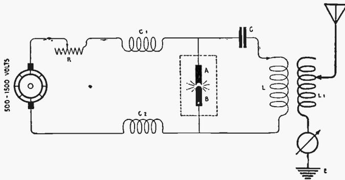
Fig. 278—Fundamental Diagram of the Poulsen Arc Generator.
