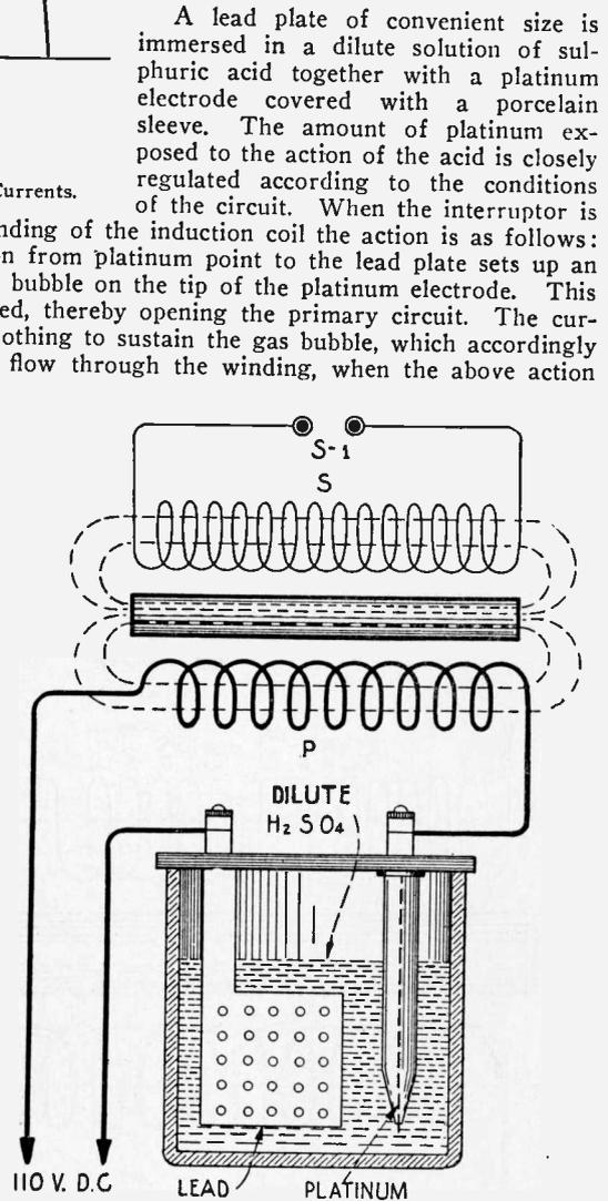
Fig. 59—Electrolytic Interrupter Connected to an Induction Coil.
