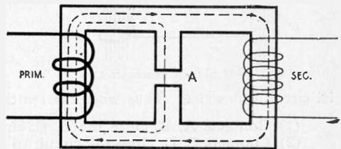
Fig. 133—Closed Core Transformer with Magnetic Leakage Gap.
