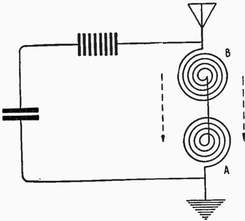
Fig. 124—Showing How Coupling is Changed by Vario-meter.
