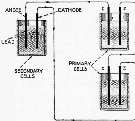
Fig. 4—Simple Diagram for "Charging" a Storage Cell.
