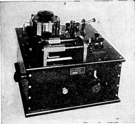
Fig. 268—The Tuned Receiver for the Direction Finder.
