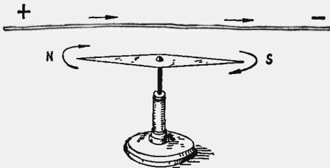
Fig. 11—Deflection of Compass Needle by Electric Current.
