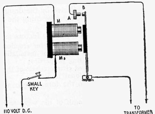
Fig. 138—Circuits of Magnetic Key.
