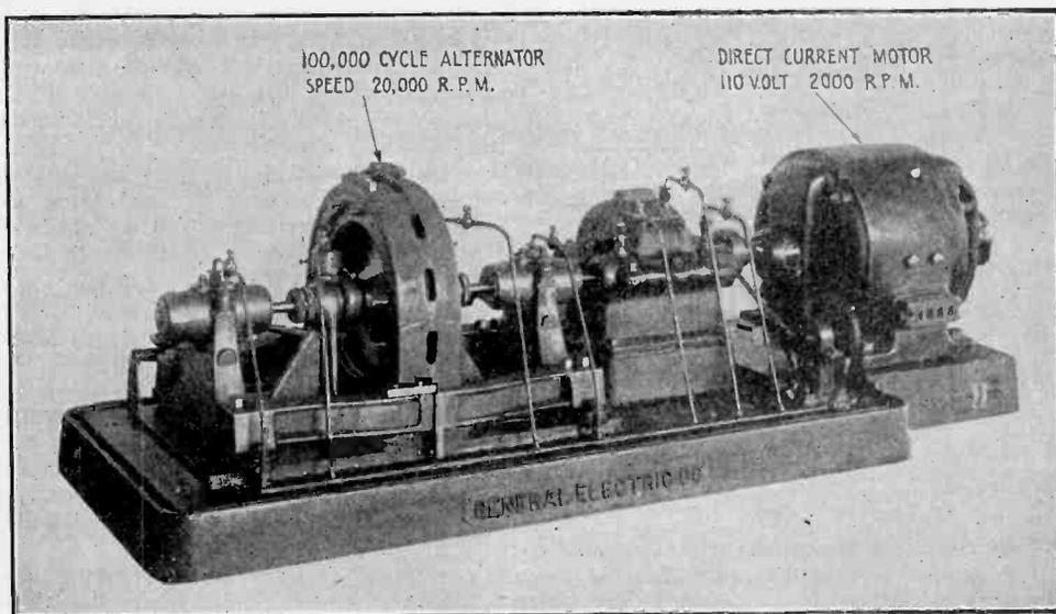
Fig. 280a—The 2 K. W. 100,000 Cycle Alexanderson Alternator.
