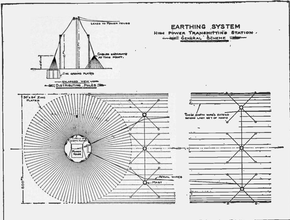
Fig. 320—General Scheme of Earth Connections for High Power Stations.
