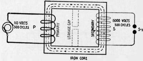
Fig. 37—Magnetic Circuit of Step-up Closed Core Transformer.
