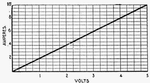
Fig. 155—Characteristic Curve of Ordinary Resistance.
