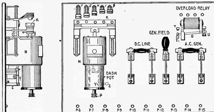
Fig. 251—Automatic Starter Panel (2 K. W. 500 Cycle Transmitter).
