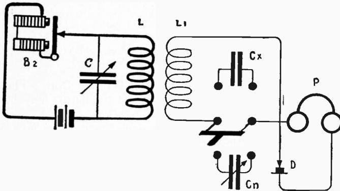
Fig. 228—Measurement of Electrostatic Capacity at Radio Frequencies.
