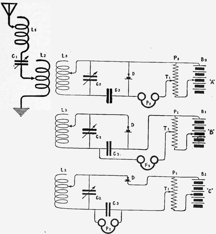
Fig. 153a, b, c—Complete Circuit for the Carbide Rectifier and Receiving Tuner.
