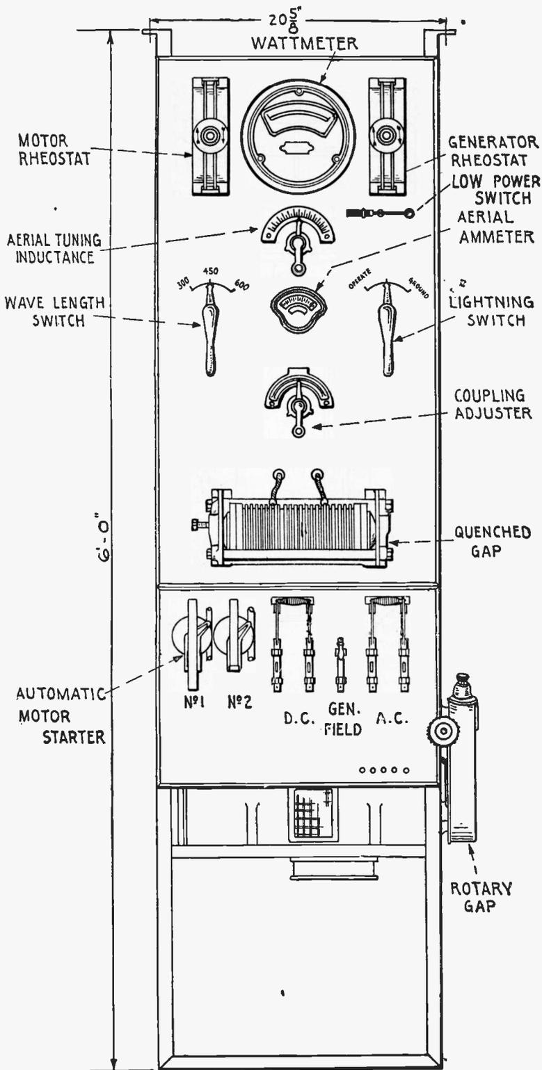
Fig. 257—Front View of the Marconi 1/4 K. W. 500 Cycle Transmitter.
