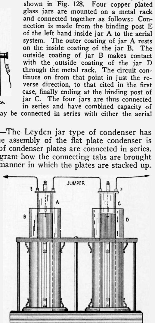
Fig. 128—Short Wave Condenser American Marconi Company.
