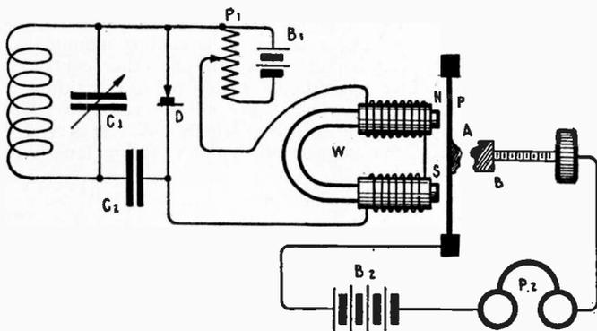
Fig. 196—Diagram Showing the Principle of Microphonic Relay.
