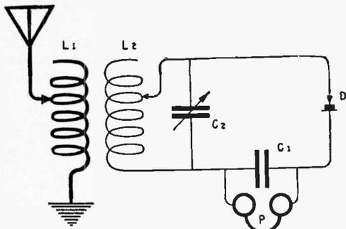
Fig. 150.—Fundamental Diagram of the Inductively Coupled Receiver.
