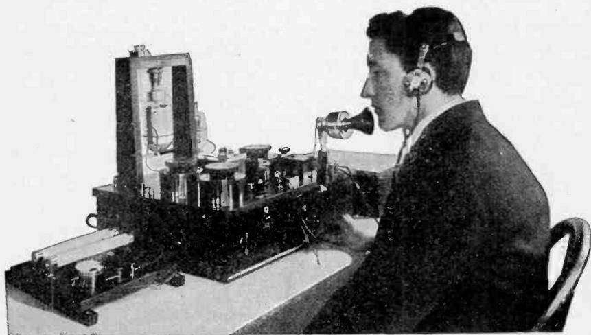
Fig. 325B—Oscillating Valve Wireless Telephone Set Developed by Marconi's Wireless Telegraph Co., Ltd.
