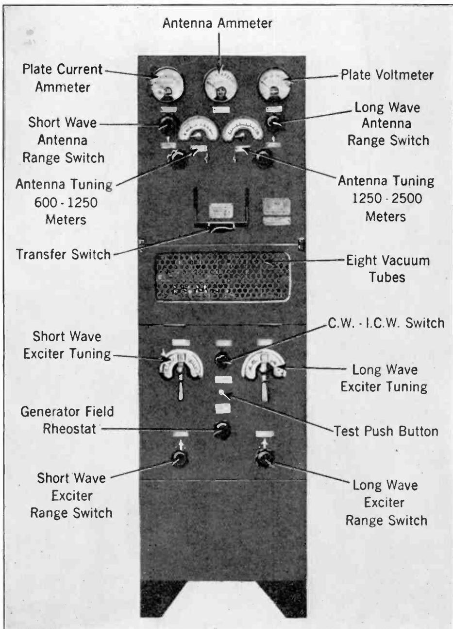
Front panel view of the ET-3626B Radiomarine Corporation of America commercial tube transmitter. *Frontispiece.*
