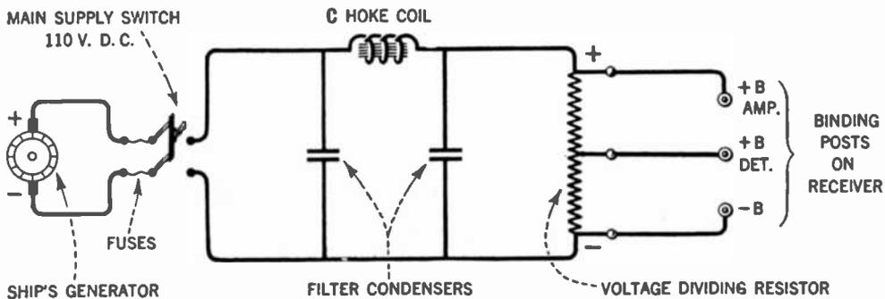
FIG. 60.—Diagram showing how the plate voltage for receiving tubes may be obtained from the d.c. ship supply.
