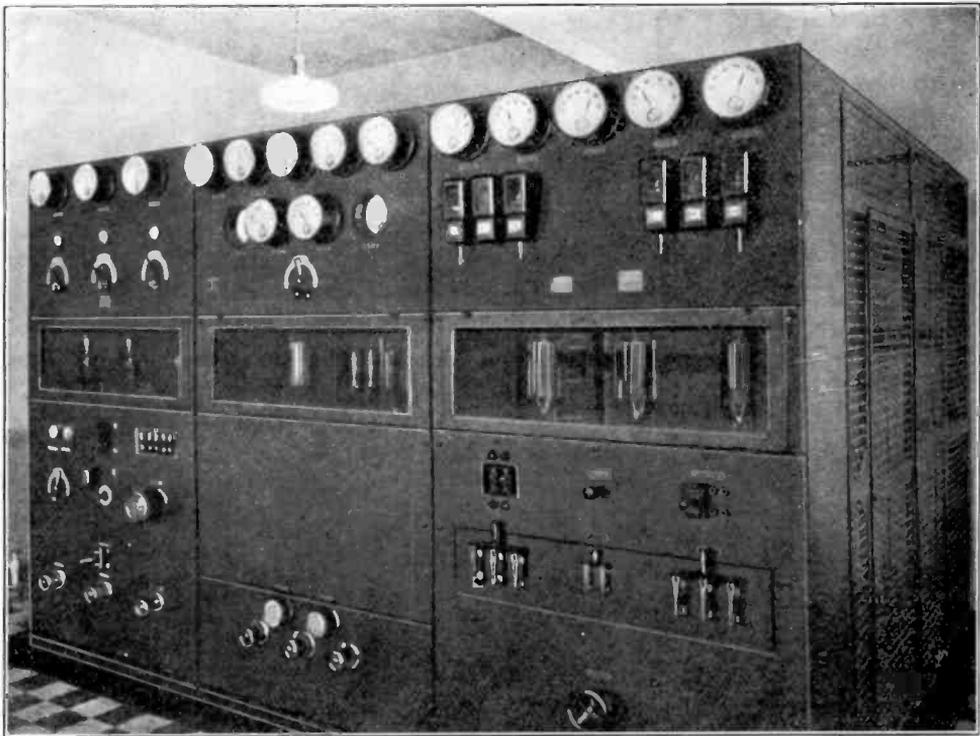
FIG. 34.—The main unit of the 1005-A 5-kw. broadcast transmitter equipment manufactured by the RCA.
