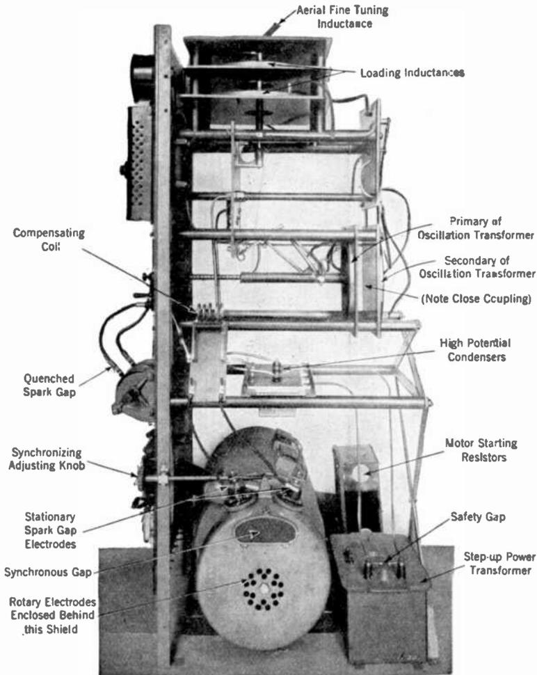
FIG. 11.—The 2-kw. spark transmitter, type P-8. Observe the close mechanical relationship between the primary and secondary coils of the oscillation transformer. This adjustment is known as “close” or “tight” coupling.
