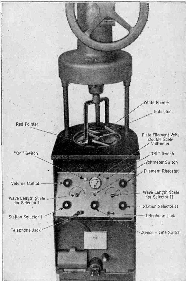
FIG. 71.—The RCA radio direction finder showing receiver controls and indicator. The rotating element with the red and white pointer is clearly shown mounted directly over the compass scale.
