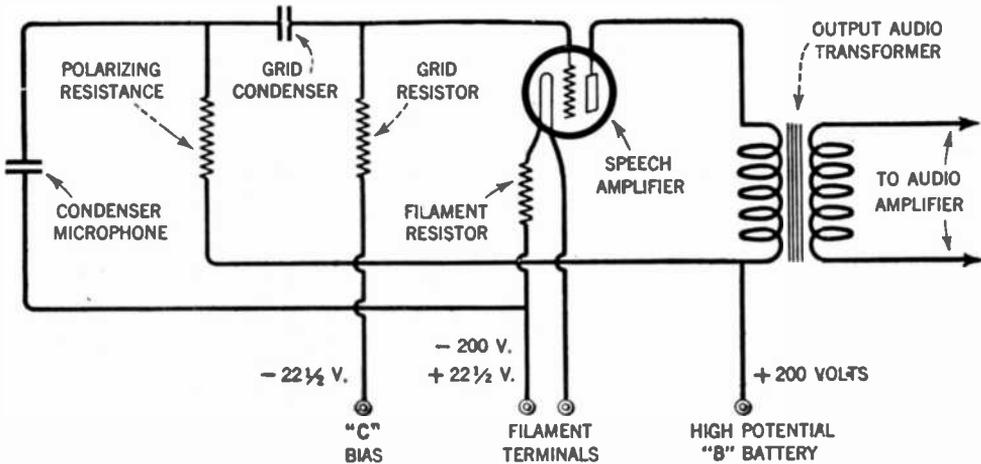
FIG. 40.—Showing how the electrostatic field is set up in the condenser type microphone by connecting a high potential "B" battery across its plates through a polarizing resistance.
