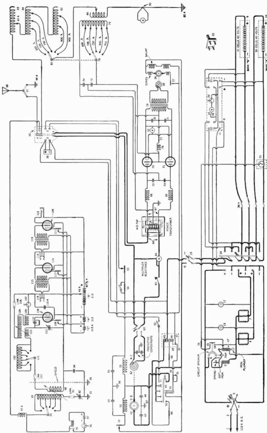
Fig. 1.—Diagram of a complete shipboard radio installation consisting of the ET-3628 ACCW 500-watt transmitter, IP-501 receiver, and emergency (battery) source of power.
