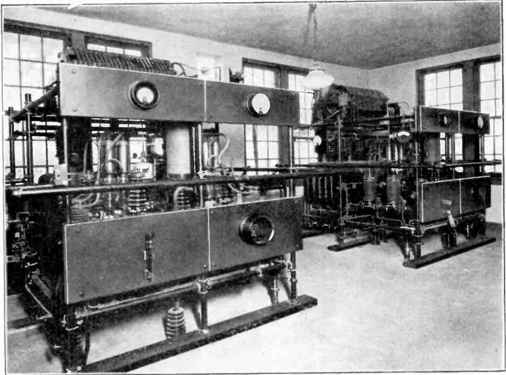
FIG. 47.—The oscillators at WJZ.
