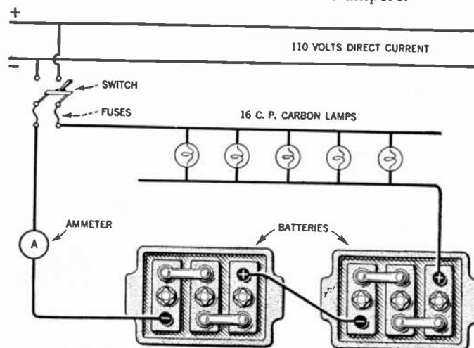
FIG. 83.—Another method of charging "A" batteries. Five 16-candle-power carbon lamps in parallel are connected in series with the 110-volt line to regulate the charging current.
