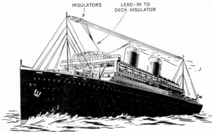
FIG. 43.—The inverted "L" type antenna. If the antenna lead-in is connected at the center of the antenna as shown by the dotted lines, the antenna then becomes the "T" type.
