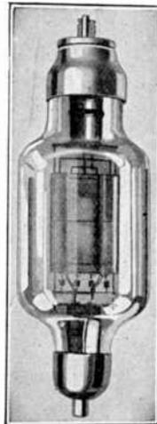
FIG. 49.—A 1000-watt transmitting tube.
