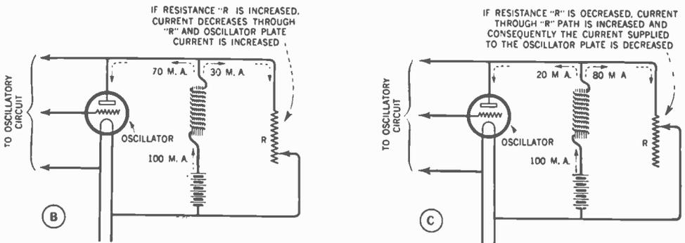
Fig. 25.—Diagrammatic explanations of the Heising (constant current) system of modulation.
