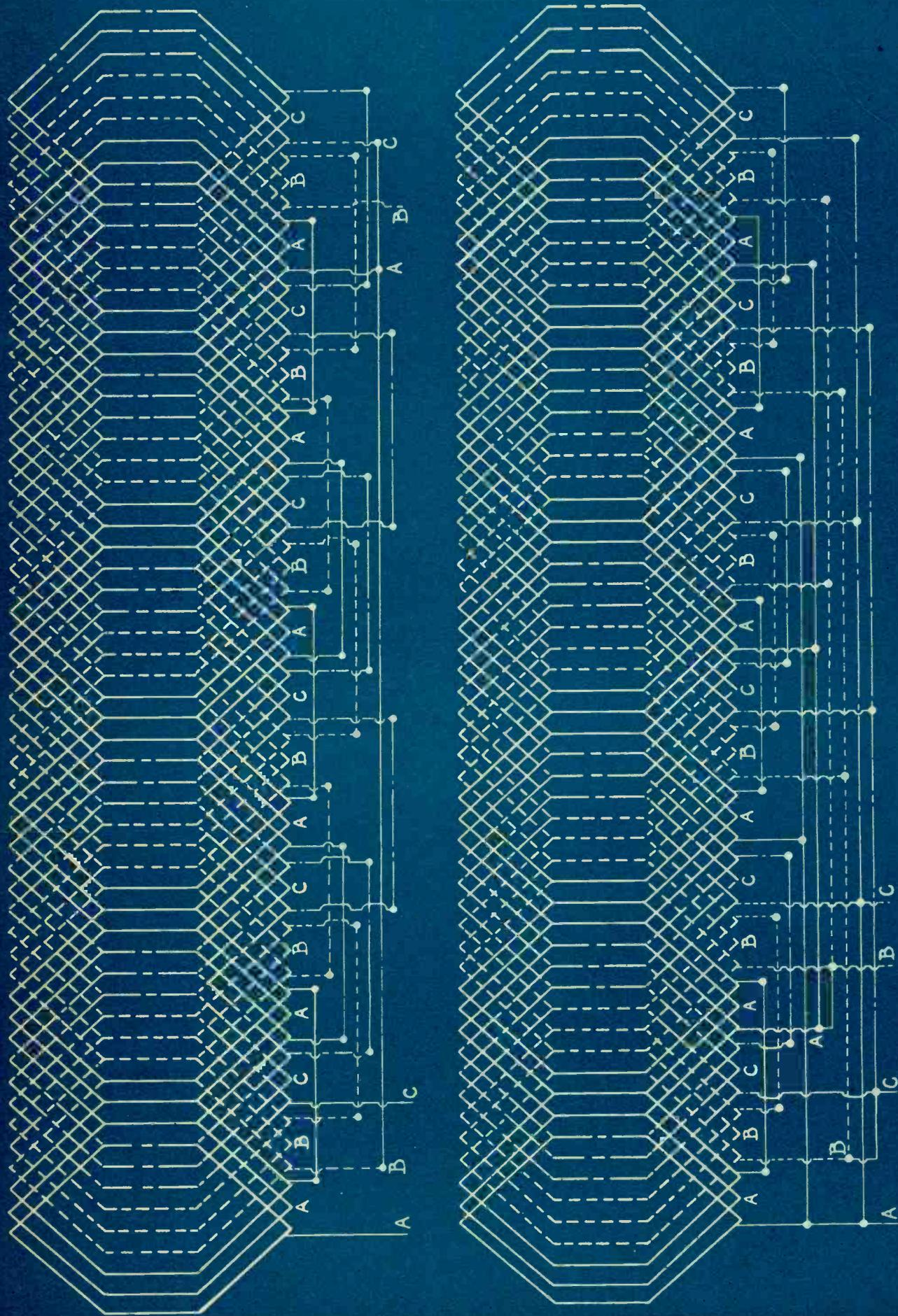
PLATE II (Top). DEVELOPMENT OF A SIX-POLE, THREE-PHASE, SERIES-STAR-CONNECTED ARMATURE WINDING
