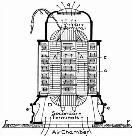
Fig. 265. Section of Air-Blast Transformer Showing Circulating Currents
