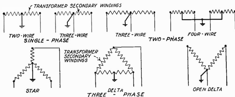
Fig. 276. Theoretical Diagrams of Secondary Ground Connections
