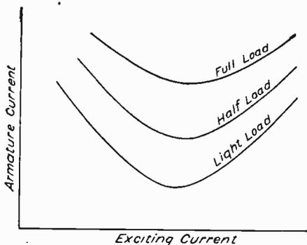
Fig. 188. Curve Showing Variation of Armature Current with Field Excitation
