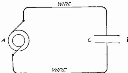
Fig. 12. Alternating Circuit Containing Condenser
