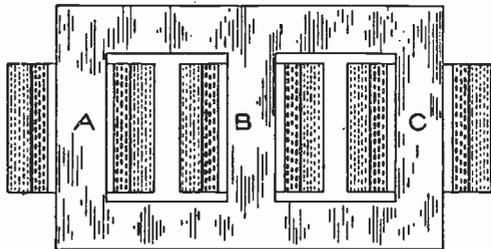
Fig. 216. Three Transformers for Three-Phase System with Common Magnetic Return Circuit
