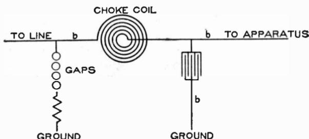
Fig. 409. Combination of Condenser and Choke Coil as Lightning Arrester
