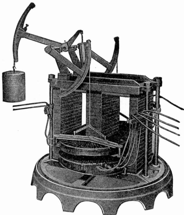
Fig. 269. Mechanism of General Electric Two-Coil Constant-Current Transformer
