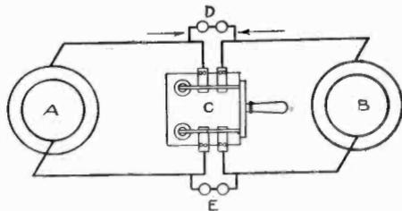
Fig. 410. Wiring Diagram Showing Method of Determining Coincidence in Phase and Frequency of Two Generators
