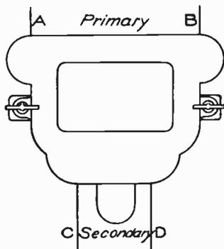
Fig. 281. Transformer Connected for Polarity Test
