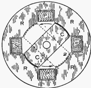
Fig. 392. Diagram of Magnetic Voltage Regulator
