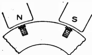
Fig. 73. Concentrated or Uni-coil Winding
