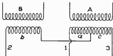
Fig. 224. Complete Connections of Scott Transformer
