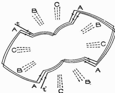
Fig. 328. Complete Connections for Four Poles of One Circuit of Three-Phase Induction Motor
