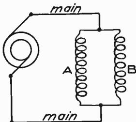
Fig. 39. Coils in Parallel with an Alternator
