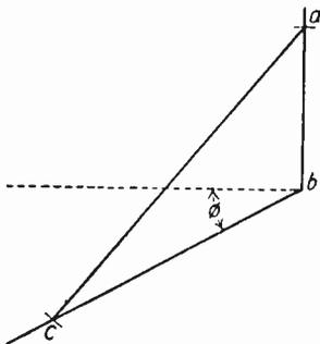
Fig. 168. Terminal Voltage without Reactance
