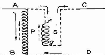
Fig. 209. Connections for an Auto Step-Down Transformer
