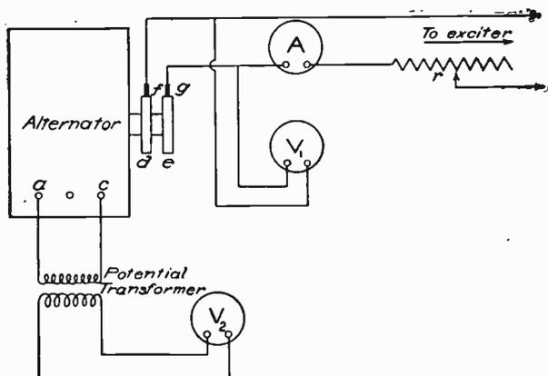
Fig. 160. Diagram of Connections for Saturation Curve Test of Alternator
