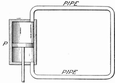
Fig. 11. Water Analogy for an Alternating Circuit
