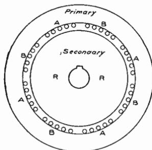
Fig. 321. Diagram of Four-Pole Two-Phase Induction Motor
