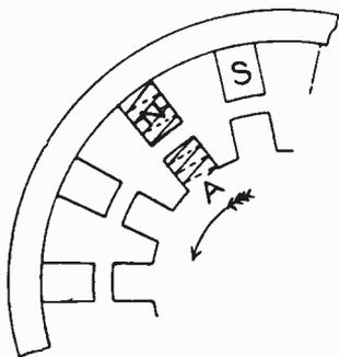
Fig. 80. Portion of Armature and Field Coil for Single-Phase Alternator
