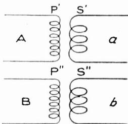
Fig. 210. Transformer Connections on a Two-Phase System
