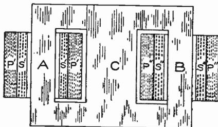
Fig. 215. Two Transformers for Two-Phase System with Common Magnetic Return Circuit
