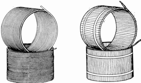
Fig. 237. Specimen Coils for General Electric Core-Type Transformer
