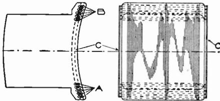
Fig. 301. Diagram Showing Copper Dampers in Place in Field Poles
