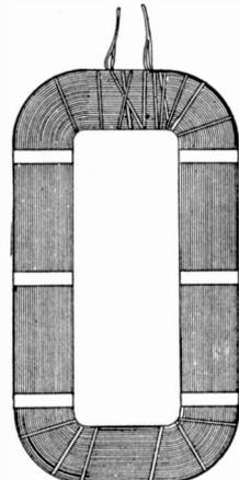
Fig. 253. Method of Binding up Pancake Strip Coils
