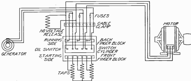
Fig. 340. Electrical Connections for Three-Phase Starting Compensator
