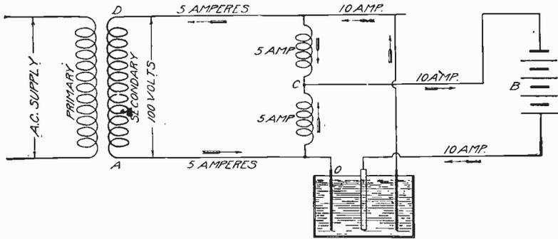
Fig. 283. Diagram of Connections for Aluminum Valve Rectifier
