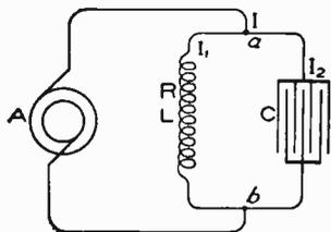
Fig. 59. Circuit Showing Condenser and Inductance in Parallel
