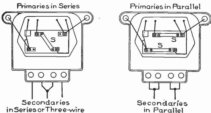
Fig. 233. Plan of Transformer Showing Strap Connections for Arranging Primaries in Series or Parallel
