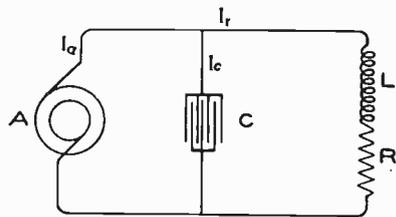
Fig. 62. Diagram of Condenser Compensating for Lagging Current
