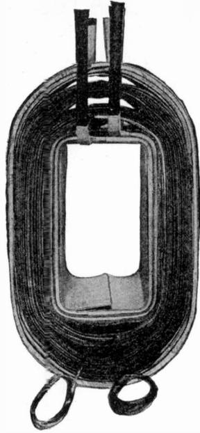
Fig. 241. Method of Assembling Coils Showing Oil Ducts
