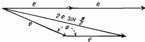
Fig. 364. Vector Diagram Showing Effect of Chord Winding
