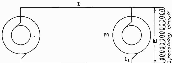
Fig. 189. Diagram Showing Synchronous Motor Used as a Condenser
