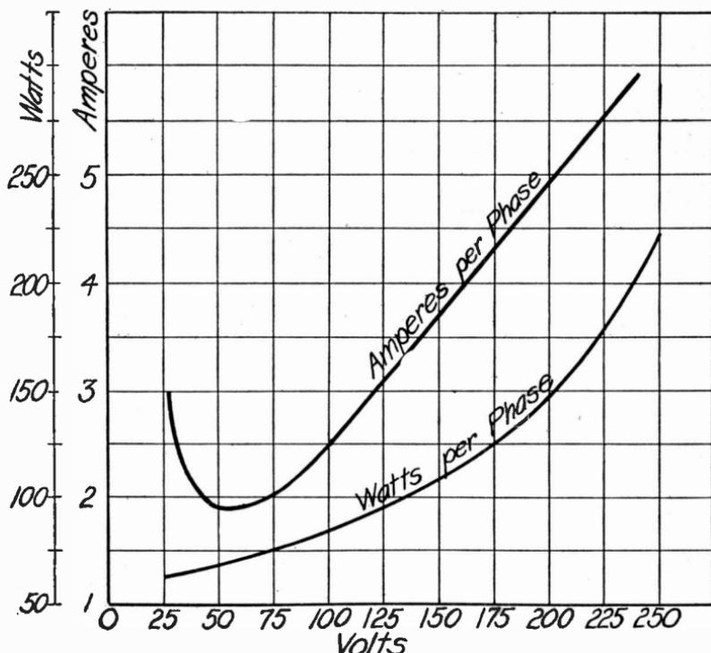
Fig. 356. Running Saturation Curves
