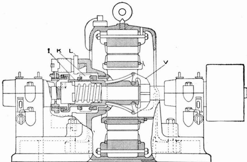
Fig. 251. Part Section of Wagner Single-Phase Induction Motor
