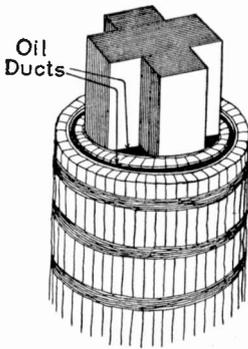
Fig. 236. Coils and Core of General Electric Transformer Showing Oil Ducts
