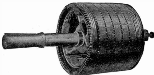
Fig. 335. Rotor with Definite or Polar Winding with Starting Resistance Inside Core
