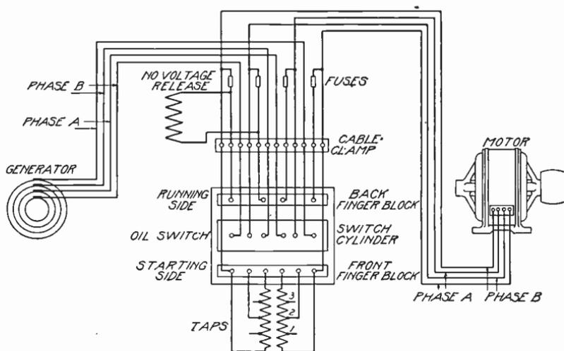
Fig. 341. Diagram of Electrical Connections for a Two-Phase Compensator for Starting Two-Phase Induction Motors
