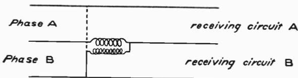
Fig. 104. Diagram of Power Connection for Three-Wire Two-Phase Induction Motor
