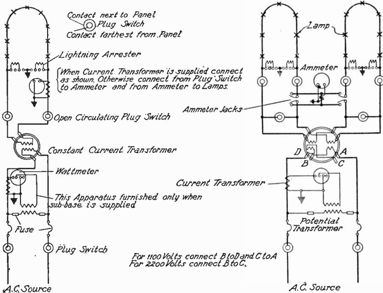
Fig. 271. Connections for Constant-Current Transformer for 5, 35, 50, 75, and 100 Lights
