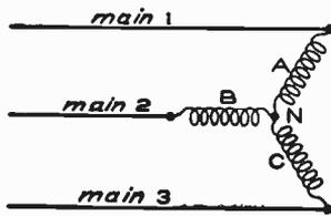
Fig. 102. "Y" Method of Connecting Receiving Circuits
