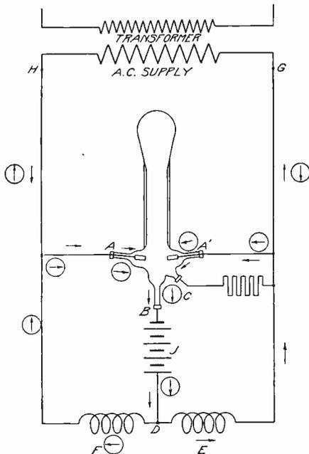
Fig. 285. Connections for Mercury-Vapor Arc Rectifier
