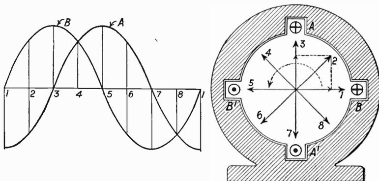
Fig. 183. Two-Phase Two-Pole Synchronous Motor and Magnetic Field Produced by Polyphase Current
