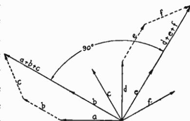
Fig. 363. Vector Diagram of Voltages Connected for Two-Phase Operation
