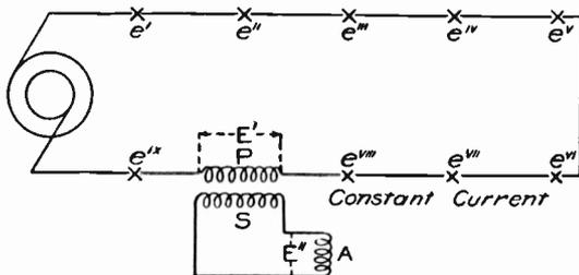
Fig. 207. Diagram of Connections for Transformer in Series with a Number of Lamps
