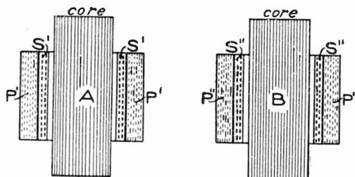
Fig. 214. Diagrammatic View of Two Separate Transformers for Step-Up or Step-Down Transformation—Two-Phase System
