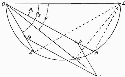
Fig. 67. Vector Diagram of Current Conditions for Fig. 66
