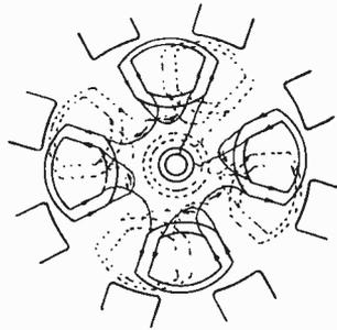
Fig. 117. Two-Phase Armature Winding, Two Slots Per Pole Per Phase
