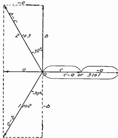
Fig. 222. Vector Diagram of E.M.F. Relations in Scott Transformer
