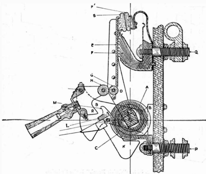
Fig. 381. Half Section of Over-Load Type of Circuit Breaker—Closed
