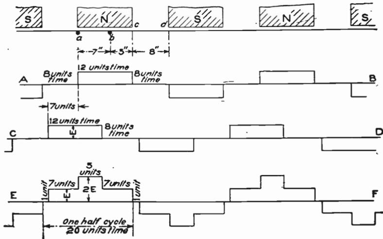
Fig. 79. Development and E. M. F. Curve of Four-Pole Alternator with Two Conductors for Each Field Pole
