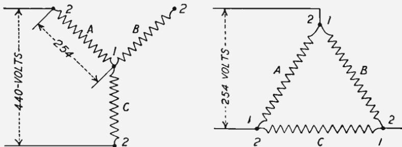
Fig. 360. Typical Delta to Star Connections
