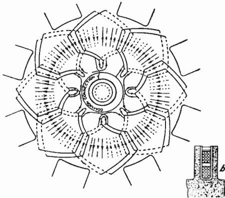
Fig. 121. Three-Phase Coil Winding, Two Slots Per Pole Per Phase
