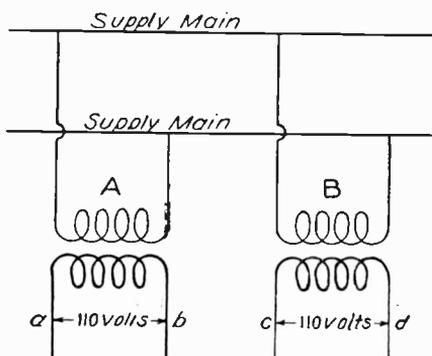
Fig. 282. Wiring Diagram for Transformer Polarity Test
