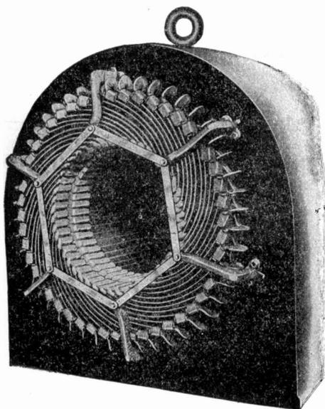
Fig. 151. Method of Bracing Armature Coils
