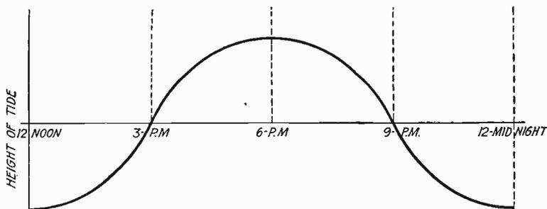
Fig. 2. Curve Showing Height of Tide
