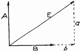
Fig. 218. Vector Diagram of E.M.F. Relations for Fig. 217
