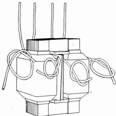
Fig. 227. Core-Type of Transformer
