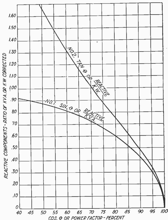
Fig. 193. Ratio of Reactive Power to True Power
