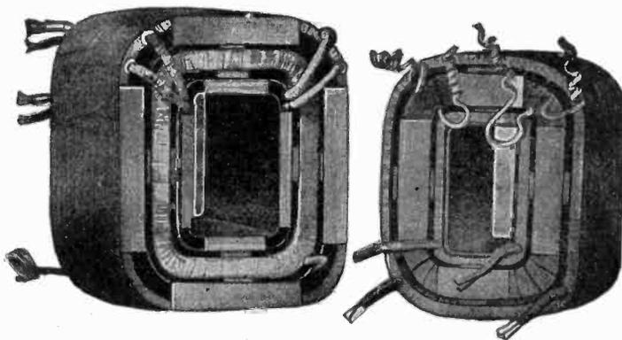
Fig. 247. Assembled Coils for Westinghouse Transformer
