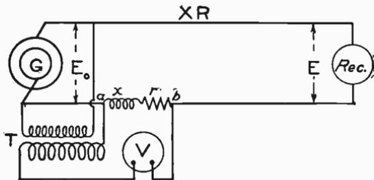
Fig. 397. Diagram of Connections for Voltmeter Compensator
