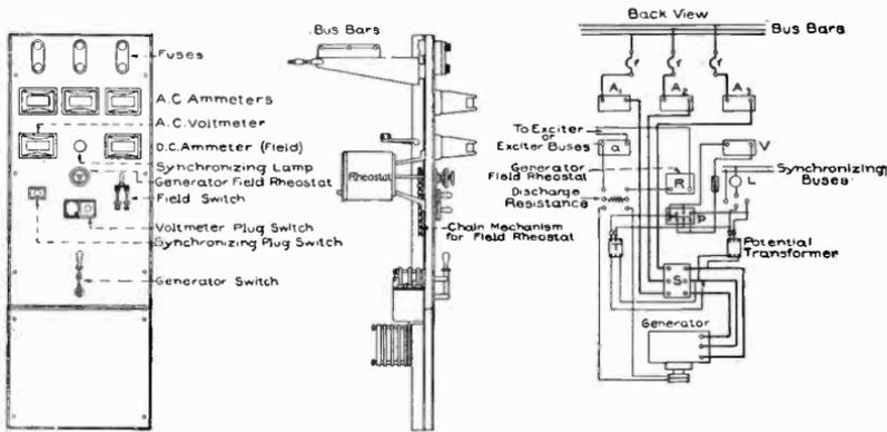
Fig. 373. Front and Side View and Complete Wiring Diagram for a Three-Phase Generator Operated in Parallel with Other Three-Phase Machines
