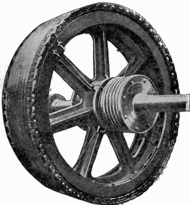
Fig. 112. Completed Armature with Strap Winding, Four Slots Per Phase
