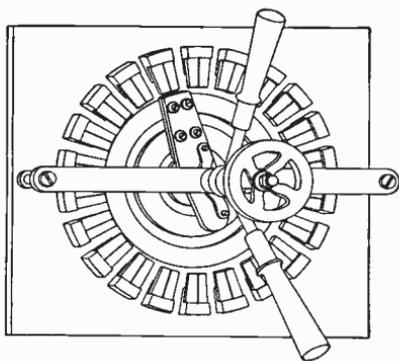
Fig. 389. Dial of Stillwell Single-Phase Voltage Regulator
