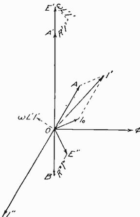
Fig. 197. Clock Diagram Showing Effects of Coil Resistance and Magnetic Leakage
