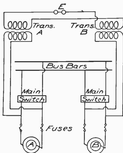
Fig. 411. Wiring Diagram Showing Method of Determining Phase Relation by Synchronizer
