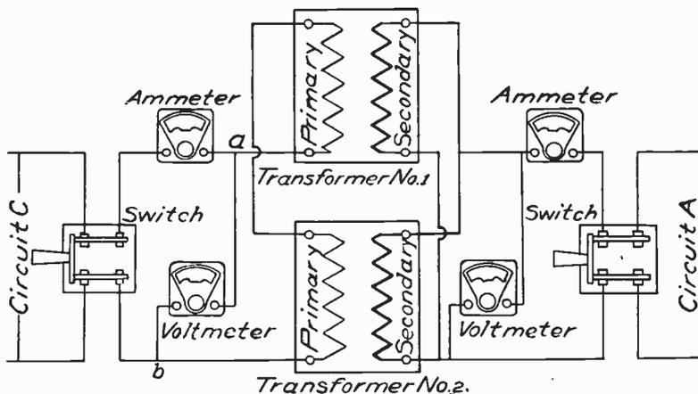
Fig. 278. Connections for Transformer Heat Test
