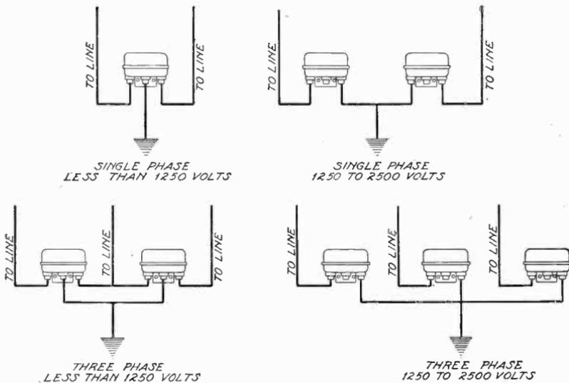
Fig. 405. Lightning Arrester Connections for Single-Phase and Three-Phase Circuits
