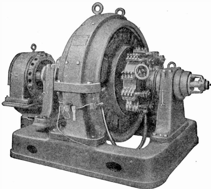
Fig. 298. Westinghouse Rotary Converter Equipped with Separate Starting Motor on Same Shaft
