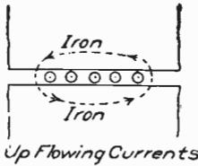
Fig. 323. Magnetic Action of Conductors Carrying Currents between Iron Poles
