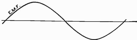
Fig. 17. Typical E. M. F. Curve for Alternator —
