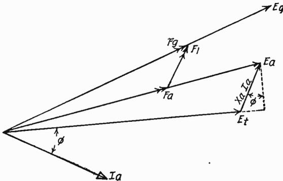
Fig. 173. Potier Construction Diagram
