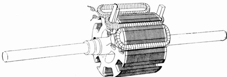
Fig. 125. Westinghouse Single-Phase Armature with Coils in Place
