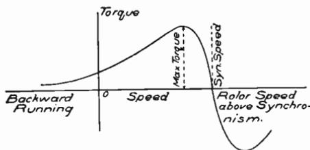
Fig. 329. Graphical Relation of Torque and Speed of Induction Motor
