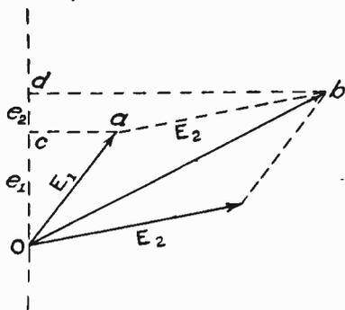
Fig. 31. Diagram Showing Addition of Harmonic E. M. F.s
