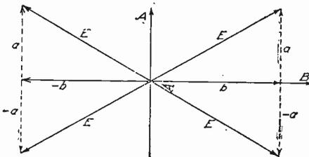
Fig. 219. Vector Diagram of E.M.F. Relations for  $E$  in any Quadrant
