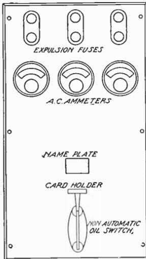
Fig. 374. Front Elevation of Typical Three-Phase Feeder Panel
