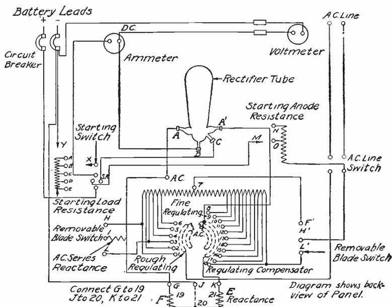
Fig. 287 Diagrammatic Views of Front, Back, and Side of Rectifier Equipment
