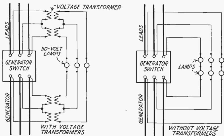
Fig. 412. Connections for Phasing Out Three-Phase Circuits
