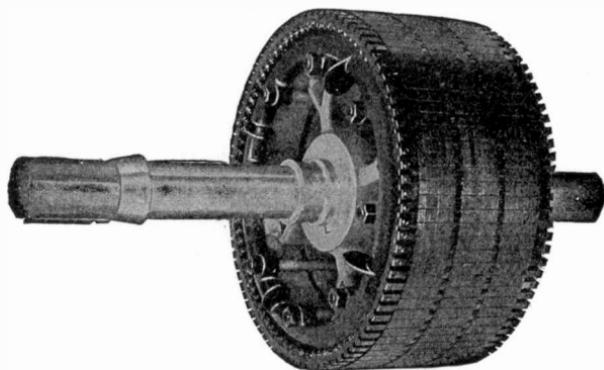
Fig. 334. Squirrel-Cage Type of Rotor
