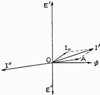
Fig. 196. Clock Diagram for Transformer with Load—highly Inductive Receiving Circuit
