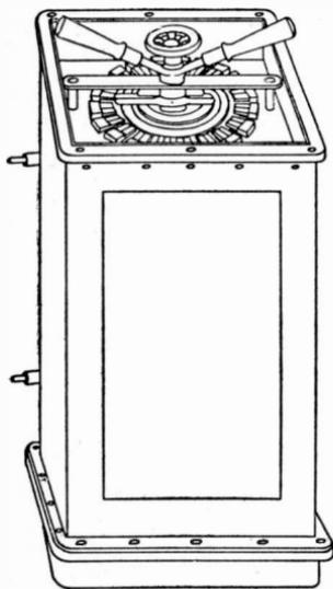
Fig. 388. Stillwell Single-Phase Voltage Regulator Complete
