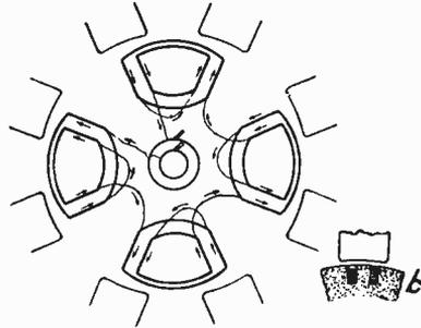
Fig. 115. Single-Phase Armature Winding, Two Slots Per Pole
