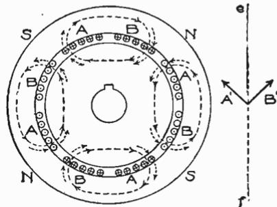
Fig. 326. Magnetic Effect of Alternating Current  $\frac{1}{4}$  of a Cycle Later than in Fig. 325
