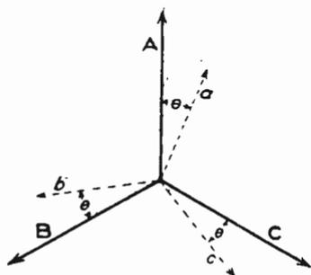
Fig. 94. Clock Diagram of Three-Phase E. M. F.'s and Currents
