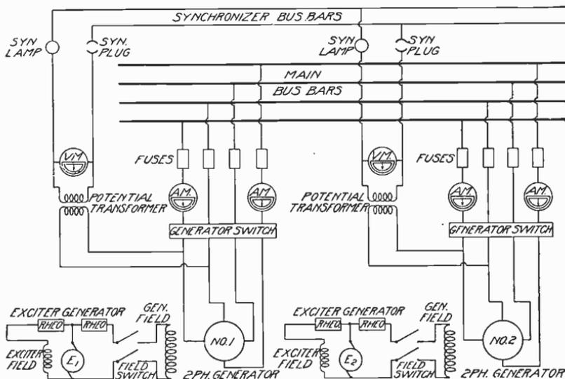
Fig. 372. Complete Wiring Diagram for Two Two-Phase Generators Running in Parallel
