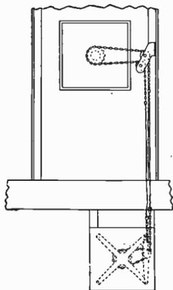
Fig. 335. Diagram Showing Switchboard Control for Large Rheostats
