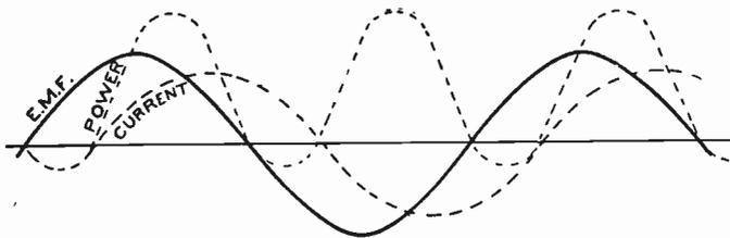
Fig. 19. E. M. F., Current, and Power Curves for an Alternator in a Circuit Containing Inductance
