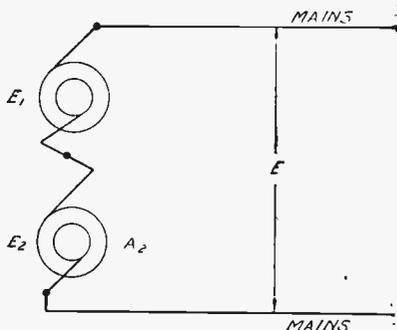
Fig. 6. Two Alternators in Series
