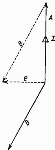
Fig. 187. Effect of Normal Excitation, Power-Factor Normal
