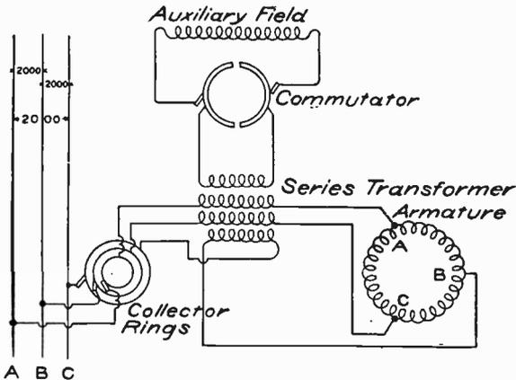
Fig. 85. Three-Phase Alternator Diagram with Composite Field Excitation with Balanced Receiving Circuits
