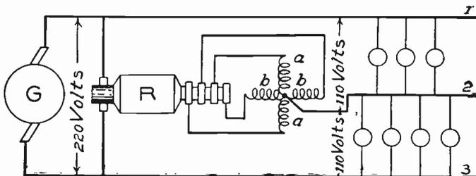
Fig. 305. Connections for D. C. Generator on Edison Three-Wire System with Two-Phase Rotary Converter Connected as a Balancer
