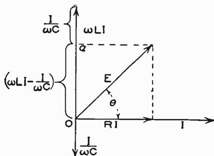
Fig. 47. Complete Diagram of Conditions in Fig. 45
