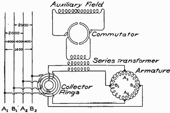
Fig. 84. Two-Phase Alternator Diagram with Composite Field Excitation with Balanced Receiving Circuits
