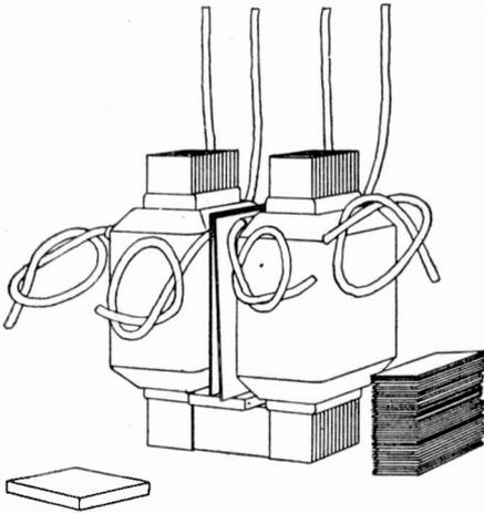
Fig. 230. Both Transformer Coils in Position, Showing Laminated Strips Which Form the Upper Yoke of Core
