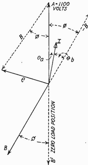
Fig. 179. Calculation of  $\theta_b$
