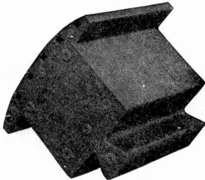
Fig. 139. One of the Field Poles Which Fits into the Core of Fig. 138
