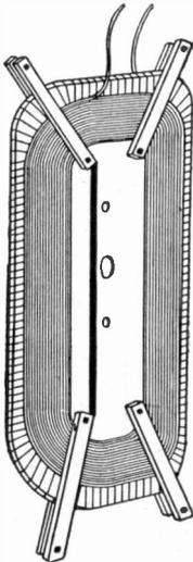
Fig. 250. Pancake Coil for Shell-Type Transformer
