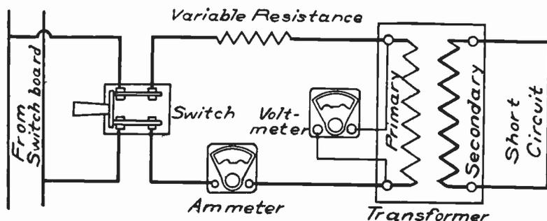
Fig. 280. Diagram of Connections for Making Transformer Impedance Test
