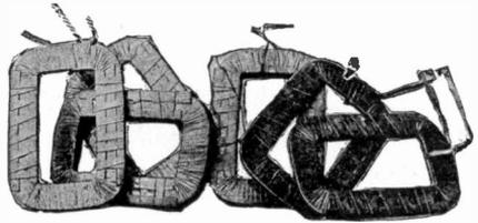
Fig. 256. Sample Coils for Fort Wayne Transformer
