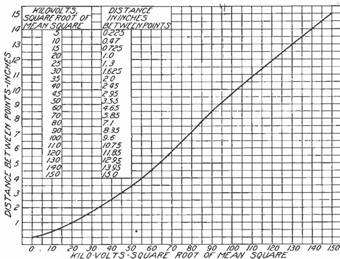
Fig. 159. Curve Showing Relation between Sparking Distance and Voltage
