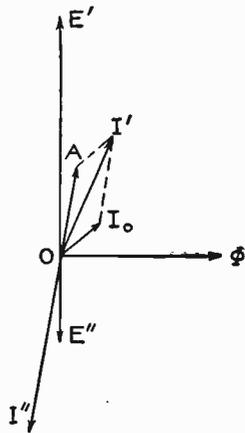
Fig. 195. Clock Diagram for Transformer with Load
