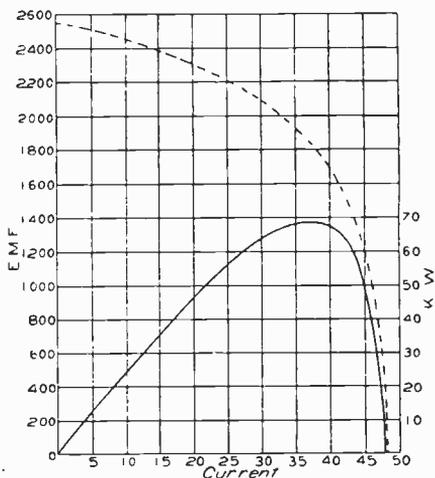
Fig. 157. Characteristic Curves of an Alternator
