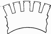
Fig. 110. Portion of Stamping for Twelve-Pole Uni-Tooth Three-Phase Alternator
