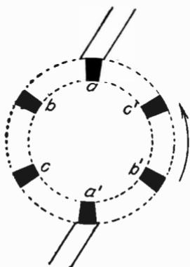
Fig. 292. Brush and Commutator Diagram for Six-Ring Converter
