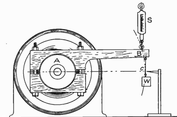
Fig. 352. Prony Brake Arrangement for Testing Starting Torque
