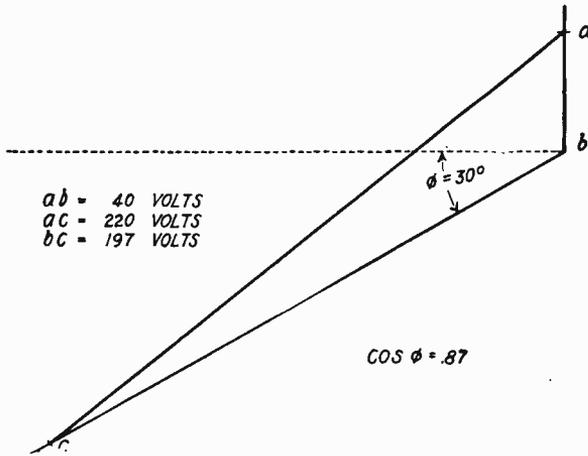
Fig. 172. Potier Method for Determining Terminal Voltage
