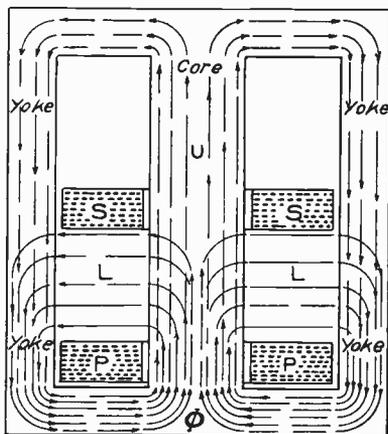
Fig. 268. Magnetic Circuit in Constant-Current Transformer
