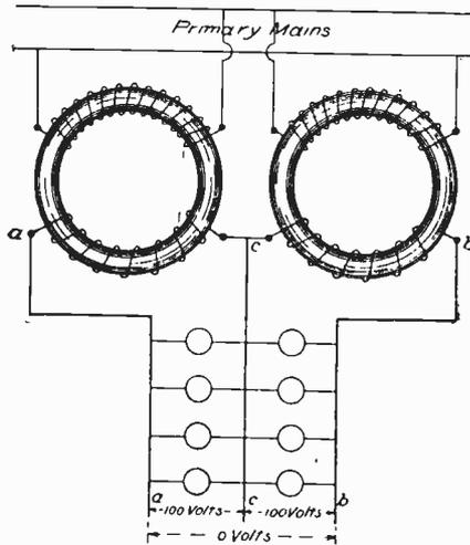
Fig. 204. Improper Transformer Connections to a Three-Wire System
