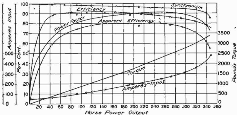
Fig. 355. Performance Curves of a 175-H. P. Three-Phase Induction Motor
