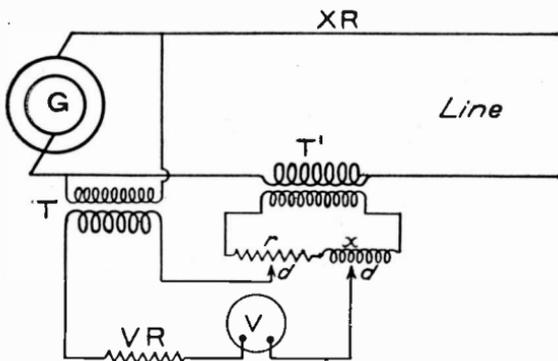
Fig. 400. Wiring Diagram for Voltmeter Compensator as Used in Practice in High Voltage Circuits
