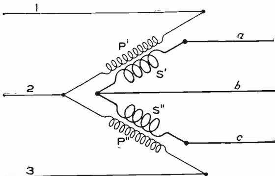
Fig. 213. System Shown in Fig. 212 with One Transformer Removed Giving V-Connections
