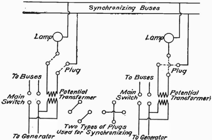
Fig. 370. Complete Connections for Synchronizing Device for Two Single-Phase Machines
