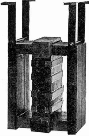
Fig. 240. Assembled Core Showing Method of Clamping
