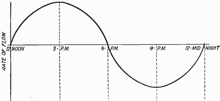
Fig. 1. Curve Showing Rate of Flow of Tide
