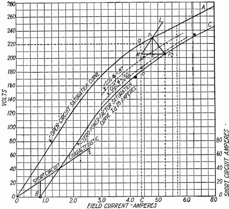
Fig. 170. Saturation and Short Circuit Characteristics
