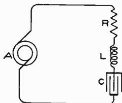
Fig. 45. Alternating Circuit Containing Resistance, Inductance, and Capacity
