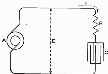
Fig. 53. Circuit Containing Resistance and Capacity
