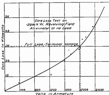
Fig. 174. No-Load Core-Loss Curve for 2,000-Kw. Alternator
