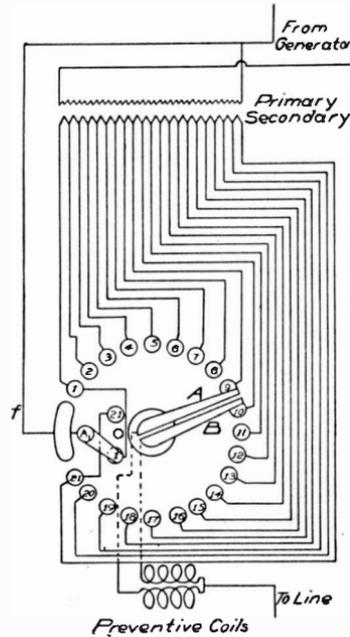
Fig. 390. Complete Internal Connections for Stillwell Voltage Regulator
