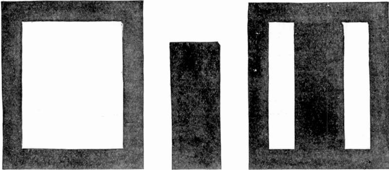
Fig. 239. Core Punchings for Crocker-Wheeler "Remek-Type" Transformer
