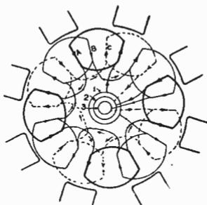
Fig. 119. Three-Phase Concentrated Winding  $\Delta$ -Connected
