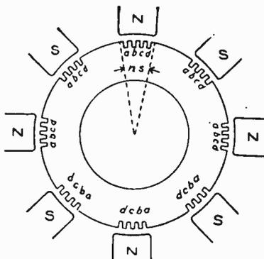
Fig. 75. Armature Winding Diagram, Four Slots per Pole
