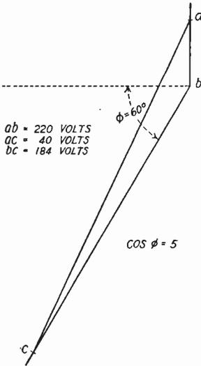
Fig. 171. Application of Terminal Voltage Rule
