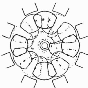
Fig. 118. Three-Phase Concentrated Winding  $Y$ -Connected
