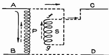
Fig. 208. Connections for Auto Step-Up Transformer
