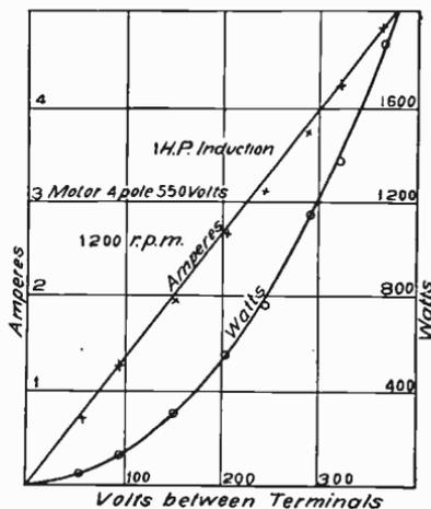
Fig. 354. Curve for Impedance Test of Induction Motor
