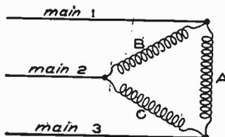
Fig. 103. " $\Delta$ " Method of Connecting Receiving Circuits
