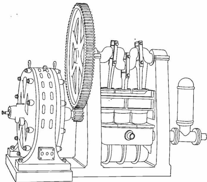
Fig. 347. Induction Motor Driving Triplex Pump
