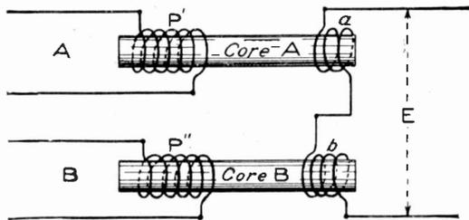
Fig. 217. Connections for Phase Transformation from Two-Phase Supply Mains
