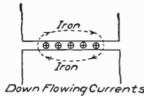
Fig. 324. Magnetic Action of Conductors Carrying Currents between Iron Poles
