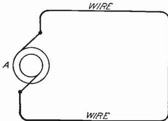
Fig. 10. Simple Alternating Circuit
