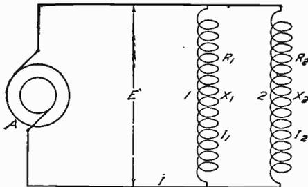
Fig. 66. Two Elements in Parallel in Alternating Circuit
