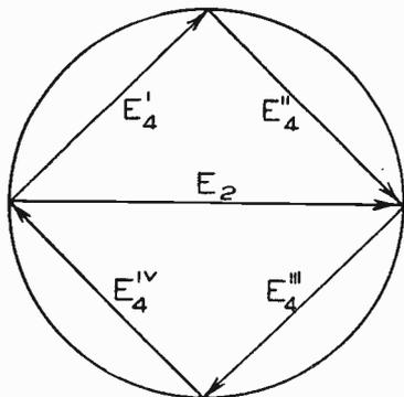
Fig. 296. E.M.F. Relations in a Four-Ring Converter
