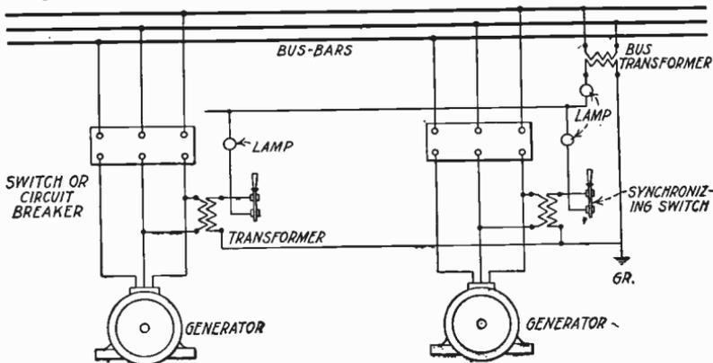
Fig. 413. Connections for Synchronizing Three-Phase Generators
