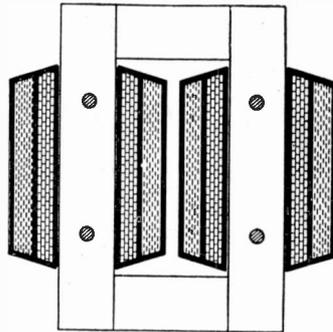
Fig. 231. Section Through Core-Type of Transformer
