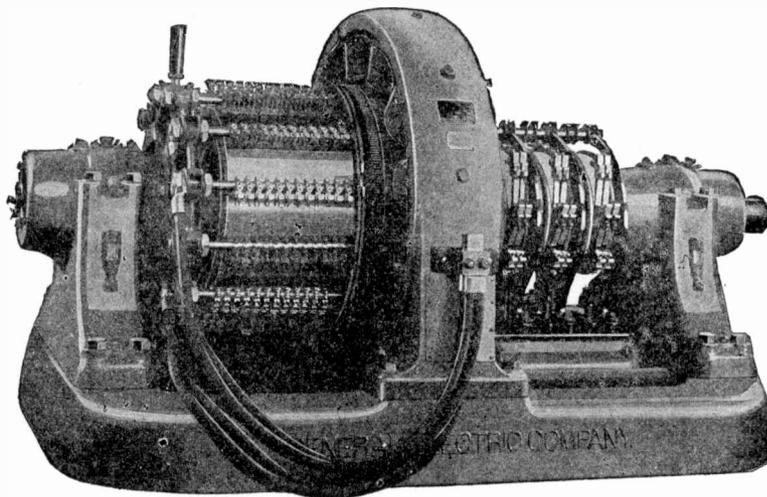
Fig. 300. General Electric Three-Phase Rotary Converter for Electric Light Service
