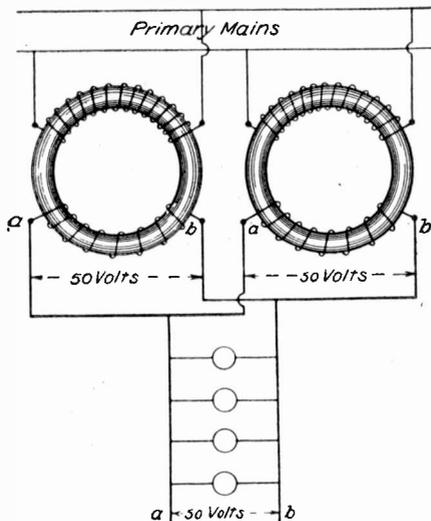
Fig. 205. Connections for "Banked" Transformers
