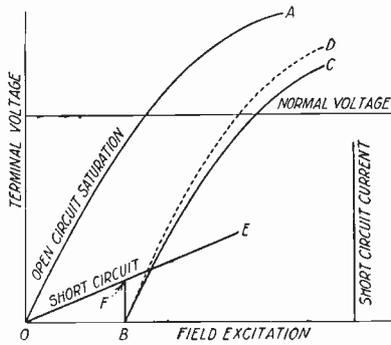
Fig. 169. Saturation Curves (Method c)
