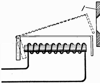
Fig. 23. Electromagnetic Visible Signal
