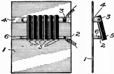
Fig. 39. Multiple-Electrode Transmitter
