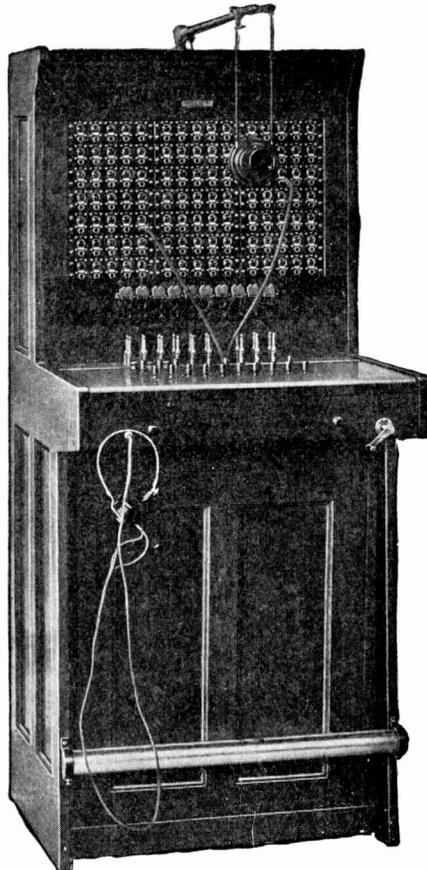
Fig. 147. Magneto Switchboard, Target Signals
