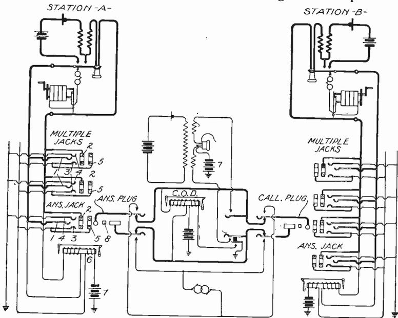
Fig. 180. Branch-Terminal Magneto Multiple Switchboard
