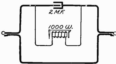
Fig. 130. Series Drop-Cord Circuit
