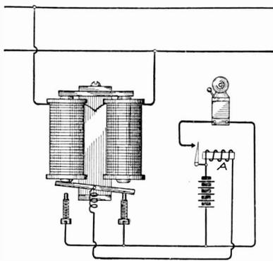
Fig. 236. Ringing Device for Composite Circuits
