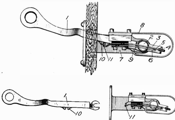
Fig. 77. Removable Lever Hook Switch
