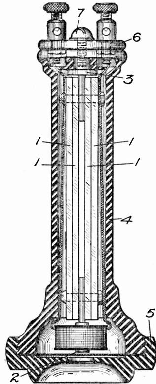
Fig. 49. Single-Pole Receiver
