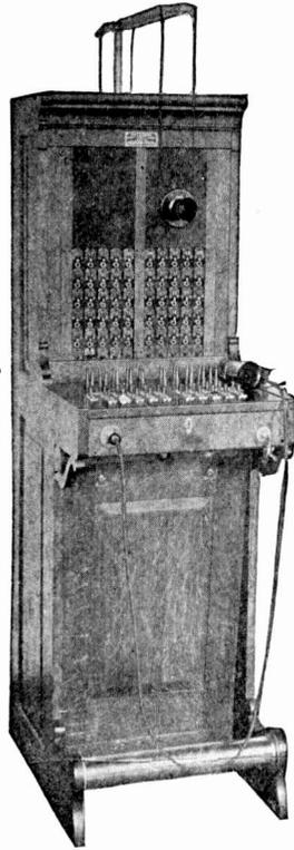
Fig. 142. Upright Magneto Switchboard
