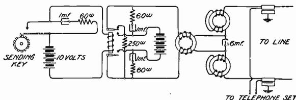
Fig. 253. Dispatcher's Station—Western Electric System
