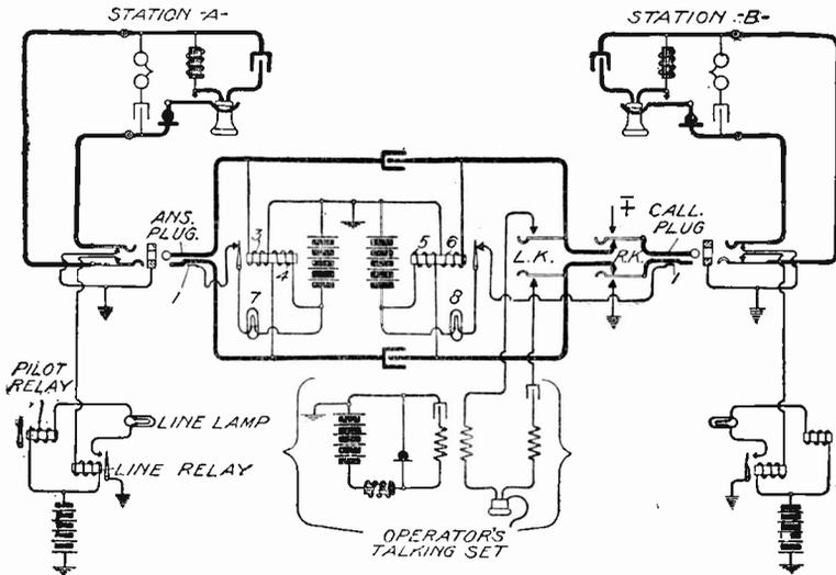
Fig. 162. Simple Common-Battery Switchboard
