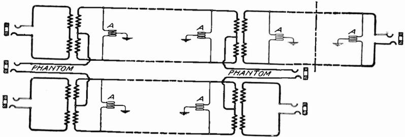
Fig. 226. Phantom from Two Physical Circuits of Unequal Length
