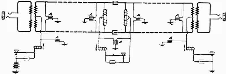
Fig. 232. Simplex Circuit with Waystation
