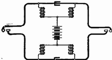
Fig. 161. Battery Supply with Impedance Coils and Condensers
