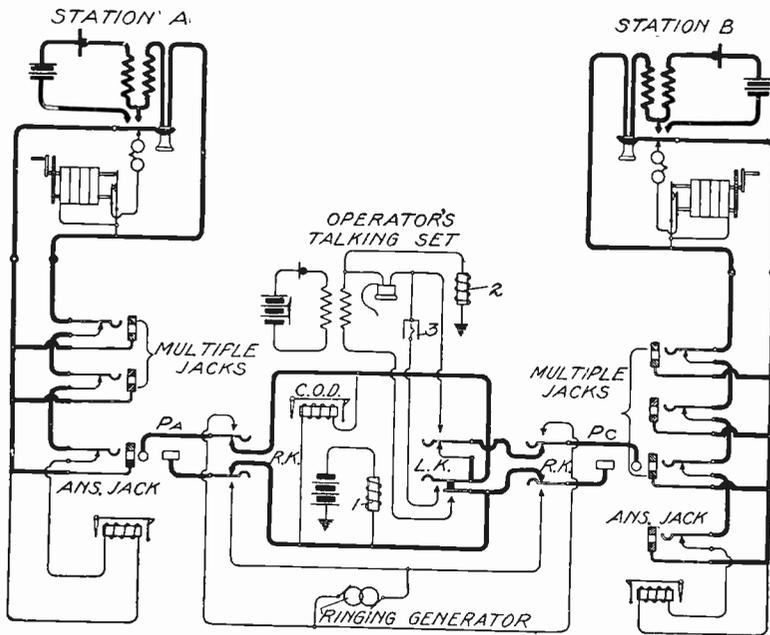
Fig. 119. Series Magneto Multiple Switchboard
