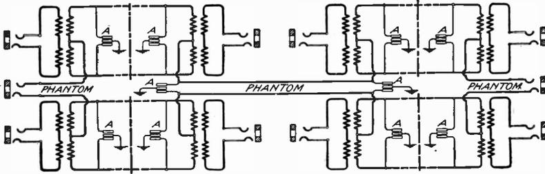
Fig. 228. Two Phantoms Joined by Physical Circuit
