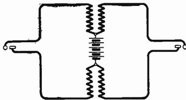
Fig. 160. Battery Supply through Repeating Coils
