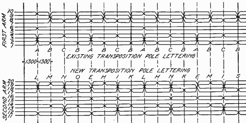
Fig. 229. Transposition of Phantom Circuits
