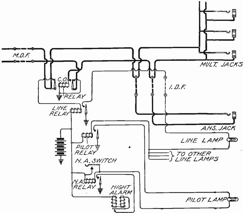
Fig. 195. Kellogg Two-Wire Line Circuit
