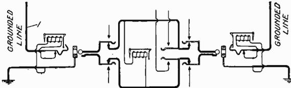
Fig. 125. Connection Between Grounded Lines
