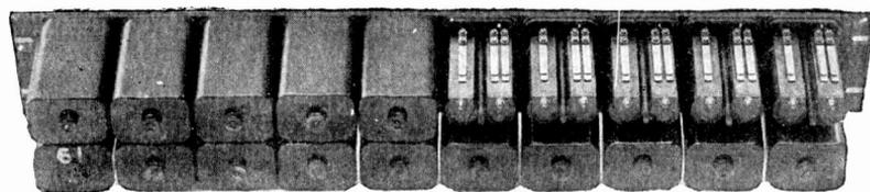
Fig. 209. Strip of Kellogg Line and Cut-Off Relays
