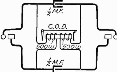
Fig. 133. Non-Ring-Through Cord Circuit
