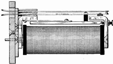
Fig. 204. Type of Cut-Off Relay
