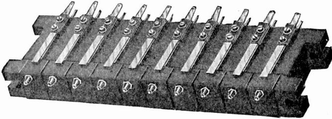
Fig. 172. Strip of Relays
