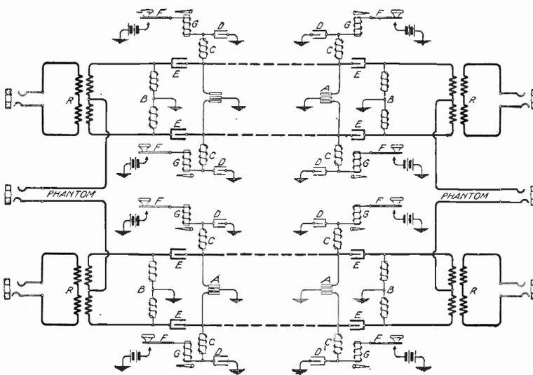
Fig. 235. Phantom of Two Composite Circuits
