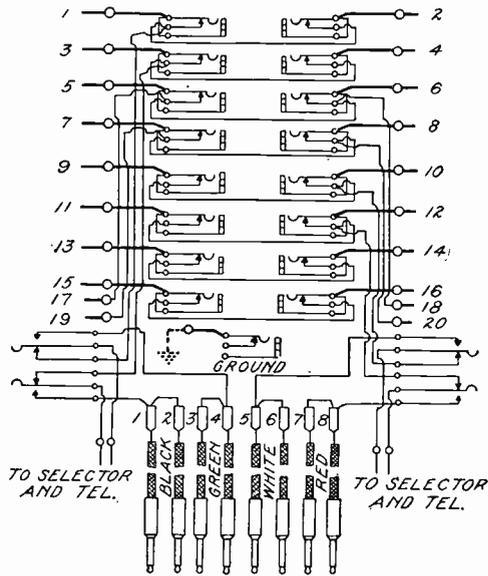
Fig. 262. Circuits of Test Board
