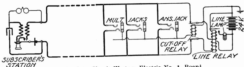
Fig. 187. Line Circuit Western Electric No. 1. Board
