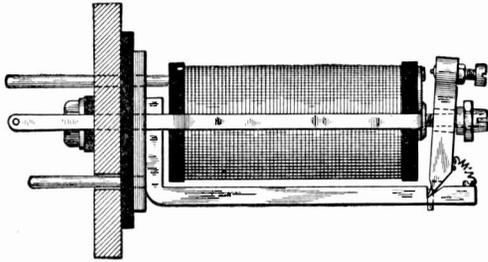
Fig. 203. Type of Line Relay
