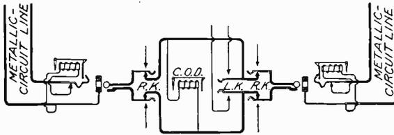
Fig. 124. Connection Between Metallic Lines
