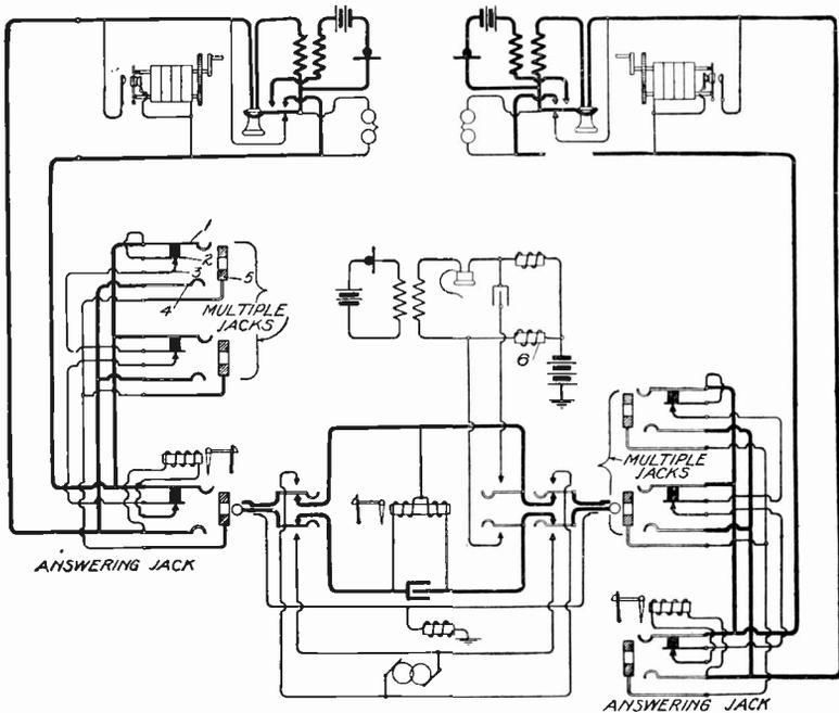
Fig. 182. Monarch Magneto Multiple Switchboard Circuits
