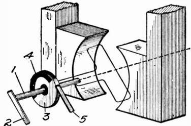
Fig. 69. Pulsating-Current Commutator
