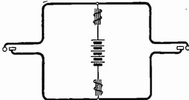
Fig. 159. Battery Supply Through Impedance Coils
