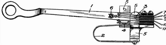
Fig. 75. Long Lever Hook Switch
