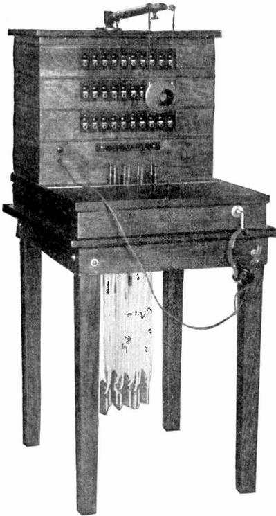
Fig. 153. Sectional Switchboard—
