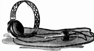
Fig. 58. Operator's Receiver and Cord
