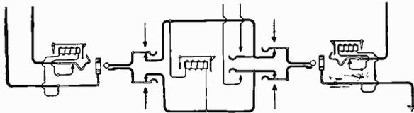
Fig. 126. Connection Between Dissimilar Lines
