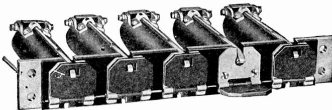
Fig. 96. Strip of Tubular Drops
