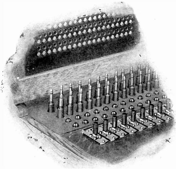
Fig. 175 Details of Lamp, Plug, and Key Mounting
