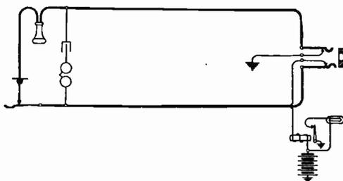
Fig. 157. Line Lamp with Relay
