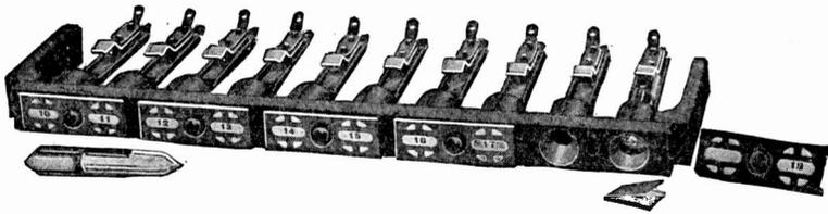
Fig. 166. Line Lamp Mounting
