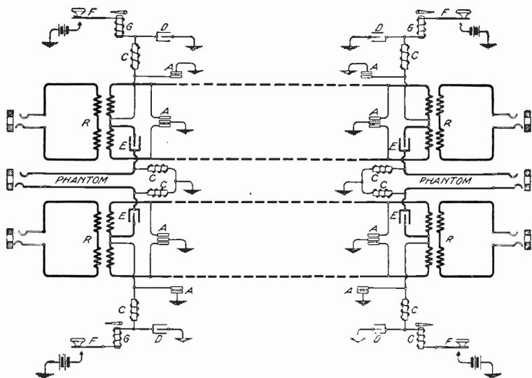
Fig. 234. Phantom of Two Simplex Circuits
