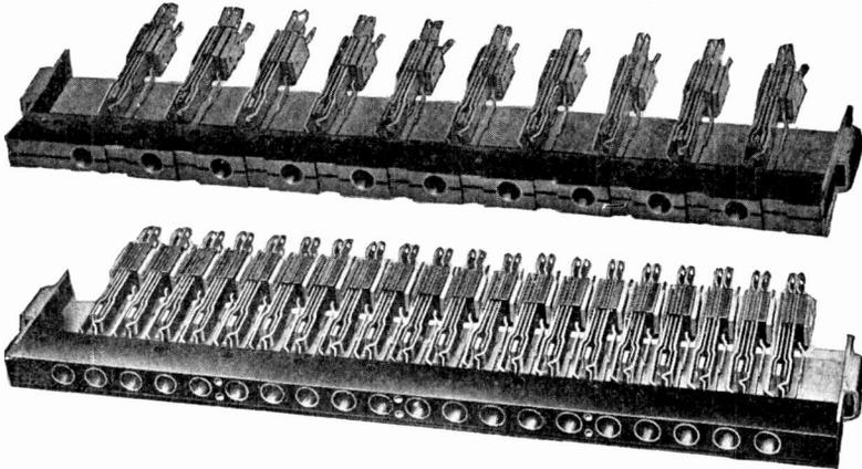
Fig. 201. Answering and Multiple Jacks for No 10 Board
