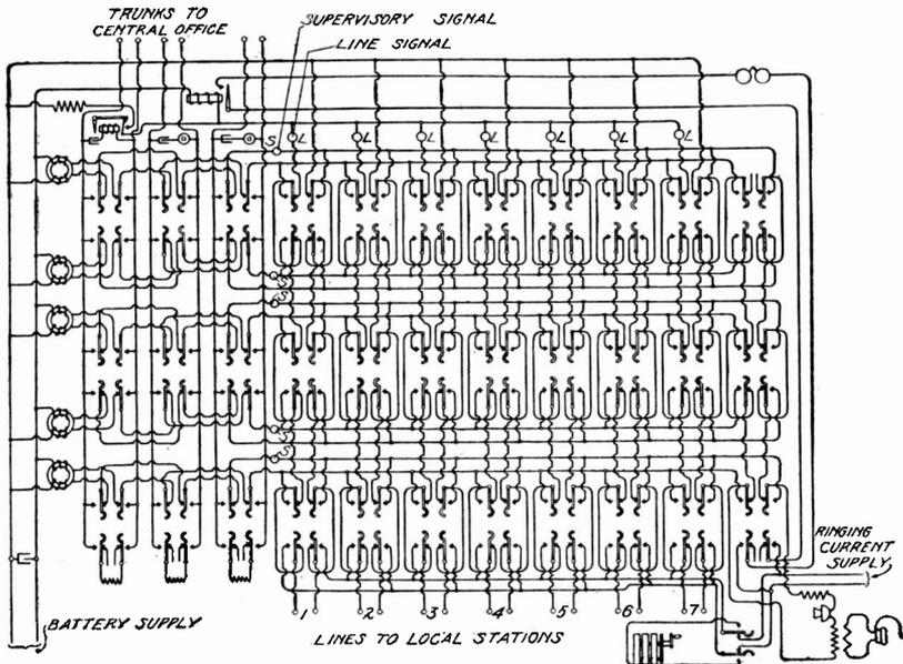
Fig. 224. Circuits, Key-Type Board
