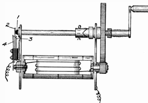
Fig. 68. Generator Cut-In Switch
