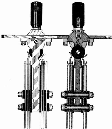
Fig. 115. Vertical-Spring Listening and Ringing Key
