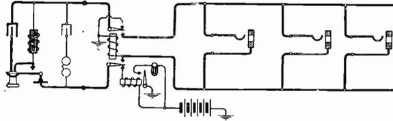
Fig. 192. Two-Wire Line Circuit
