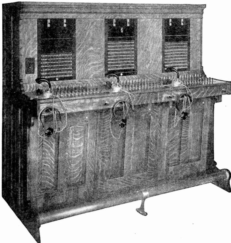
Fig. 177. Three-Position Lamp Board
