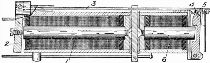
Fig. 110. Electrically Restored Drop
