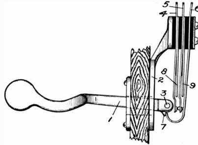
Fig. 76. Short Lever Hook Switch
