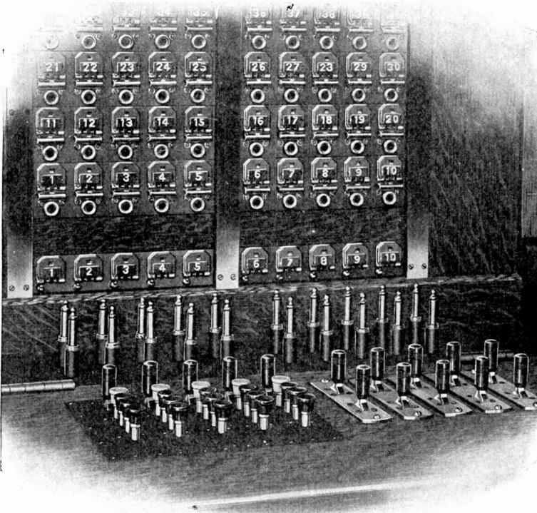
Fig. 144. Details of Drop, Jack, Plug, and Key Arrangement
