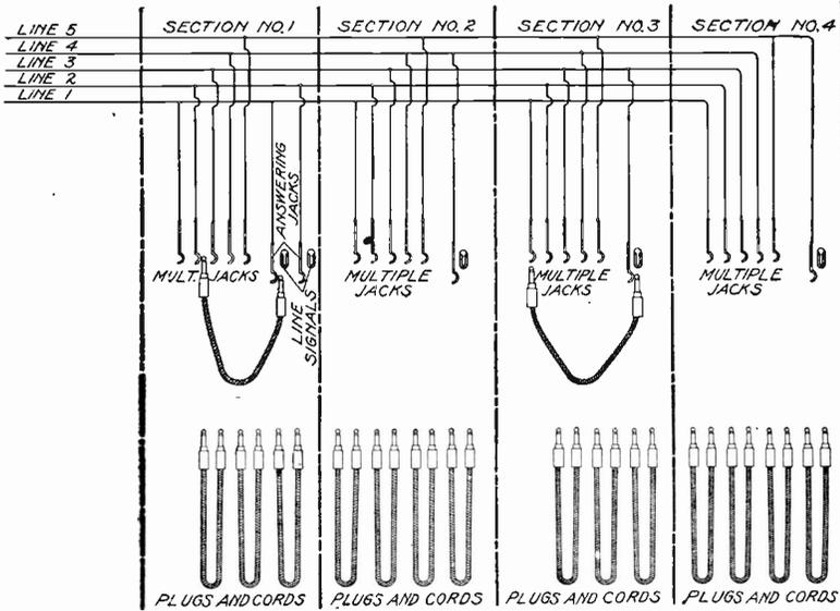
Fig. 178. Principle of Multiple Switchboard
