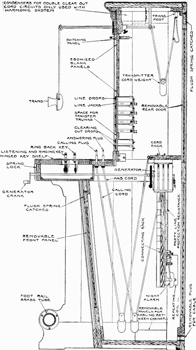
Fig. 145. Cross-Section of Upright Switchboard
