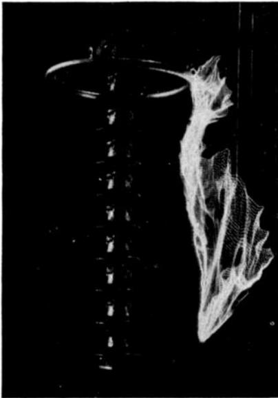
FIG. 401.—High-voltage flashover from arcing ring to arcing rod of suspension-insulator string. (*General Electric Co.*)
