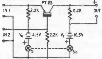
Fig. 825. Single-transistor switching circuit.
