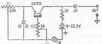
Fig. 813. Multivibrator with single transistor.
