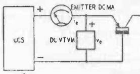
Fig. 907-a. Input resistance measurement.
