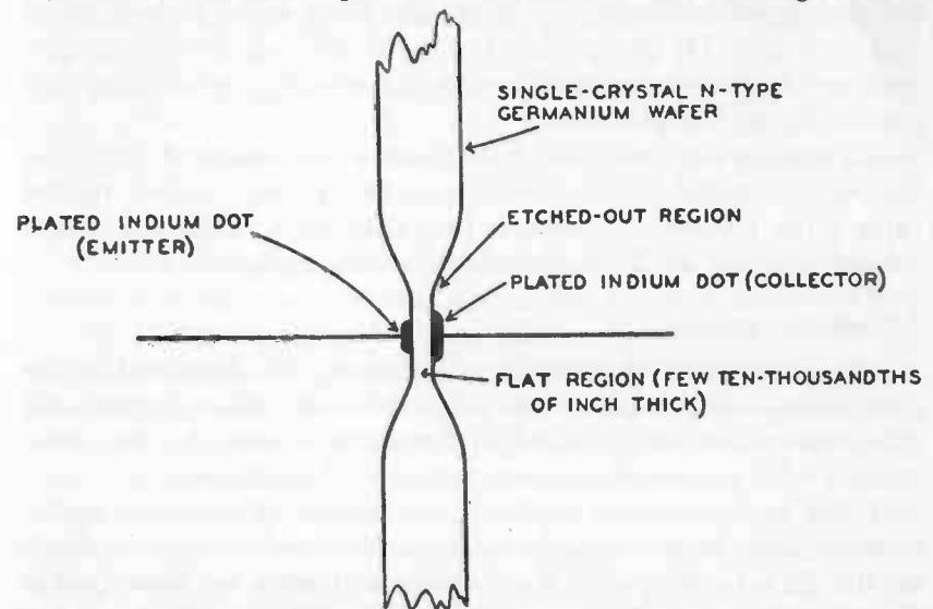
Fig. 207. Detail of surface-barrier transistor cross-section.
