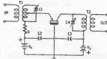
Fig. 413. Single-stage transformer-coupled r.f. amplifier.
