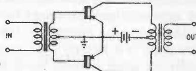
Fig. 407. Conventional push-pull amplifier.
