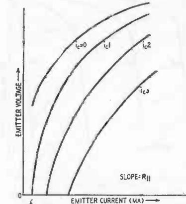
Fig. 902-b. Input characteristic curves.
