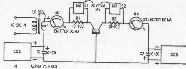
Fig. 912-a. Test circuit for checking alpha.
