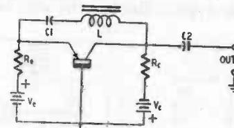
Fig. 503. Series-resonant feed-back oscillator.
