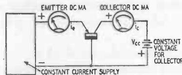
Fig. 908-a. Test circuit for current amplification, alpha.
