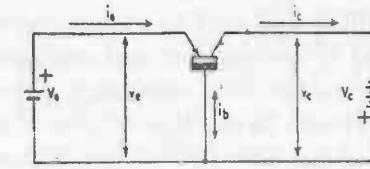
Fig. 211. Basic transistor parameters.
