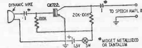
Fig. 803. Subminiature amplifier for inclusion in mobile dynamic microphone.
