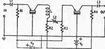
Fig. 416. Series-resonant interstage coupling.
