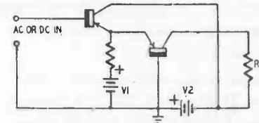
Fig. 412. Direct-coupled amplifier using identical types.
