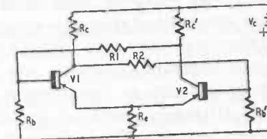
Fig. 707. Basic transistor binary counter.
