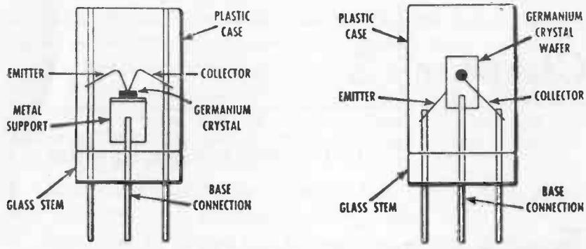
Fig. 201. Essential features of point-contact and junction transistors.
