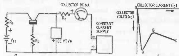
Fig. 914-a, b. Circuit for testing collector negative-resistance characteristics.
