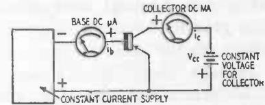
Fig. 908-b. Test circuit for current amplification, beta.
