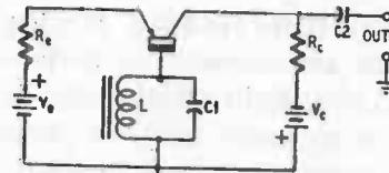
Fig. 501. Base-tuned oscillator.
