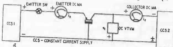
Fig. 903-a. Test circuit for measurement of output characteristics.
