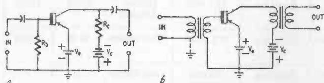
Figs. 402-a, -b. Grounded-emitter single-stage amplifiers.
