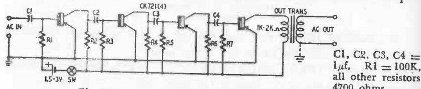
Fig. 804. Cascaded, resistance-coupled a.f. amplifier.
