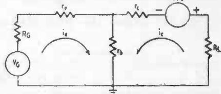
Fig. 302. Grounded-base amplifier and equivalent 3-terminal network.
