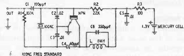
Fig. 506-b. Standard frequency oscillator. (Courtesy, Nat'l. Bureau of Standards).
