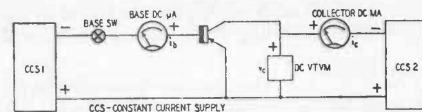
Fig. 906-a. Test circuit for measurement of grounded-emitter output characteristic.
