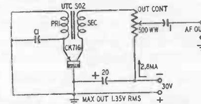
Fig. 809. Audio oscillator-modulator.
