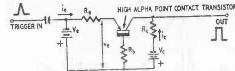
Fig. 701. Basic switching circuit using emitter negative resistance.
