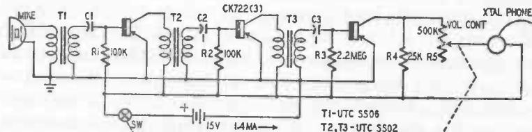
Fig. 807. Simple transistor-type hearing aid. All coupling capacitors can have the same value.
