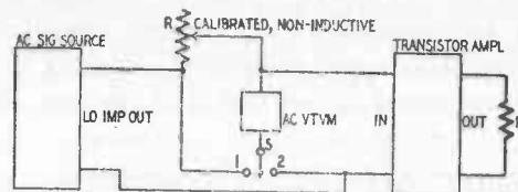
Fig. 910. Circuit for measurement of input impedance.
