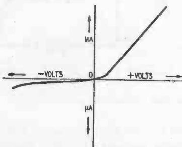
Fig. 106. Static volt-ampere characteristic curve of a typical semiconductor diode.
