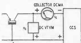
Fig. 907-b. Output resistance measurement.
