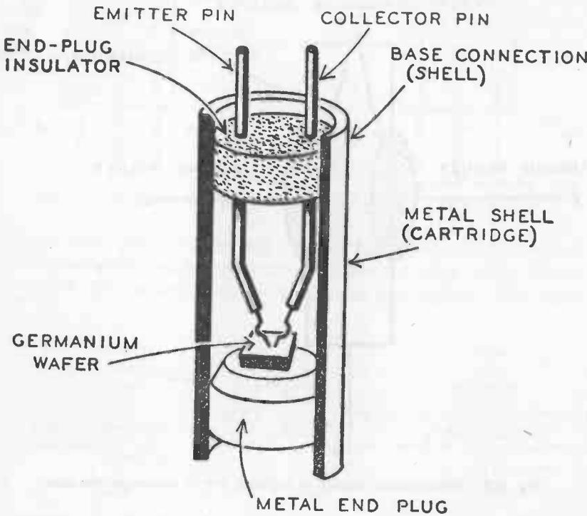
Fig. 204. Cutaway view of point-contact transistor assembly.
