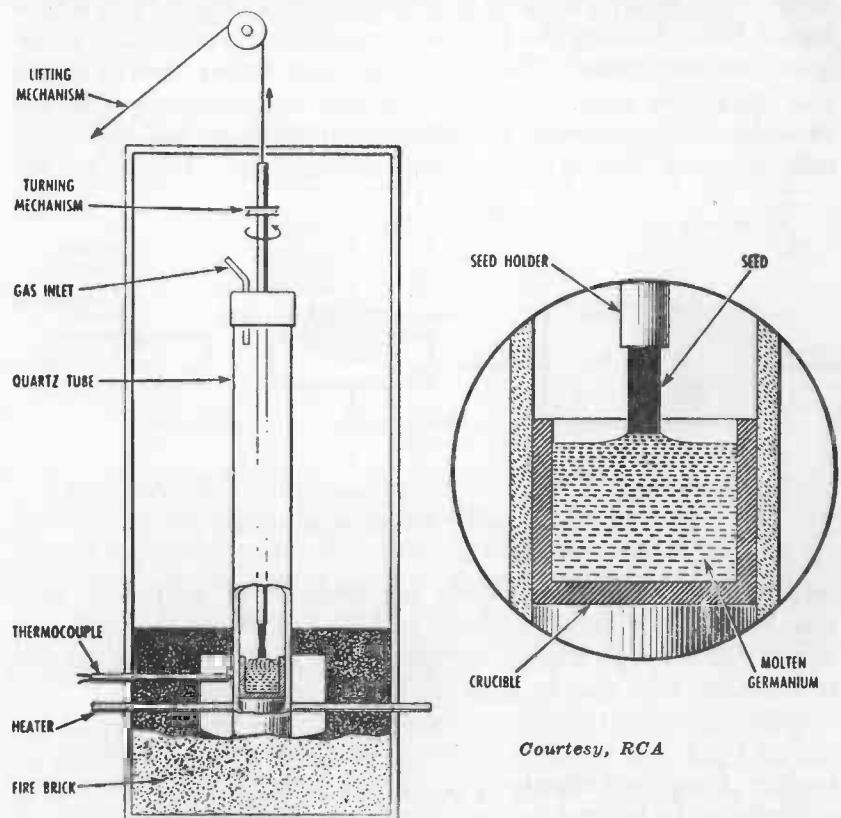
Fig. 103. One type of apparatus for growing single crystals. Rotated seed is slowly withdrawn. Inset shows early stage as the crystal starts to form.
