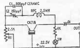
Fig. 815. Self-excited 100-kc frequency standard.
