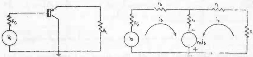
Fig. 304. Grounded-collector amplifier and its equivalent network.
