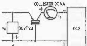
Fig. 907-c. Feedback resistance measurement.
