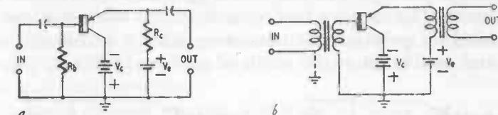
Figs. 403-a, -b. Grounded-collector single stage amplifiers.
