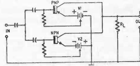
Fig. 408. Push-pull amplifier using complementary symmetry principle.
