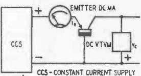
Fig. 907-d. Forward resistance measurement.
