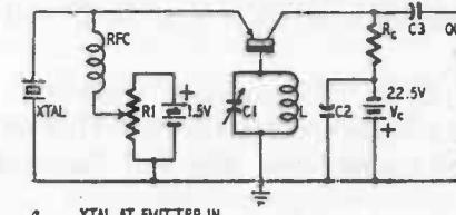
Fig. 506-a. Crystal at emitter-input.
