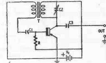
Fig. 502-b. Grounded-emitter tickler-type oscillator.
