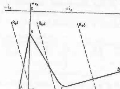
Fig. 703. Emitter negative-resistance characteristic with single operating points.
