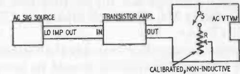
Fig. 911. Circuit for measurement of output impedance.
