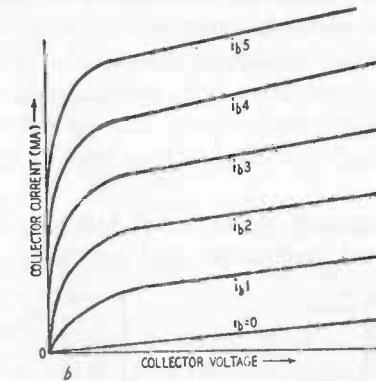
Fig. 906-b. Output characteristic curves of grounded-emitter.
