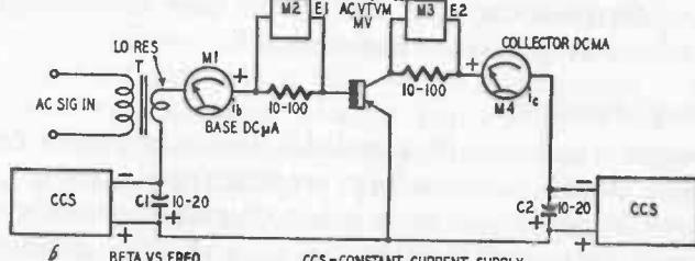
Fig. 912-b. Test circuit for checking base-to-collector current amplification.
