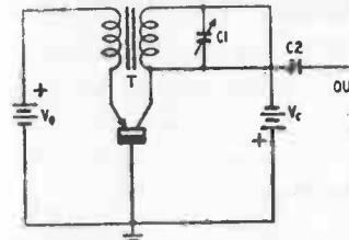
Fig. 502-a. Grounded-base tickler-type oscillator.
