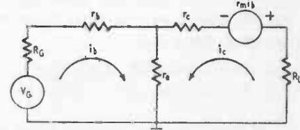
Fig. 303. Grounded-emitter amplifier and its equivalent network.
