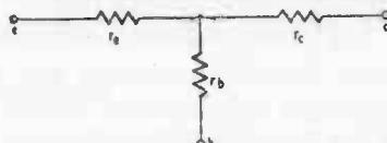
Fig. 212. Simplified equivalent 3-terminal resistance network of transistor.
