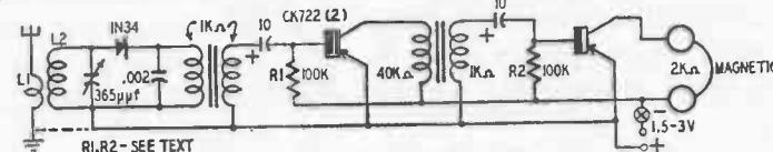
Fig. 818. Diode-type broadcast receiver with transistor a.f. amplifier.
