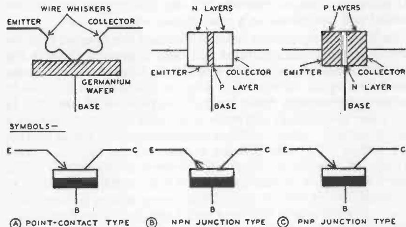
Fig. 202. Point-contact and junction type transistor triodes.
