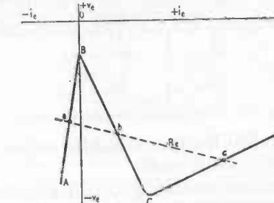
Fig. 704. Emitter negative-resistance characteristic with multiple operating points.
