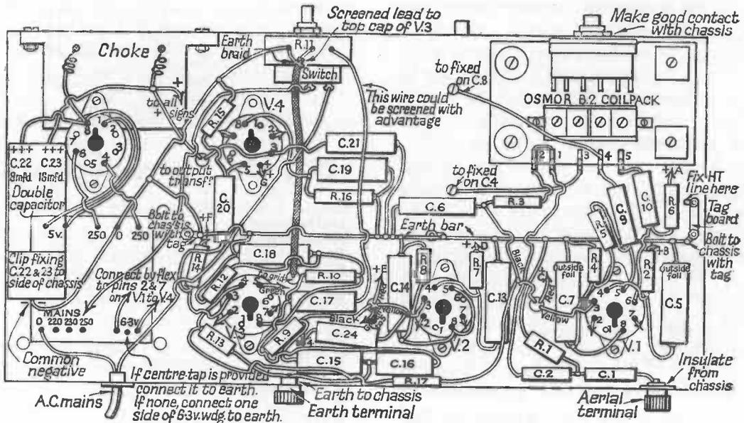
Fig. 28B Superhet Wiring Diagram
