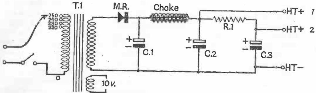
Fig. 16 Mains HT Unit. Theoretical Circuit
