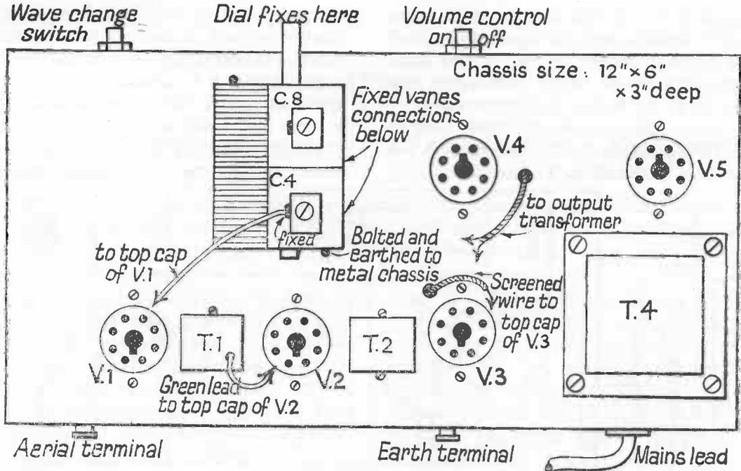
Fig. 28A Superhet Wiring. Top of Chassis
