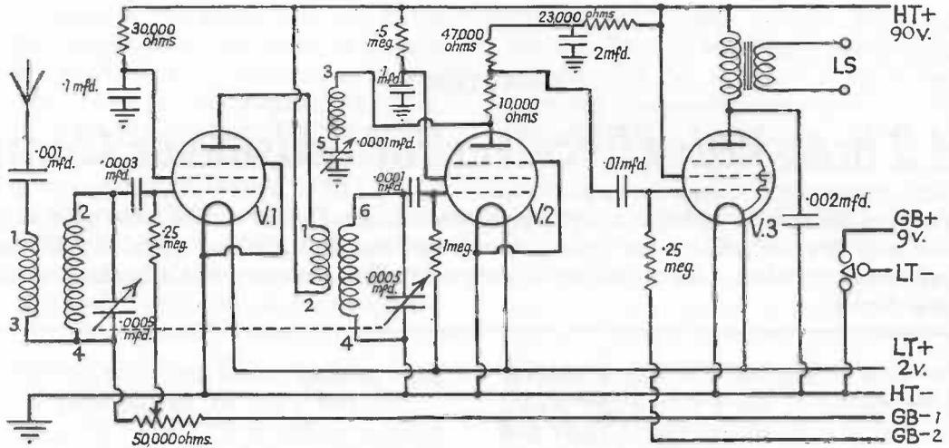
Fig. 11 Three-Valve Battery Receiver. Theoretical Diagram
