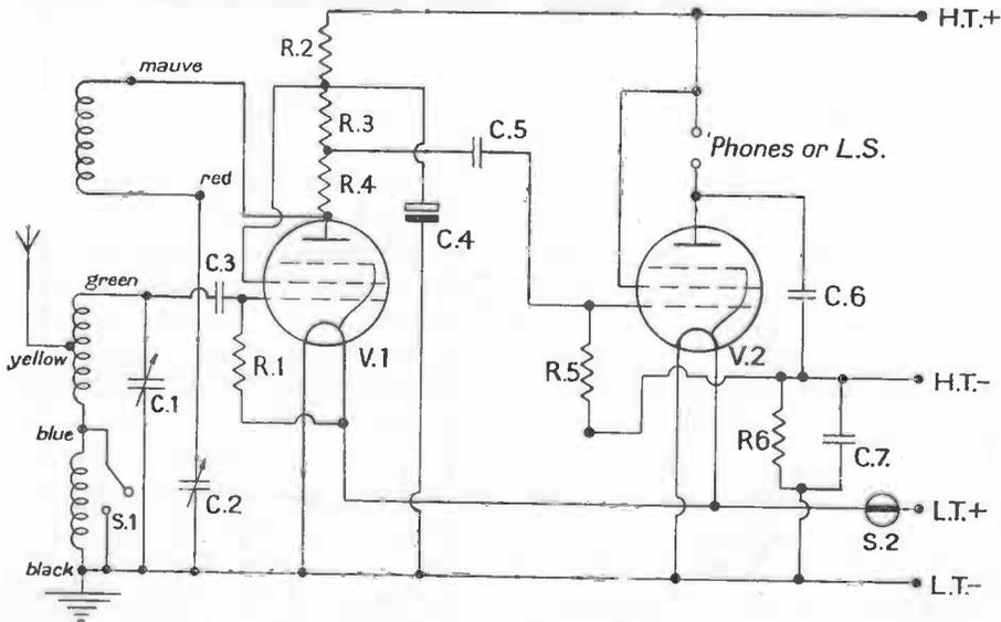
Fig. 9 Battery Two-valve Receiver
