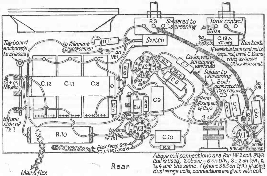
Fig. 22A Underside of Chassis
