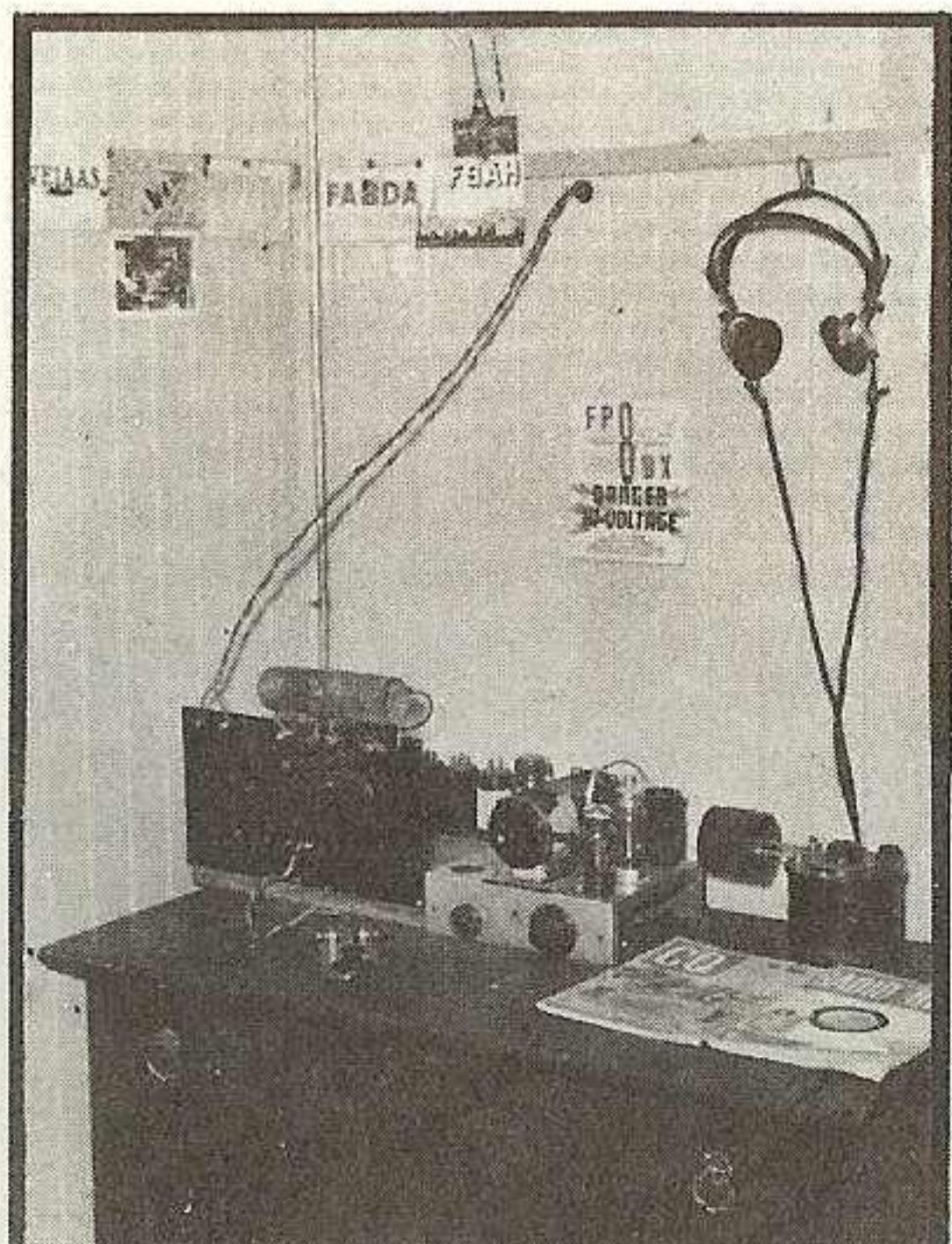
Many overseas amateurs do not enjoy radio parts, kits and equipment that is easily obtainable in W-land. Completely home built equipment is the rule, as shown in this photo of ex-FP8BX. Note the home-made coils on the transmitter at the left. Running but ten watts, FP8BX worked many DX stations in all parts of the world. What can you do with 75 watts? Try your hand at DX!
