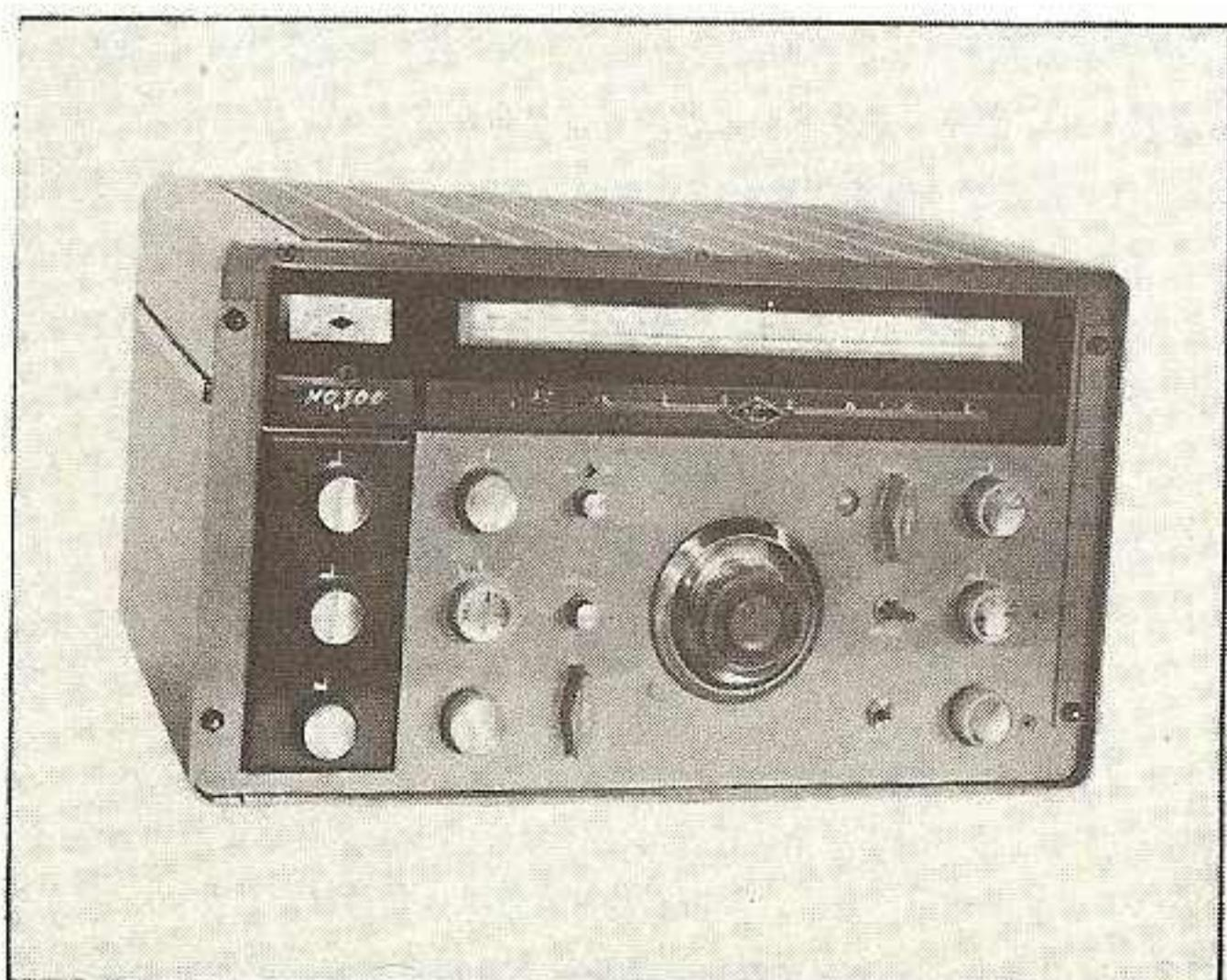
Fig. 6 Incorporating many of the special features required for serious amateur reception is the double conversion, 12 tube National NC-300 receiver. Converters are used to extend the tuning range of the set above 420 mc.
