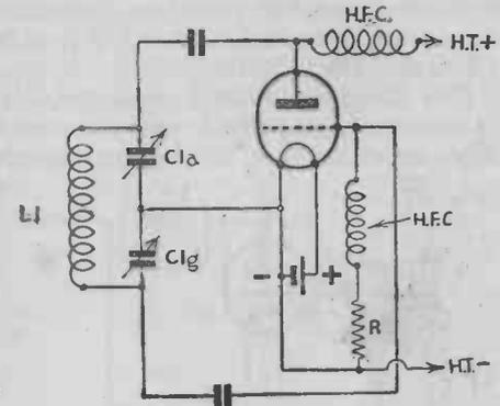
Fig. 28.—The Colpitts circuit.
