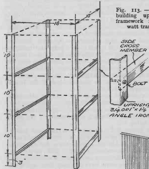
Fig. 113. — Method of building up the rack framework for the 10-watt transmitter.
