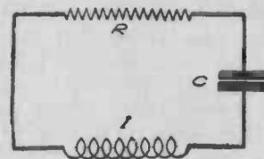
Fig. 75.—Theoretical representation of an artificial aerial system.
