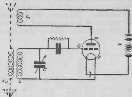
Fig. 25.—The simplest valve oscillator circuit.
