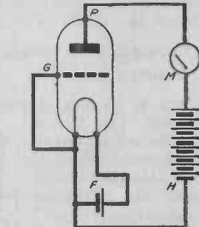
Fig. 11.—The complete circuit of a triode to show the flow of current.
