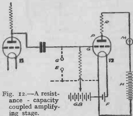
Fig. 12.—A resistance-capacity coupled amplifying stage.
