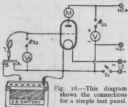
Fig. 16.—This diagram shows the connections for a simple test panel.
