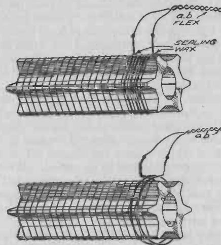
Figs. 78 and 79.—Alternative methods of affixing a coupling coil to the tank cell.
