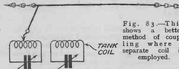
Fig. 83.—This shows a better method of coupling where a separate coil is employed.
