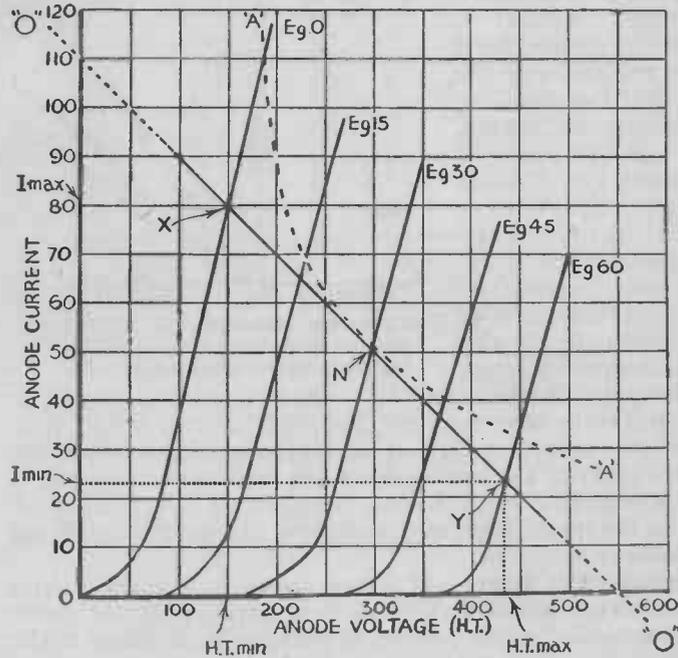
Fig. 18.—Dynamic curve, showing load line, dissipation, and other important working data.
