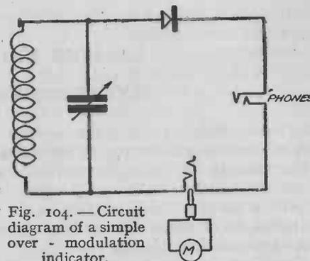
Fig. 104.—Circuit diagram of a simple over-modulation indicator.
