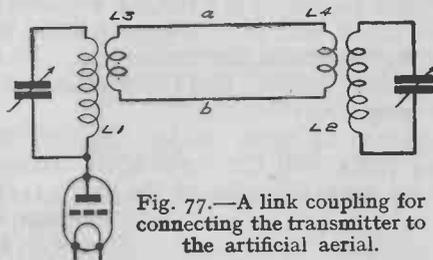
Fig. 77.—A link coupling for connecting the transmitter to the artificial aerial.
