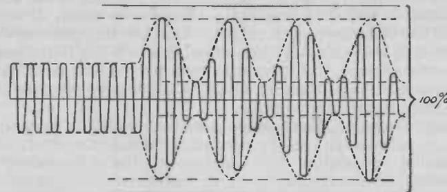
Fig. 49.—Showing the effects of modulation lower than 100%.
