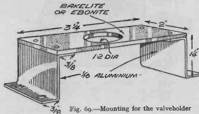
Fig. 69.—Mounting for the valveholder
