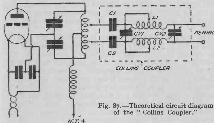
Fig. 87.—Theoretical circuit diagram of the "Collins Coupler."
