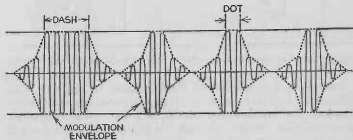
Fig. 60.—Diagram showing the effect of the letter "B" in modulating carrier.
