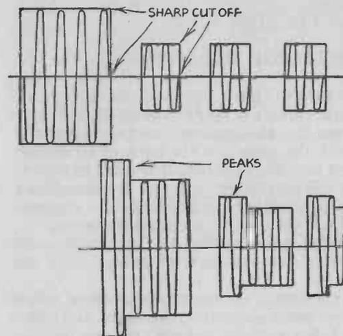
Fig. 61 (left).—In some arrangements a sharp cut-off will be obtained, whilst if poor regulation of the H.T. supply is provided, peaks will be produced as shown in Fig. 62 immediately below.
