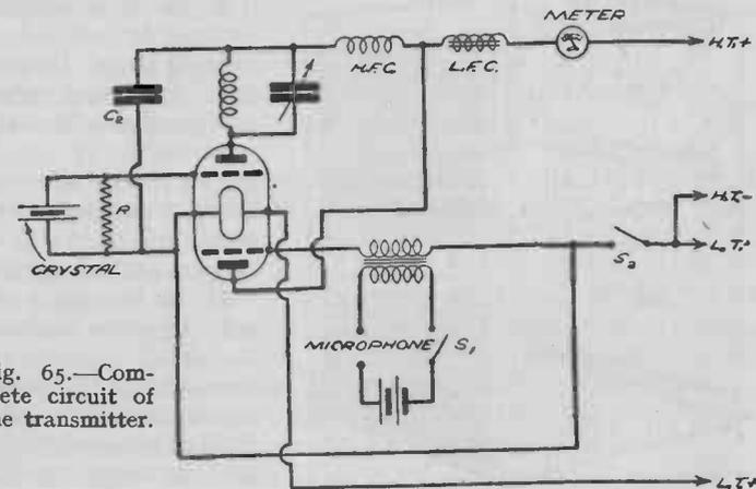
Fig. 65.—Complete circuit of the transmitter.
