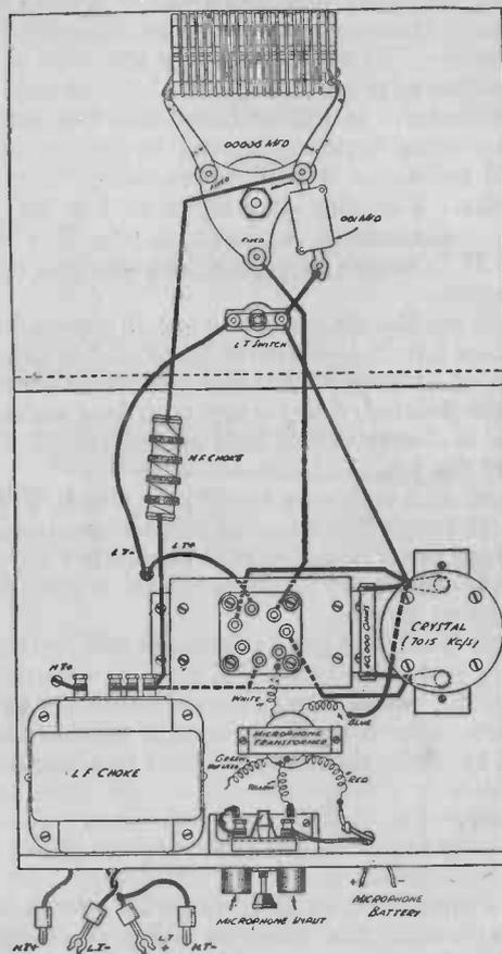
Fig. 70A.—Wiring plan of the theoretical circuit shown in Fig. 65.
