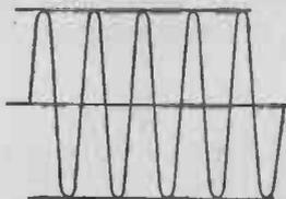
Fig. 59.—Diagrammatic representation of an unmodulated carrier wave.
