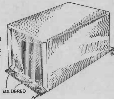
Fig. 118.—The finished metal cover and (below) developed blank for making the cover for the mains unit.
