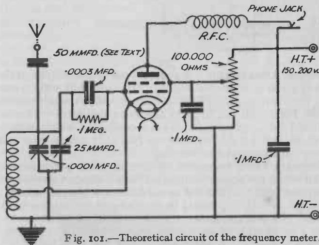
Fig. 101.—Theoretical circuit of the frequency meter.
