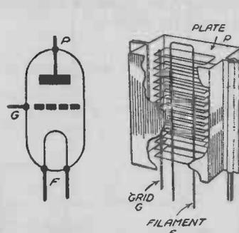
Figs. 9 and 10.—Theoretical and practical assembly of the triode valve.
