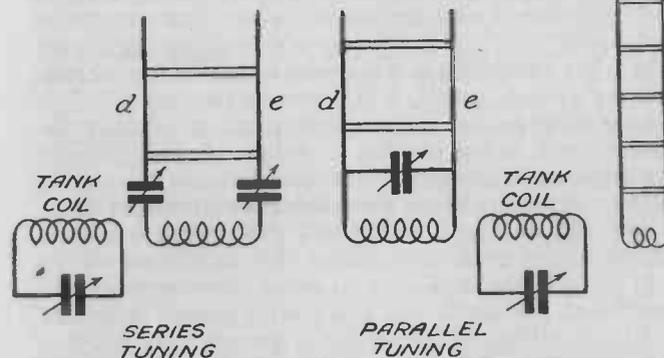
Fig. 86.—Two methods of coupling parallel feeders to the transmitter.
