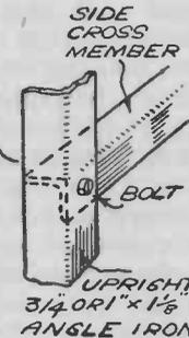
Fig. 114. — Detail showing method of fitting the back of the cabinet.
