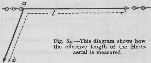
Fig. 84.—This diagram shows how the effective length of the Hertz aerial is measured.
