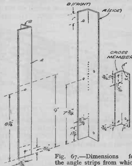
Fig. 67.—Dimensions for the angle strips from which the cabinet framework is made.
