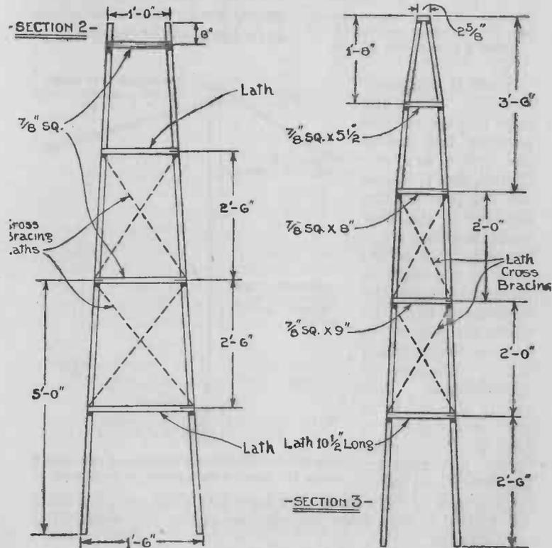
Fig. 93.—Showing the dimensions for building the second (middle) section of the mast.
