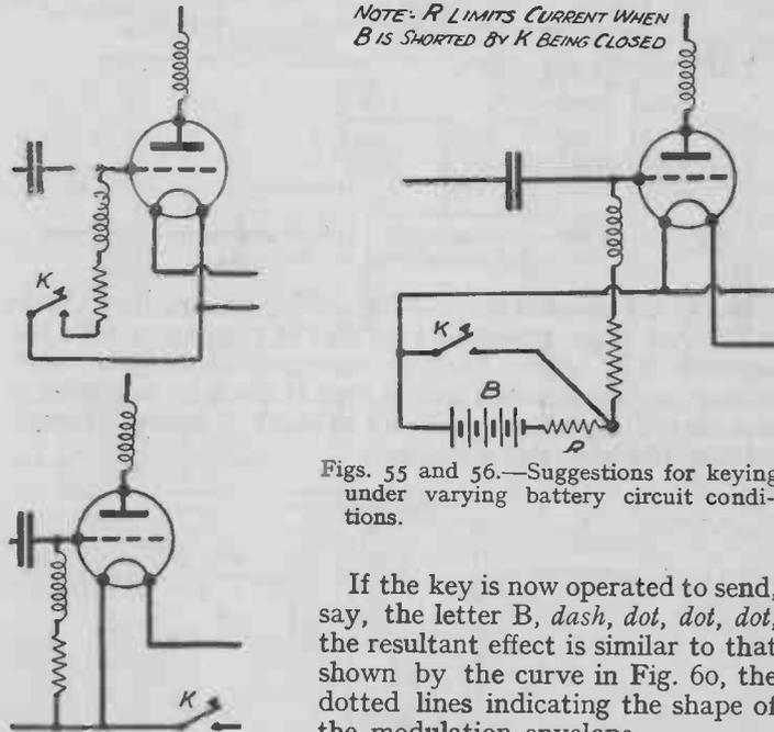
Figs. 55 and 56.—Suggestions for keying under varying battery circuit conditions.
