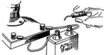
Fig. 82.—Measuring resistances by the flash method.
