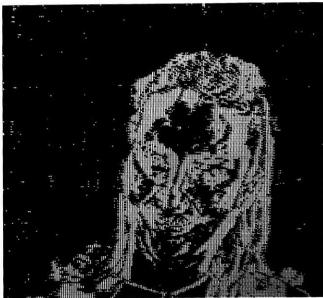
Fig. 4—A display of dots marking elements that have changed in a frame during very active motion: about 12,000 changes occurred in this frame. The picture is that shown in Fig. 1.
